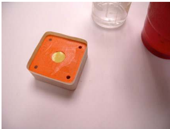
Figure 8-38. Mix the casting material gently and pour slowly to help prevent unwanted bubbles.
