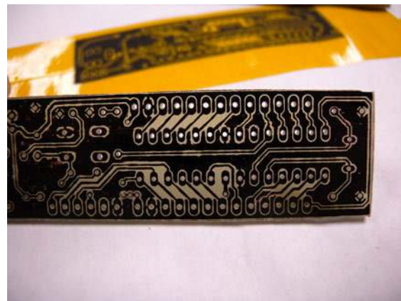
Figure 5-34. The toner-transfer project.
