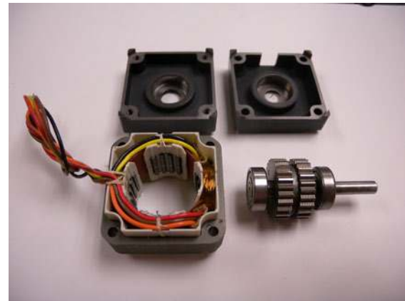
Figure 7-10. A stepper motor has a multi-toothed rotor that is pulled in line with a series of coils.
