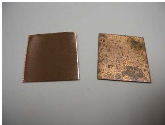
Figure 8-8. You should have two pieces of copper to complete the cell, one with cuprous oxide and one without.
