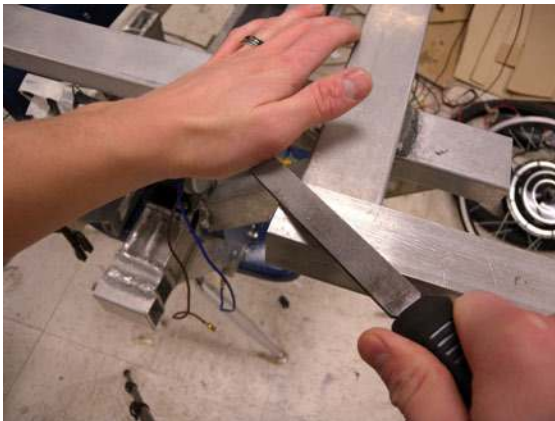
Figure 2-50. Use one hand to push the handle and the other to guide the file.
