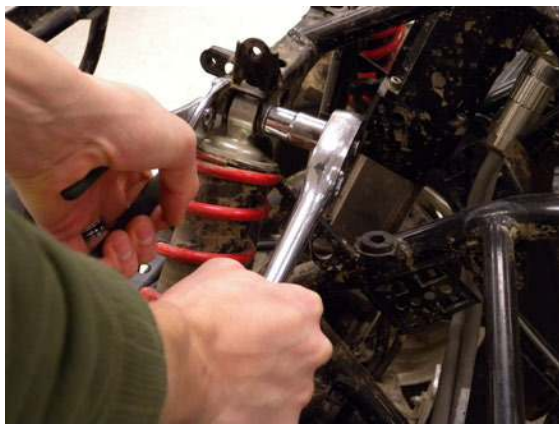
Figure 2-13. If a second wrench is not available to remove a fastener, use a pair of pliers to hold the fastener stationary while twisting only the wrench.
