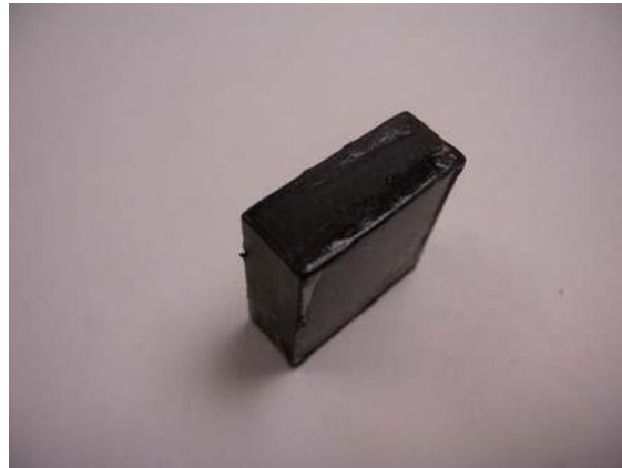
Figure 6-20. Making multiple passes results in reduced edge quality. If possible, refocus the laser to the depth of the first cut before making the second.
