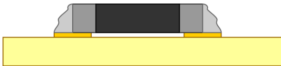
Figure 4-34. SMD with a cold solder joint.
