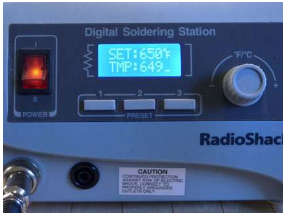
Figure 4-6. The tip temperature is set by dialing in the desired temperature.
