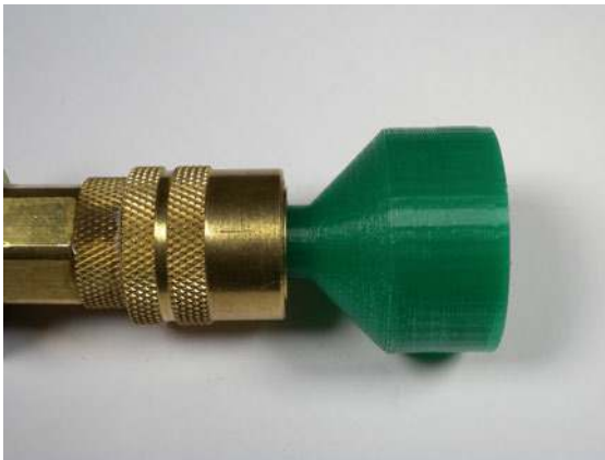
Figure 8-17. Test fit the nozzle after printing. It should be snug enough to make a seal but loose enough to pop out of the connector when released.
