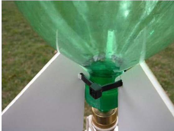
Figure 8-18. Securing the fins.
