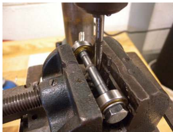
Figure 7-47. Hobbing with a drill press.
