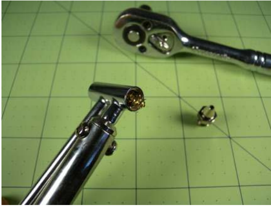
Figure 4-59. Ensure that the brass wool does not clog the air inlet.
