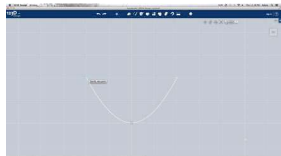
Figure 8-47. The spline tool produces a Bezier curve between two points and works well for reproducing parabolas.
