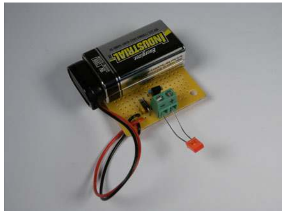
Figure 4-29. The LED tester project.
