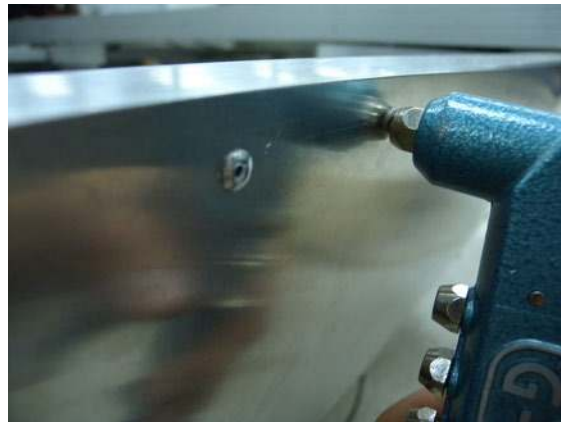
Figure 3-26. Firmly press the rivet against the material when compressed to ensure a tight joint.
