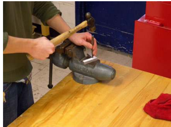
Figure 2-35. Hold the hammer at the end of the handle and hit the workpiece squarely.
