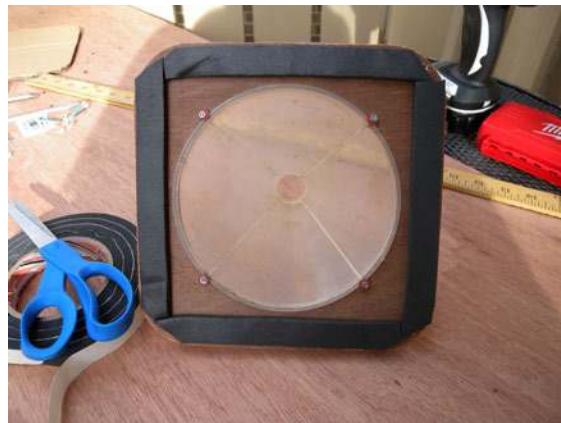
Figure 1-15. Attach foam tape to the back of the plywood plate to prevent any air leaks.
