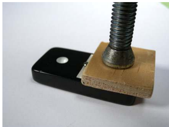
Figure 3-4. Place a piece of wood between the clamp and your material to prevent damage.
