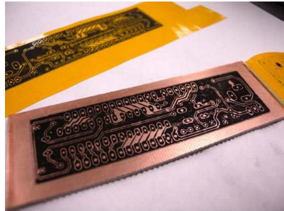
Figure 5-35. Make sure your resolution is 600 DPI or greater and the quality is set to maximum. This will help deposit the most amount of toner possible.
