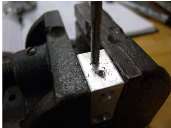
Figure 2-37. Ensure that you use a properly sized hole is used for tapping. This reduces the chance of the tap breaking off or forming poor-quality threads.
