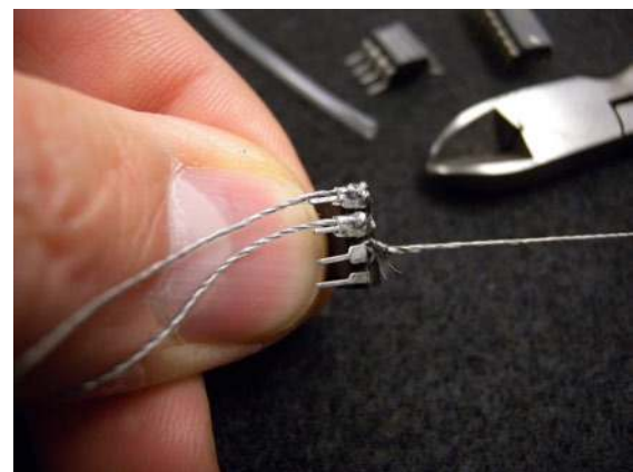
Figure 5-24. Prepare each leg prior to inserting the IC into the fabric using a two half-hitch knot followed by a small piece of heat-shrink tubing.
