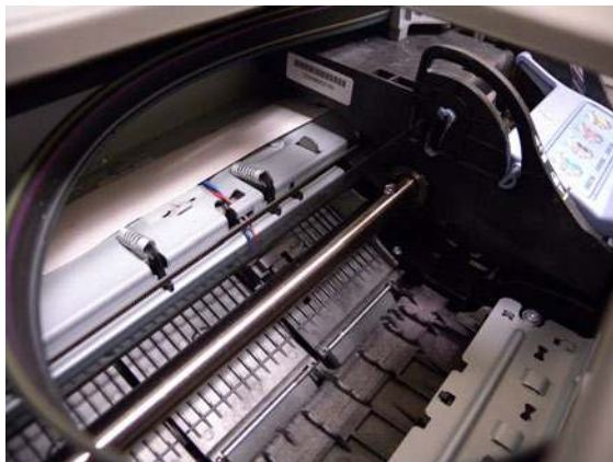
Figure 7-17. Linear rod in an inkjet printer.
