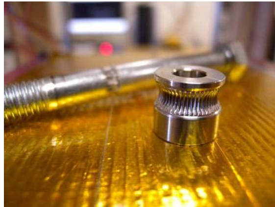
Figure 7-35. Machined feed wheels provide better consistency but at a higher price.
