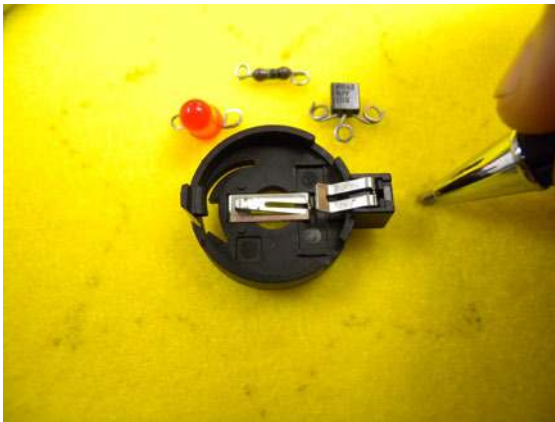
Figure 5-33. Draw an outline around your parts to ensure you have enough room.
