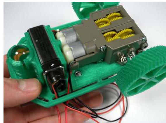
Figure 8-20. Attach the gearbox.
