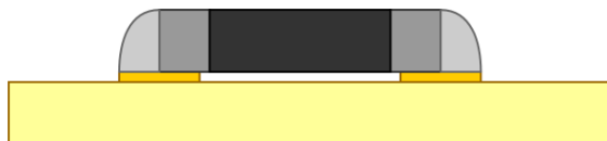
Figure 4-37. SMD with too much solder.
