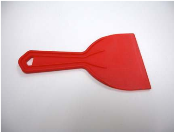
Figure 4-51. Plastic putty knives used for spackling work well for spreading solder paste. Try a few different types (plastic, rubber, and metal) and decide which works best for you.
