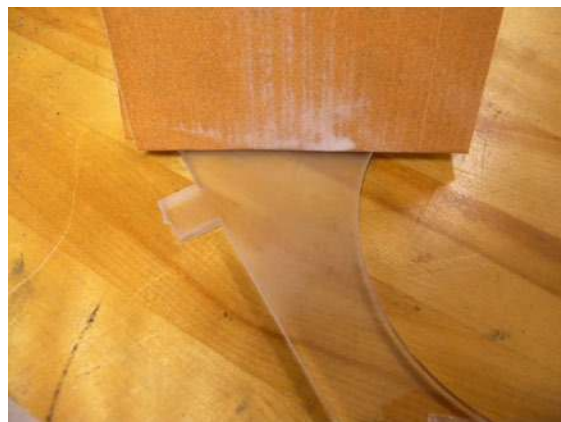
Figure 2-55. Sand in a circular pattern to create an evenly sanded surface.
