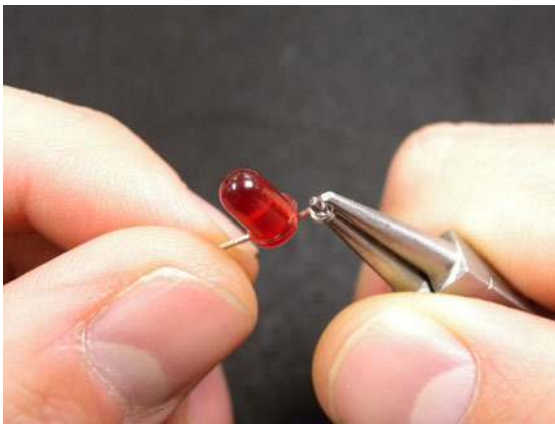
Figure 5-16. Use a pair of needle-nose pliers to wrap a small length of lead into a coil.
