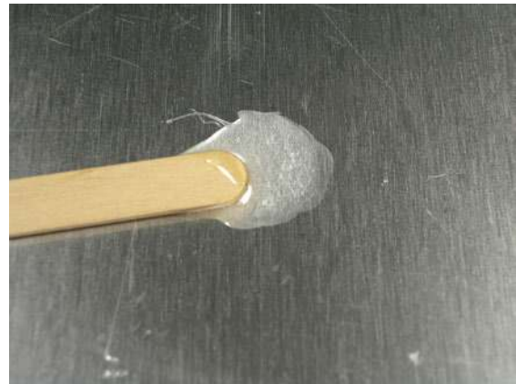
Figure 3-20. Mix epoxy until the resin and hardener have fully combined.
