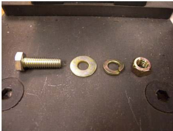
Figure 3-32. Use a washer between the head and the nut to help prevent the fastener from loosening due to flexing and vibration.
