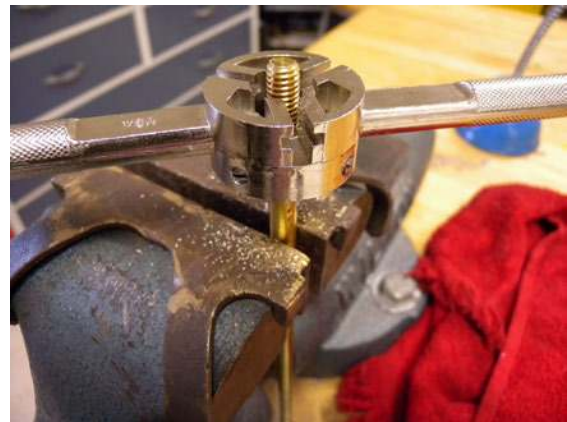
Figure 2-40. Make sure a properly sized shaft is used for thread cutting. This reduces the chance of the die's teeth breaking off or forming poor quality threads.
