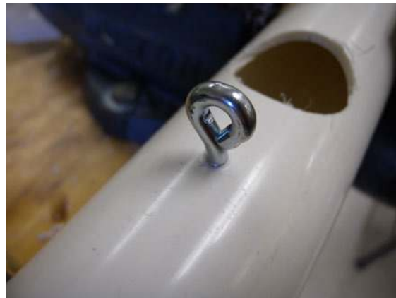
Figure 8-15. Drilling a hole in the side of the PVC pipe will allow for the air hose to pass through.
