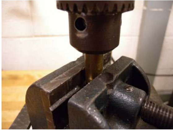
Figure 2-97. Center material in the vise by using the chuck as an alignment tool.
