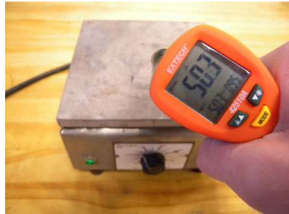
Figure 2-101. Thermostats are often inaccurate, so use an infrared thermometer to read the surface temperature.
