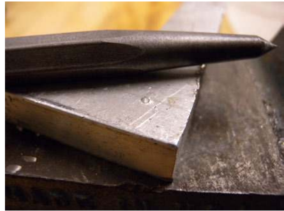
Figure 2-57. Hit a center punch only once to prevent it from jumping.
