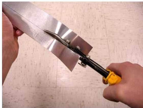
Figure 2-15. Use the appropriately colored shear that matches the direction of the cut.
