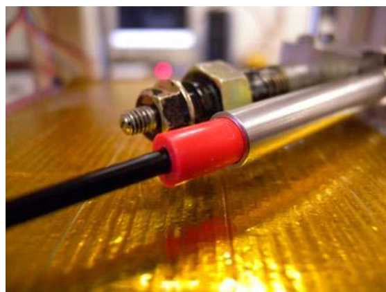
Figure 7-38. PTFE is used inside of the heater barrel due to its low friction coefficient and high heat tolerance.
