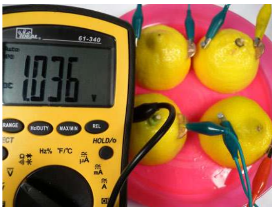
Figure 8-5. Configuring multiple lemon batteries in series and in parallel changes the amount of available voltage and current.
