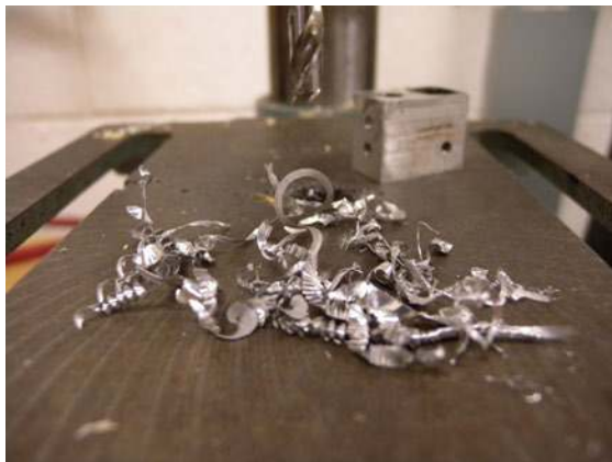
Figure 2-64. When properly used, a drill bit will eject the cut material in long spirals.
