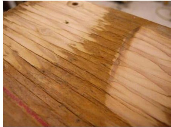
Figure 2-87. Power sanders have the ability to remove a lot of material quickly. Take care to move the tool constantly to preventing pitting the workpiece.
