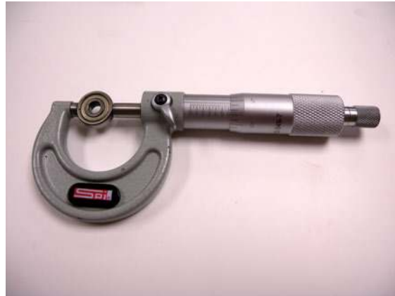
Figure 3-54. Use the ratchet to ensure proper pressure and accurate measurement.
