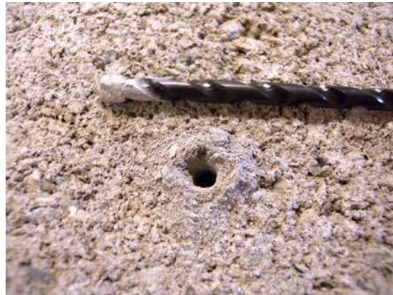
Figure 2-79. The pounding action of the hammer drill helps to break apart hard masonry.
