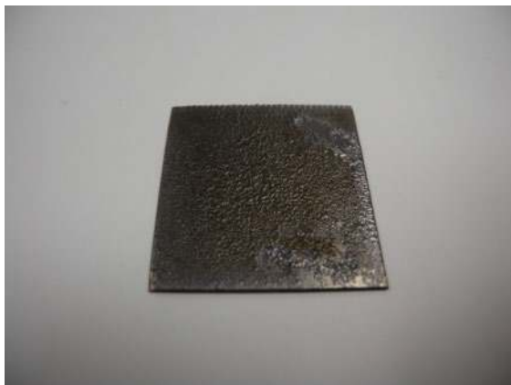
Figure 8-7. As the copper is heated, a rainbow of cuprous oxide forms, followed by a layer of dark cupric oxide.
