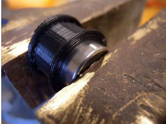
Figure 7-9. You can use a vise to press the bearings into their seats.
