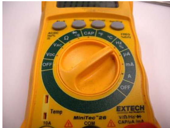
Figure 3-56. Use the multimeter's dial to select the desired tool and measurement range.
