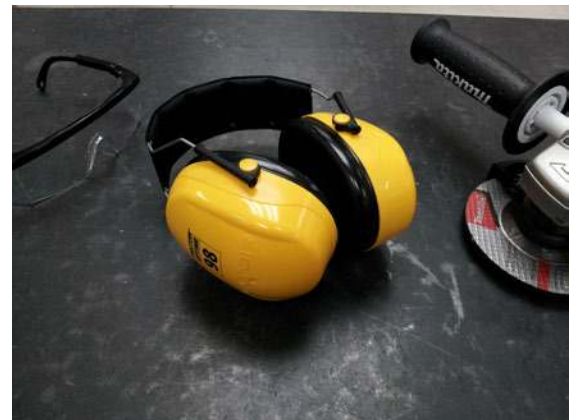
Figure 1-5. Ear protection should always be worn when working in a loud environment.
