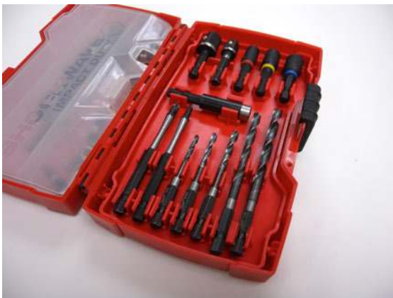
Figure 2-81. Use only bits and sockets that are designed for impact driving; normal bits will crack under the load.
