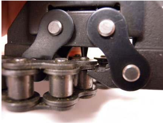
Figure 2-59. Be careful to align the punch over the pin because the punch can produce enough force to bend the links if not properly aligned.
