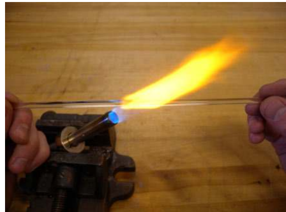
Figure 8-10. Roll the rod in the flame until it begins to wilt and then carefully pull it into a 1 mm filament.
