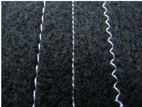
Figure 2-89. The most common stitch types are the basting stitch , used as a temporary stitch; the straight stitch , which is universal; the zig-zag stitch , used to finish edges with stretch fabrics and to attach patches.
