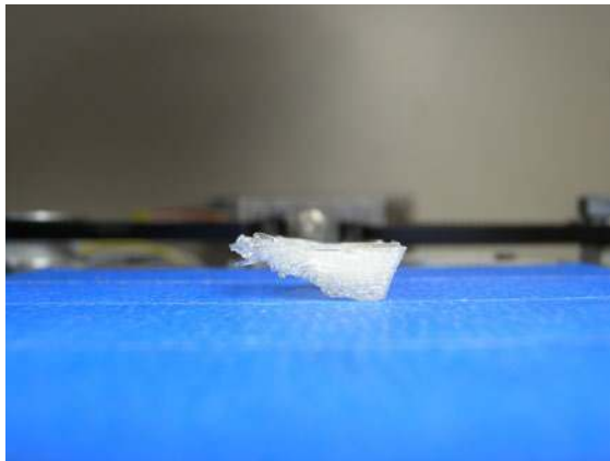
Figure 7-1. Unless you use support material, a 3D printer cannot print overhangs greater than 45 degrees.
