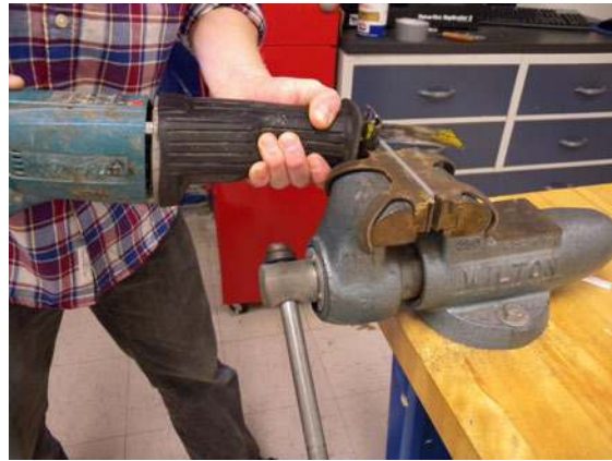
Figure 2-85. Ensure that the saw's foot is pressed firmly against the material and the saw is not in line with your body.
