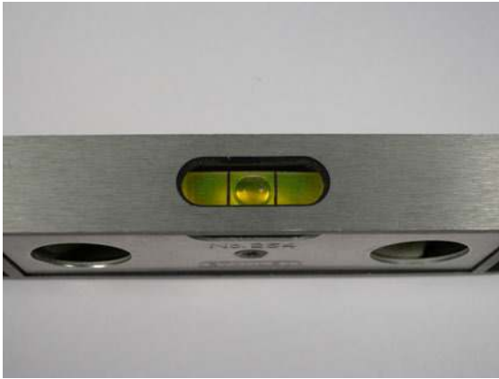
Figure 3-41. A level indicates a level surface when the bubble is positioned between the vial's indicator lines.
