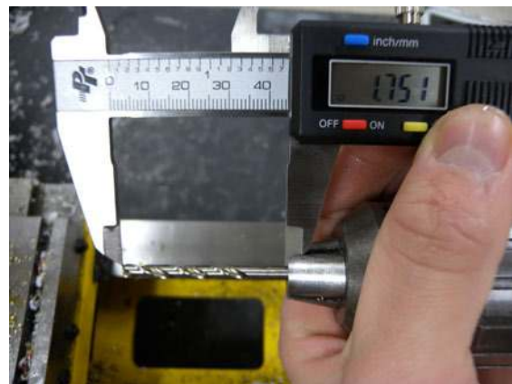
Figure 3-51. Always calibrate (zero out) a caliper prior to use and use the appropriate measurement feature.
