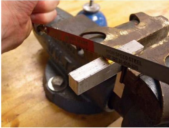
Figure 2-46. Use cutting oil whenever you saw metal.
