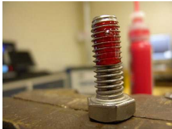
Figure 3-22. Always clean the threads of the fastener prior to applying thread-lock.
