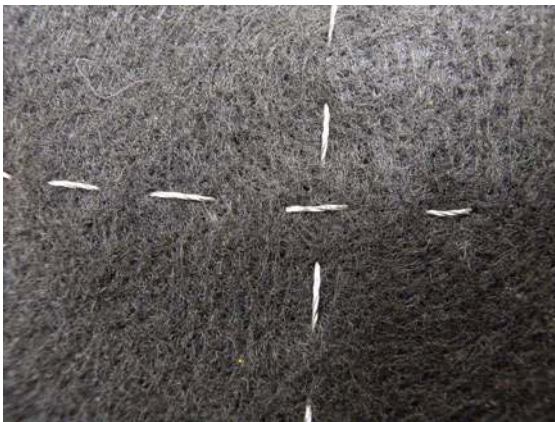
Figure 5-28. Overlapping stitches without letting them touch allows for you to create much more complicated designs without the risk of shorting out the connection.
