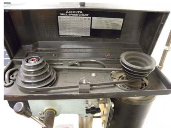
Figure 2-96. Always adjust the spindle speed appropriately for the material and secure your work to the drill press's table prior to drilling.
