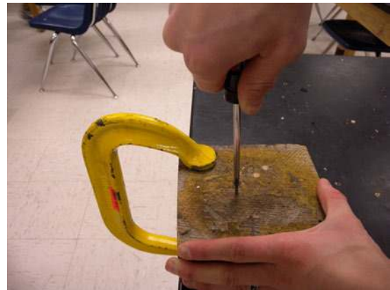
Figure 2-7. Apply downward pressure on the fastener when driving and removing fasteners with a screwdriver.
