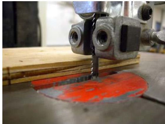
Figure 2-93. Lower the blade guide until it is just above the workpiece.
