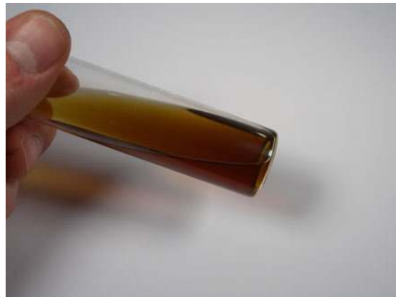
Figure 4-19. Adjust the alcohol-to-rosin ratio until the desired viscosity is achieved.
