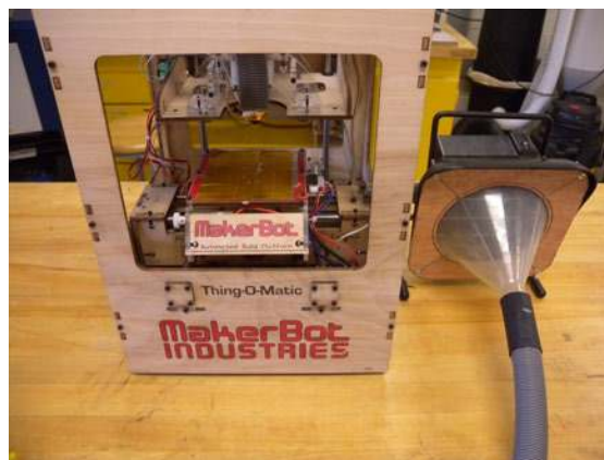
Figure 1-12. Soldering fume extractors can be used for ventilating the 3D printer when printing materials like ABS.
