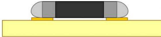
Figure 4-36. SMD with too little solder.
