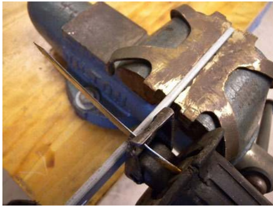
Figure 3-7. When cutting material, cut as close to the vise as possible to prevent vibration.
