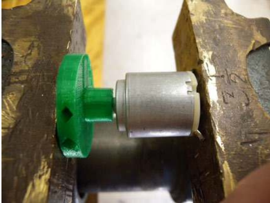
Figure 8-28. Use a vise rather than a hammer to attach the hub to the motor because the blows of a hammer will damage the motor's internal components.
