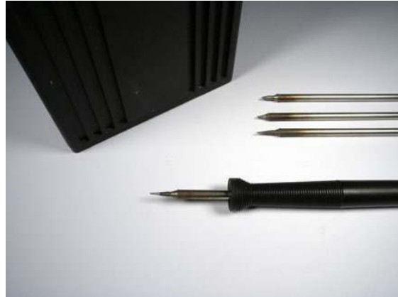
Figure 4-7. Induction-based soldering irons.
