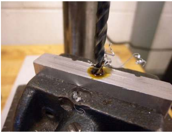
Figure 2-71. When drilling metal, use plenty of cutting oil and clear the chips often to prevent the bit from overheating.
