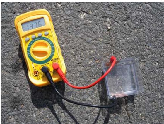
Figure 8-6. Measuring the output of the solar cell.
