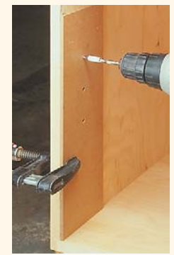
▲ A hardboard template allows you to accurately drill holes for the shelf pins.
