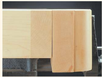
▲ The top edges of the jaws tilt in slightly to counteract the forces of clamping that tend to drive the top edges apart.
