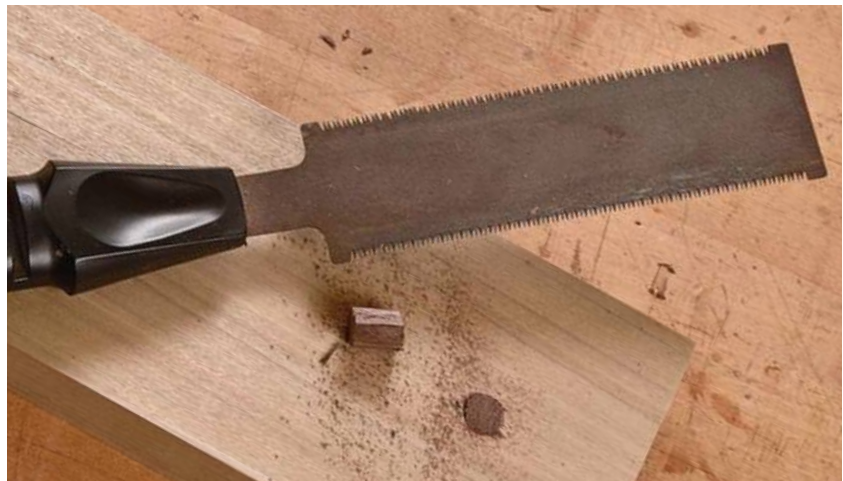
A flush-trim saw is “set” only to one side to avoid scratching the surface.
