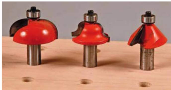
Profile bits cut moldings, table edges, and other decorative shapes.
