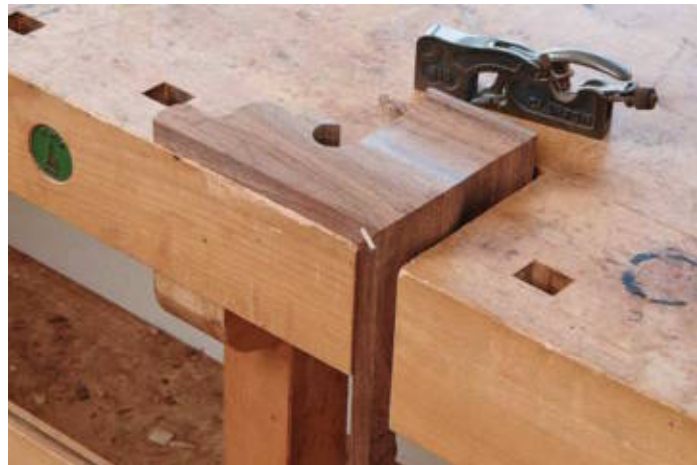
A tail vise positions work 90 degrees from a face vise.
