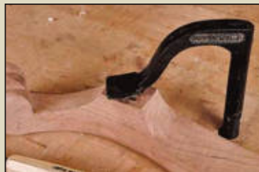
A traditional holdfast fits within a hole in the benchtop.
