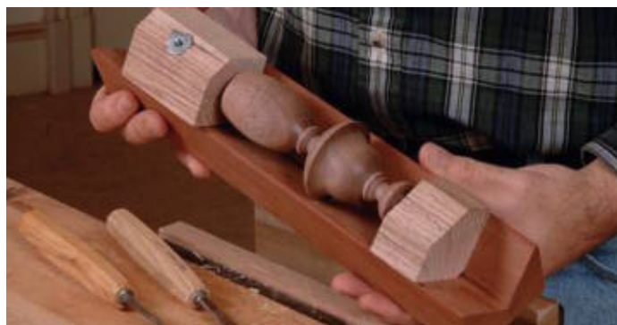
Some work, such as this finial, may require construction of a fixture.
