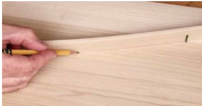
To mark free-form curves, try flexing a thin stick between brads.
