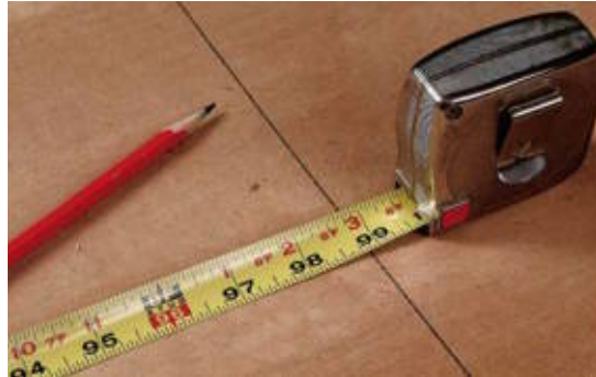
The steel tape is a great choice for measuring long lengths of lumber.
