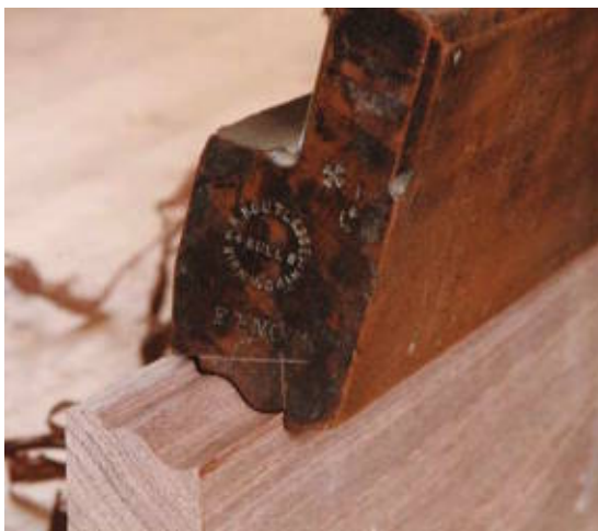
Molding planes create profiles with a hand-made look.
