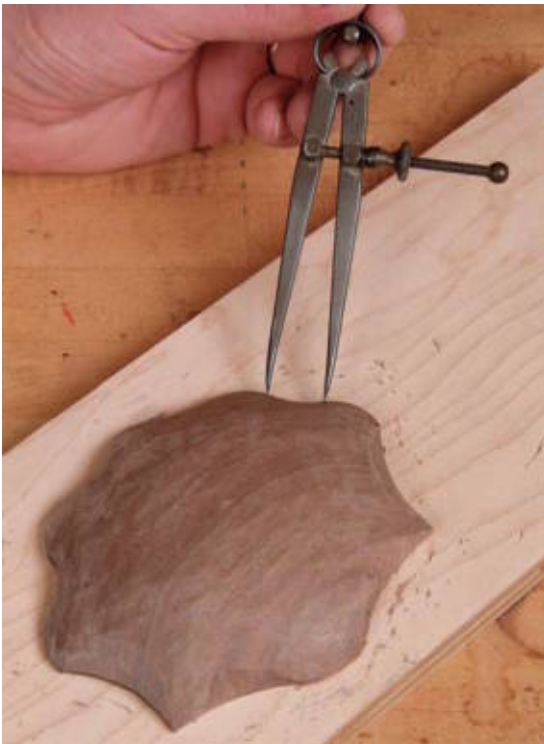
Dividers measure and allow you to transfer points on irregular shapes, such as carvings.
