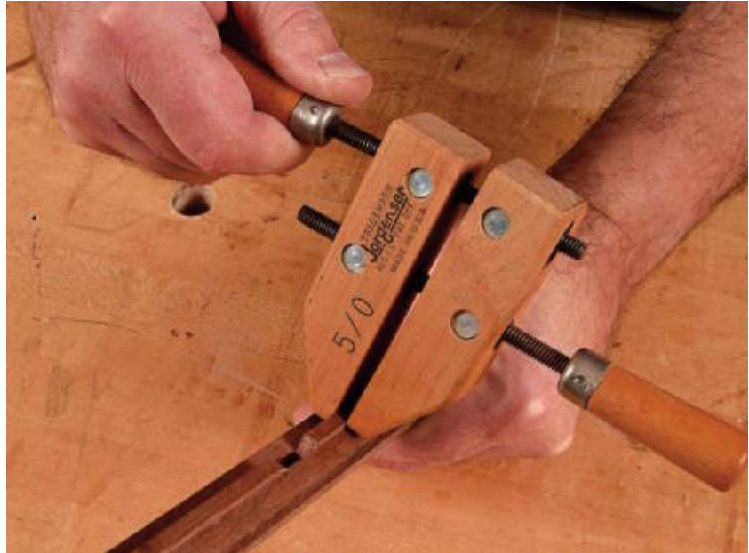
The handscrew clamp has jaws that adjust for various angles.
