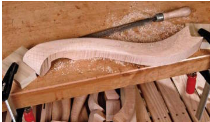
To hold odd-shaped work such as this chair arm, cut blocks that conform to the shape of the workpiece.
