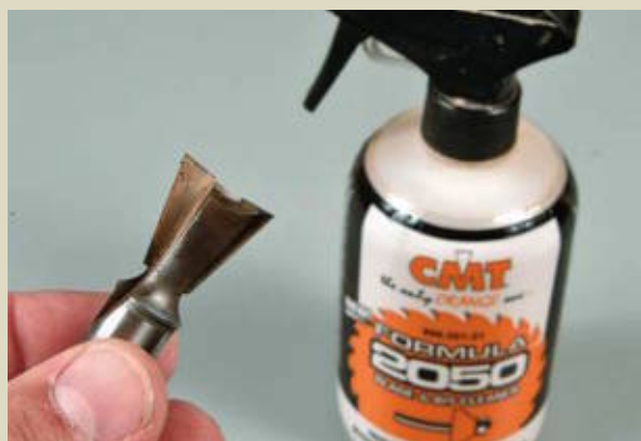
Use a liquid cleaner to break down stubborn buildup on bits and collets.
