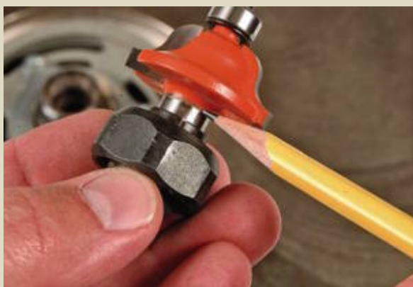
Don't allow bits to bottom out in the collet.
