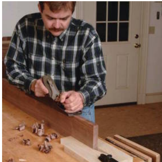
This bench hook grips long stock for truing an edge.
