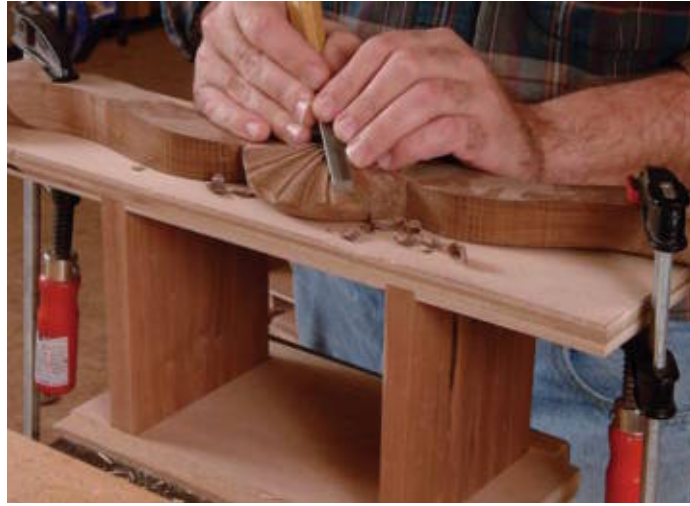
This simple box raises carvings and other detailed work to a comfortable height.
