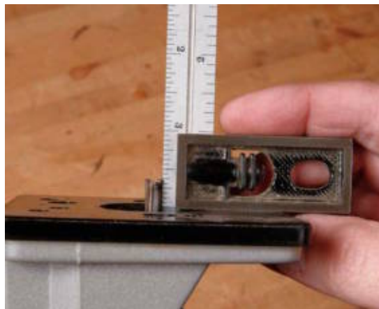
This small square is ideal for setting the depth of a router bit.
