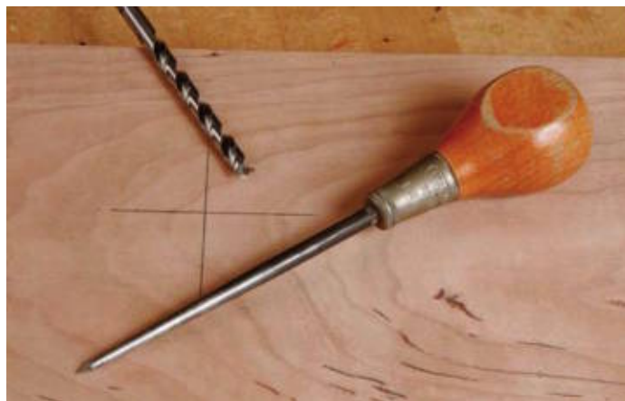
An awl will accurately locate the center point for drilling.
