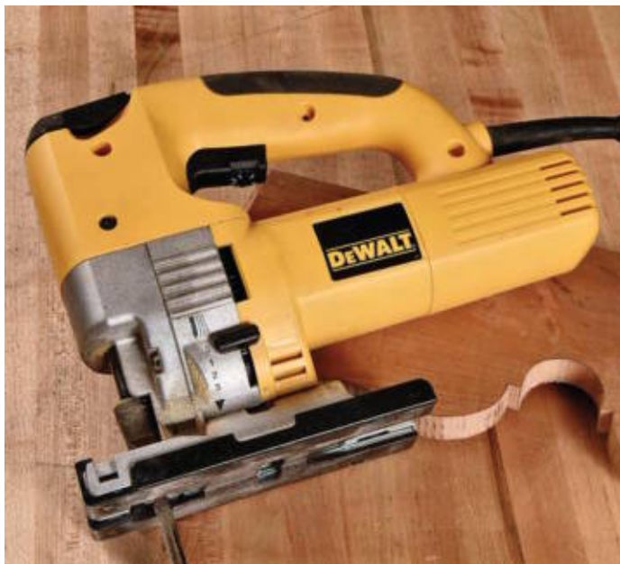
A jigsaw will cut curves on work too large to maneuver at the bandsaw.
