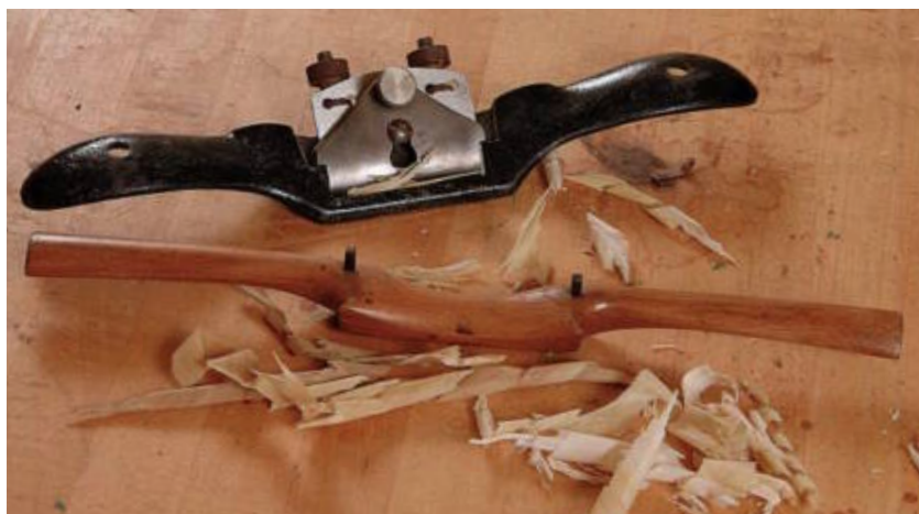
Spokeshaves are available with either wood or metal bodies.
