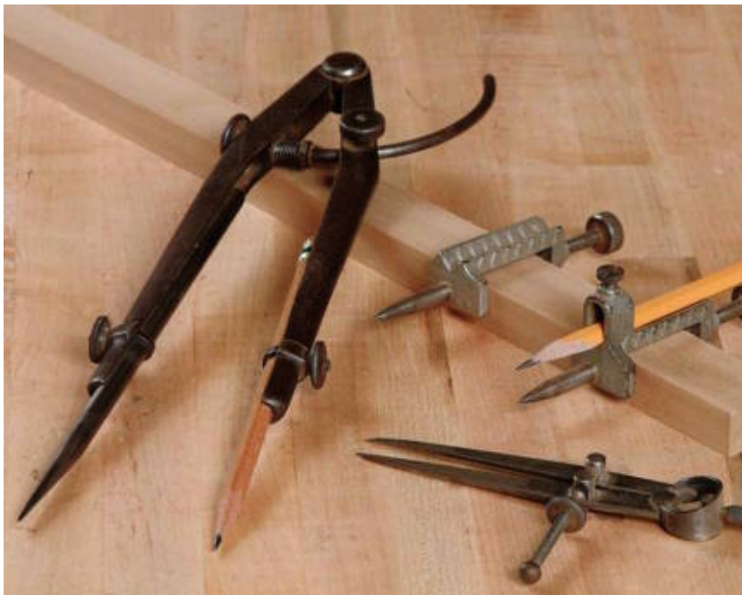
Trammel points, the compass, and dividers are useful for layout of circles and arcs.
