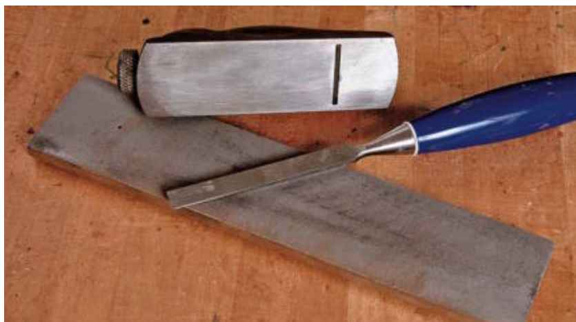
This “stone” is actually diamond particles bonded to a steel plate.
