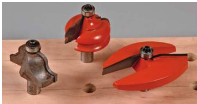
Large-diameter bits should always be run in a table-mounted router.
