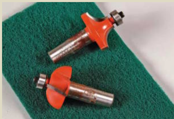
Abrasive pads are perfect for removing gunk buildup from router-bit shanks.
