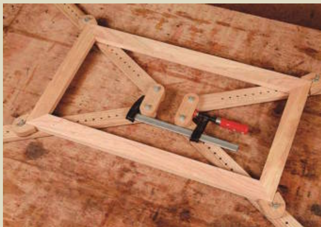
This shop-made mitered frame jig uses just one clamp to assemble an entire frame.
