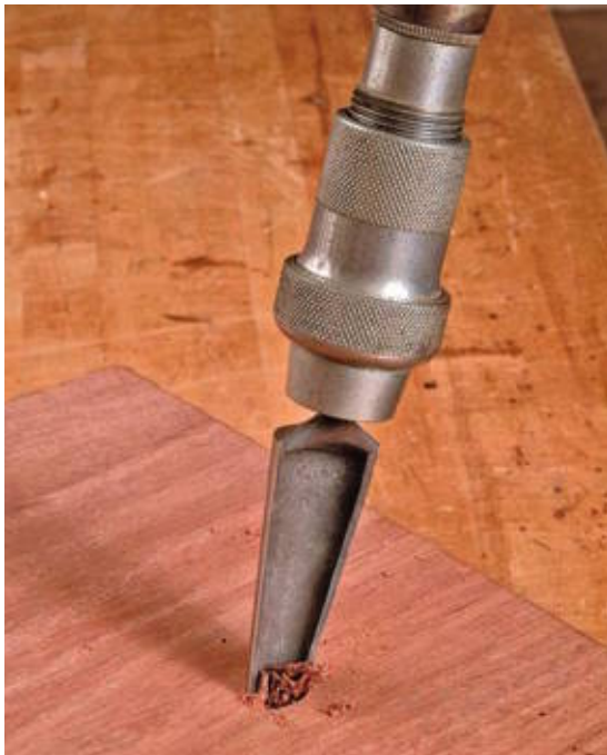
A reamer is used to taper a hole to fit a tapered leg.
