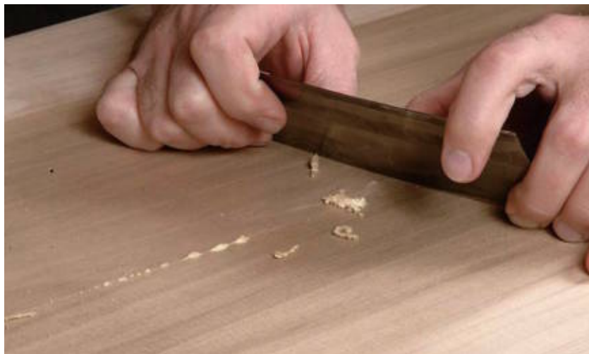
After an hour of drying time, yellow glue easily scrapes off.
