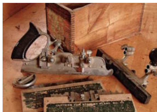
This Stanley No. 45 will adjust to cut beads or rabbets.
