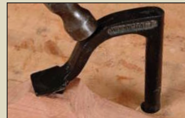
Strike the front of the hook to lock it into position.
