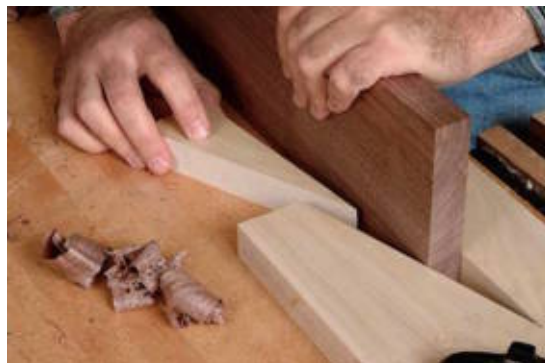
A wedge locks the board firmly into position.
