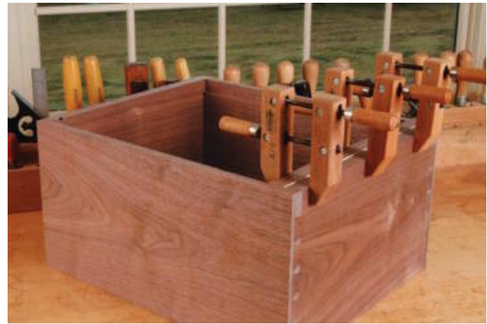
Handscrews apply broad clamping pressure, even on nonparallel surfaces.
