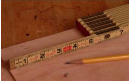
The 6-ft. folding rule is versatile and compact.
