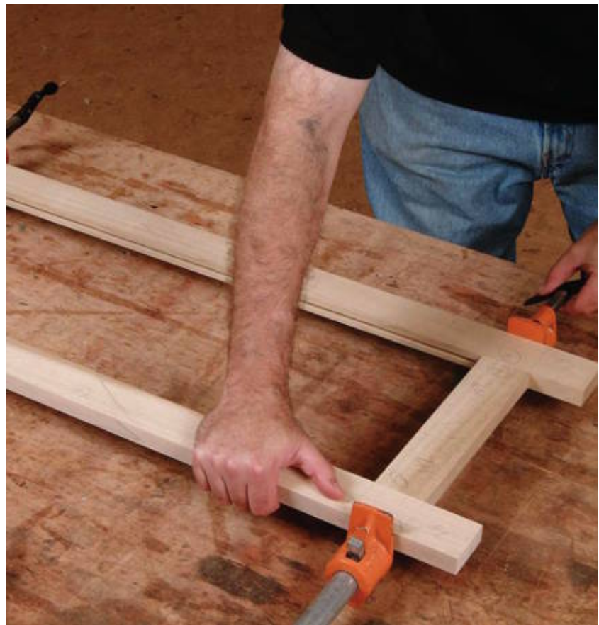
Pipe clamps are inexpensive and useful for a wide array of assembly tasks.
