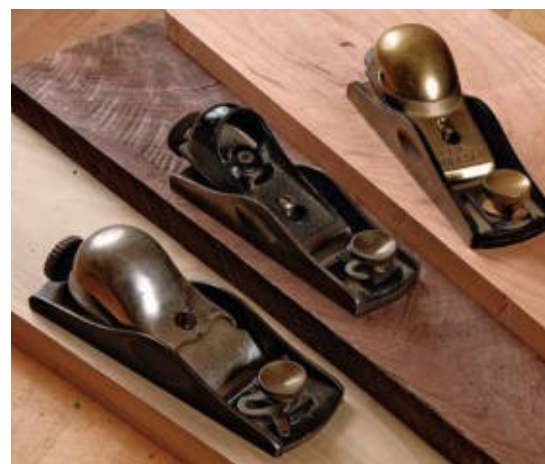
Block planes are small enough for one-handed use.
