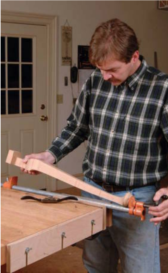
Pipe clamps are versatile and will easily hold legs for shaping.
