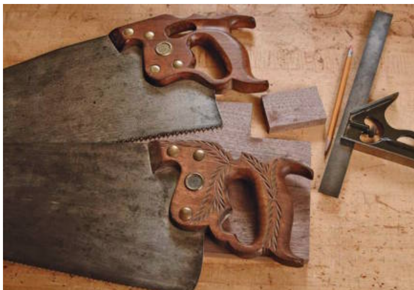
Panel saws create a wide kerf that is unsuitable for fine joinery.
