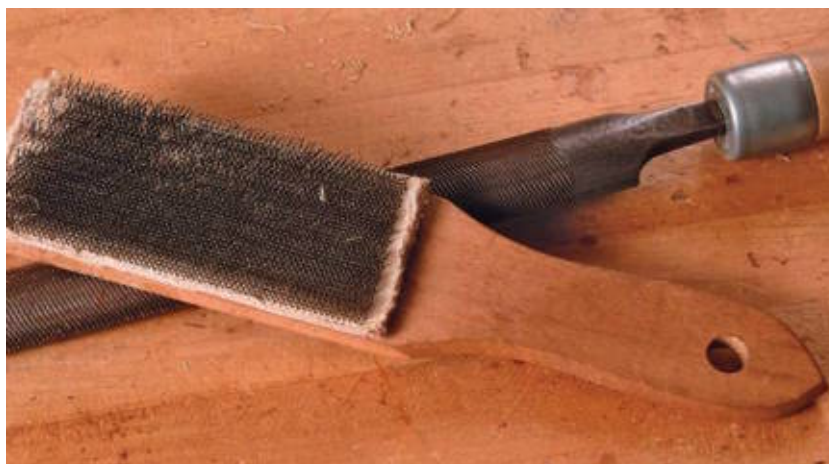
The short, stiff wire bristles of a file brush are specially designed for cleaning files.
