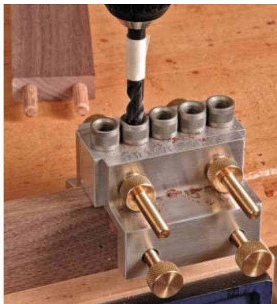
A drill guide will enable you to bore accurate holes without a drill press.
