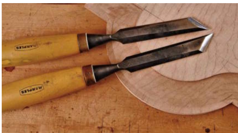
A pair of skew chisels will carve into corners.
