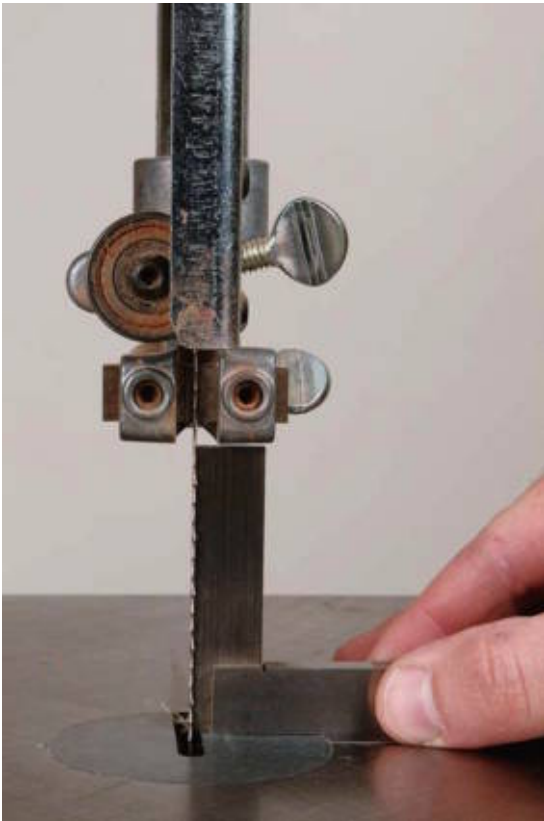
A small machinist's square is handy for squaring blades and bits.
