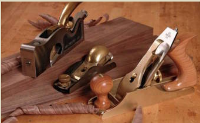
The bench, block, and shoulder planes (right to left) are essential for any furniture craftsman.
