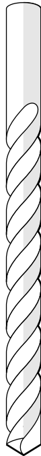
Twist drill bits cut metal as well as wood; are relatively inexpensive.
