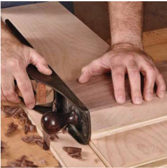
A shooting board holds stock for precise end-grain planing.
