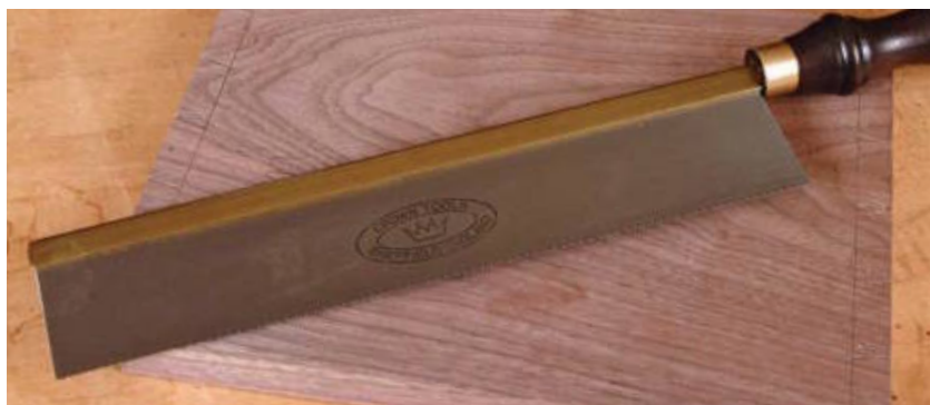
Dovetail saws are scaled-down backsaws with very fine teeth.
