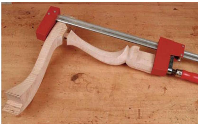
The deep reach of this clamp firmly grips the compound curves of an arm for a chair.
