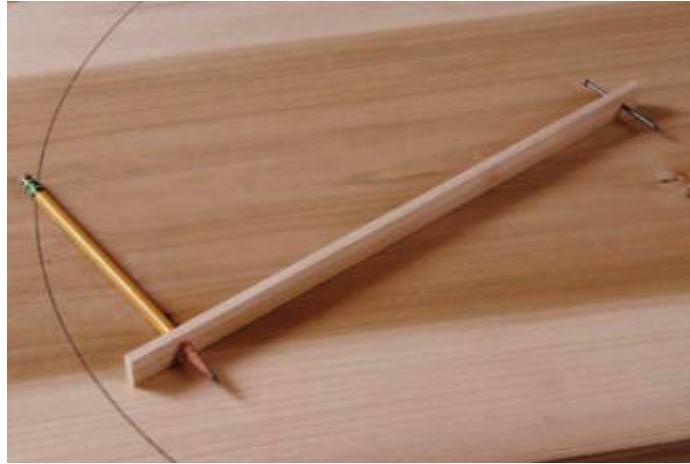
A stick fitted with a nail and pencil makes an economical trammel.
