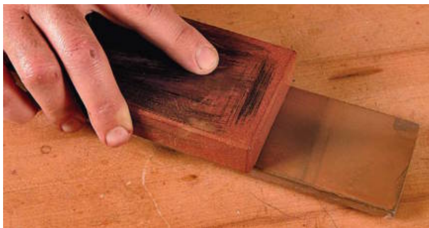
A diamond plate works well for flattening a sharpening stone.
