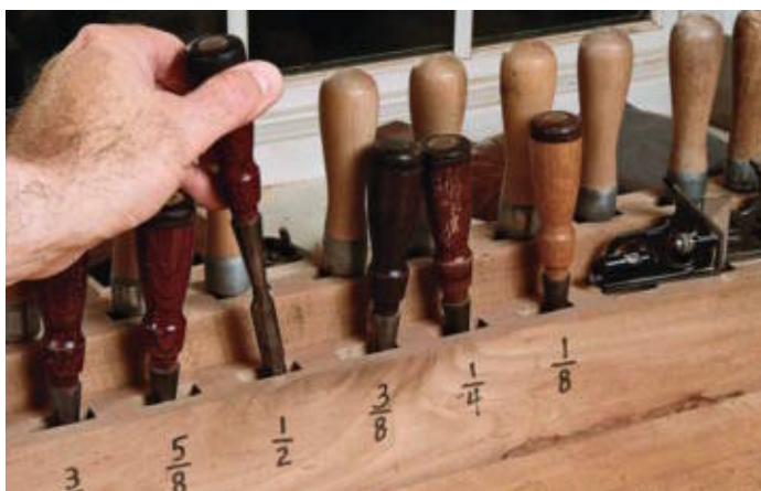
A chisel rack keeps tools sharp and close at hand.
