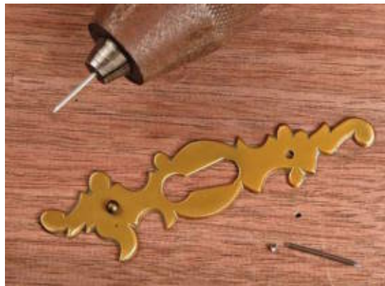
For a tiny drill bit, just snip the head off a brad.
