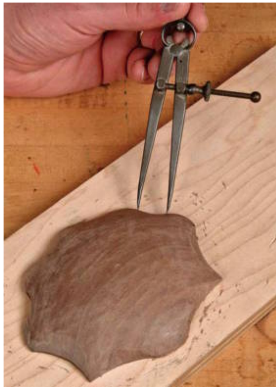
A divider is the best tool for layout of carvings.
