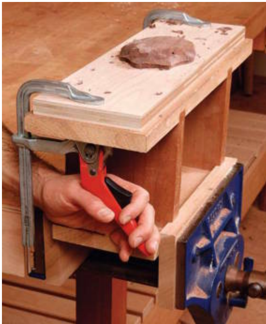
Ratchet clamps can be quickly repositioned.
