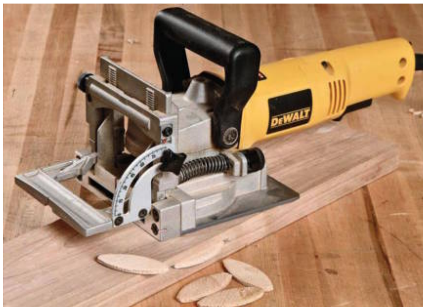
The plate joiner cuts fast joints for simple cabinet construction.
