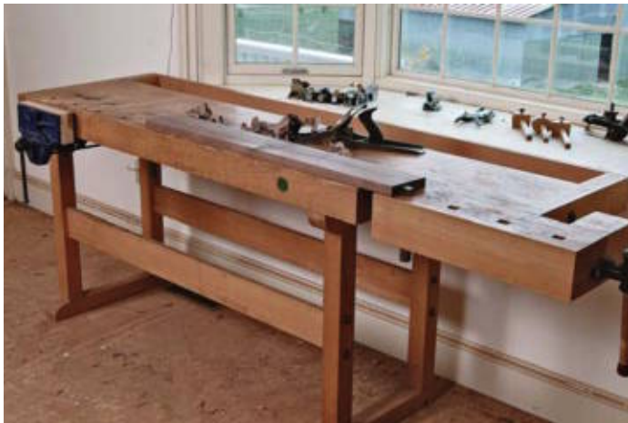
A European bench is outfitted with two vises and a row of dog holes.
