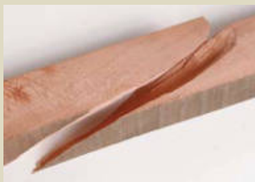
Short grain is weak and prone to breakage.
