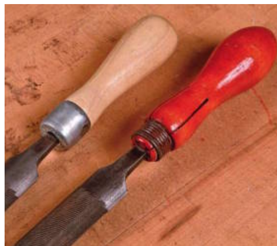
For safety and greater control, equip your files with handles.
