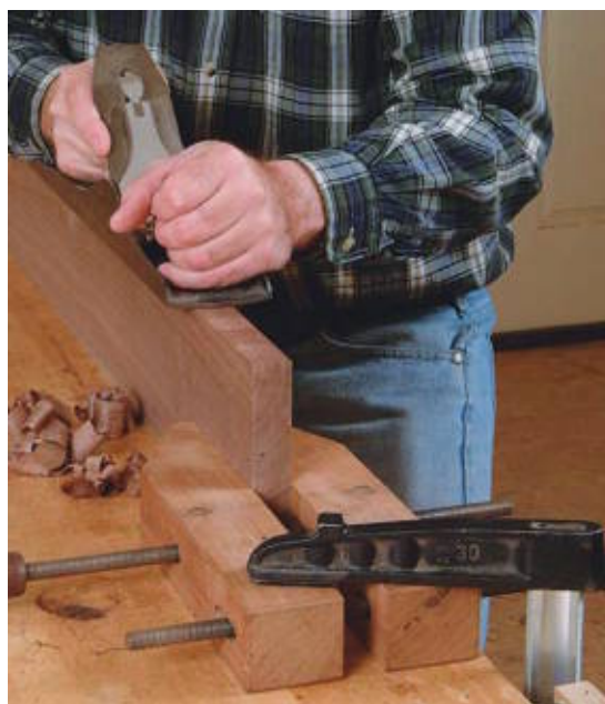
If you lack a vise, try gripping work with pairs of clamps.
