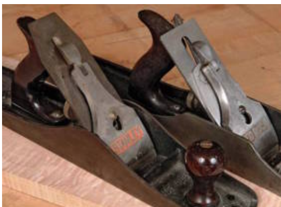
A Bedrock plane is easily distinguished by its square sides.
