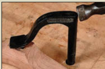
Striking the back corner will release it.
