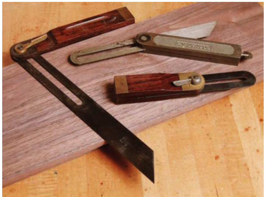
The bevel gauge is used to lay out, copy, and transfer angles.
