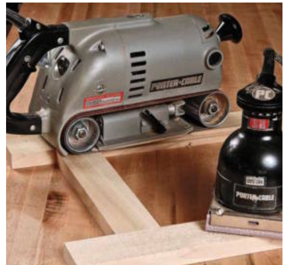
Power sanders don't leave the surfaces flat, so avoid using them on your finest work.
