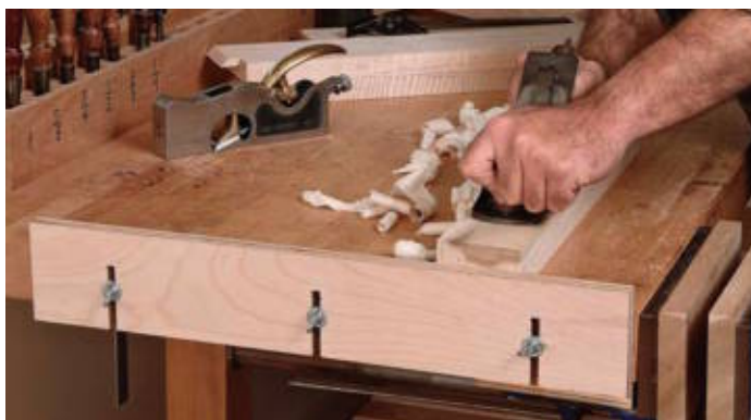
A drop-down stop is essential for planing.
