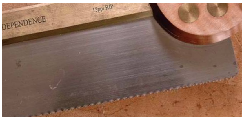
The fine teeth (15 tpi) and slight “set” of this dovetail saw are ideal for sawing precise joints.
