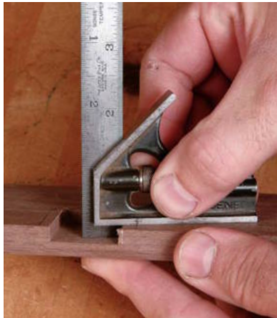
To check the depth of a mortise, use a combination square.
