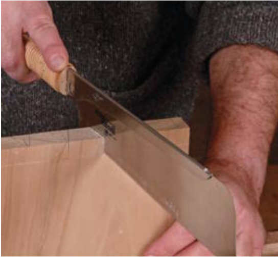
Japanese saws cut on the pull stroke and create a very fine kerf.
