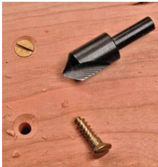
The countersink bevels the edge of a hole to fit the head of a screw.
