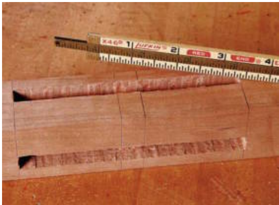
The slide on a folding rule is ideal for measuring the depth of a mortise.
