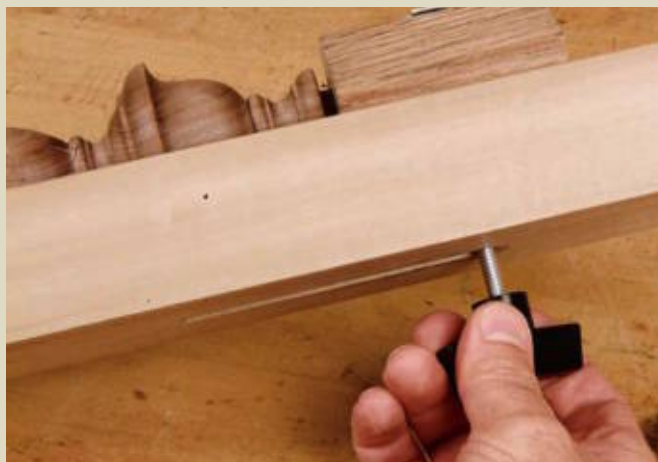
Threaded rod allows you to make clamp fixtures for unusual shapes.
