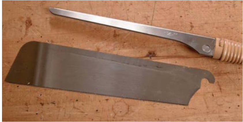
This Japanese saw has a replaceable blade.
