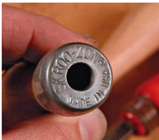
This file handle has threads that seat firmly on the tang of a file.
