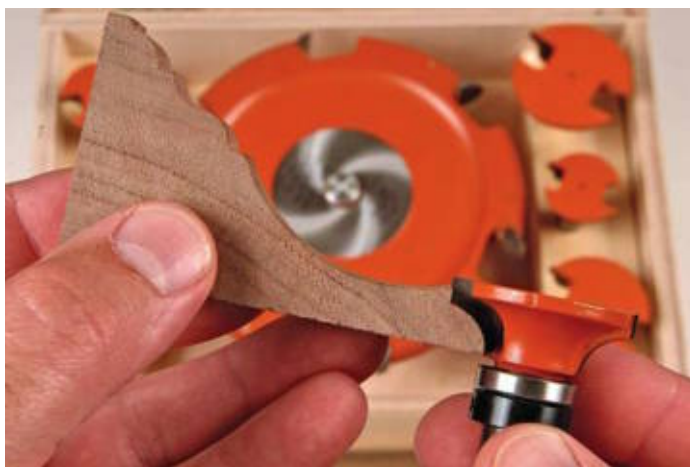
This unique bit is inverted on the shank and can shape profiles ordinary bits can't.
