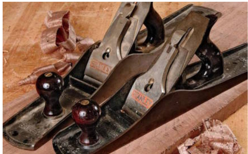
Long bench planes are best for flattening rough stock and straightening edges.
