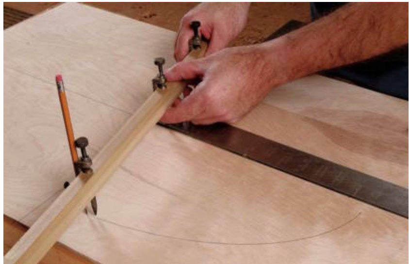
Trammels are used to lay out circles and ellipses.
