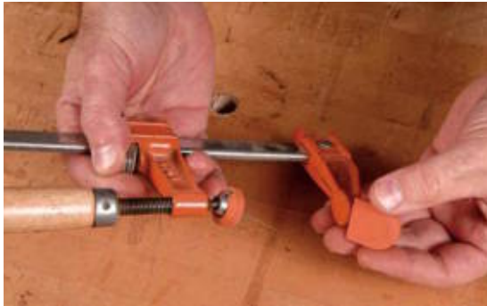
Plastic clamp pads slip onto the jaws to cushion the work and prevent damage.
