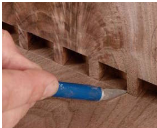
A marking gauge inscribes the wood with a tiny knife.
