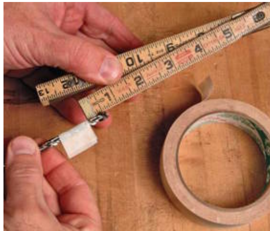
Another simple depth stop is a piece of masking tape.
