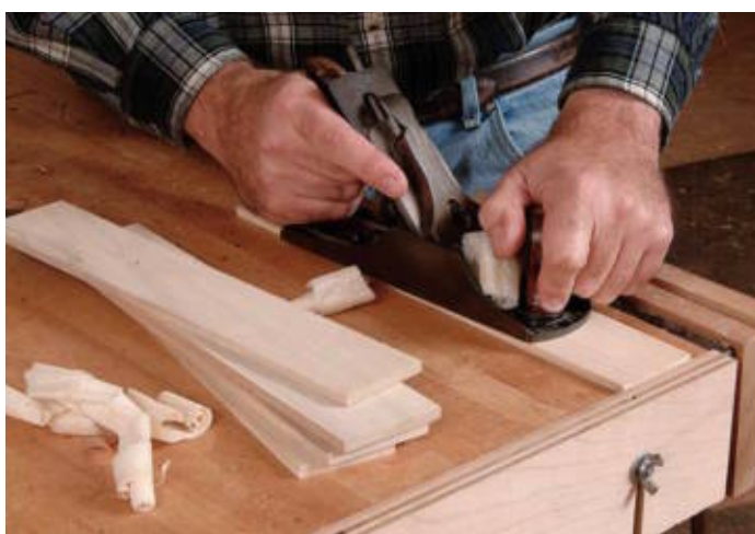
A drop-down bench stop will accommodate stock of various thicknesses.
