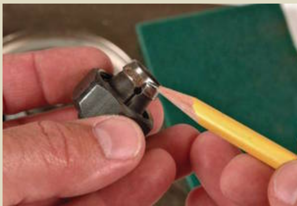
Be sure to keep the router collet clean.
