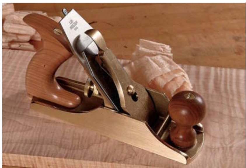
A Bedrock plane is easily distinguished by its square sides.
