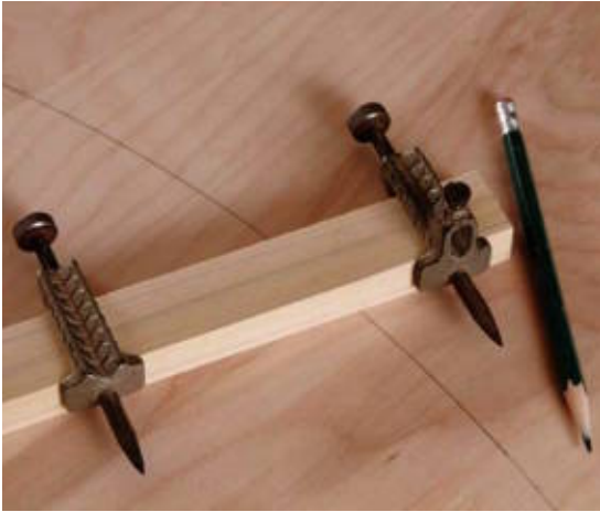
Trammel points clamp to a stick used to draw large arcs and circles.
