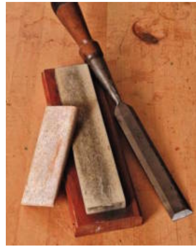
Arkansas stones require oil as a lubricant.
