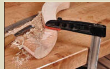
This deep-reach clamp has plenty of holding power.
