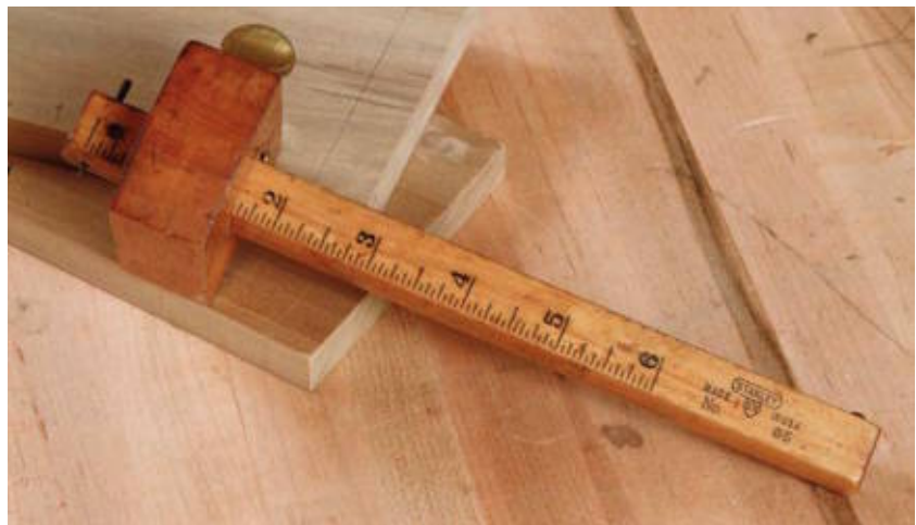
A marking gauge inscribes the wood with a tiny knife.
