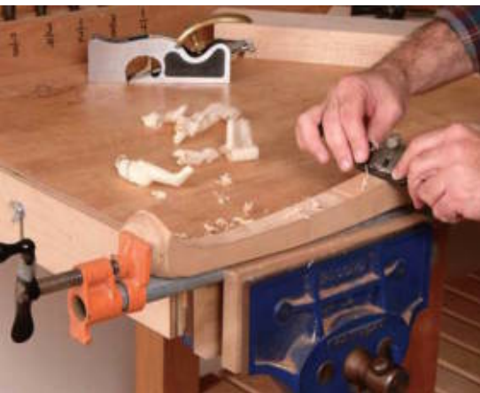
A strong vise completes the workbench. A pipe clamp locked in a vise is a great way to hold irregular work, such as this cabriole leg.
