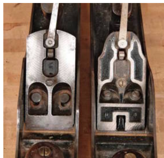
The frog of “Bedrock”-style planes is a much-improved design over “Bailey” planes.
