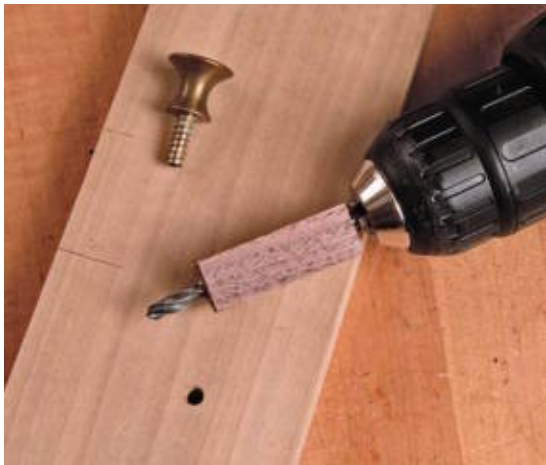
A block of wood works well for a depth stop.
