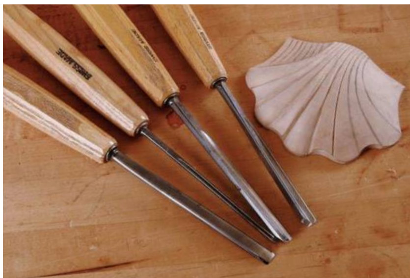
Gouges are used for carving.
