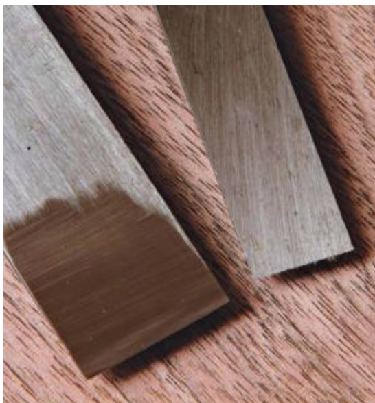
New chisels must be polished on the back.
