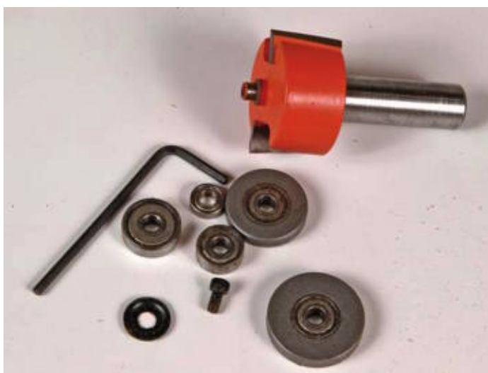
You can change the cutting depth of many router bits by switching to a different bearing diameter.
