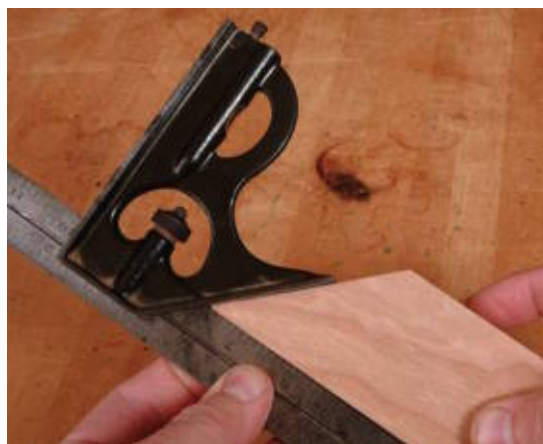
A combination square is also effective for checking miters.
