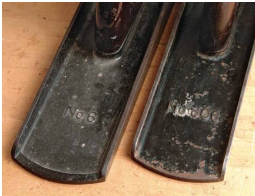
Bedrock planes can be identified by the “60” prefix. The plane at left is a standard No. 6; at right is a Bedrock No. 606.
