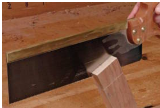
A backsaw has fine teeth and a stiff back for sawing fine joinery.
