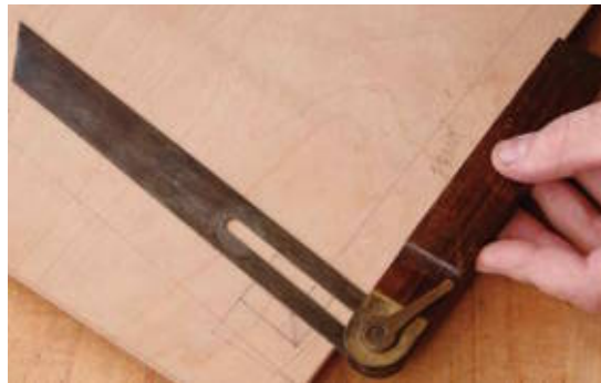
A bevel gauge will adjust to transfer any angle.
