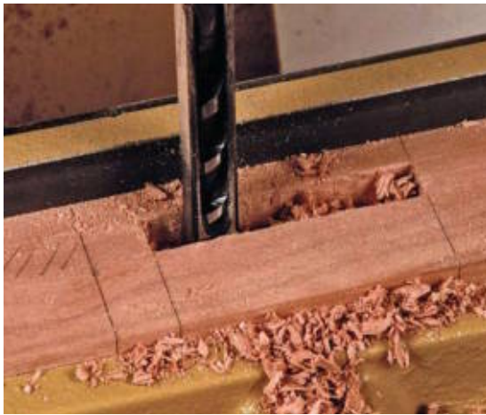
A mortise is created by boring a row of overlapping holes.
