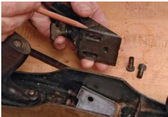
A machined groove in the Bedrock frog keeps it aligned with the sole.
