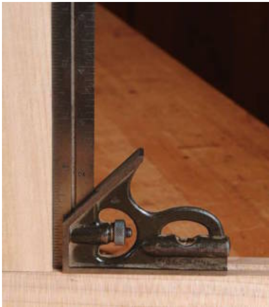
The sliding head of the combination square can be positioned for inside corners.
