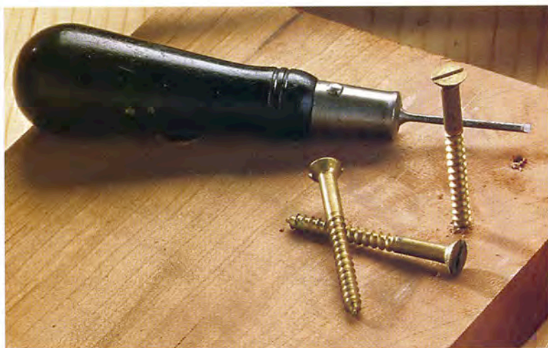
The chisel tip of this bradawl severs—rather than just parts—the fibers as it is pushed and twisted into the wood to drill a small hole for a screw or nail.
