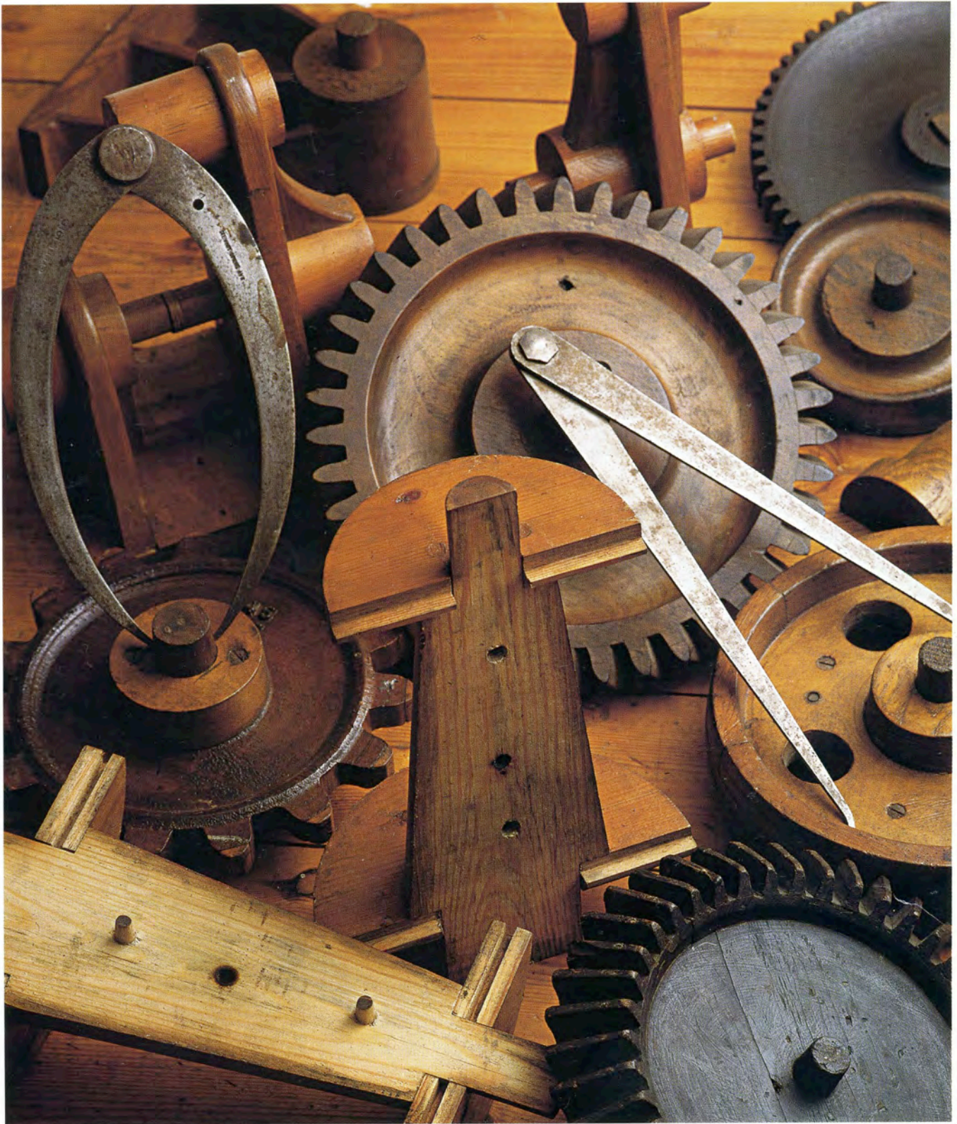
Patternmakers rely on inside and outside calipers for transferring dimensions from drawings to accurately size the round section of wooden patterns for casting anything from gears to shafts and wheels.
