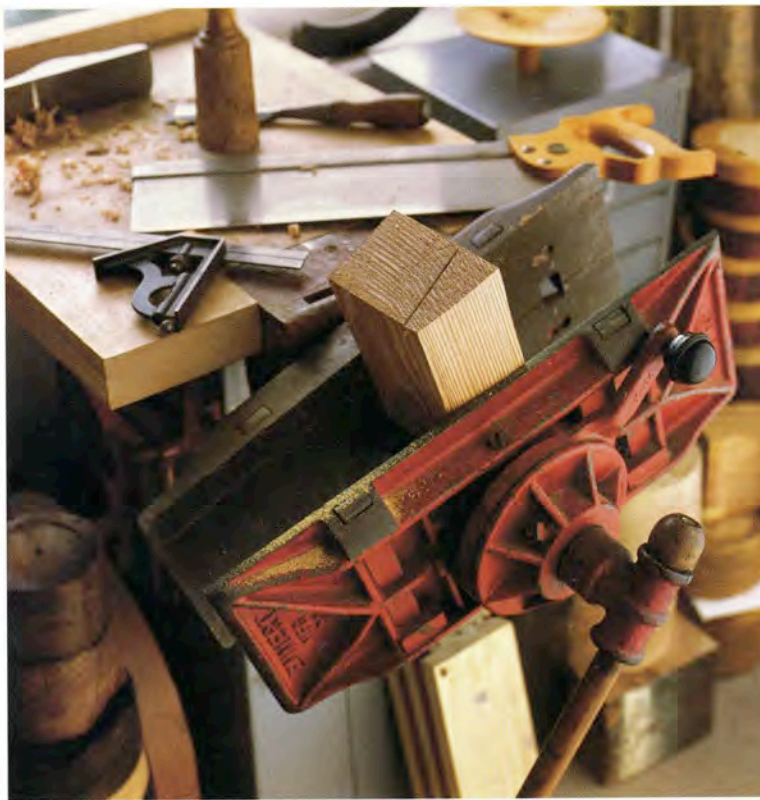
The Emmert patternmaker's vise swivels, tilts, locks in any position, and clamps odd shapes with pivoting jaws.
