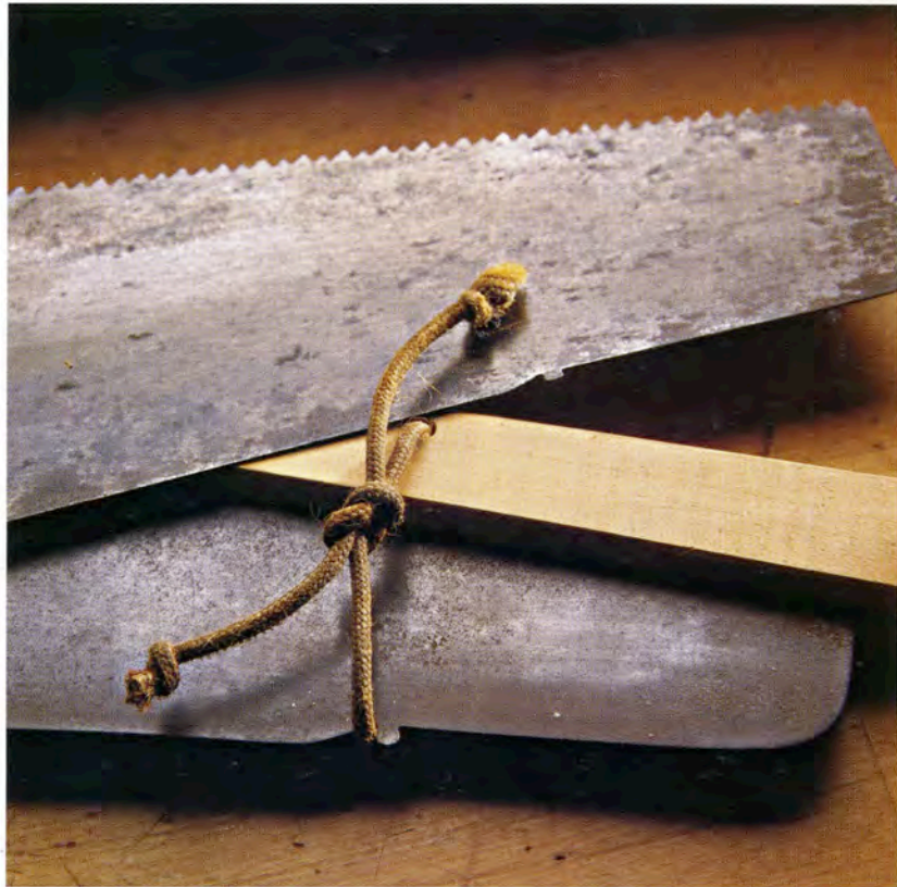
The little nib on the end of fine handsaws has sparked much curiosity about its function and origins. It's a vestigial decoration dating back to the 17th century.
