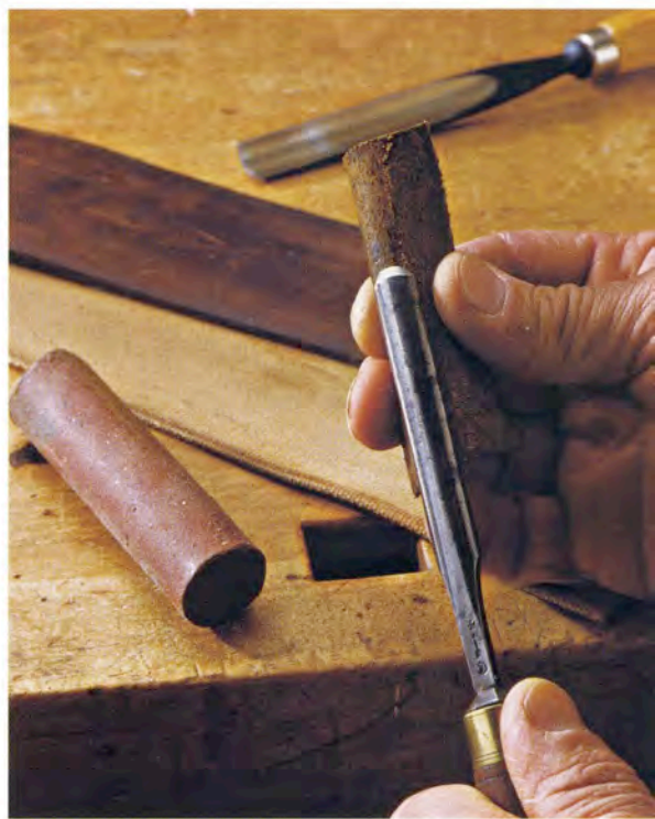
A piece of leather charged with rouge, an extremely fine abrasive, makes a good strop for the final honing of curved or straight cutting edges.
