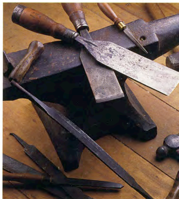
The high-quality steel in old rasps and worn files can be forged or ground into practical new tools, such as rugged timber-framing chisels (with rasp teeth clearly visible), a lathe tool, a burnisher, and a drawknife.
