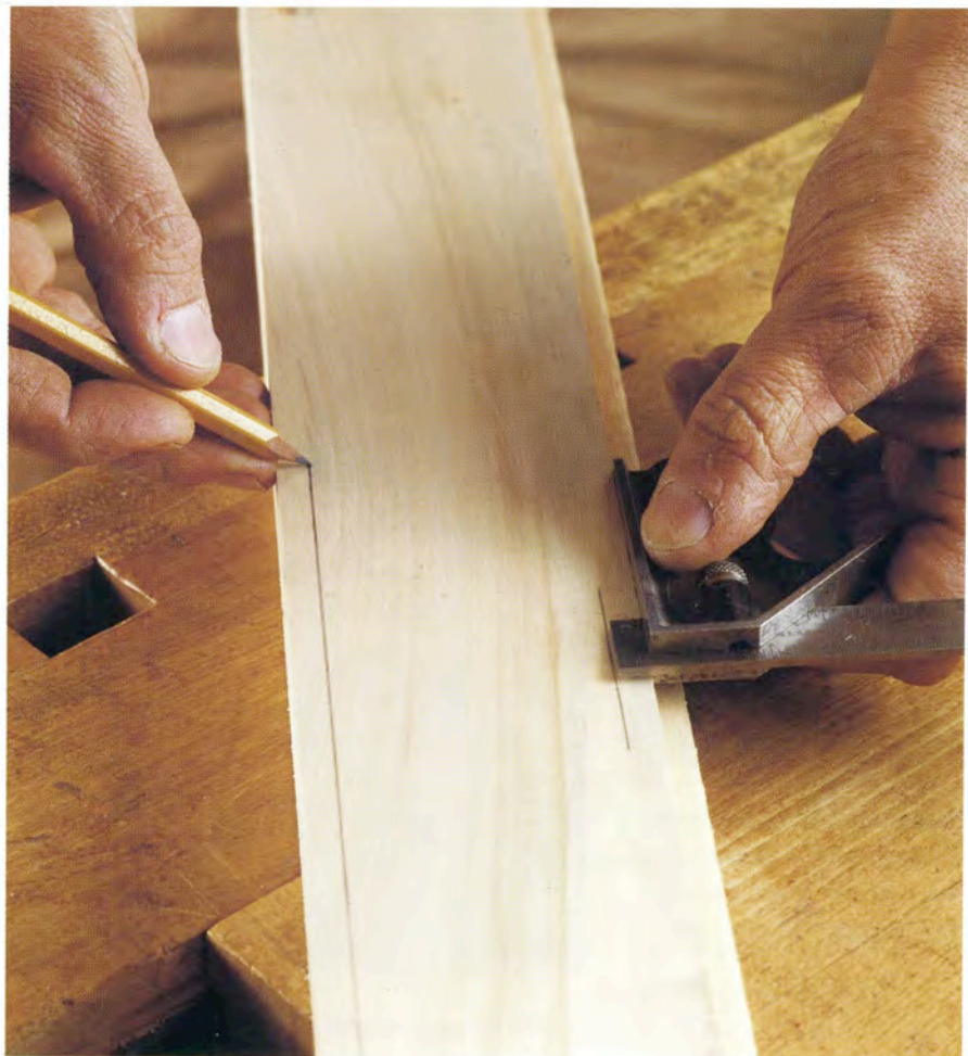
A combination square and pencil make a quick marking gauge, but it's almost as accurate and faster to wrap a couple of fingers over the corner of the board for gauging a pencil line.
