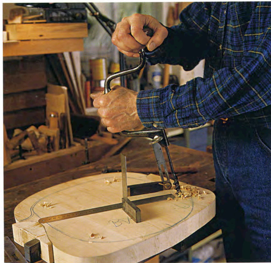
Drill at a compound angle by sighting against a square and bevel gauge set to the required angle. A ruler establishes a sighting plane against the square, to keep the bit angled yet plumb. Steady yourself by planting your feet, leaning against the bench, and locking your upper body.
