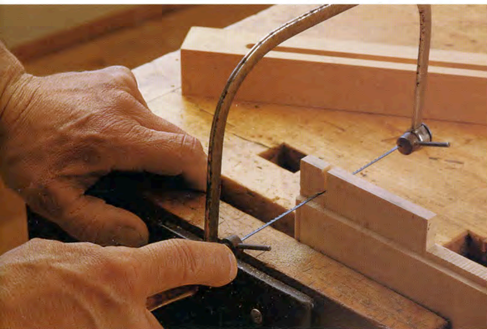
The fine, narrow blade of a coping saw allows you to change direction easily, when sawing a tenon and haunch in one continuous motion, for example. The blade pivots in the frame (note the levers front and back) for even more maneuverability.
