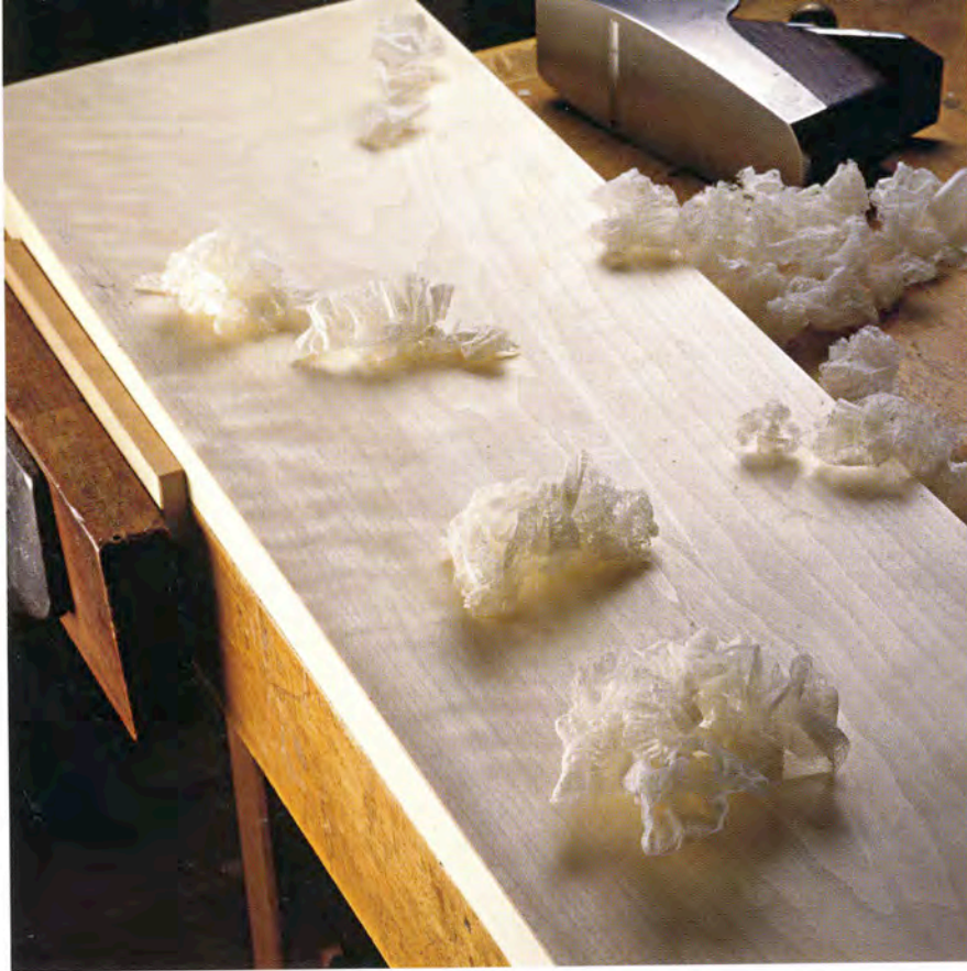
Planes, especially tight-mouthed smoothers, favor controlled cutting of the wood fibers over splitting, producing an exceptionally smooth surface on the hardest of woods.
