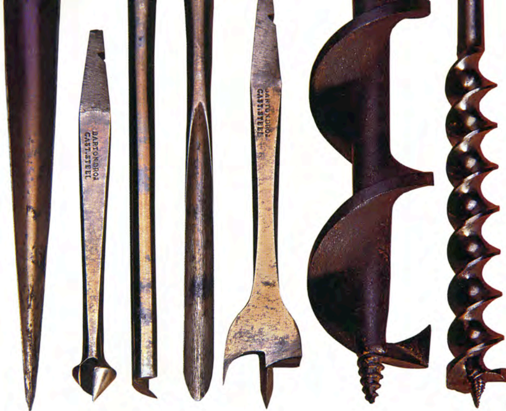
Bits have evolved from sharpened points to sophisticated cutting tools. Shown here (from left to right) is a reamer for enlarging and tapering holes, a countersink, early nose and shell bits similar to spoon bits, a center bit with single spur and cutting lip, a single-twist auger without cutting spurs, and a double-twist auger with cutting spurs.
