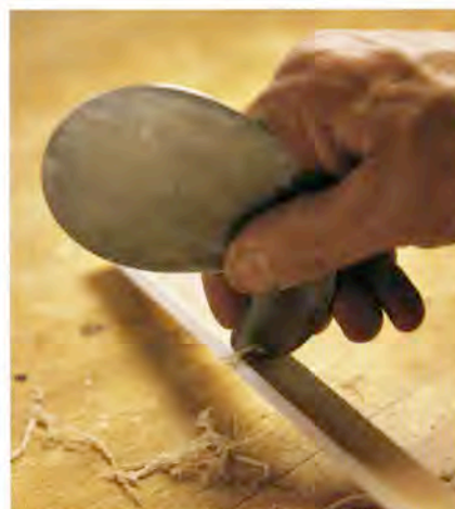
A gooseneck scraper has curved edges of different radii to scrape moldings and shaped parts. It's faster than sanding, cuts a more consistent profile, and leaves a smoother surface.
