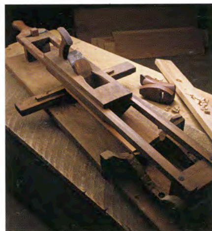
Sometimes the line between hand tool and machine is hazy. This interesting device probably was made by a cooper, who cleverly attached a round-soled plane to rails in order to make his efforts hollowing pail staves more efficient and uniform. In the background is a stoup plane for doing similar work freehand.
