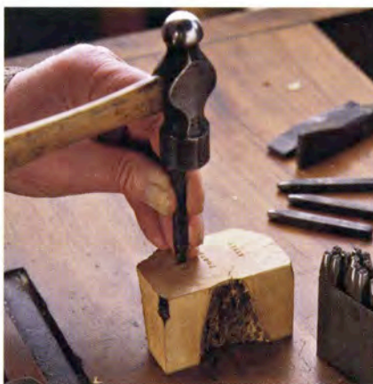
With a set of number and letter punches, you can impress your name (or any other inscription) into the wood or soft metal parts of a tool.
