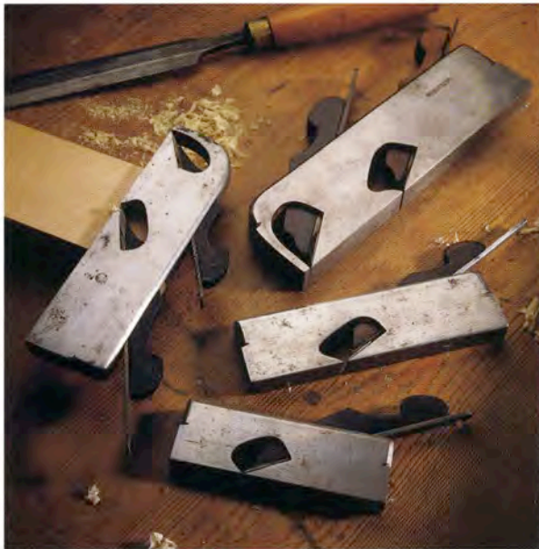
Shoulder planes such as the four shown here are typical of the work of Stewart Spiers, an early maker of stuffed planes. Two of the planes have unusual double irons for two cutting positions.
