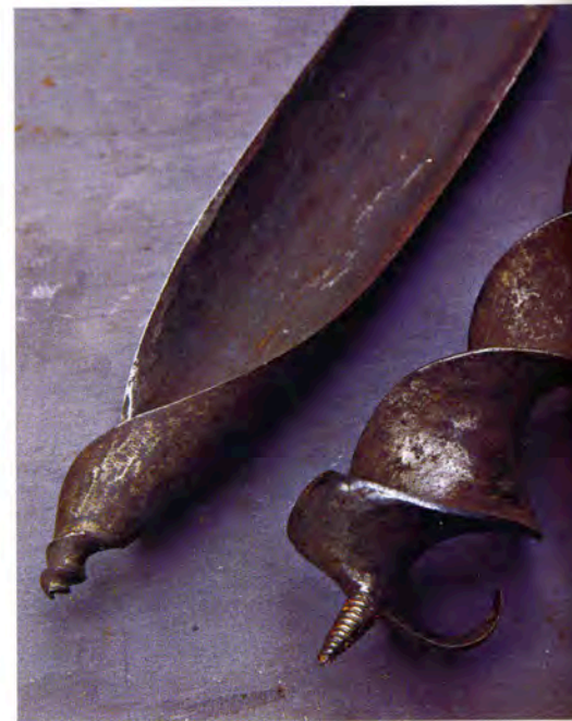
Although they express beauty beyond their function, every detail of the shape and cutting edges of these large gimlet-point and Scotch-eyed augers is designed to cut wood fibers and spiral the chips away.
