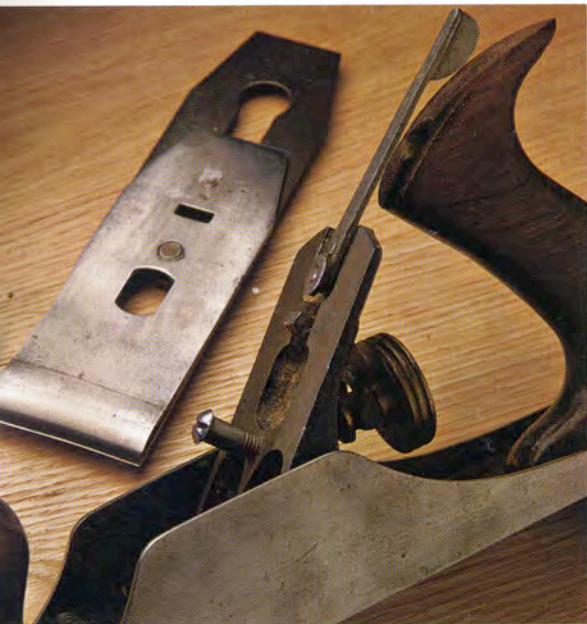
Bailey-type planes have two adjusters: a lateral adjustment lever that engages with the slot in the iron and pushes it right or left, and a brass adjuster wheel that slides the iron in and out by pushing against a slot in the cap iron.
