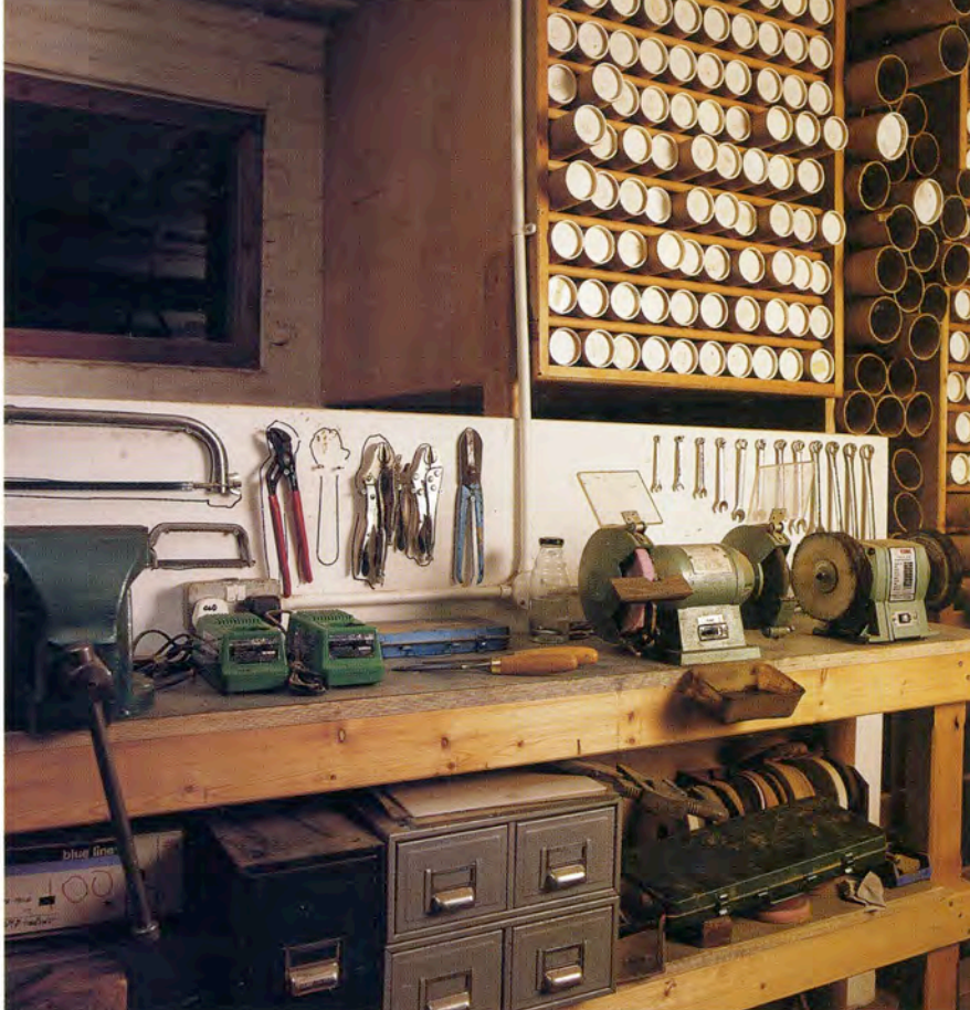
Isolate the dirt and mess of toolmaking on a separate bench, preferably with a metal top, a large metalworking vise, a grinder, a buffer, and the necessary hand tools nearby.
