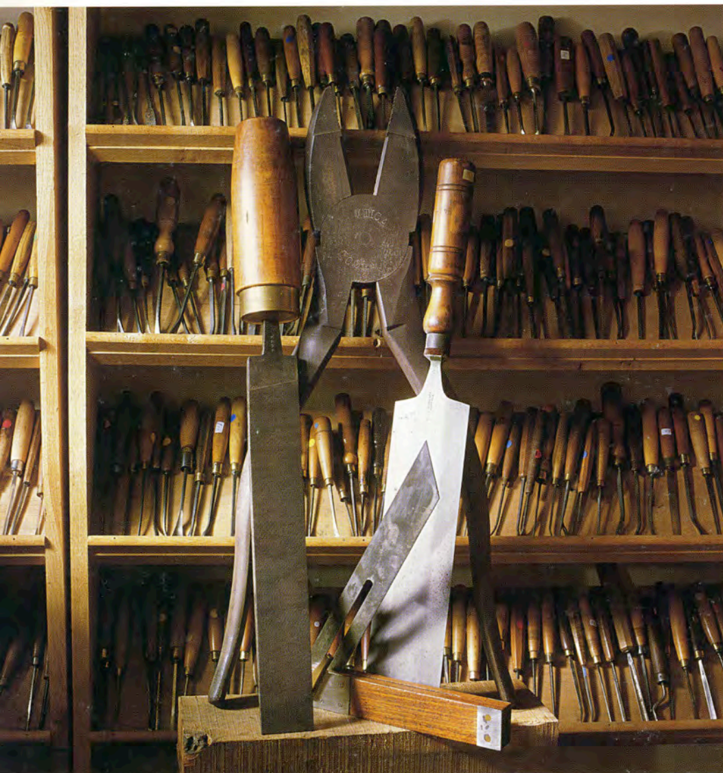
Oversized hand tools were sometimes used as advertising props, but all of these tools are capable of extra large work, such as filing the huge bearings of a steam engine.
