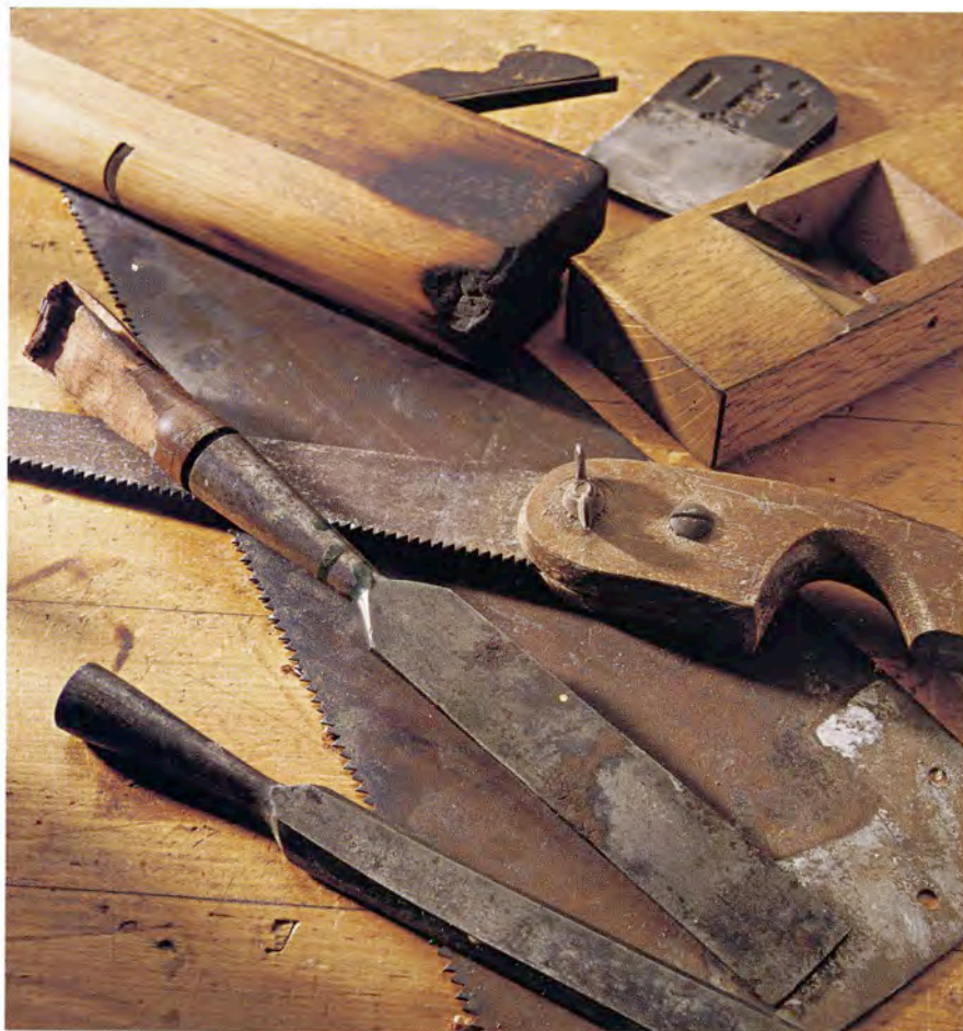
Any woodworker with modest skills could restore these flea-market finds with some basic repairs, such as shaping a new handle, replacing a missing wedge, or piecing in the charred heel of the round plane.
