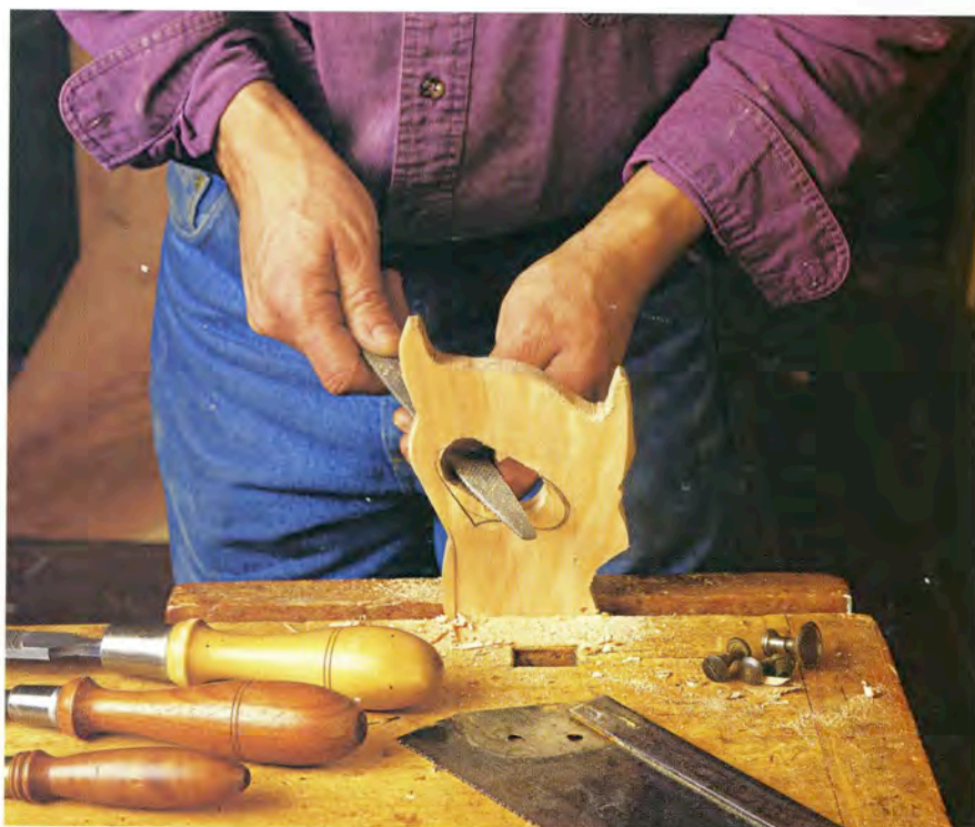
Cut out a new saw handle with a bandsaw or coping saw, and refine and smooth it with rasps and files. All three handles on the bench were turned on a lathe and fitted with old ferrules. (Photo by Jon Binzen.)
