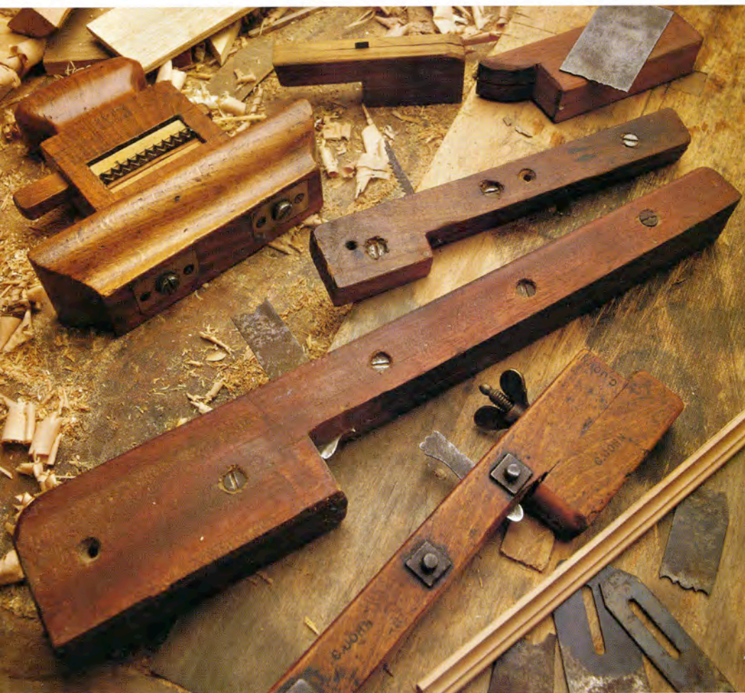
Scratch stocks are versatile scraping tools for cutting anything from inlay grooves to small moldings. They are no more complicated than a profiled blade secured in a simple wooden holder that also functions as a fence.
