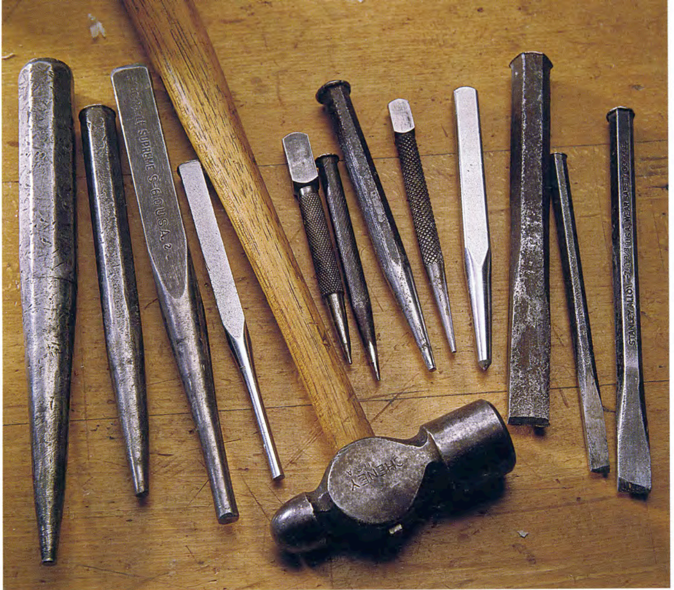
For many woodworking and metalworking tasks, especially for making and repairing tools, you'll need some small cold chisels of different sizes (at right) as well as (from left) a center punch for marking drill holes, nail sets, punches, and a ball-peen hammer.
