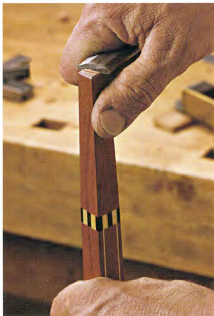
A chisel functions as a flat-backed knife for light paring cuts, such as trimming the end of a delicate table leg. Use your thumb for leverage and a slicing or skew cut. Chamfer the edges first to prevent breaking out the fibers.
