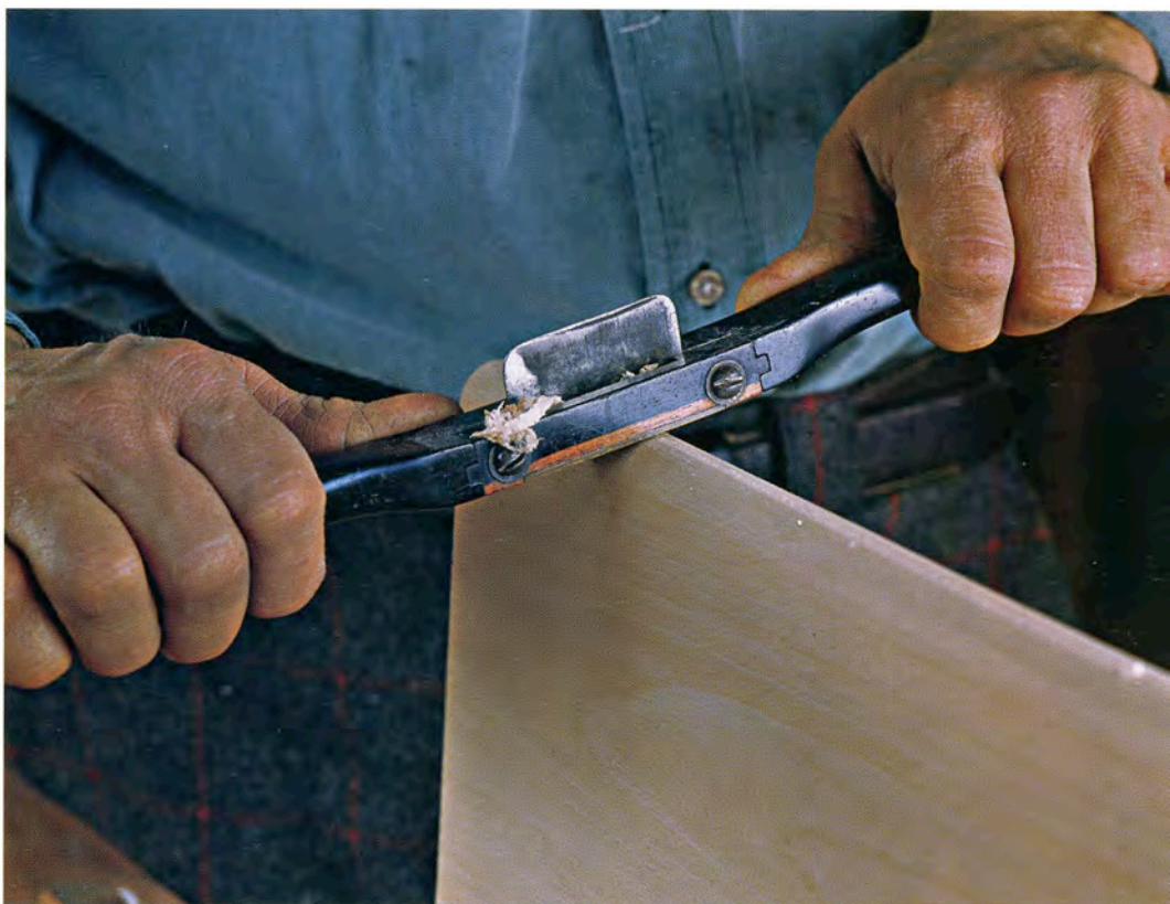
This sleek ebony spokeshave scraper with comfortable handles, a thin scraper blade, and a microscopically fine throat will smooth and fair curves.
