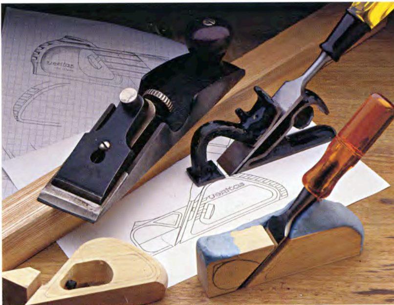
At Lee Valley Tools, the process of designing and refining the prototype for a new chisel plane involves drawings, wooden models, and plenty of close inspection of older tools such as this Stanley #97 and an anonymous cast-iron plane for inspiration. (Photo by Ray Pilon.)
