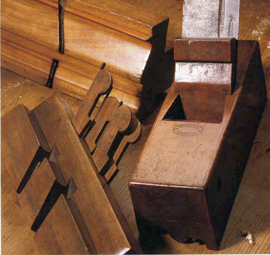
The multiple irons in these complex molding planes are much easier to sharpen and tune than a single, large iron.
