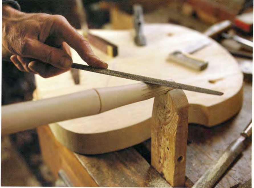
One of the best rasps still on the market is the #50 patternmaker's rasp made by the venerable Nicholson File Co. of Providence, Rhode Island. It's the ideal tool for making light, controlled cuts, such as filing away high spots to fit a tapered leg to its mortise.
