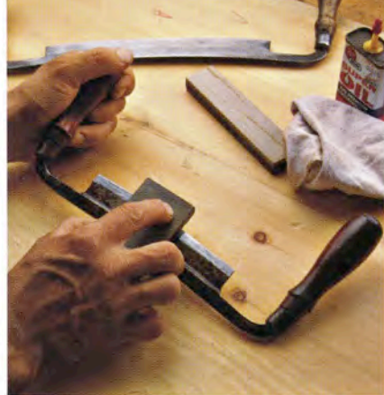
Sharpen a drawknife as you would a chisel, with about a 20° bevel and slight back bevel. It's easiest to hold the tool steady on a surface and bring the stone to the blade.
