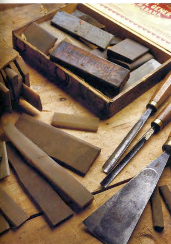
Natural or man-made slipstones hone curved or small edges such as gouges and molding-plane irons. Many useful shapes are available, but if need be, you can shape your own against a diamond stone.
