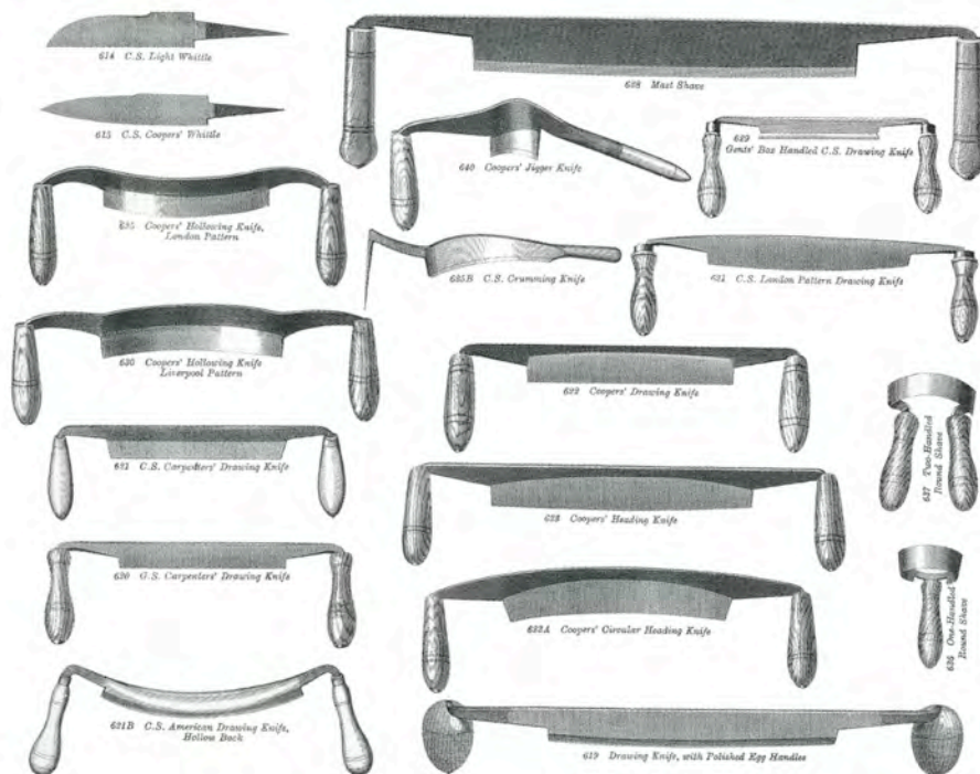
Coopers used many drawknives: one for beveling the head and bottom of the barrel, another for shaping the staves inside and out, another for leveling an area for the head (a cooper's jigger), and yet another for smoothing the inside of the barrel.
