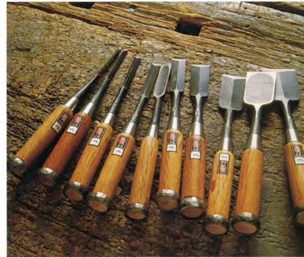
With blades as wide as 4 in. and handles 12 in. or more in length, slicks are the largest chisels, but they are capable of finer work than their size suggests. They were traditionally a shipbuilding tool, used to pare, level, and fit decking and frames.
