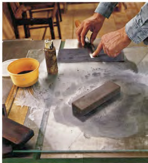
A lapping table made with silicon-carbide powder or a sheet of abrasive paper on plate glass is ideal for flattening chisel backs, plane soles, and sharpening stones.
