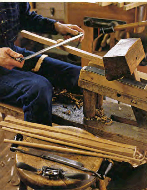
Coopers used many drawknives: one for beveling the head and bottom of the barrel, another for shaping the staves inside and out, another for leveling an area for the head (a cooper's jigger), and yet another for smoothing the inside of the barrel.
