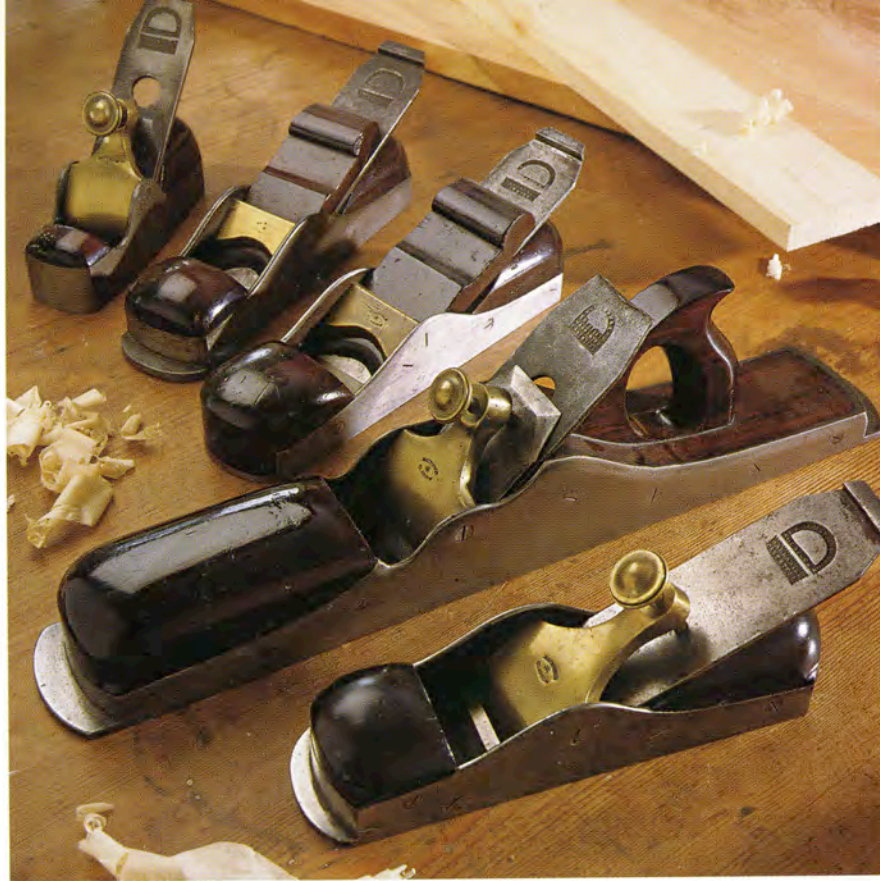
These late 19th-century bench planes by Mathieson of Glasgow, Scotland, do not have cast bodies but are made of steel plates dovetailed together. Combined with an overstuffed wood infill (like over-risen bread), they are massive enough to work figured or ornery timbers more easily than comparable Bailey planes.
