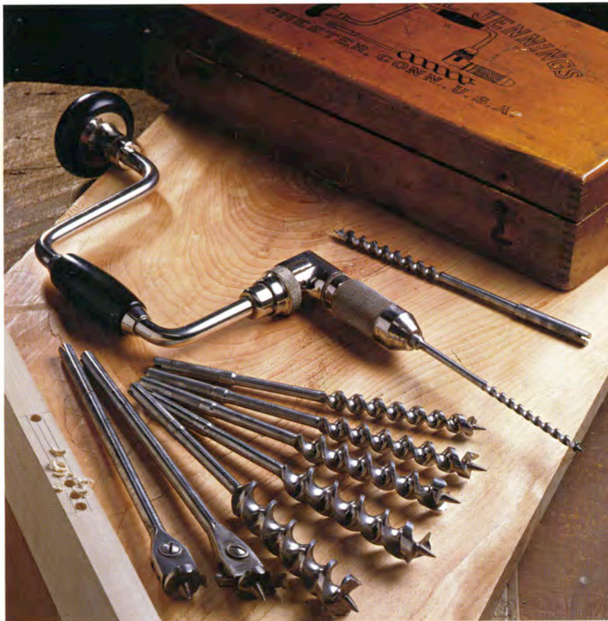
This elegantly boxed set of Russell Jennings "Precision Shank" twist bits (1855) slip securely into the ratcheting brace for boring quick and accurate holes.
