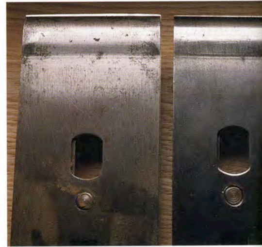
One rule of thumb for positioning the cap iron is to set it as close to the cutting edge as the shavings you will cut. Set it extremely close for a smoothing plane (right) and with about a \frac{1}{16} -in. reveal for a cambered jack-plane iron (left).
