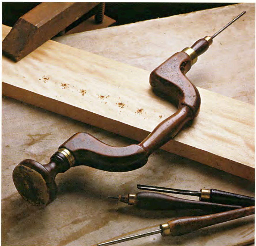
Typical of early shopmade braces, this small piano maker's brace is sawn and shaped from a single piece of beech. It has bits fitted to separate pads that merely jam into the tapered chuck.
