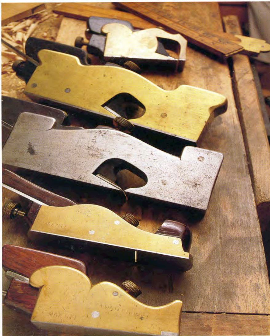
Norris bullnose, shoulder, and chariot planes for fine-tuning joinery are among the most beautiful planes ever made—and the most rare today.
