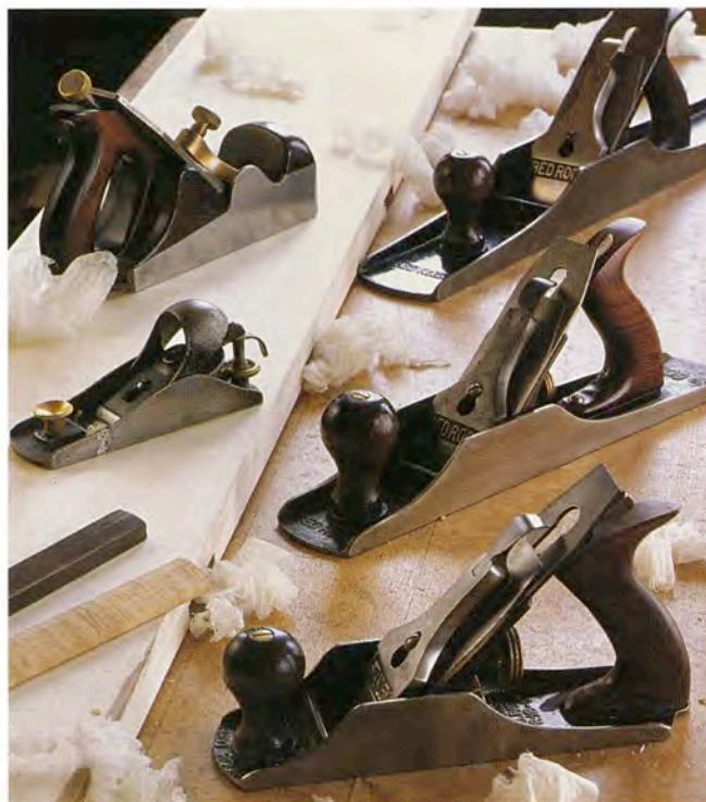
Planes are the most useful and beautiful of hand tools. These bench planes, which include a Norris #A6 smoother and Stanley Bedrocks #604, #605, and #607, can make delicate fitting cuts, shoot long straight edges, or flatten a surface to a polished sheen.
