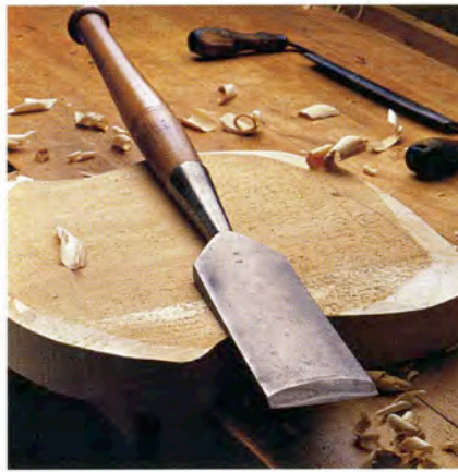
With blades as wide as 4 in. and handles 12 in. or more in length, slicks are the largest chisels, but they are capable of finer work than their size suggests. They were traditionally a shipbuilding tool, used to pare, level, and fit decking and frames.
