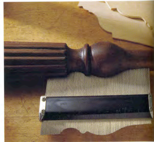
The fine steel fingers of a profile gauge conform to any contour, producing both a positive and negative profile.
