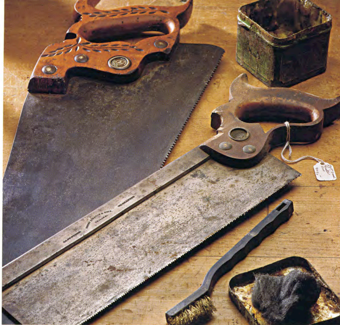
A stiff brass brush, fine steel wool, and a mixture of boiled linseed oil and beeswax will clean and polish both wood and metal surfaces.
