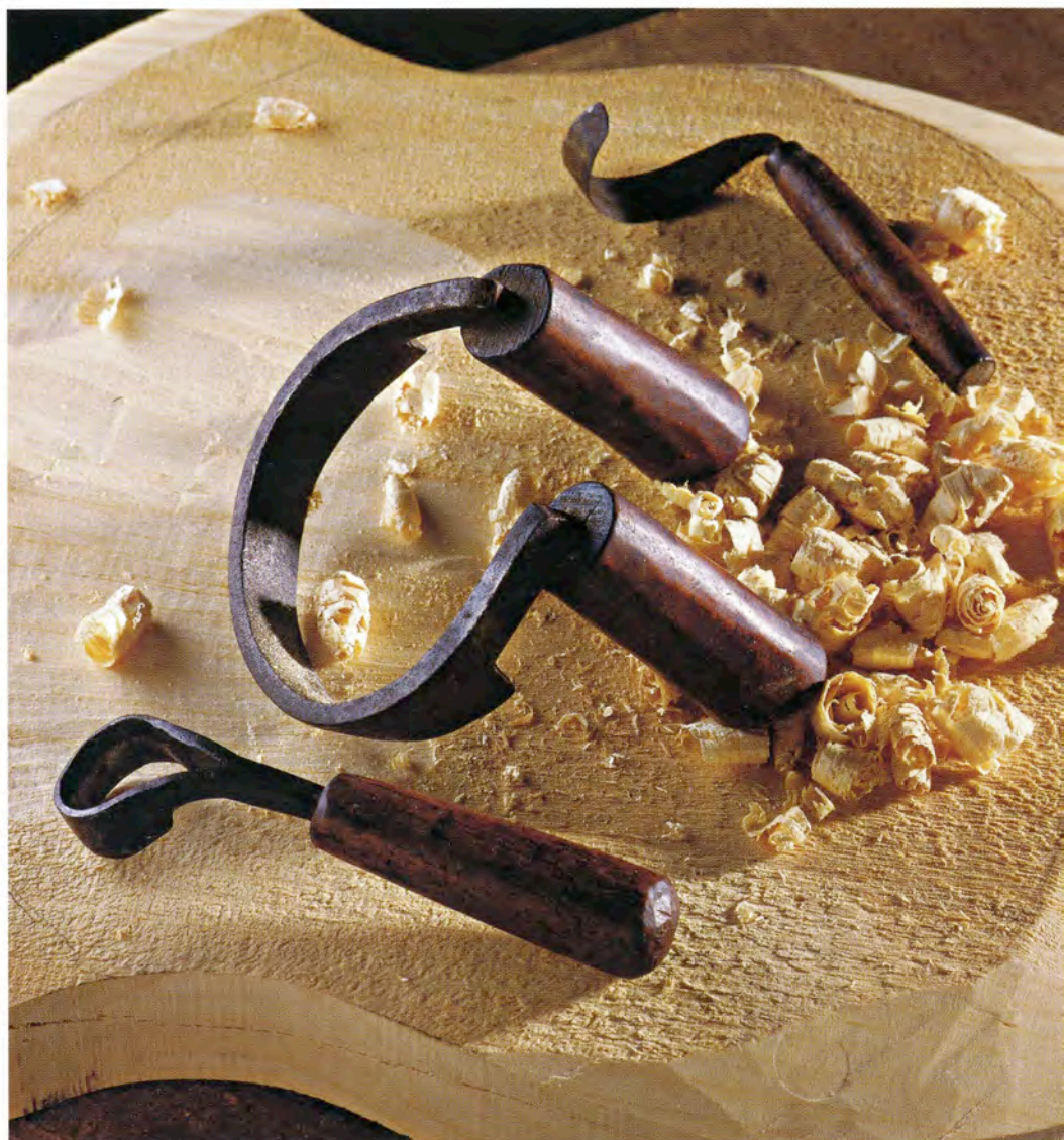
Sharpen a drawknife as you would a chisel, with about a 20° bevel and slight back bevel. It's easiest to hold the tool steady on a surface and bring the stone to the blade.
