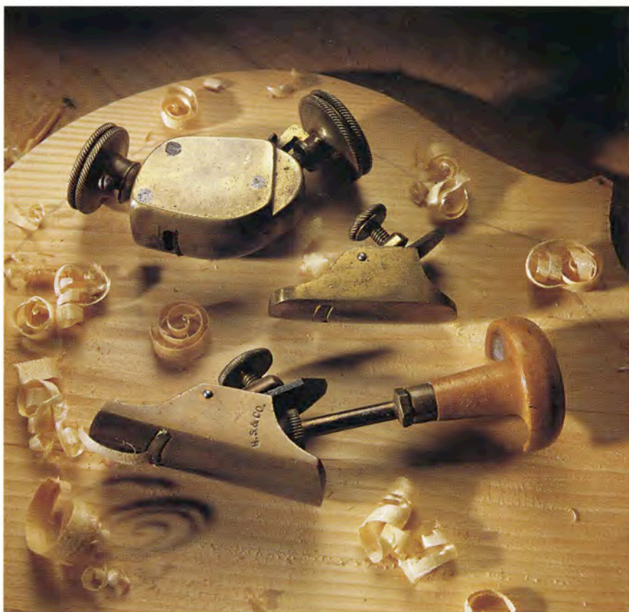
Among the tiniest planes are the violinmaker's hollowing planes for shaping the arched back and top of stringed instruments. A tail handle that snuggles into the palm of the hand helps give the user a firm grip.
