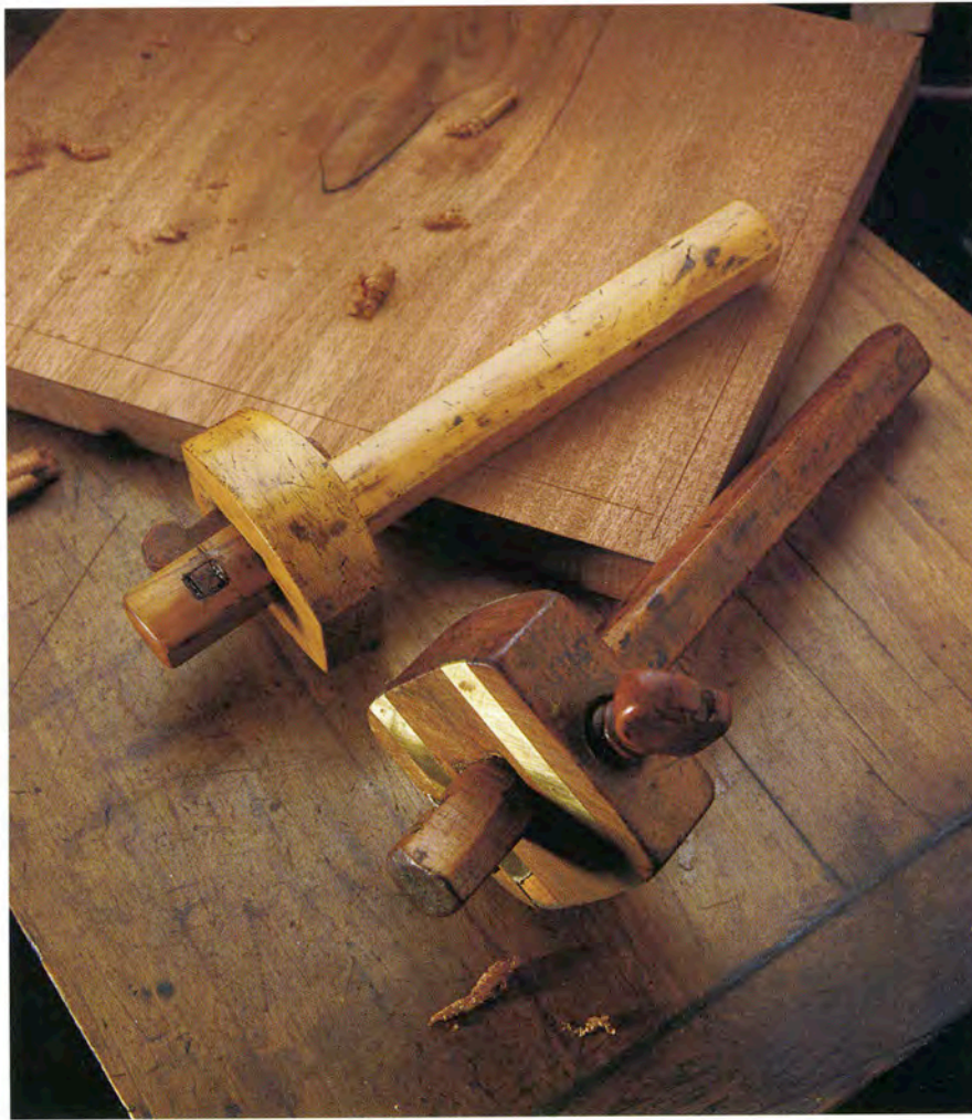
A gauge with a pin works well for cutting with the grain, but across the grain a knife scores the fibers more cleanly.
