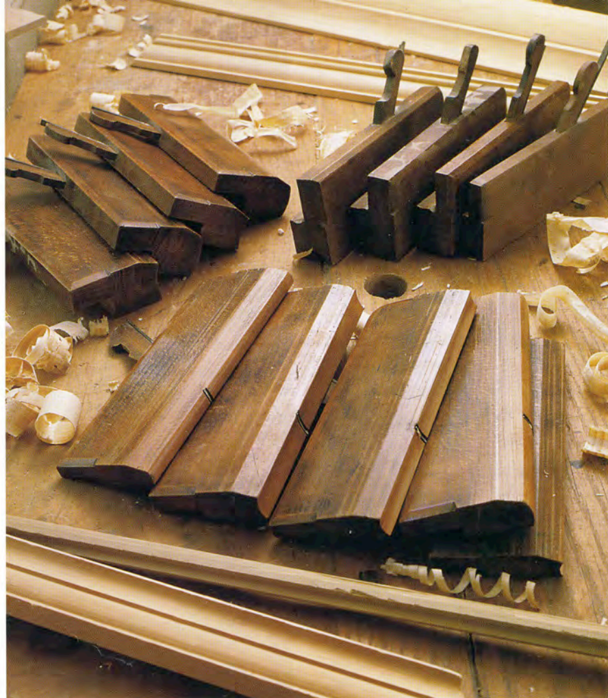
A small collection of hollow and round molding planes (plus a quarter-round, ogee, and ovolo at rear) can cut a wide range of decorative profiles. Molding planes were made by the thousands until the turn of the century.
