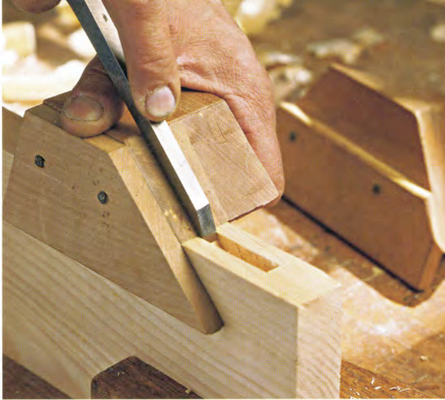
For cutting angled mortises accurately, a wooden block with a fence makes a good guide for your chisel. Use a chisel with a long blade, as wide as possible, and take paring cuts.
