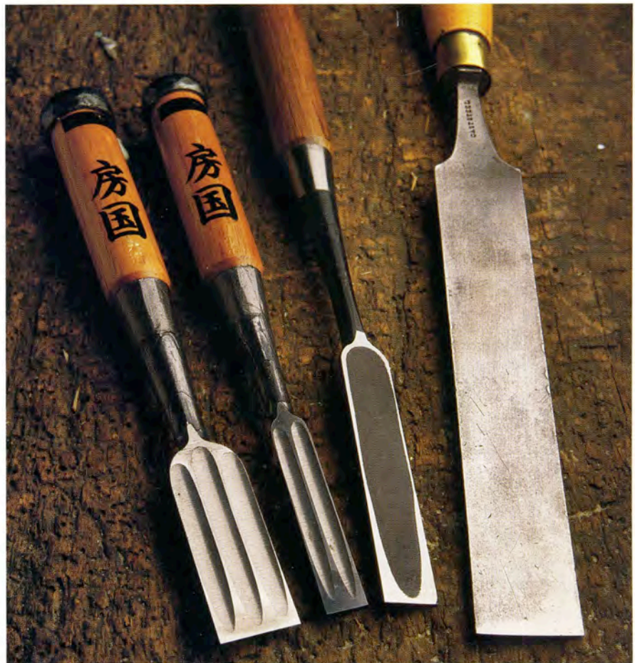
With blades as wide as 4 in. and handles 12 in. or more in length, slicks are the largest chisels, but they are capable of finer work than their size suggests. They were traditionally a shipbuilding tool, used to pare, level, and fit decking and frames.
