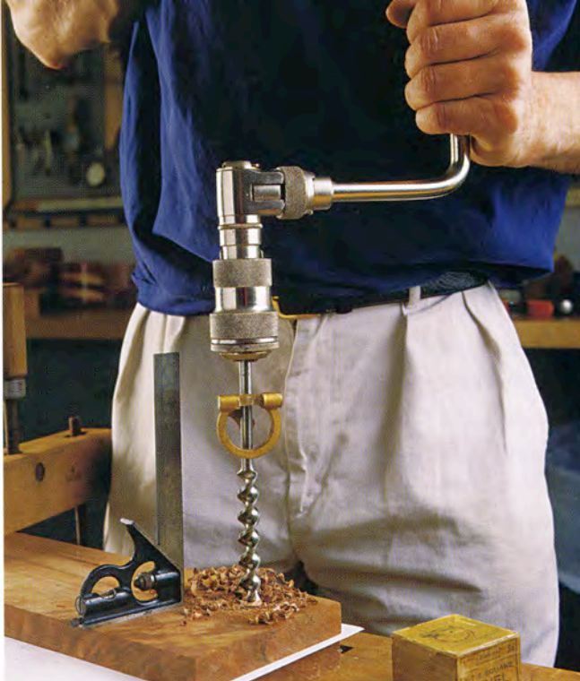
Useful for more than just drilling holes, braces can turn hollow augers, such as this one by A. A. Woods, used for cutting the round tenons on the ends of the bowback on a Windsor chair.
