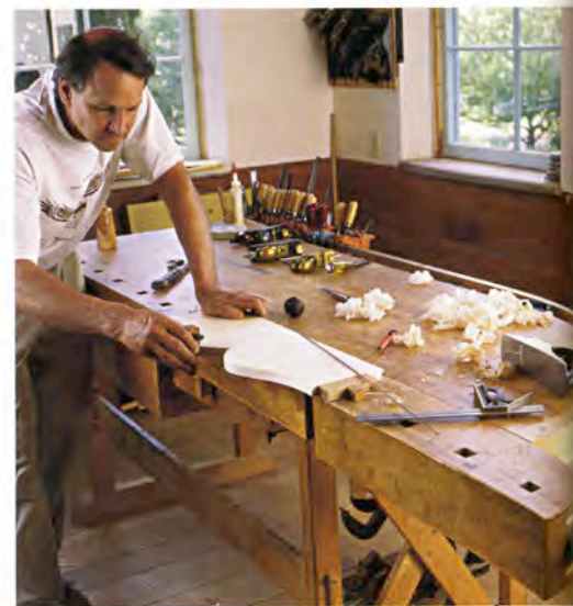
The large end or tail vise on the author's bench clamps work securely between wooden dogs, leaving him with both hands free to control the tool.
