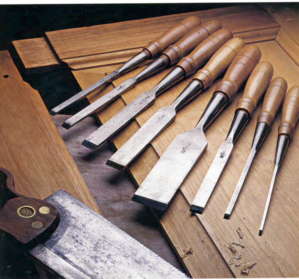
A typical set of bench chisels, ranging in size from \frac{1}{8} in. to 1\frac{1}{4} in., for chopping mortises, cutting tenons, or paring joints. This set was made by Buck Brothers, of Millbury, Mass., one of largest and best-known makers of chisels and gouges.
