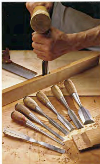
Stanley “Everlasting” beveled firmer chisels are easy to control, and the design of the tang makes for a very rugged chisel that can withstand hammer blows.
