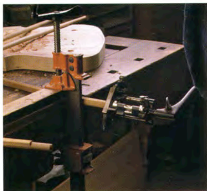
Useful for more than just drilling holes, braces can turn hollow augers, such as this one by A. A. Woods, used for cutting the round tenons on the ends of the bowback on a Windsor chair.
