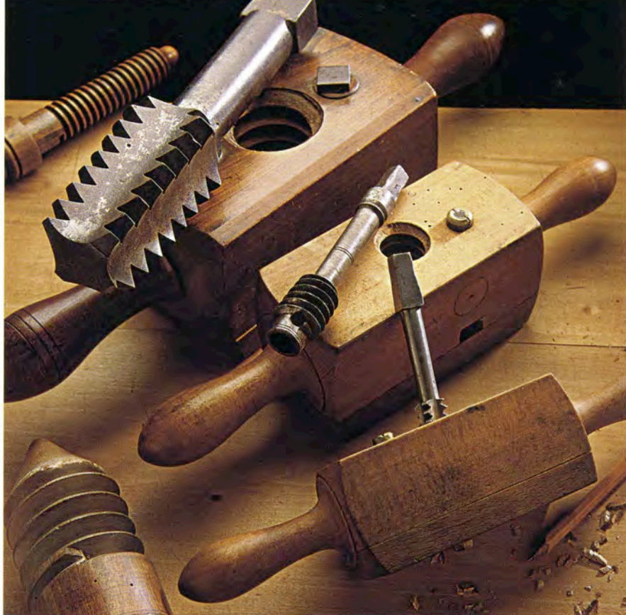
Taps and dies cut consistent wooden threads and mating nuts for such tools and tool parts as clamps, saw vises, and locking screws. An older hand-cut tap is at top; a modern continuous thread is in the foreground.
