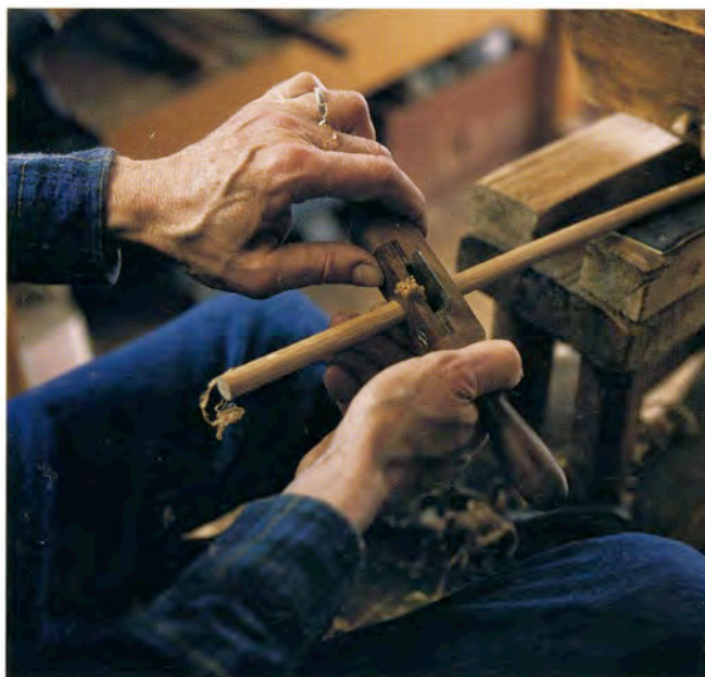
A chairmaker uses a few sizes of specialized shaves, or “devils,” for smoothing round parts such as spindles and legs. Placing a few fingers under the spindle helps to stabilize it and damp out vibration.
