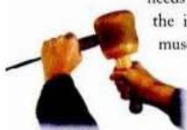
LEFT: Tap with the mallet while maneuvering the gouge.
