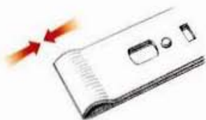
ABOVE: Setting the irons for finishing and hardwoods.
