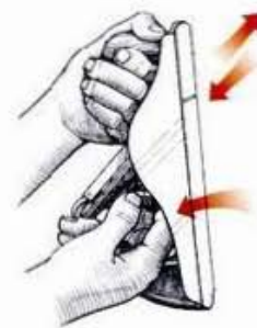
ABOVE: Adjust the depth of the cut by advancing or retracting the blade.
