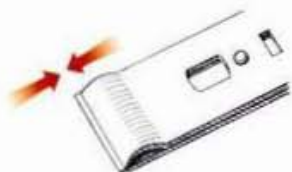
ABOVE: Setting the irons for rough work.
