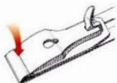
ABOVE: The lever cap must be a flush fit on the cap iron.
