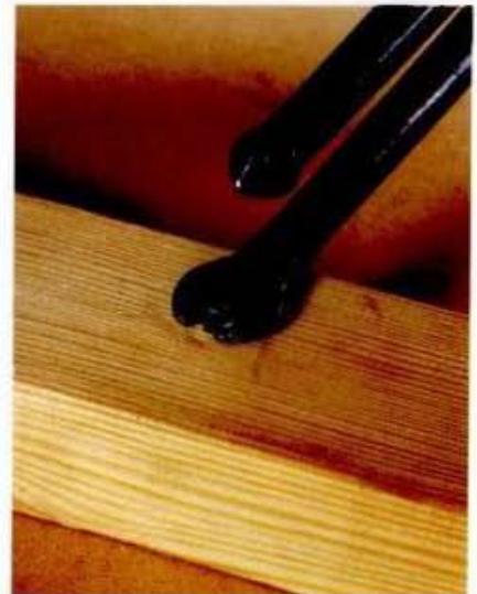
ABOVE: The split end of the handle is designed to be used as a tack extractor.
