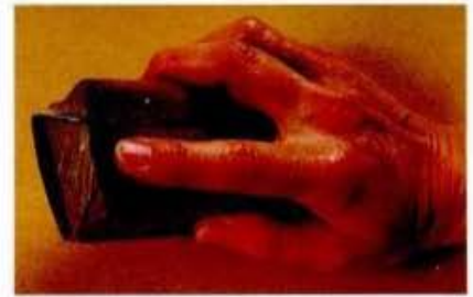
ABOVE: A clever little block device, made in the 1950s, that holds a sheet of sandpaper.
