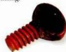
ABOVE: Boxwood is extremely close, even and dense in its grain – good for complex forms that show a lot of short grain.
