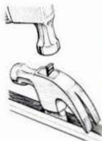
ABOVE: Securing a new handle with a wedge.
