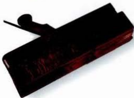
RIGHT: Triple-reed – a good quality plane with a fully-boxed sole.
