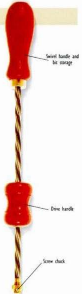
ABOVE: Archimedean drill, also called a fret drill, is used for boring small-diameter holes in thin-section wood.
