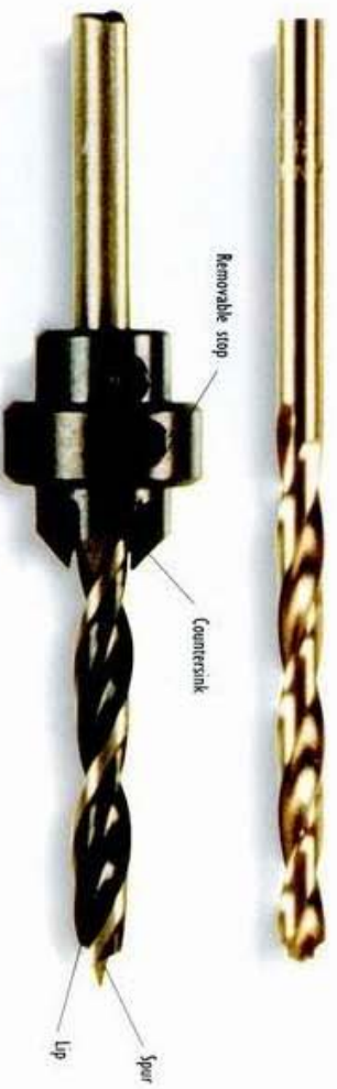
TOP: Twist drill bit. BELOW: Combined lip and spur drill bit with countersink – good for countersinking and boring at the same time.
