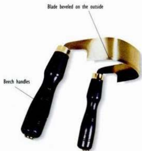
ABOVE: The inshave or scorp is the perfect tool for hollowing out dishes and bowls.
