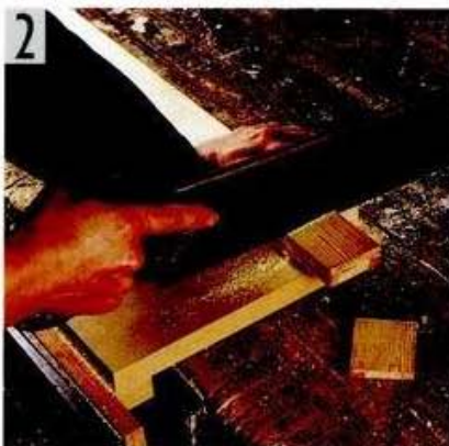
ABOVE: The handle of the dovetail saw is designed for maximum comfort. The notch at the top of the handle enables the woodworker to point and hook his index finger for optimum control.
