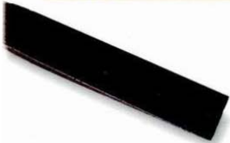
ABOVE: Flat-backed pattern maker's chisel
