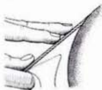
ABOVE: Grinding the primary bevel.
