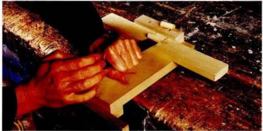
ABOVE: The bench hook stop prevents tool-exit damage.
