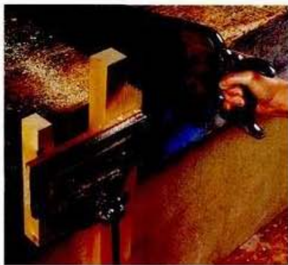
ABOVE: The wood set to the left of the vise screw saves the mechanism from damage.
