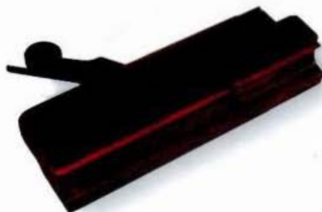
LEFT: Ogee plane – with characteristic flat "s" profile and inset "quirk" slip.
