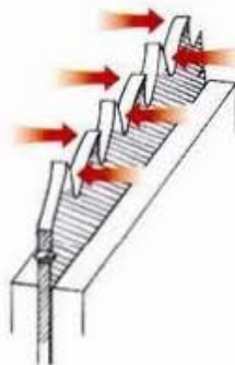
ABOVE: Setting the rip saw.
