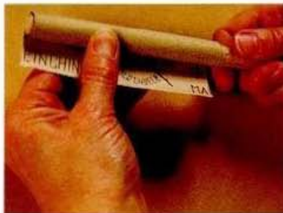
ABOVE: Dowels make good sanding sticks – perfect for cleaning out concave curves.
