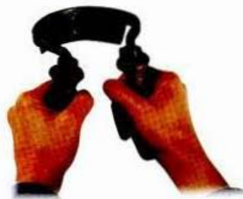
ABOVE: Hold the drawknife with well-braced arms, and clear the waste with a series of short, shallow slicing strokes.
