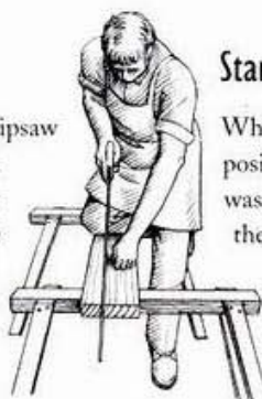
ABOVE: Using the rip saw – front view of correct stance.
