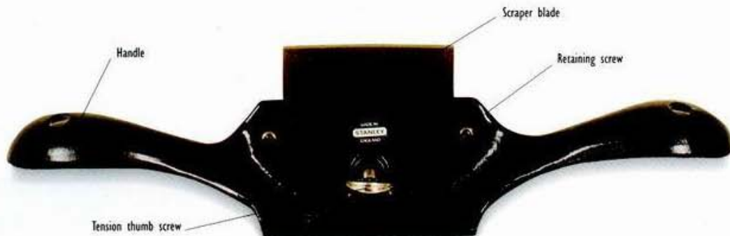
ABOVE: The design of the scraper plane means that it can be used for long periods without cramping or fatigue.
