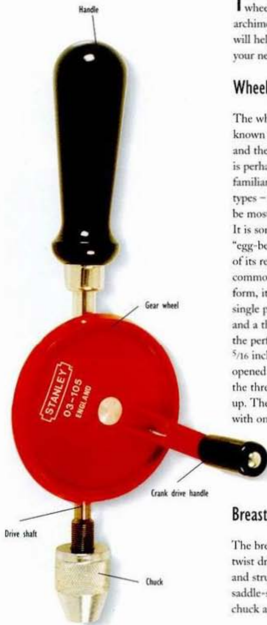
ABOVE: Single pinion hand drill with die-cast gear wheel.
