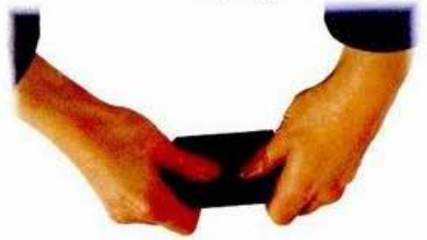
ABOVE: Bow the scraper with your thumb until it begins to “feel and bite.”
