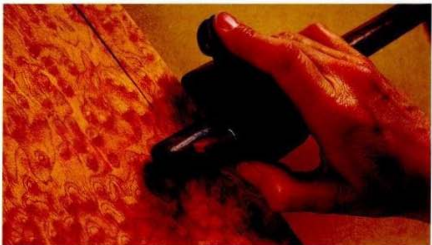
ABOVE: Repeatedly run the gauge along the edge until the veneer is cut through.
