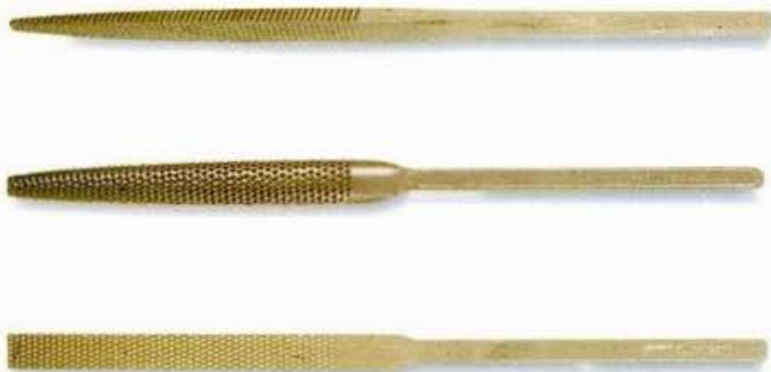
ABOVE: Three carver's rasps – each forged from one piece to create an integral handle.
