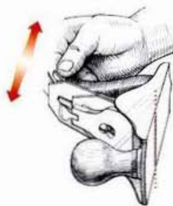
ABOVE: Move the lateral lever left or right to set the iron square in the mouth.
