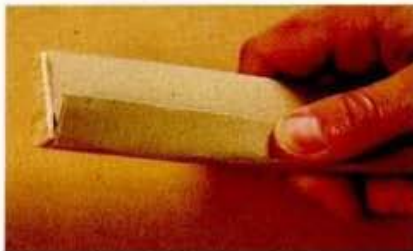
ABOVE: If you need to clean out a narrow slit, a good technique is to wrap the sandpaper around a strip of plywood.
