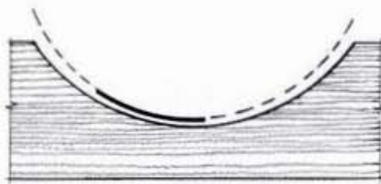
ABOVE: Adjust the sole to a smaller curve than the workpiece when working concave shapes.
