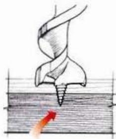
ABOVE: The lead screw drags the body of the bit into the wood
