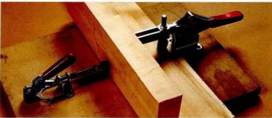
ABOVE: Toggle clamps screwed to a base board make a good jig board.
