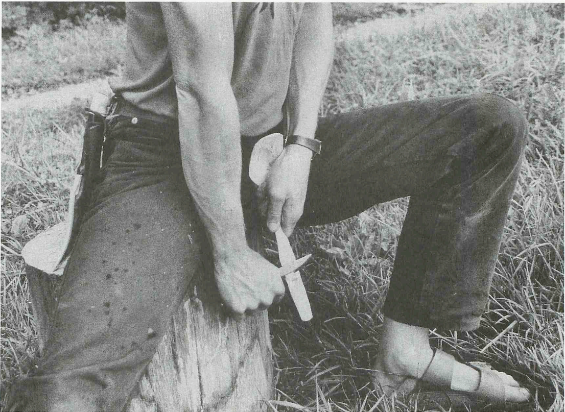
Jogge Sundqvist demonstrating the most basic grasp, used for large shavings. Be sure to slice across the blade as you push outward.
