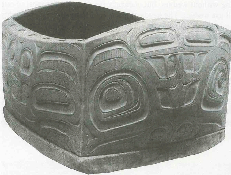
A northwest coast Indian box made from rived yellow cedar. The sides are a single plank which is kerfed at the corners, then steamed and folded. The fourth corner, and the bottom board, are secured with angled pegs.
