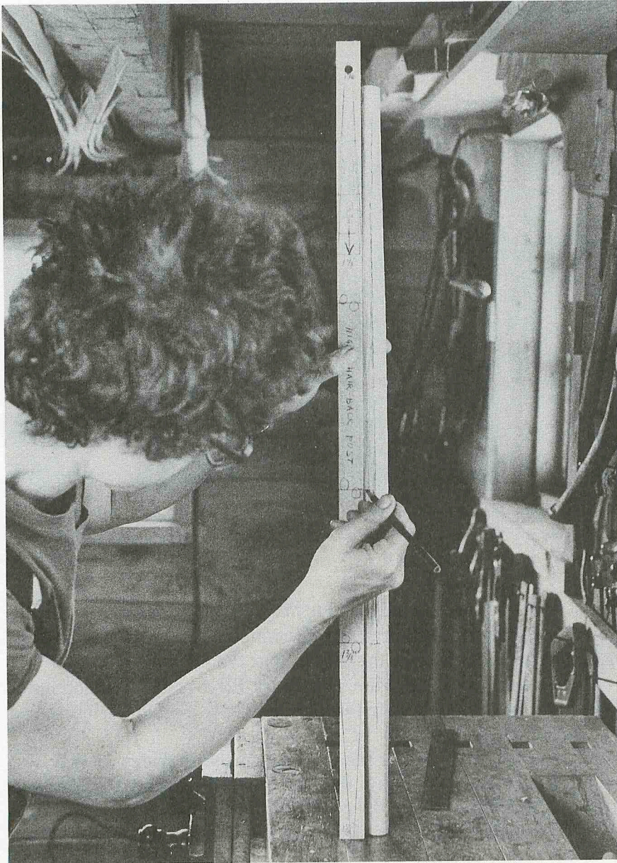
Using a chair stick to locate boring tangents on the back posts of Naomi's high chair. Make a separate stick for each design that you build.
