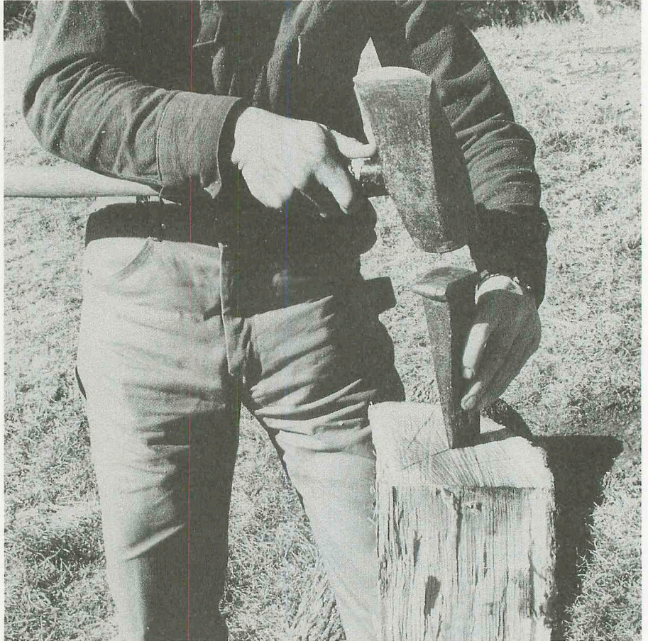
To split short stock, such as chair posts, it's much easier to stand the log on end.
