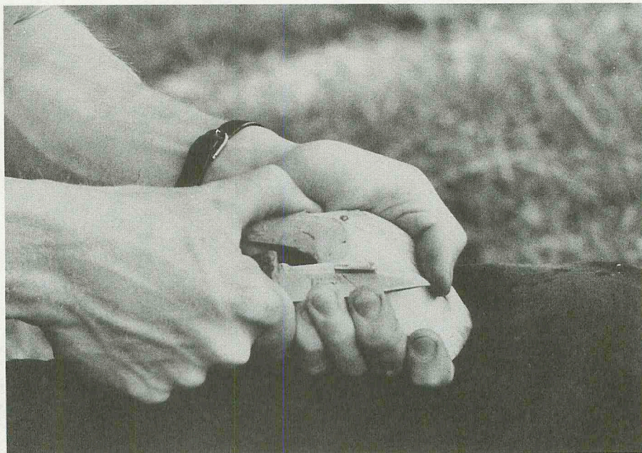
Using this two-handed grasp, the right thumb acts as a pivot point. Fingers of the left hand provide additional force.
