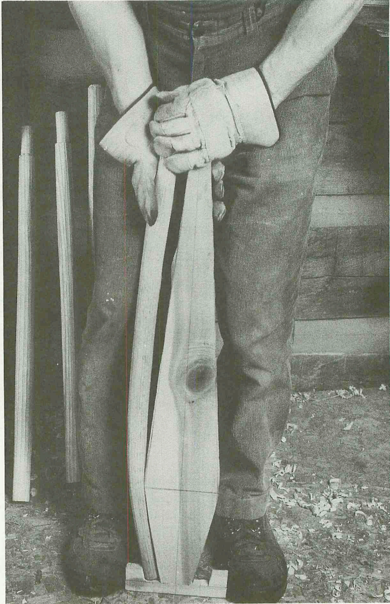
Jigging a ladder-back post. A second post will be bent on the other side. The posts are held in place with pre-knotted loops of twine.
