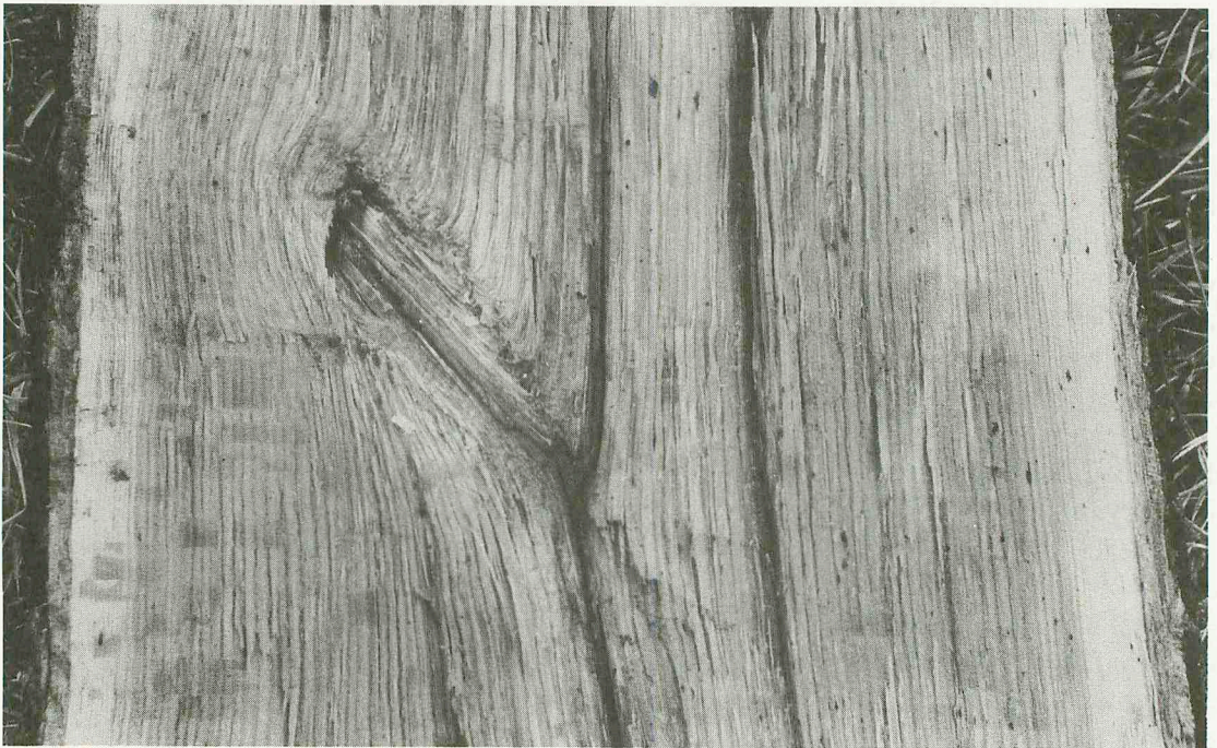
This split log shows how branches (and knots) originate at the pith. Note the distorted grain surrounding the knot.
