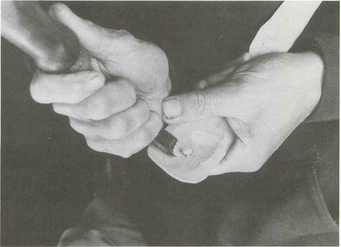
Hollowing a spoon. The left thumb acts as a fulcrum and a safety stop for the gouge.
