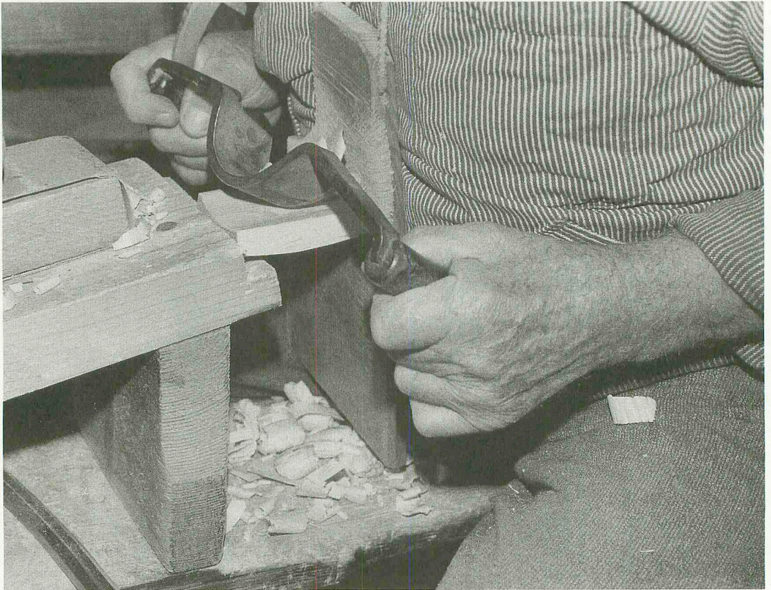
Hollowing a very short bucket stave. Wood is secured between a breast bib and a ledge at the end of the shaving horse bridge.
