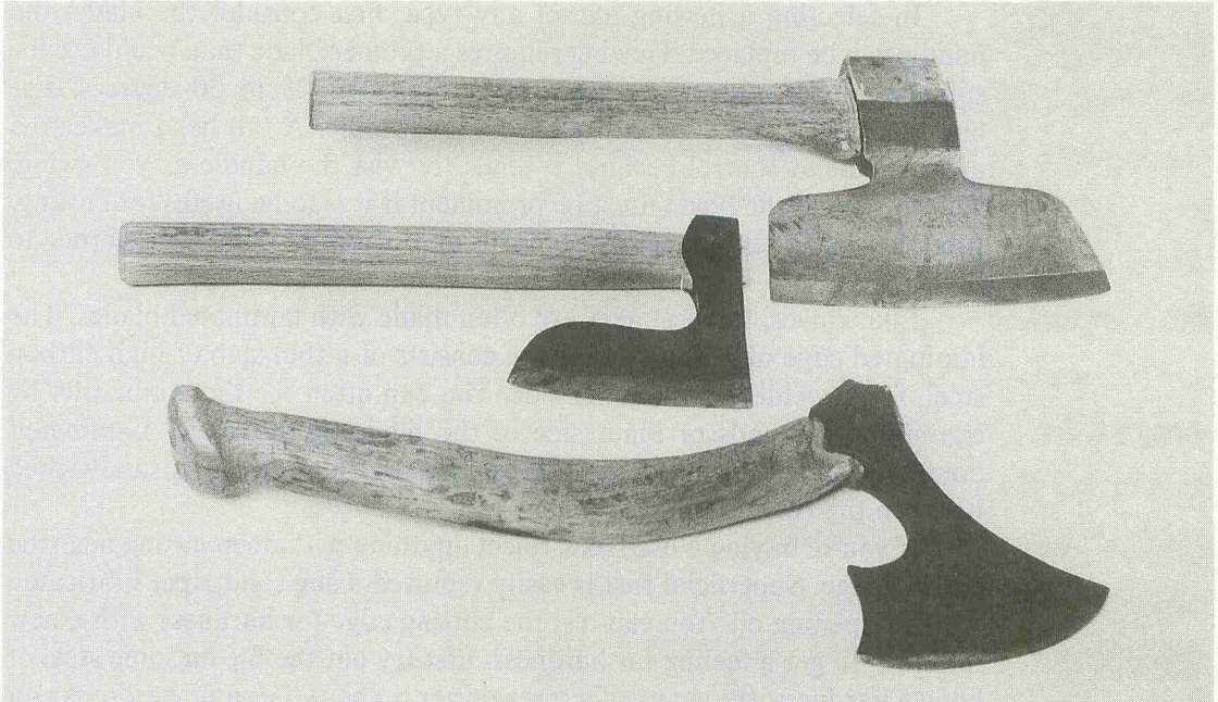
Three of my favorite bench axes. The axe at the top is a broad hatchet, made in Germany before World War II. It has a single bevel and a laminated blade. The middle axe is a Japanese carpenter's hatchet. The lower hatchet is a reproduction of a 12th century Viking axe from Sweden. The blade is double beveled.
