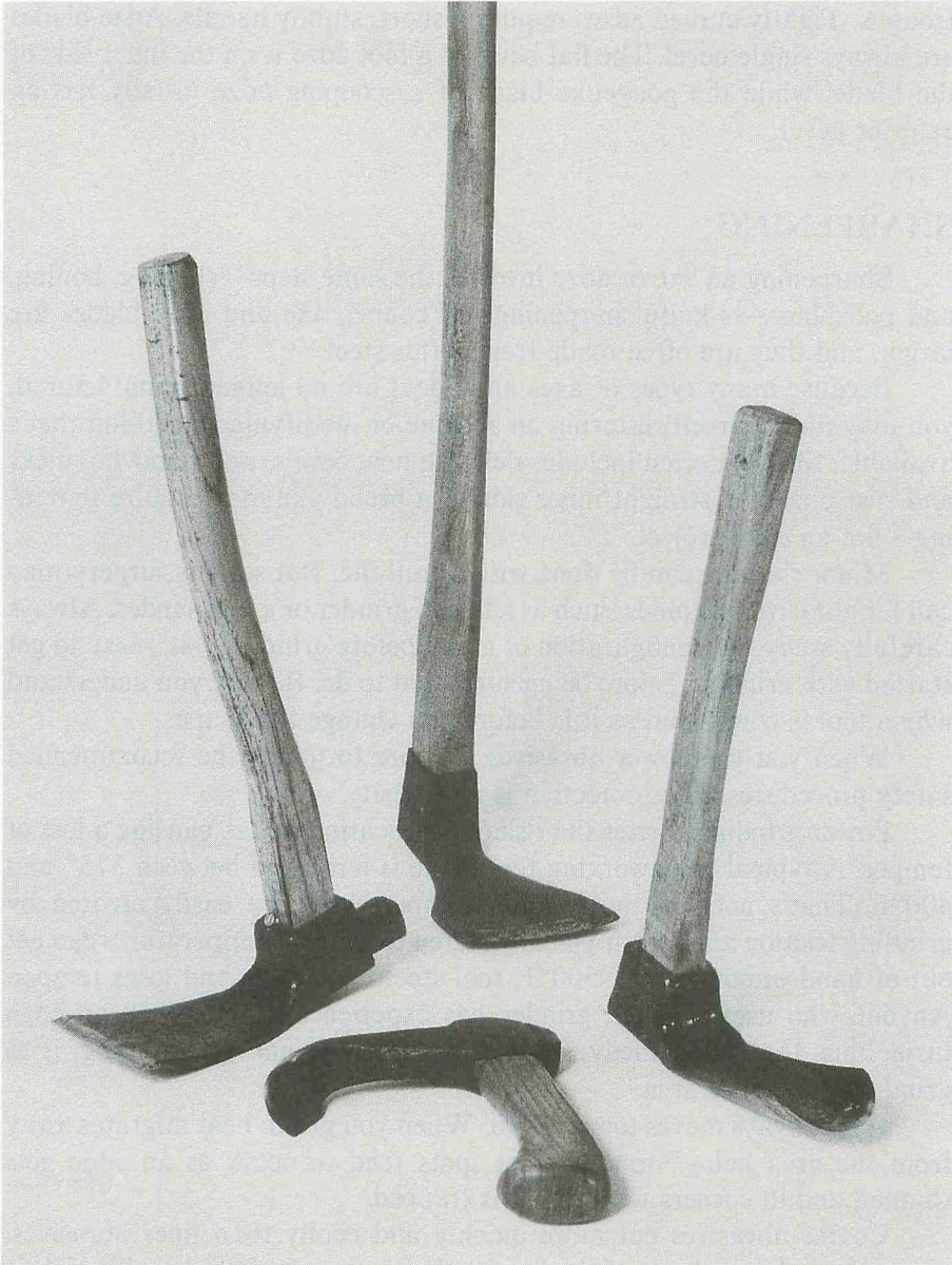
A flat-bladed hand adze (left) and a foot adze (top, center) have a single bevel on the inner side of the blade. Hollowing hand adzes (right and bottom) usually have an exterior bevel.
