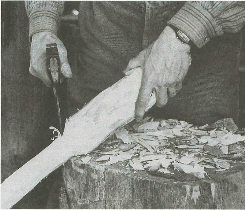
Hewing the handle of a small root club. The edge of the chopping stump is directly below the axe blade.
