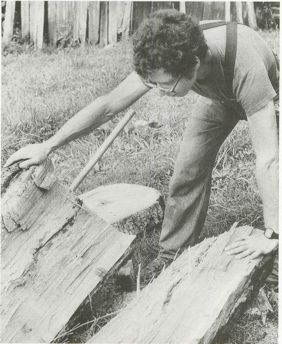
Green woodworking often begins by splitting stock from a log. This red oak will be converted into ladder-back chair parts.
