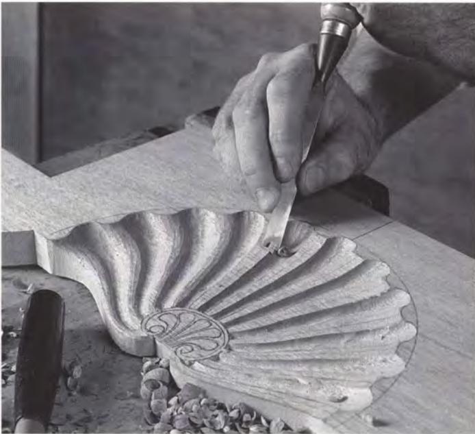
A flat chisel is used to round the convex lobes of the shell.
