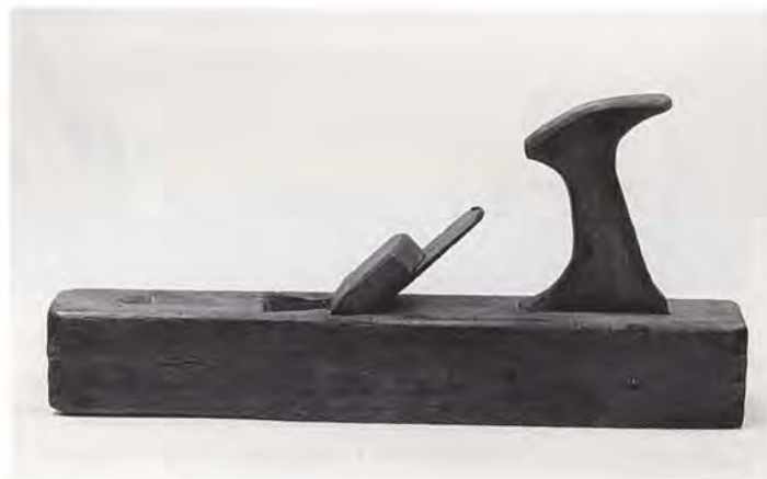
Measuring from 12 in. to 18 in. long, the fore or jack plane was used to flatten and true rough-sawn lumber and to plane it to the appropriate thickness. (COURTESY BUD STEERE)
