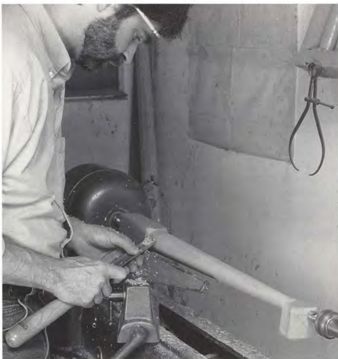
The taper of the leg is turned first, using the center points for the skewed axis.
