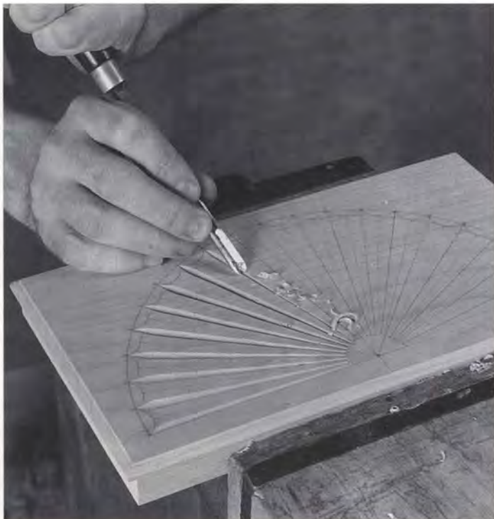
A V-shaped carving tool is used to cut a channel between the rays of the fan.
