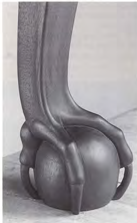
The completed ball and claw foot. Wetting the foot with water offers a preview of what the foot will look like with a more lustrous finish.
