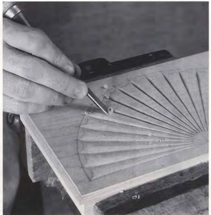
Each ray is rounded with a flat chisel.
