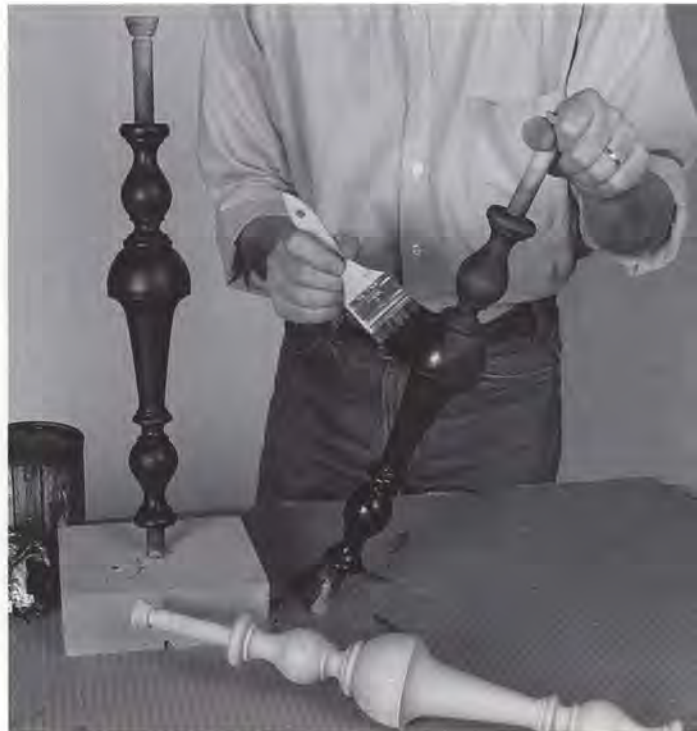
Ebonizing is the application of a heavily pigmented black oil paint/stain to simulate ebony. It is brushed on and the excess is rubbed off, leaving a soft luster on the wood. The process is repeated as needed to reach the desired opacity.
