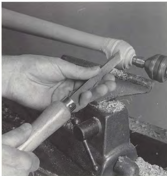
The leg is remounted on its true centers to turn the bottom of the foot.
