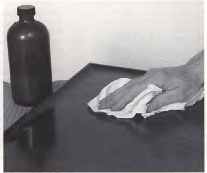
The final step in finishing is to polish the surface. Here, a linseed-oil polish has been applied and buffed off.
