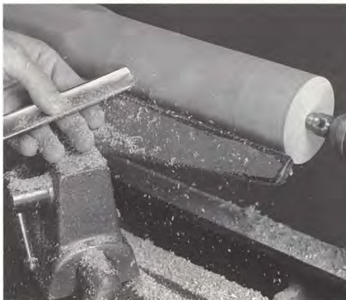
The square or octagonal workpiece is first turned to a cylindrical shape with a large gouge.
