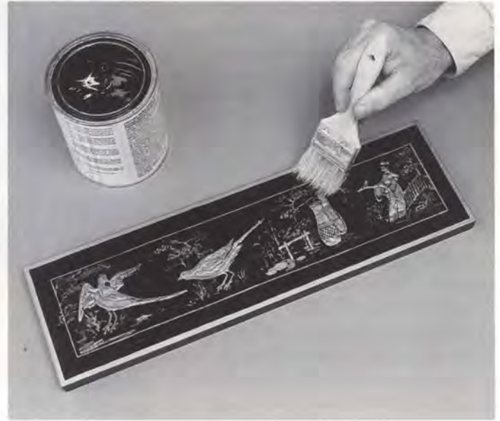
Several coats of a spirit varnish are applied to seal the work.
