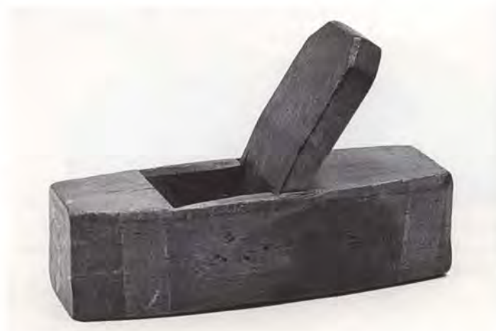
Smoothing planes, which measure from 7 in. to 9 in. long, were used for smoothing primary surfaces. This smoothing plane was made by Cesar Chelor, slave of Wrentham, Massachusetts, plane maker Francis Nicholson, some time between 1753 (when Chelor was given his freedom) and 1784 (when he died). (COURTESY BUD STEERE)
