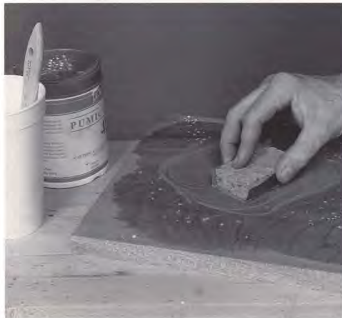
Using waterproof silicon-carbide sandpaper and powdered pumice to fill the pores of an open-grained wood simulates the original method, which called for rubbing the surface with a solid block of pumice.
