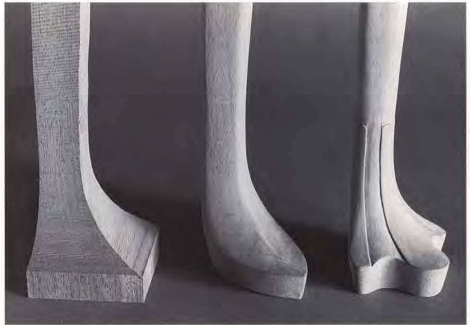
Cabriole legs with slipper feet or trifold feet begin in the same manner as those with pad feet (left). With slipper feet (center), the foot is shaped to a tapered teardrop shape rather than turned. Trifold feet are similar but are cut to a three-toed pattern with chisels and gouges (right).
