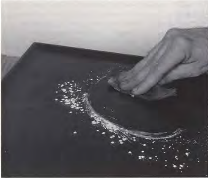
The luster of the finish is increased by rubbing it with finer pumice or rottenstone lubricated with oil. Here, mineral oil and mineral spirits, mixed in equal parts, serve as the lubricant.
