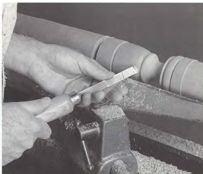
The shape between the diameters is turned with skews and gouges.
