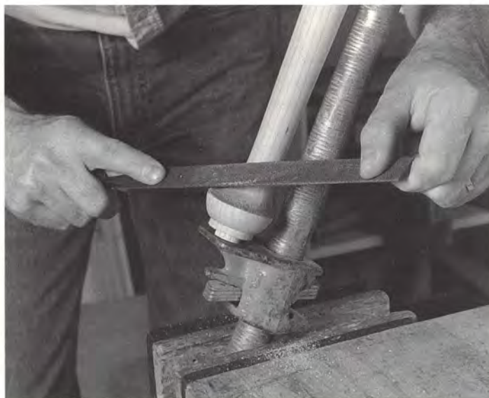
The top of the foot is shaped with rasps and files, as on the pad feet of cabriole legs.
