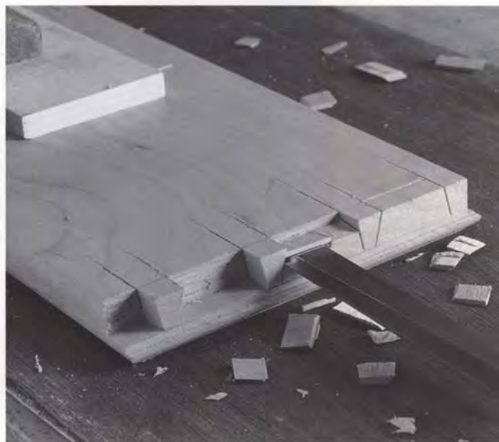
Since the front dovetails are half-blind, the material between the pins must be chiseled away in layers and trimmed to the scribed lines.
