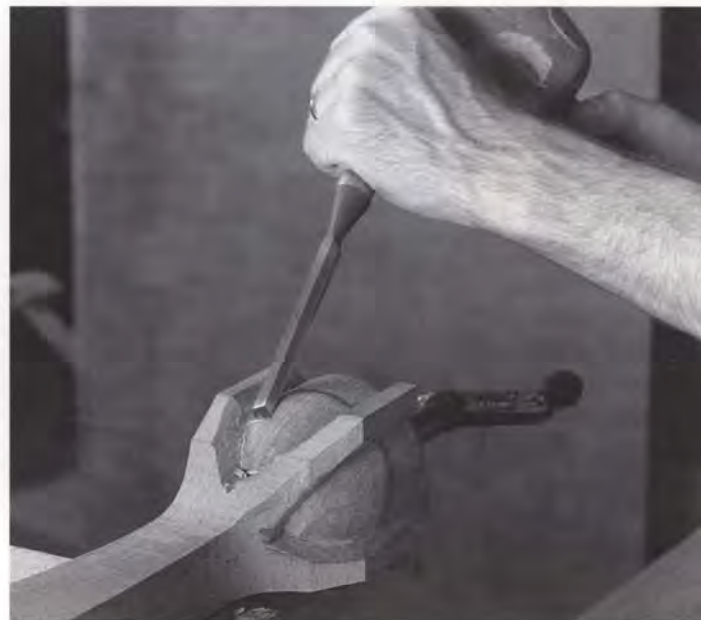
The midpoint of the ball is drawn on the cylinder and the top of the ball is cut to a hemispherical shape. The claws are left uncarved until the ball has been fully shaped.
