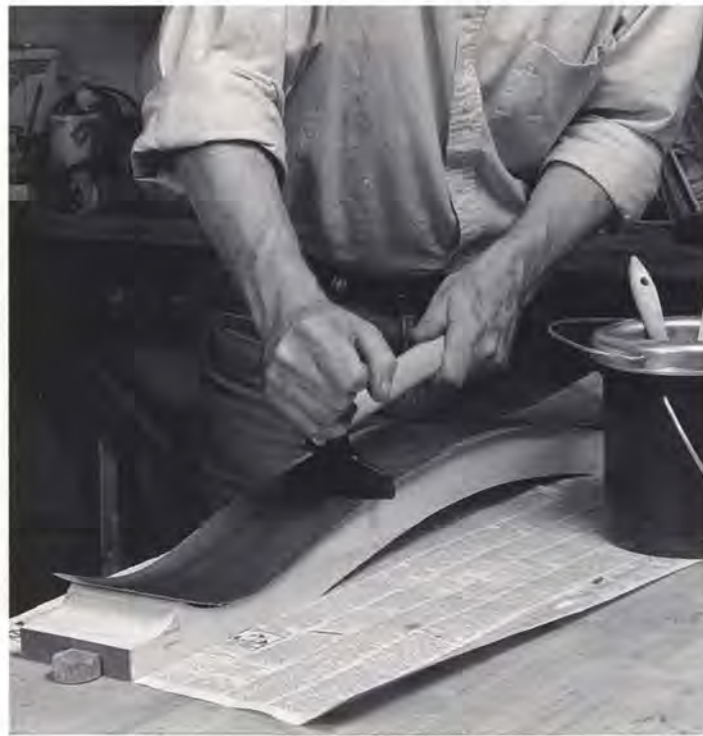
A veneer hammer is the traditional tool used to press thin veneer into place and force out excess glue.
