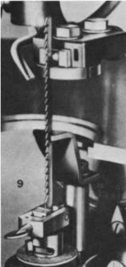
Figure 7-19 Saber saw blades might be used without being chucked in at the top. This can be convenient when making certain cuts. (Courtesy of Rockwell)
