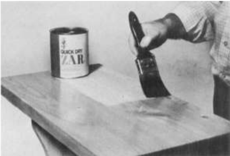
Figure 5-21 Polyurethane dries in an hour. It is good on unpainted wood. (Courtesy of United Gilsonite)
