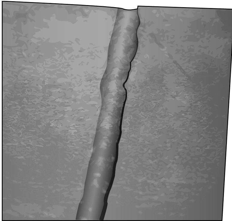
Figure 18-3: Example of a crack along a weld.
