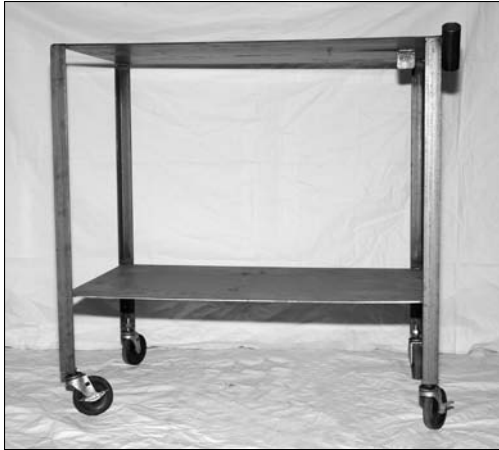
Figure 16-5: A completed portable welding table.
