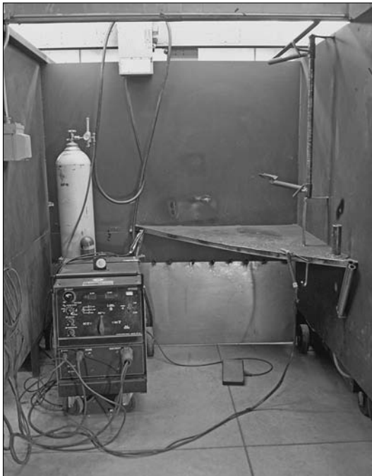
Figure 7-1: A tig welding setup.
