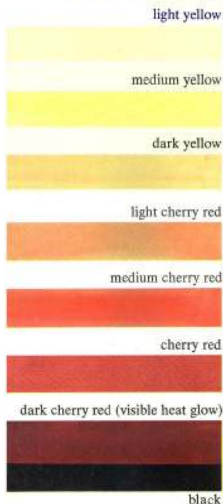
Heat-glow colors of steel as seen in a semi-dark shop allow the smith to judge malleability during forging, and hardness at moment of quenching.
