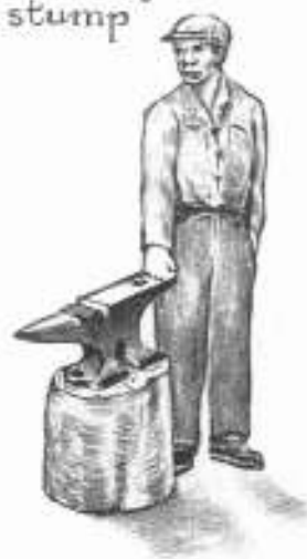
correct height of anvil on stump
