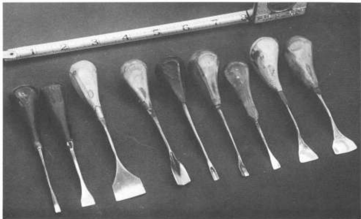
These small woodcarving gouges are designed to be manipulated in the manner of engravers' burins.
