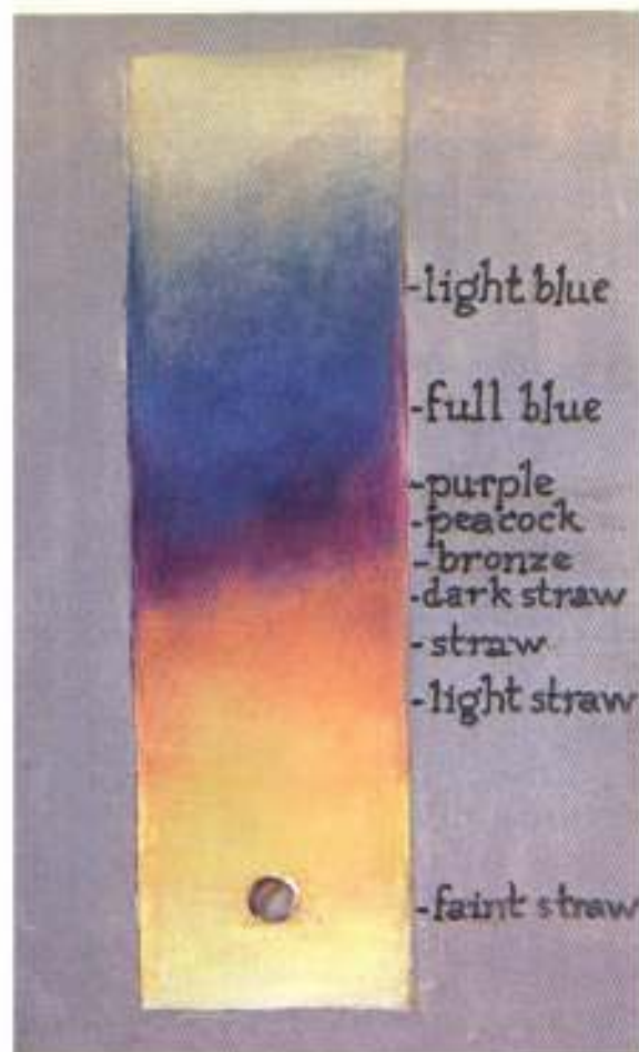
Graduated colors in the oxidation spectrum on polished surface of brittle-quenched high-carbon steel are used as hardness indicators in a tempering process.
