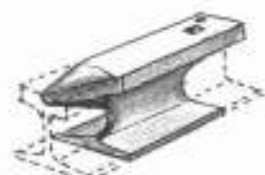
anvil made from scrap railroad rail
