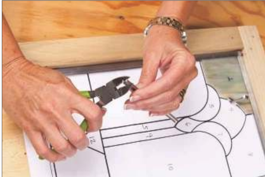
Figure 9-26: Securing your first glass piece with spacers and horseshoe nails.
