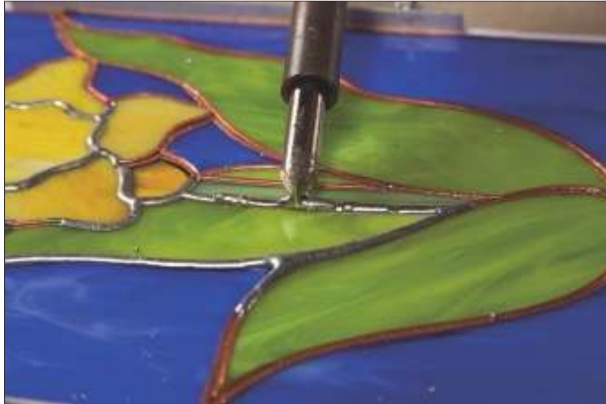
Figure 7-9: Reintroducing the iron to a seam for repairs.
