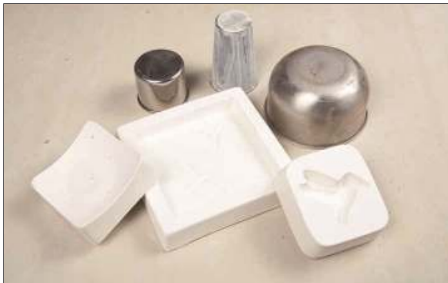
Figure 13-4: A collection of ceramic and stain- less steel molds for slumping glass.
