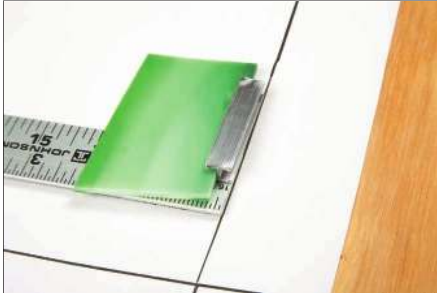
Figure 4-9: Measuring cut size by inserting glass into an H-shaped came.
