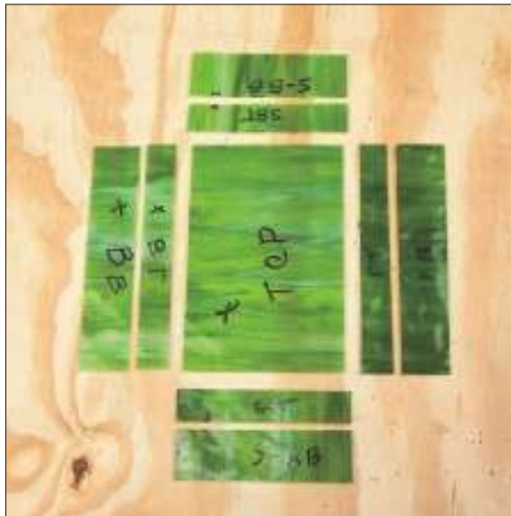
Figure 10-13: Glass pieces cut to size and laid out ready for assembly.
