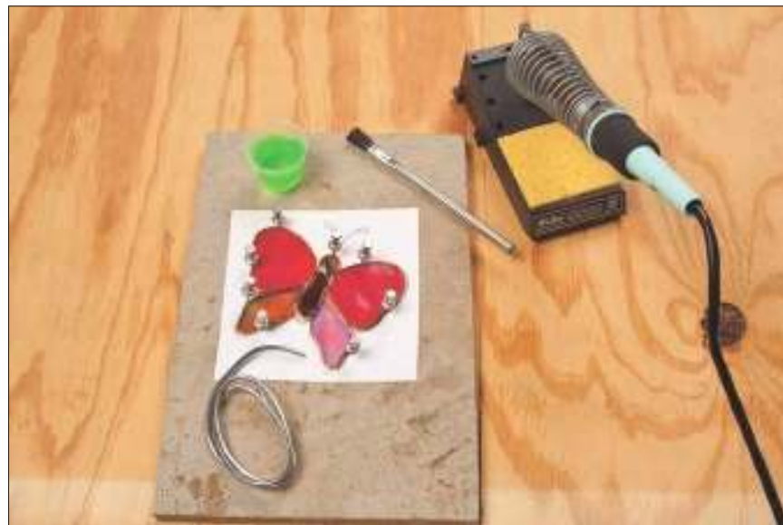
Figure 8-10: Stained-glass project, soldering iron, brush, flux, and coiled solder ready to use.
