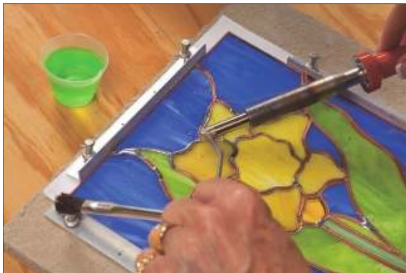
Figure 7-6: Running a bead of solder on a copper-foil project.
