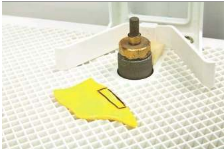
Figure 6-6: Marking glass before making adjustments with the grinder.
