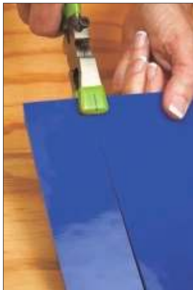
Figure 5-12: Completing the break with running pliers.
