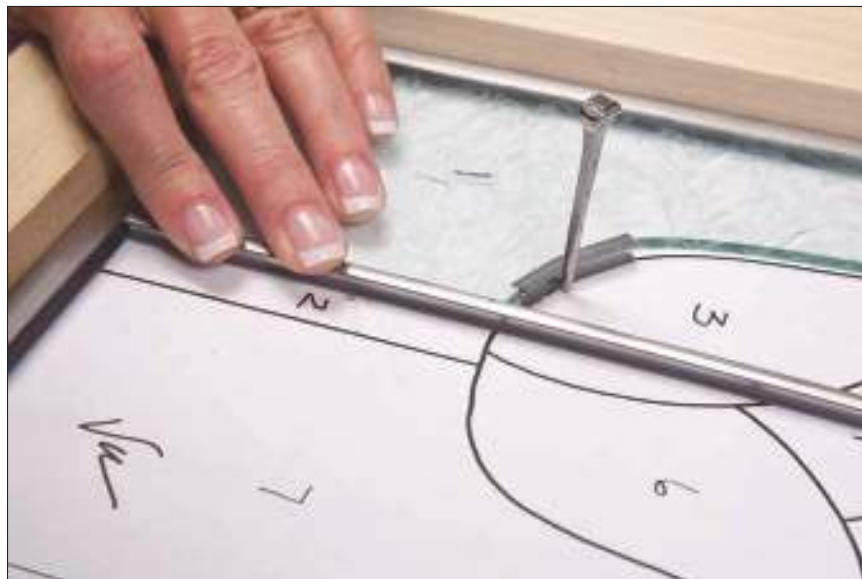
Figure 9-9: Using a scrap piece of lead to mark where to cut an intersecting lead came.
