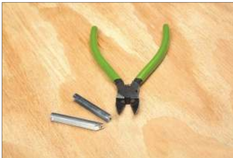
Figure 2-19: Lead nippers and some angles they can cut.
