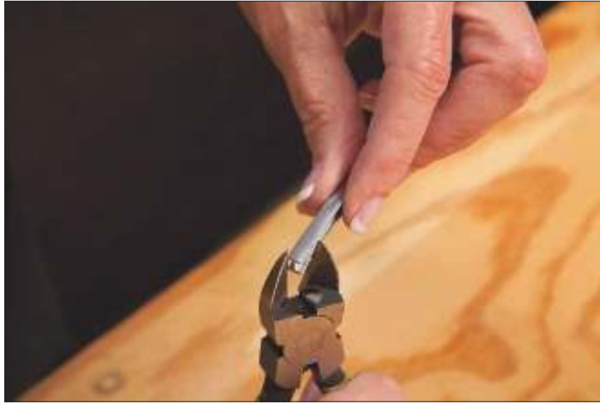
Figure 9-5: Proper position for cutting a slight angle with lead nippers.
