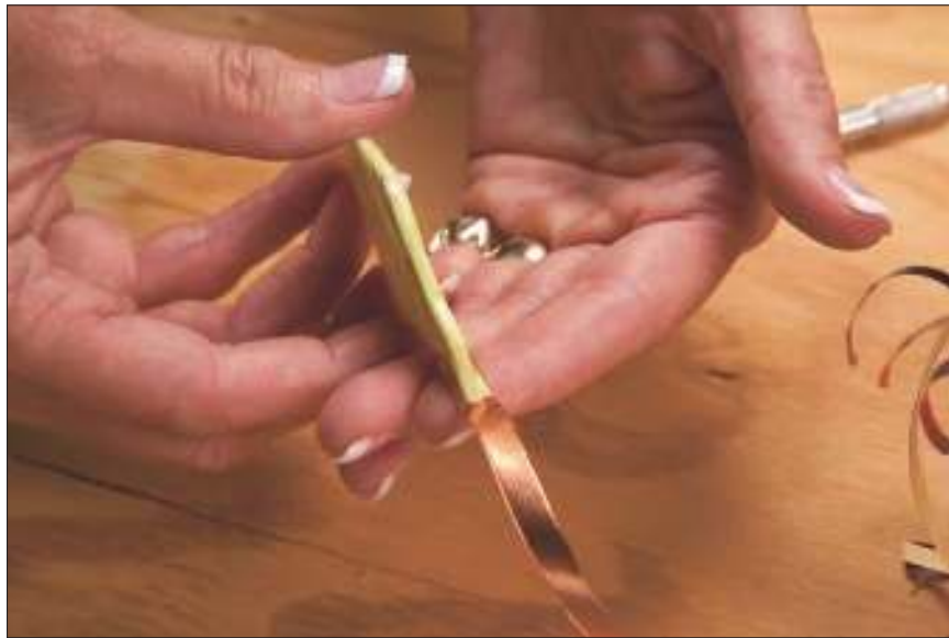
Figure 8-6: Centering a glass piece on the foil.
