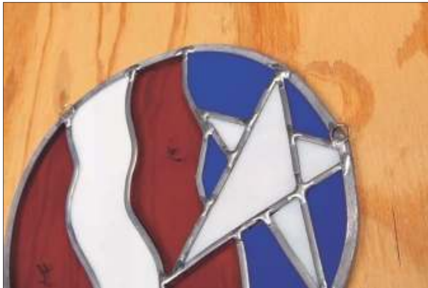
Figure 9-33: The back of the panel with hang- ing hooks soldered in place.
