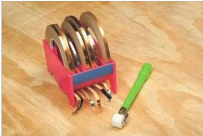
Figure 2-21: Foilmate roller and foil dispenser loaded with rolls of foil.
