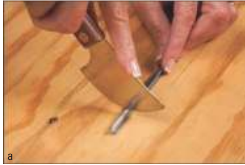
Figure 9-3: Incorrect versus correct cutting posi- tions when using the lead knife.
