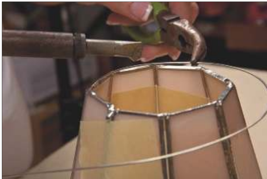
Figure 11-8: Tack soldering the wire to the top of the shade.
