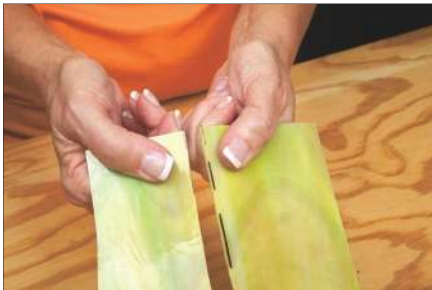
Figure 5-8: Rotating your hands to break the glass.
