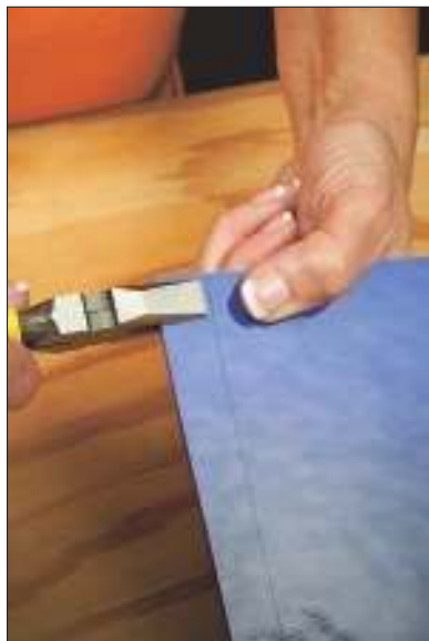
Figure 5-9: Positioning breaking pliers to break the glass.
