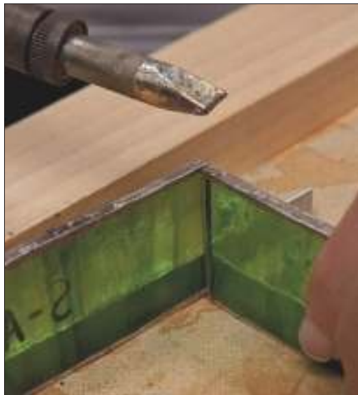
Figure 10-16: Tack soldering the box sides together.
