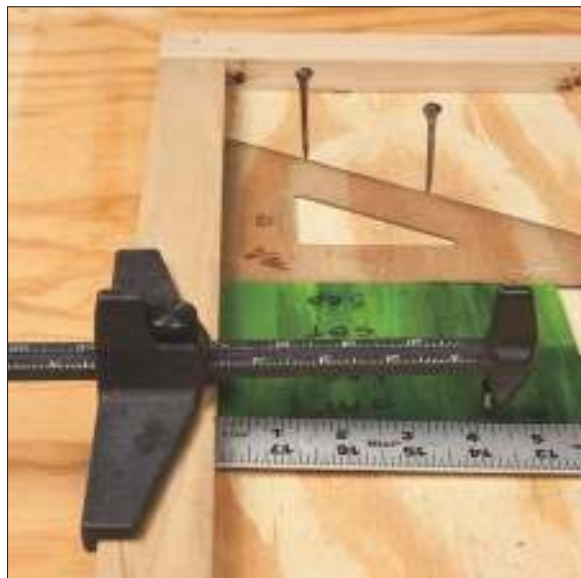
Figure 10-11: Side pieces ready to be trimmed to 4\frac{1}{4} inches.
