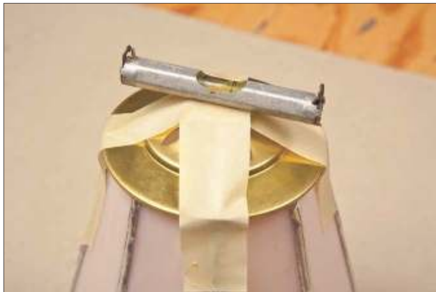
Figure 11-13: Temporarily securing the vase cap on top of the shade.
