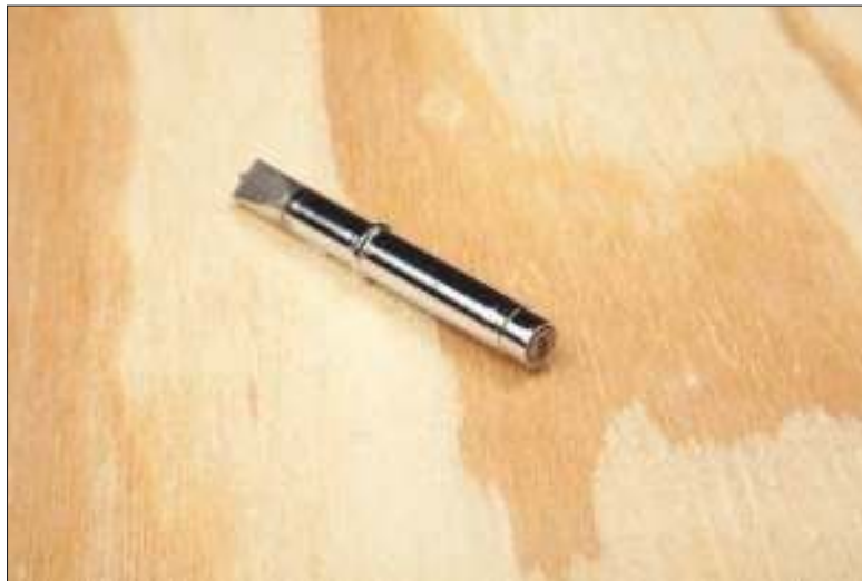
Figure 2-8: A thermo- statically controlled iron tip showing its temperature number.
