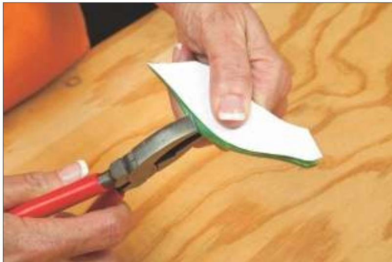
Figure 6-3: Using grozing pliers to nip at excess glass edges.
