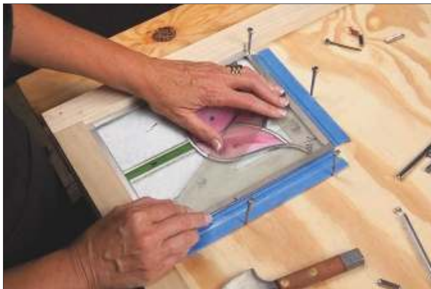
Figure 9-11: Checking a leaded panel for square corners.
