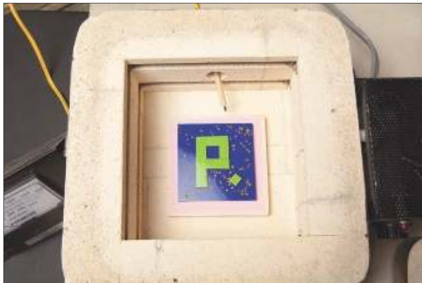
Figure 14-3: Placing a project on a small kiln shelf in the kiln.
