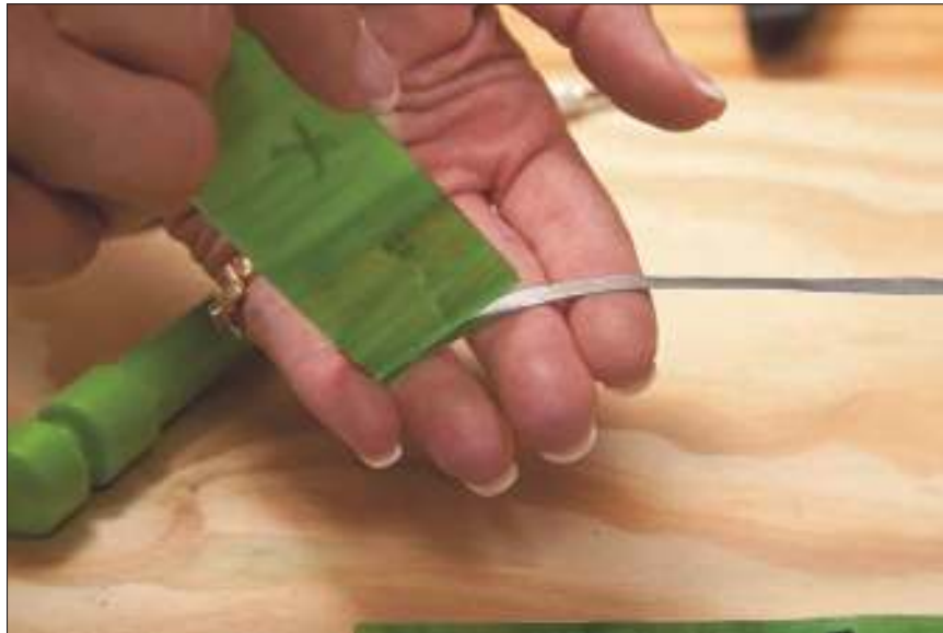
Figure 10-14: Applying copper foil.
