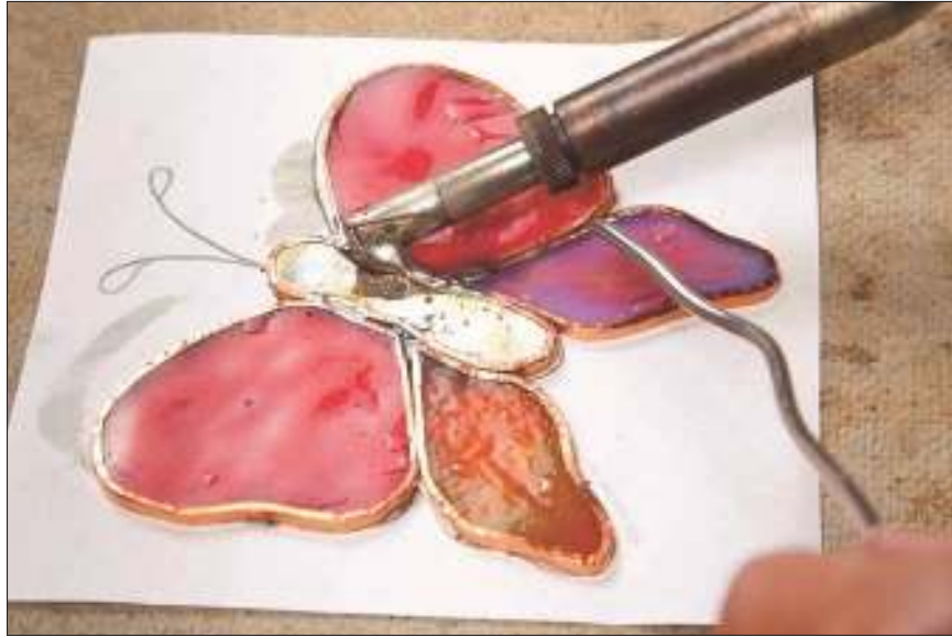
Figure 8-13: Creating a pool of hot solder and dragging it down the foil seam.
