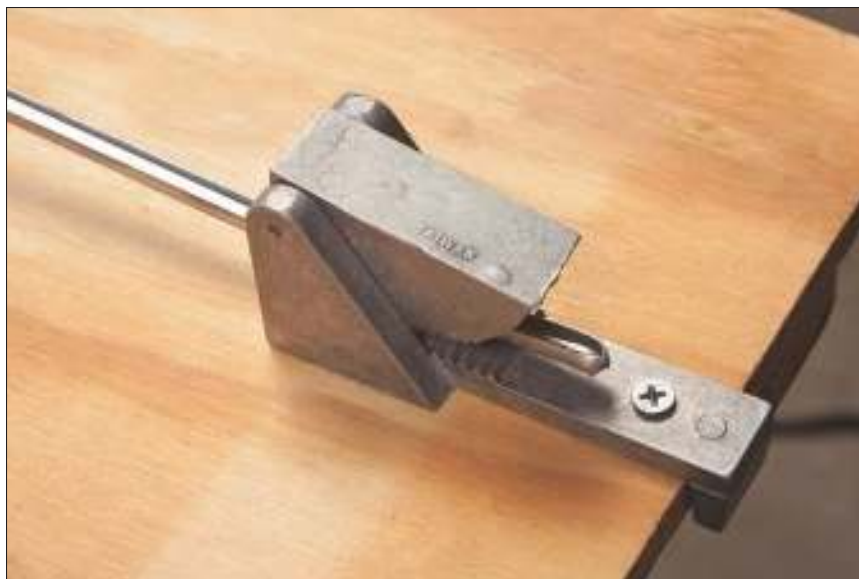
Figure 9-2: Inserting lead came into the lead vise.
