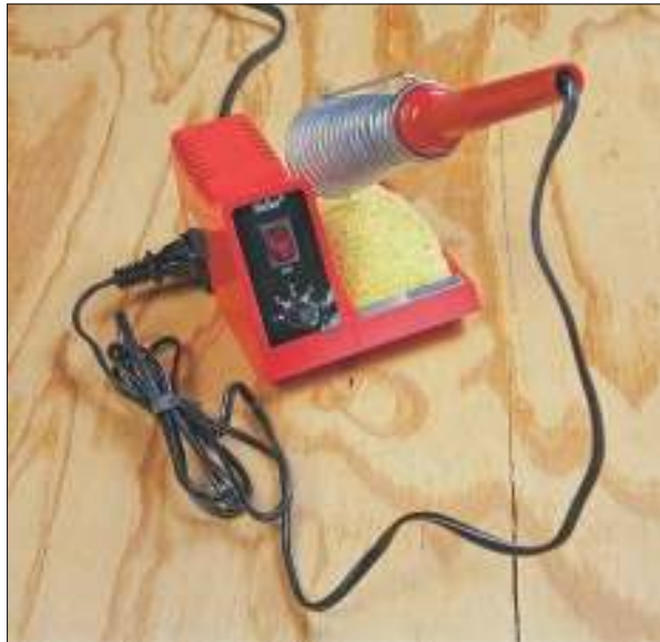
Figure 7-1: Setting up a rheostat- controlled iron for a copper-foil project.
