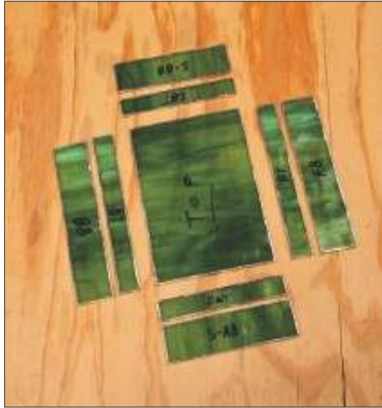
Figure 10-15: Foiled and tinned box pieces.
