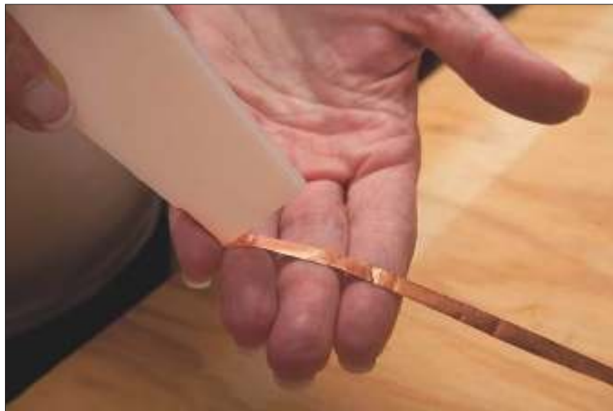
Figure 11-5: Glass piece centered on the strip of copper foil.
