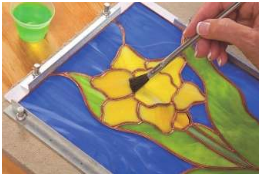
Figure 7-4: Applying flux to a copper-foil project.
