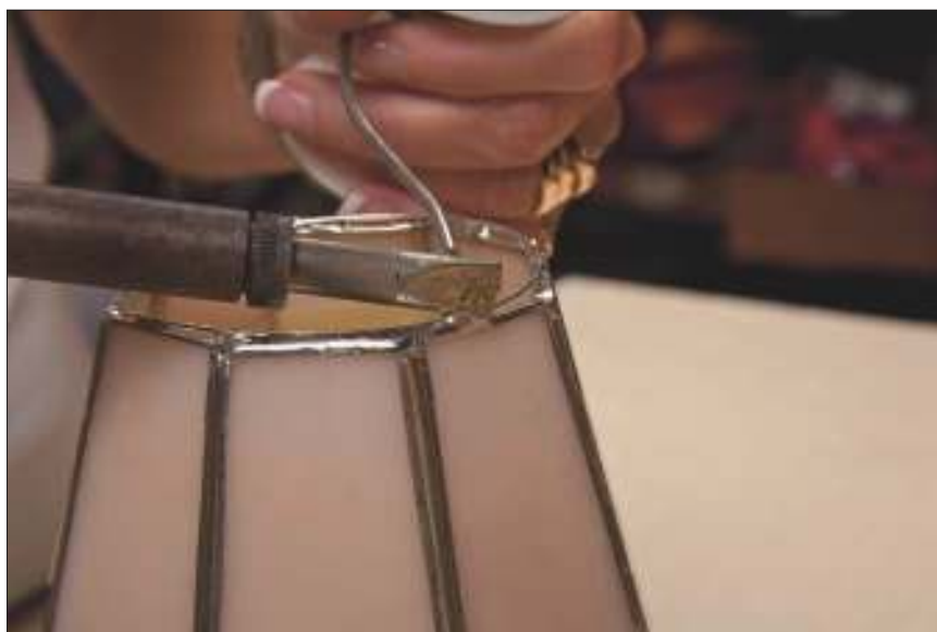
Figure 11-9: Covering the support wire with solder.
