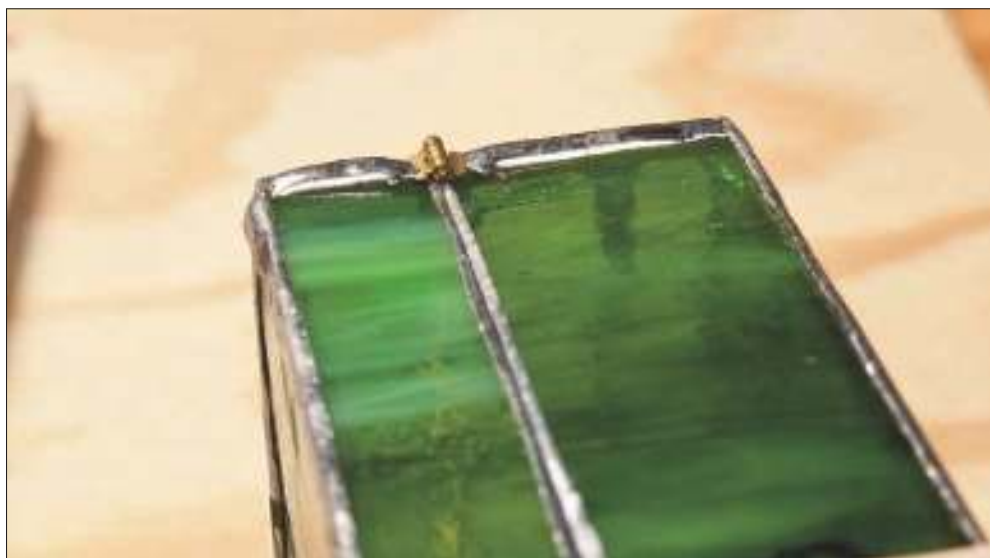
Figure 10-20: Soldering the back and front side seams after attaching the hinges.
