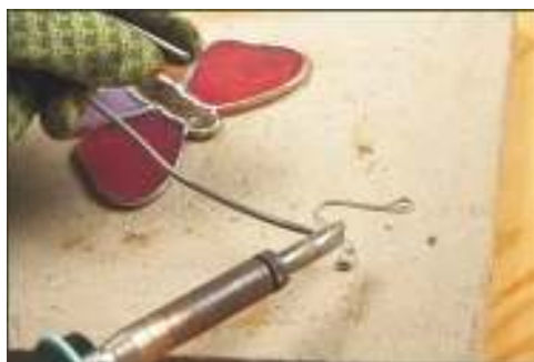
Figure 8-22: Shaping the antennas.
