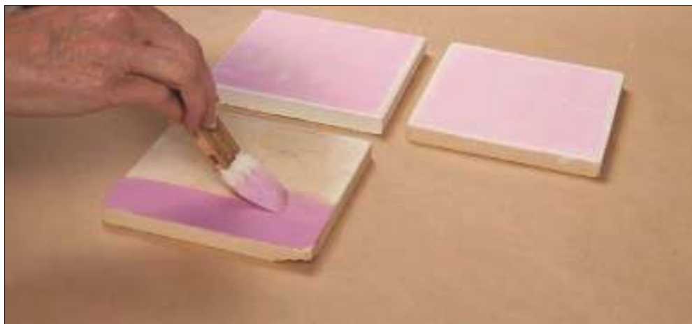
Figure 13-9: Applying the first coat of kiln wash to a shelf.
