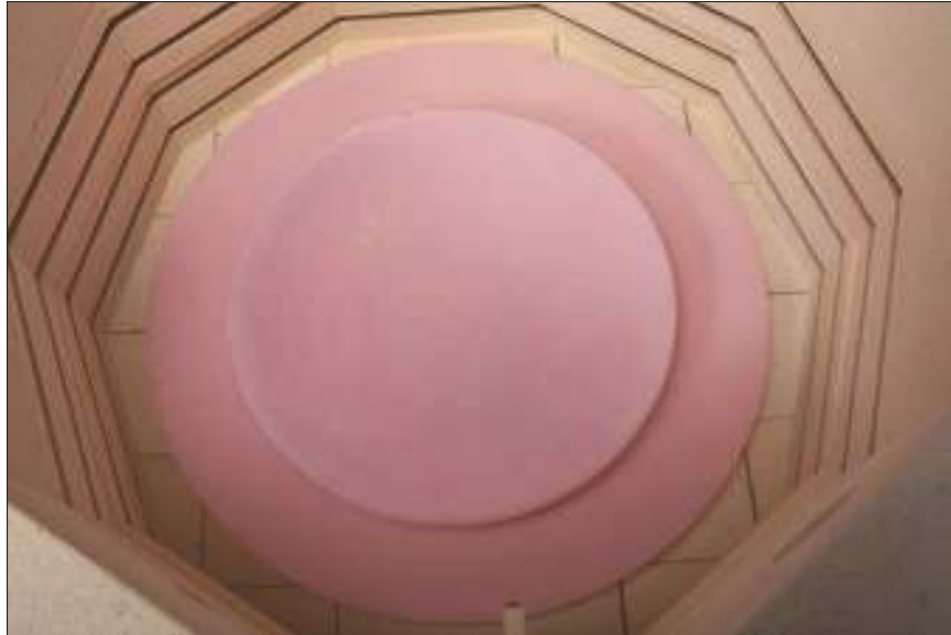
Figure 16-8: Positioning the mold on the kiln shelf.
