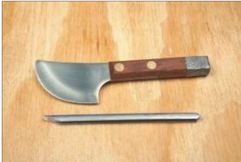
Figure 2-18: A lead knife and a cut came.
