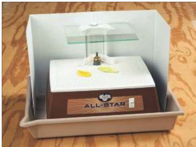
Figure 3-2: Effective homemade grinder station.
