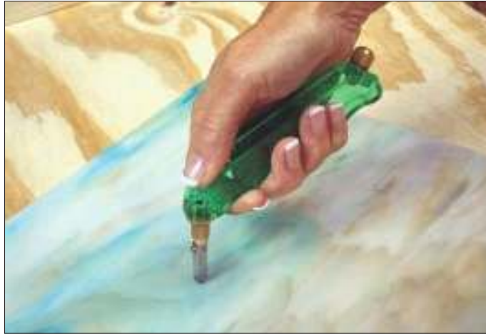
Figure 2-3: A pistol-grip cutter and the proper way to position it in your hand.
