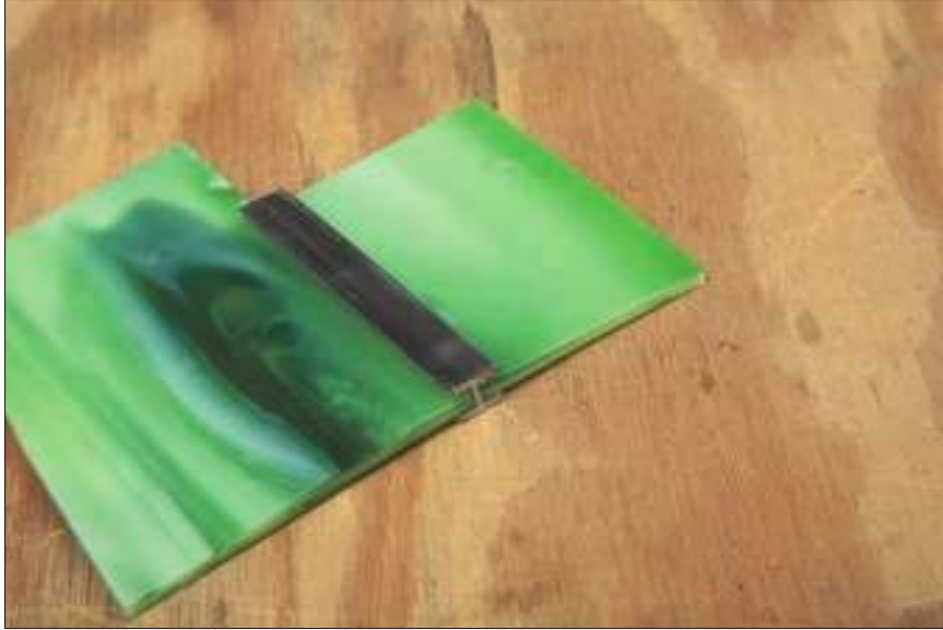
Figure 1-2: Lead came shaped into an H profile links the interior pieces of a panel together.
