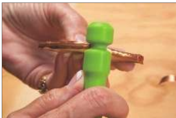
Figure 8-8: Crimping the foil over the glass's edges.
