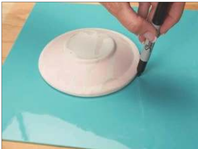
Figure 16-6: Tracing the shape of a ceramic mold onto the glass surface so you know where to cut your glass.
