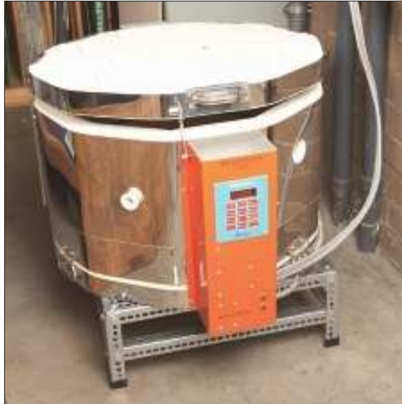
Figure 16-1: A large, top-loading kiln with a digital controller.
