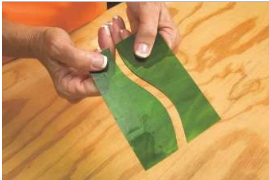
Figure 5-17: Use your hands to finish the run and break the glass.
