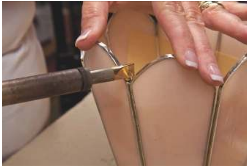
Figure 11-10: Tack soldering the bottom panel intersections together.
