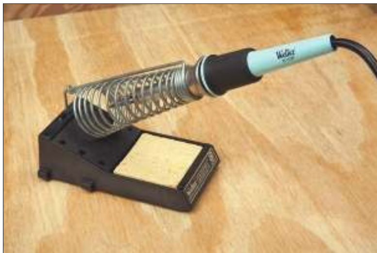
Figure 2-12: Sturdy iron stand with weighted bottom.
