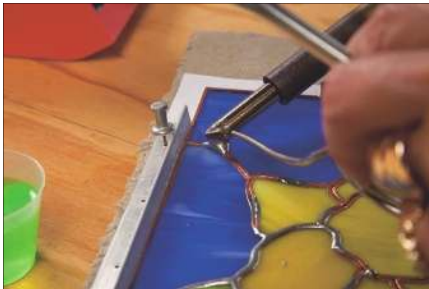
Figure 7-8: Molten solder ball under the soldering tip.
