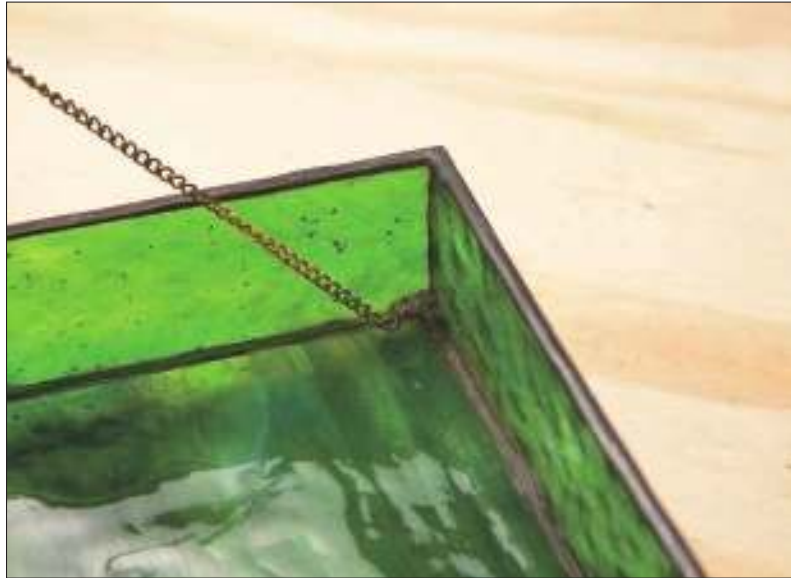
Figure 10-21: Box with chain soldered in place.
