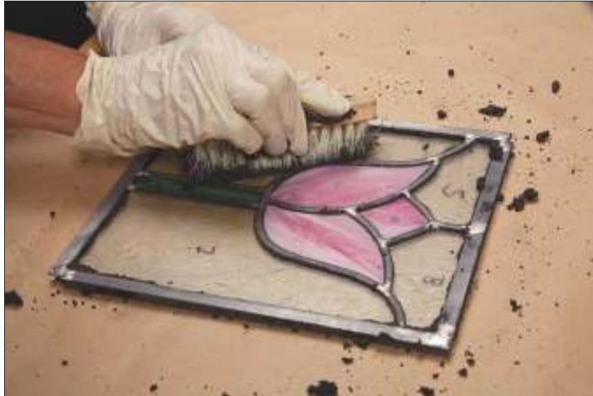
Figure 9-15: Using the brush to remove excess cement from the panel.
