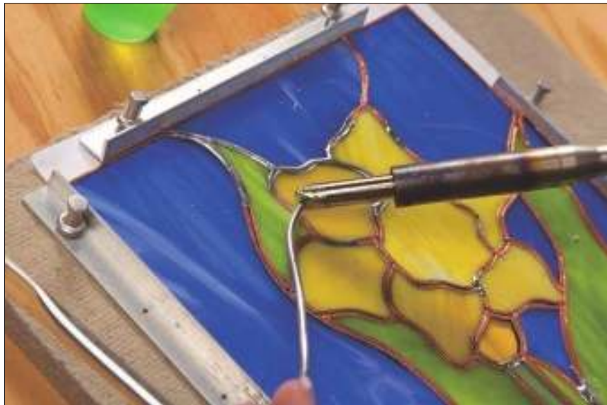
Figure 7-7: Positioning the iron and solder to run a bead.
