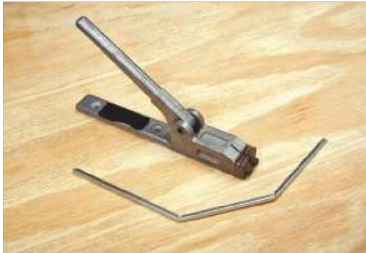
Figure 2-23: A notcher with examples of came cuts.
