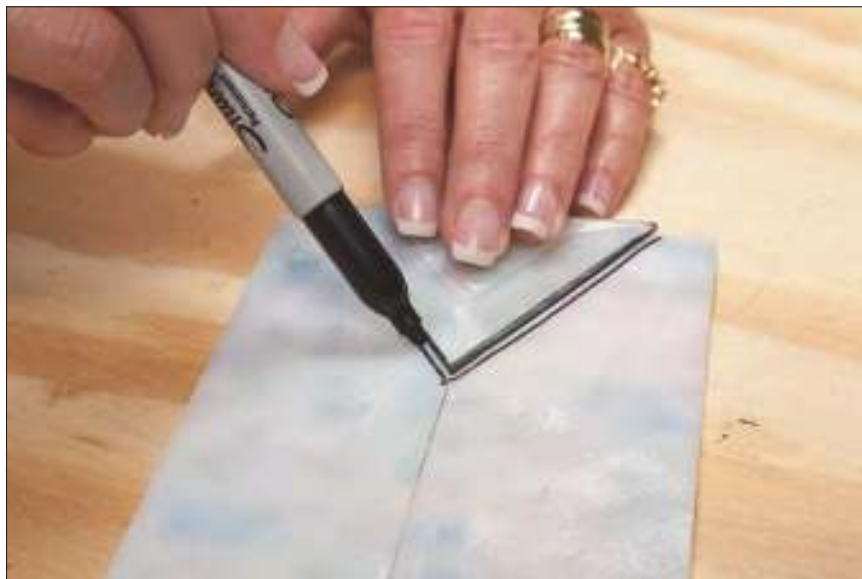
Figure 10-23: Tracing the shape of the bevel onto the box's top pieces.
