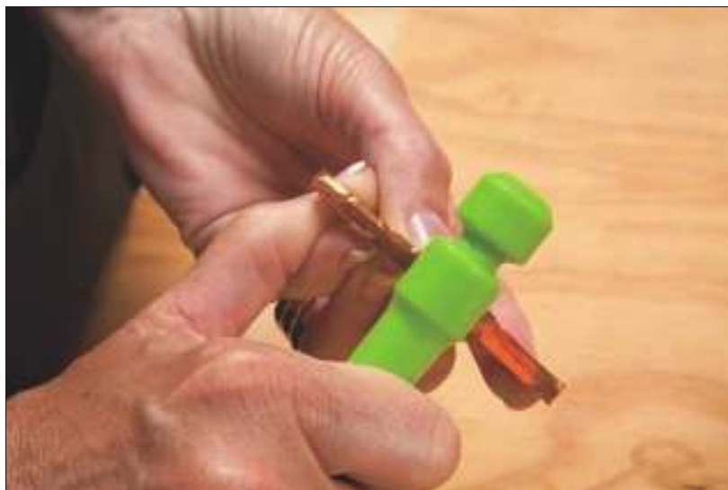
Figure 8-7: Burnishing the foil to the glass's edge.
