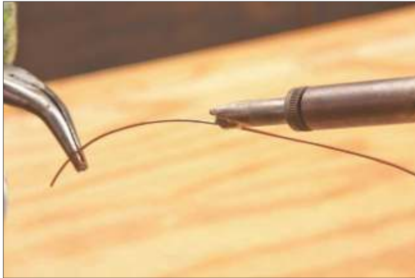
Figure 8-19: Tinning wire with 60/40 solder.
