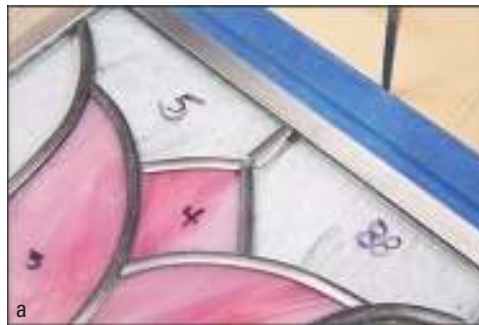
Figure 9-12: A joint with too big of a gap and a perfectly sized joint.
