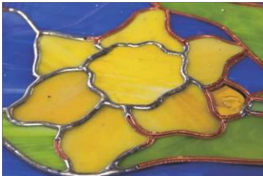
Figure 7-11: Soldered intersec- tions with multiple seams.
