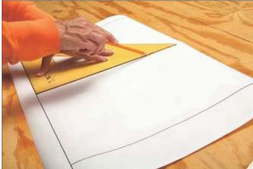
Figure 4-6: Establishing the middle design line.
