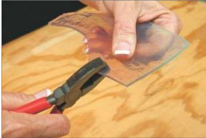
Figure 6-2: Grozing a piece of glass.
