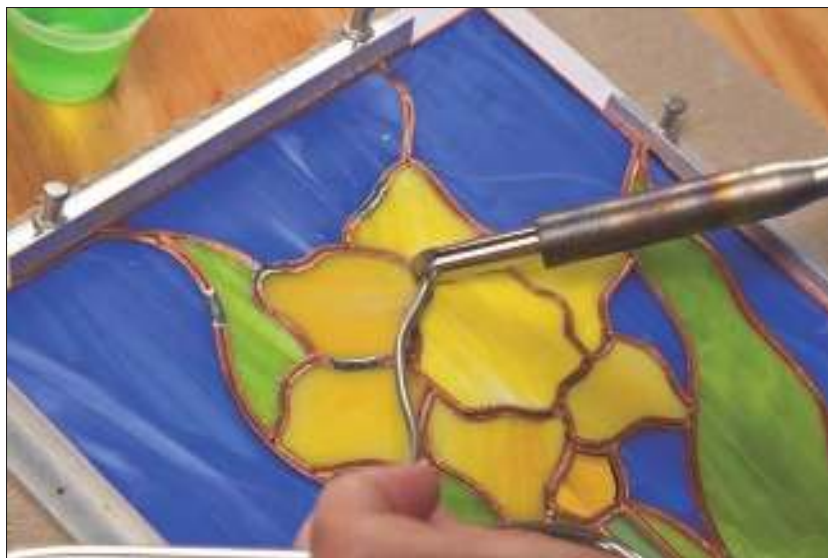
Figure 7-5: Tack soldering a copper-foil project.
