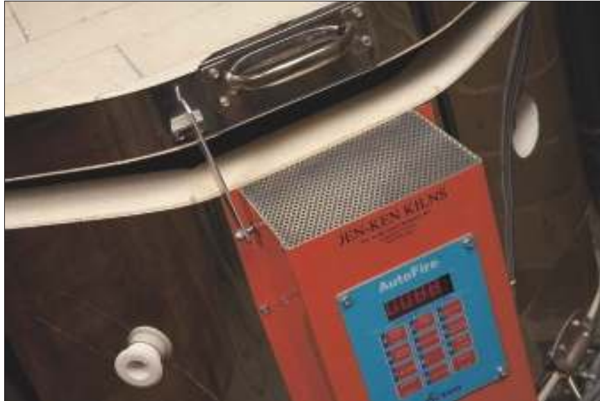
Figure 14-1: Venting the kiln during the initial heat-up.
