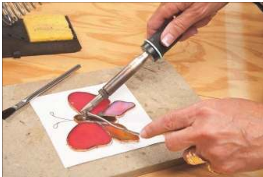
Figure 8-12: Correct way to hold your soldering iron.
