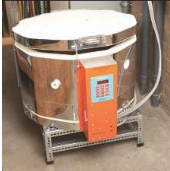
Figure 13-10: Test firing a new glass kiln.
