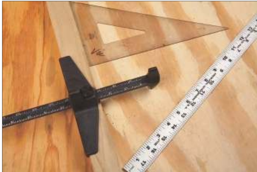
Figure 10-6: Strip cutter, ruler, triangle, and work board rail.
