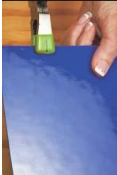
Figure 5-11: Positioning running pliers for breaking the score.
