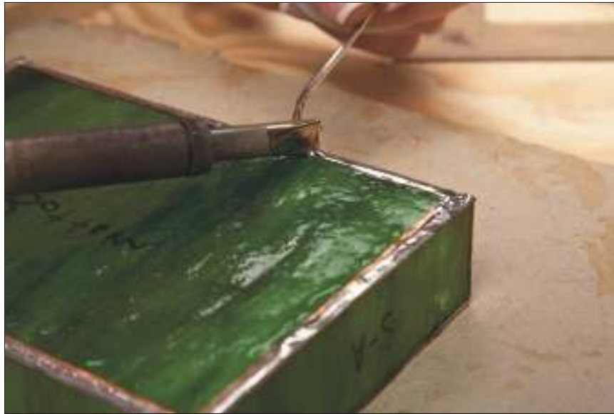
Figure 10-17: Running a flat bead around the bottom of the box.
