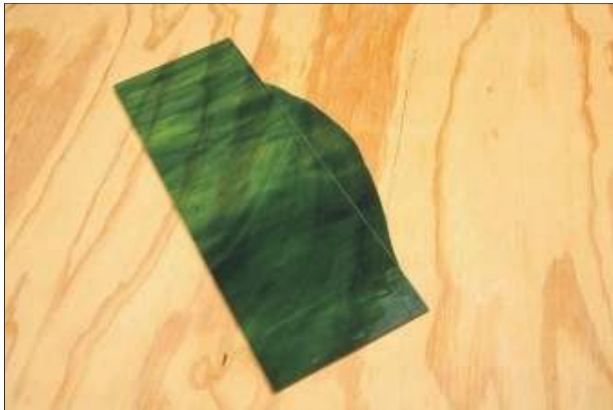
Figure 5-15: A bad break and run.
