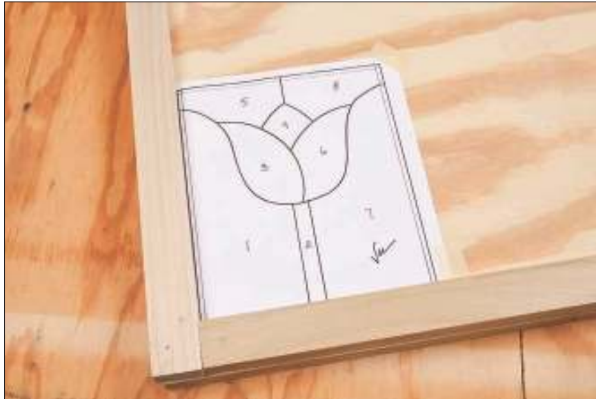
Figure 9-6: Laying out your trimmed pattern on the work board.
