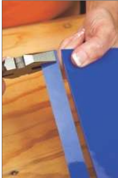
Figure 5-10: Breaking the glass with break- ing pliers.
