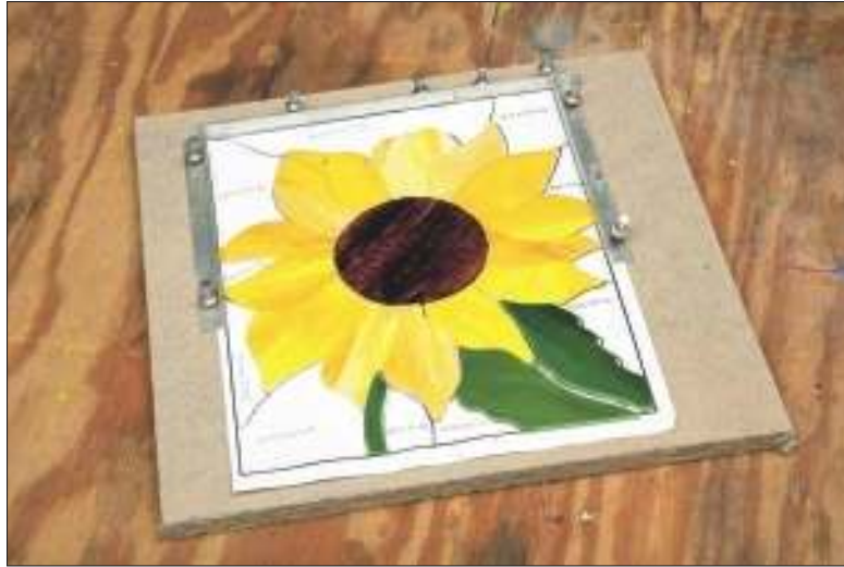
Figure 2-22: Homasote work board with project being constructed using layout blocks and push pins.
