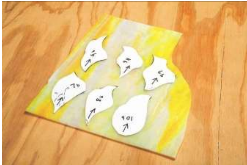
Figure 5-18: Laying out your pattern templates.
