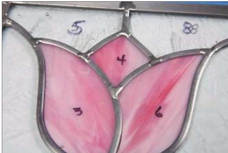
Figure 9-13: Examples of perfectly sized solder joints.
