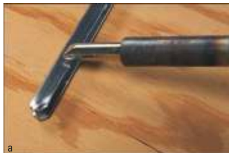
Figure 7-13: Use some scrap lead came to see if your iron is too hot.
