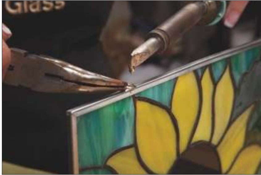
Figure 8-27: Attaching wire rings to the frame.
