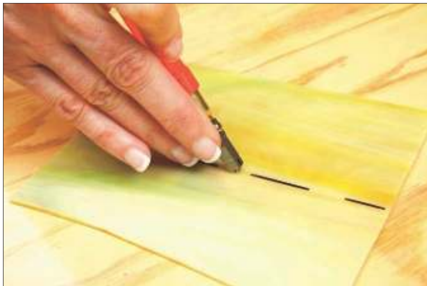
Figure 5-5: Applying even, steady pressure to make the score line.
