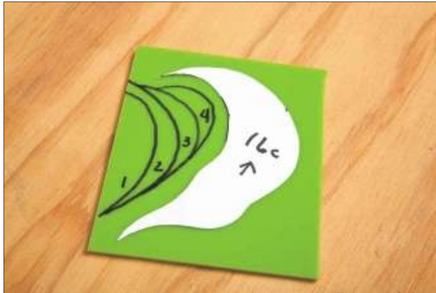
Figure 5-19: Making relief cuts when cutting curves.
