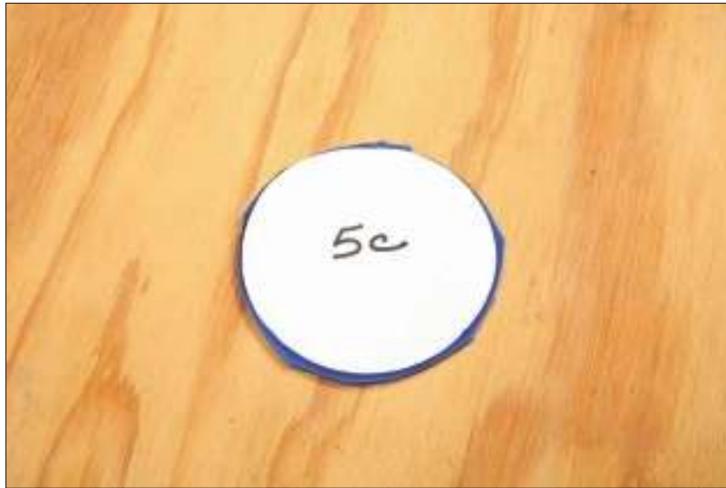
Figure 6-1: A circle-shaped glass piece after you cut it but before you file it.
