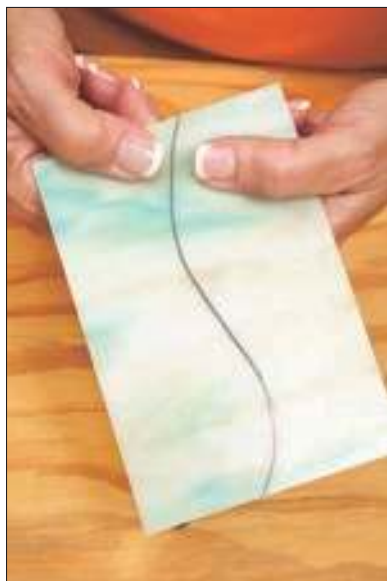
Figure 5-14: Breaking glass along a curved score line.
