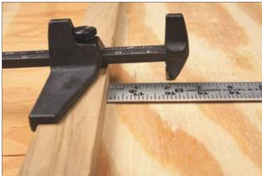
Figure 10-10: Setting the cutting wheel at 2 inches.
