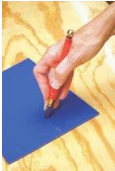
Figure 5-1: Holding a barrel cutter with extended fingers.
