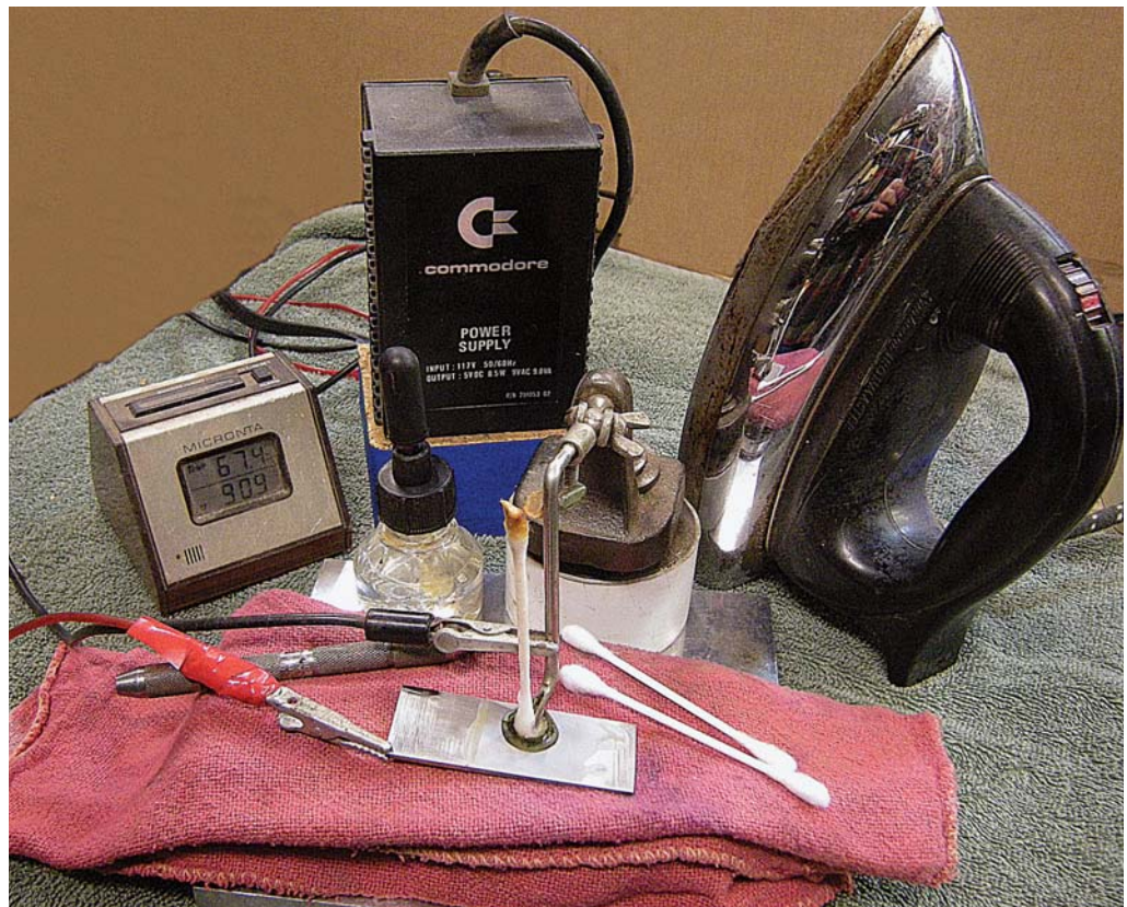
The complete etching outfit. Salt water and good quality direct current will etch every metal I've tried.
