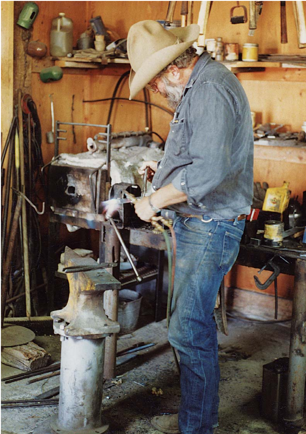
“Master of The Torch” Ed Fowler heating the edge of a blade. I’ll bet it’s made of ball bearing steel and will be edge quenched.
