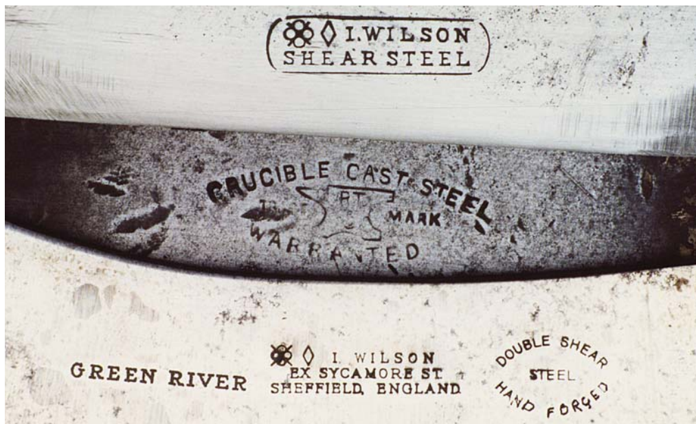
Shear steel, double shear steel and cast steel markings on knives from the 1800s.
