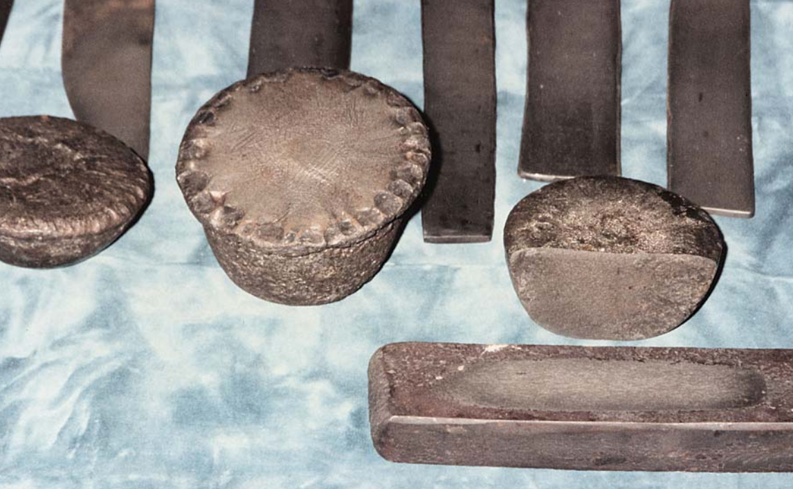
Wootz cakes and billets made by Al Pendray. The cake at the right has been cut in half to show the crystalline structure.
