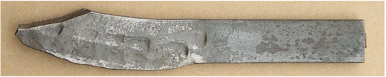
A four minute demo blade that started as a hot cut preform.
