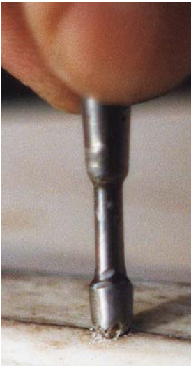
This is the hand-turned countersinking tool.
