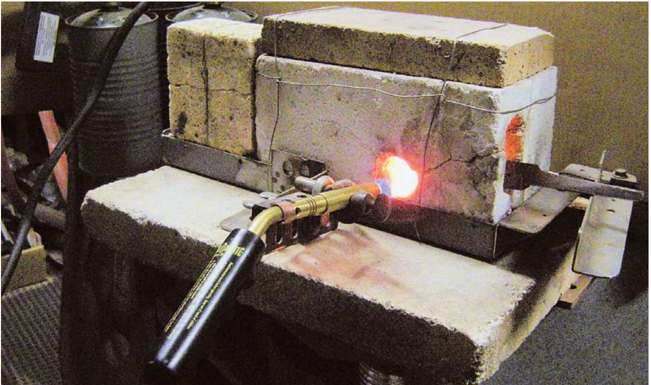
The one-brick forge, extendo model.
