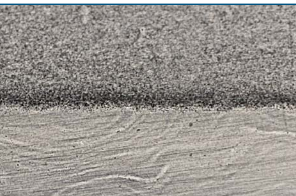
Close up of the “damascus” pattern that shows up in old shear steel when etched. This blade was made from a large old circular saw.
