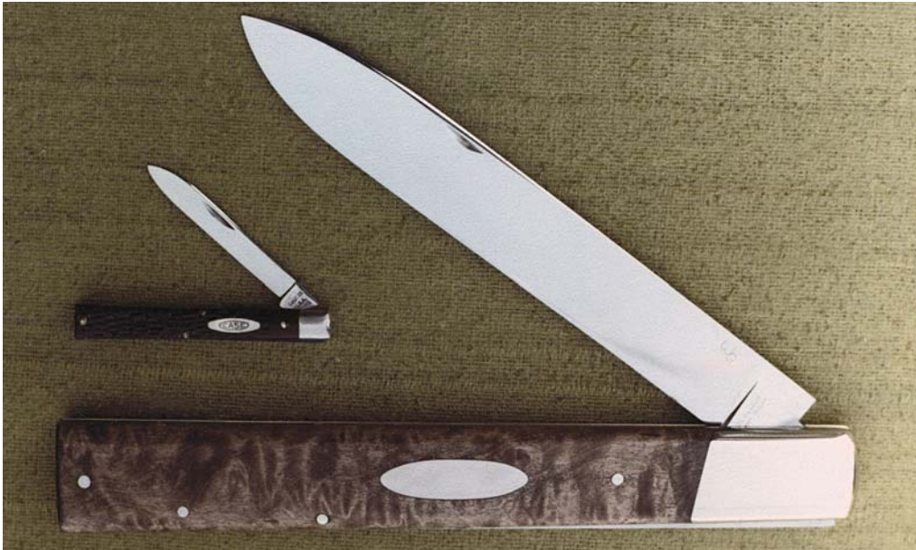
Doctor's Knife, 12 inch handle, brass fittings, maple handle slabs. This style folder goes back at least to Civil War days. The flat end of the handle was used to crush tablets, and some doctor's knives have spatulas as a second blade. It was used for mixing ointments.
