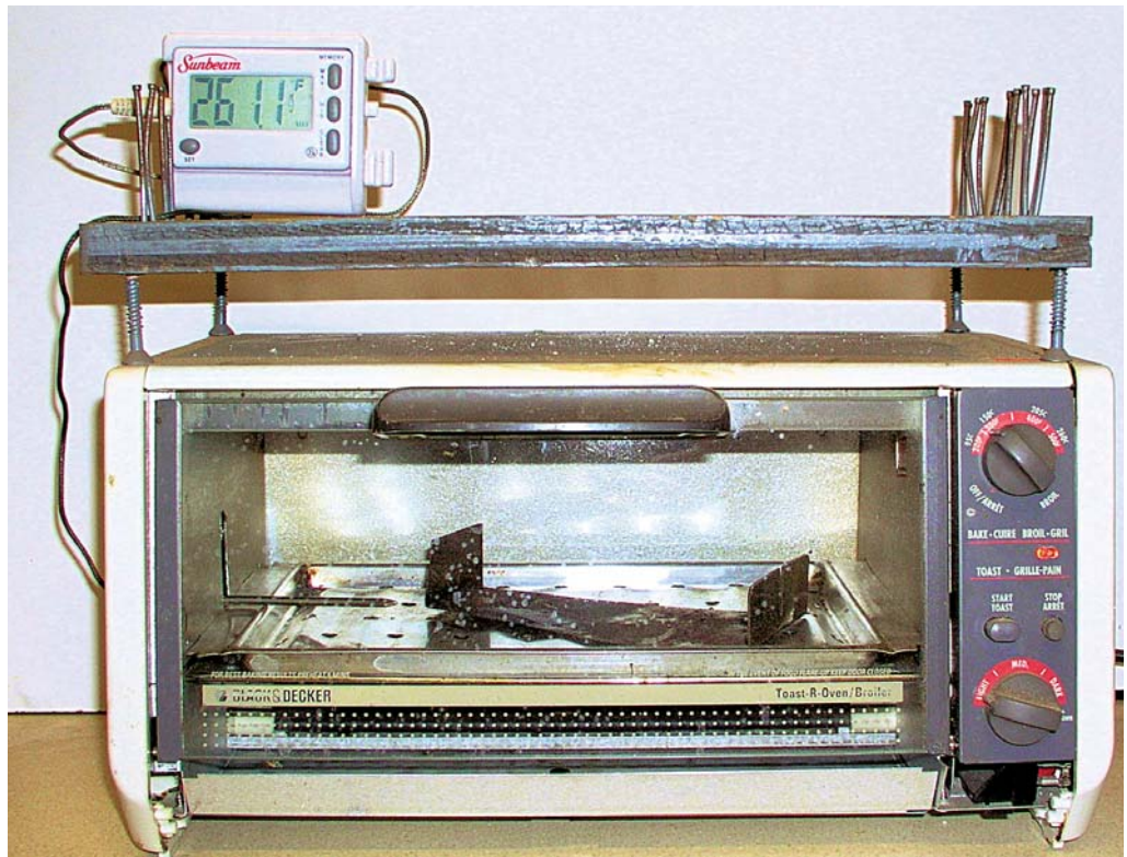
The knife shop toaster oven. Note the plywood shelf on top, the finish nails hold blades back-side down for air cooling between tempers.
