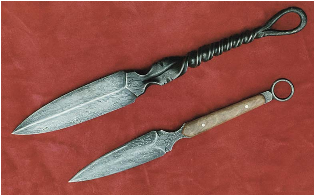
Early wire damascus work, from my “all steel” phase. The one with the fossil ivory handle sneaked in.
