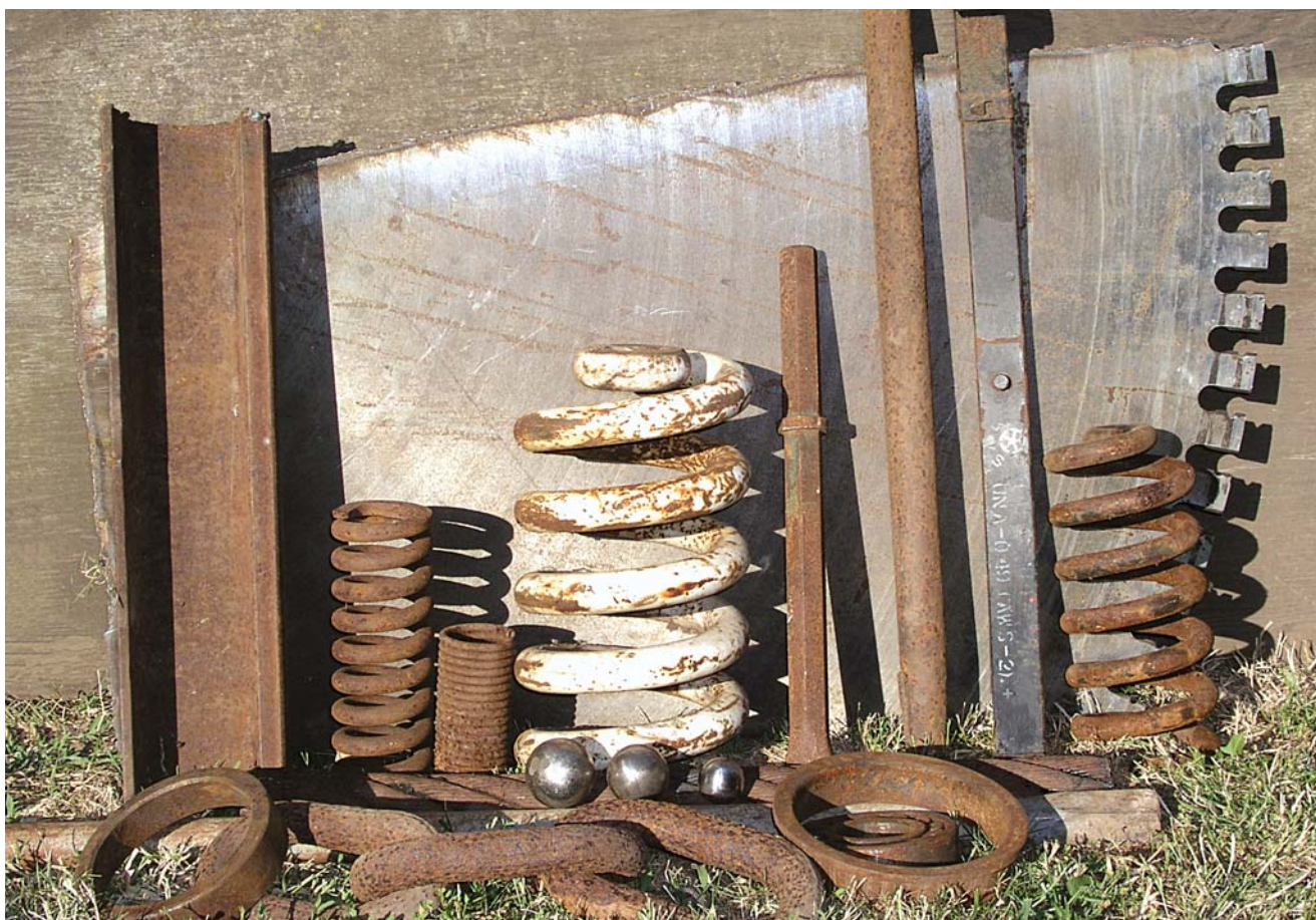
A nice assortment of junkyard materials, everything from old wrought iron to nearly new 50-pound coil springs made of 5160.
