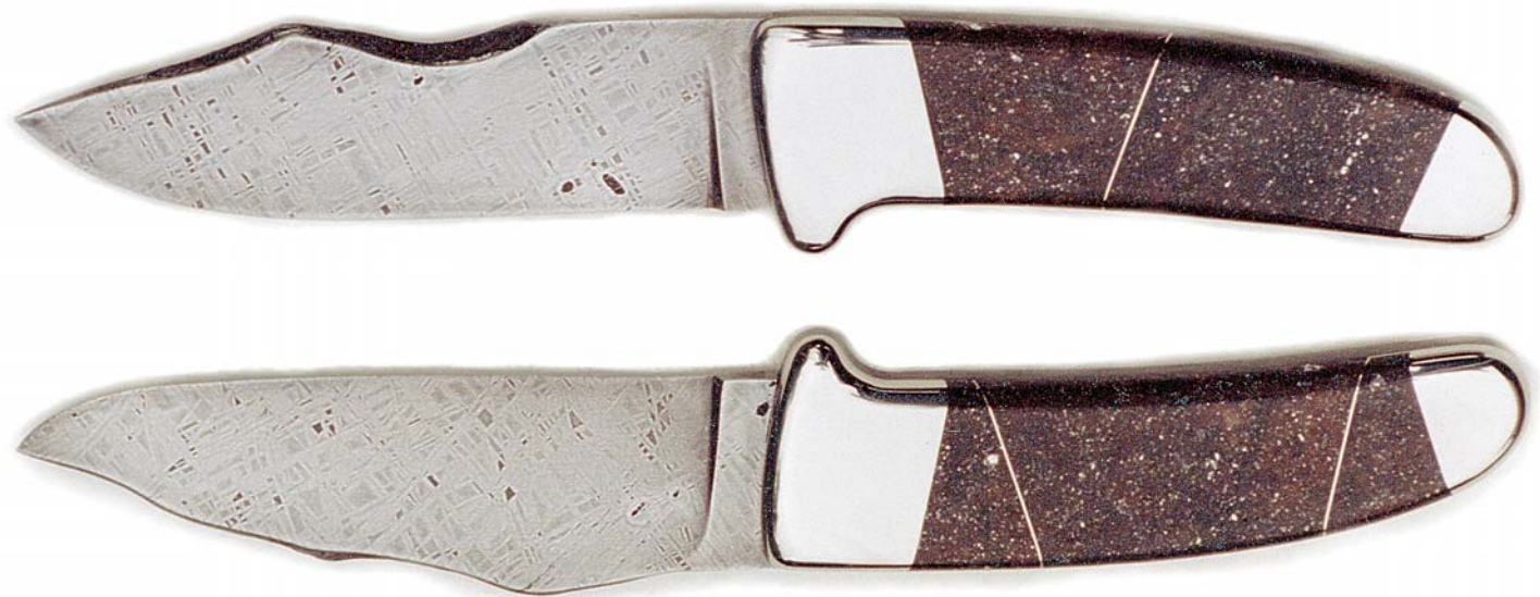
One knife is completed, the other ready for the stony meteorite slabs. Note the silver brazed tang extension.
