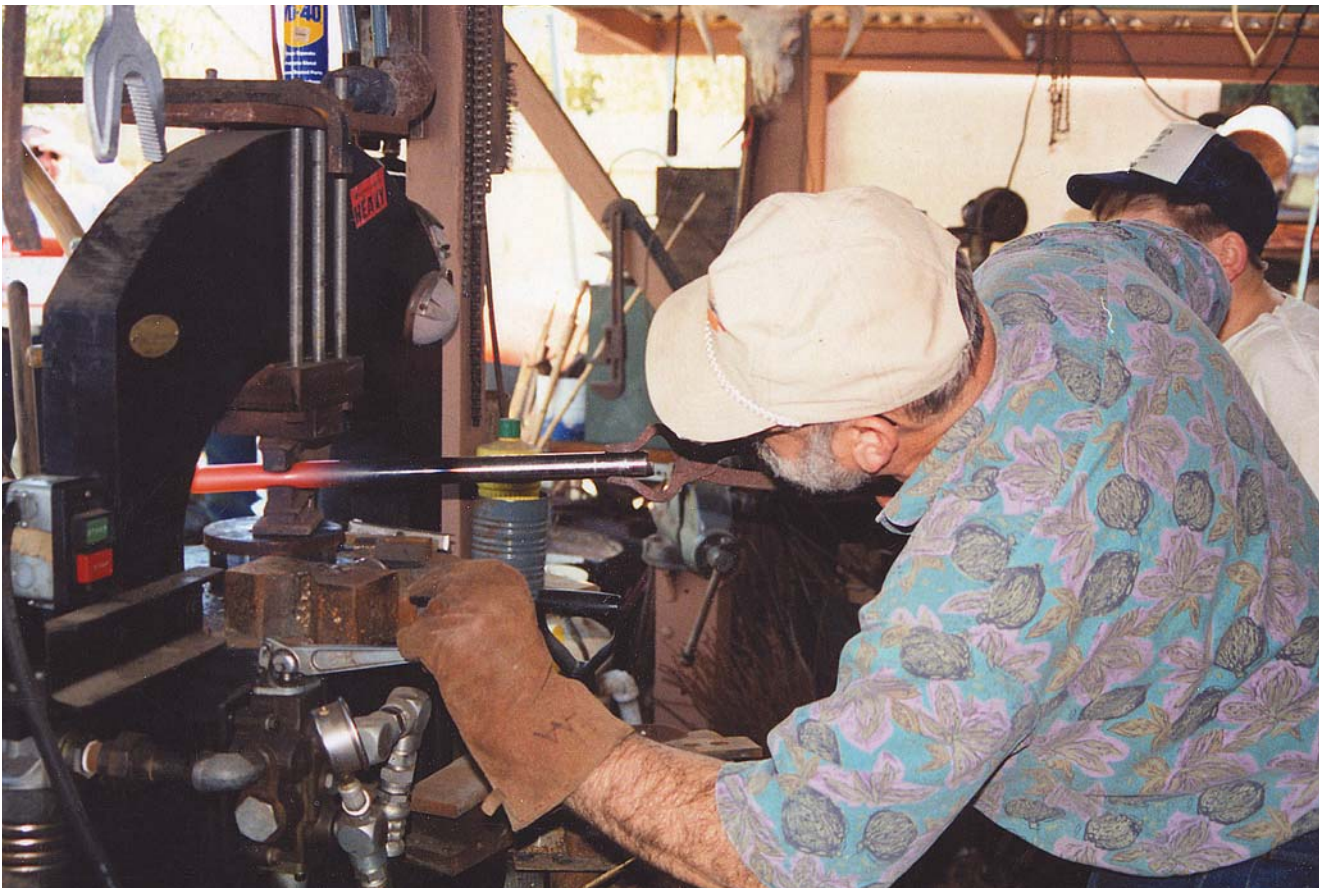
Putting the big squeeze on a one-inch diameter bar of 52100.
