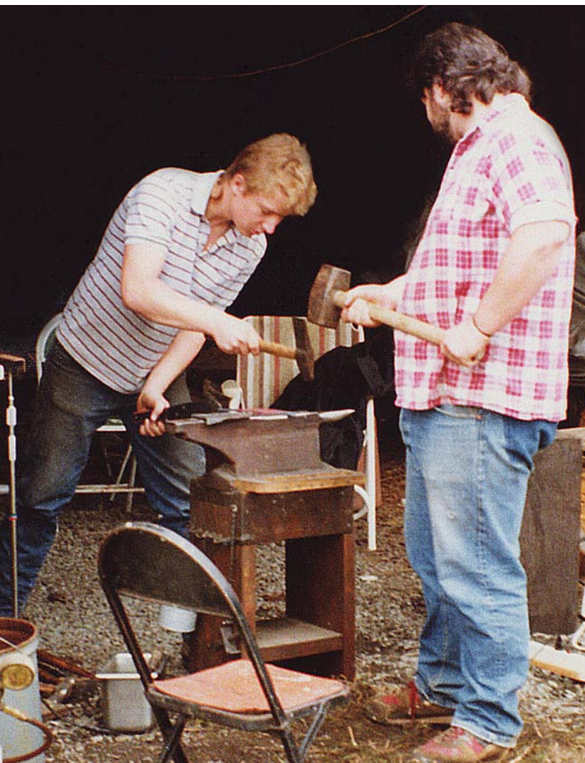
That's the first anvil I made being used at a hammer-in at Wendell Fox's smithy. Larry Milligan is holding and Shawn Vallotton is being the striker. The base that it is on is too light for doing serious forging but is nice when it comes time to haul it around the country.
