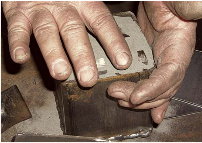
The elements that will make the mosaic are packed in the can and it is filled with the proper powder.
