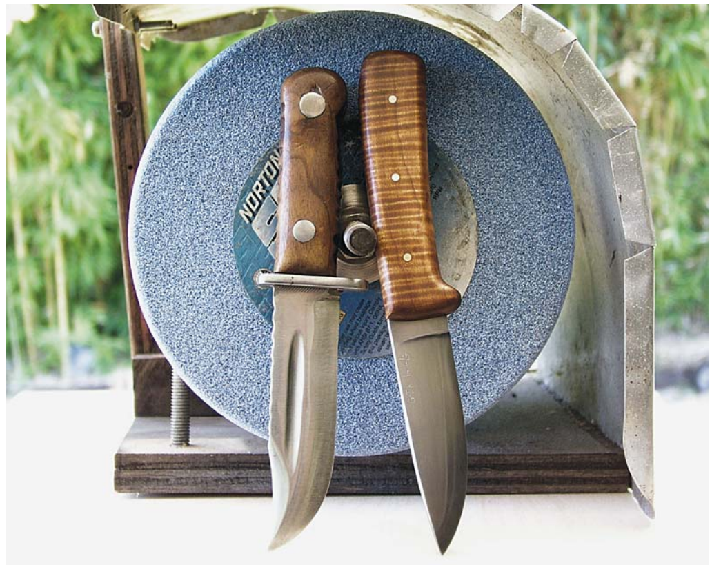
The knife on the left is the first knife I made from scratch. I used an oven-tempered lathe rasp for the blade, steel for the guard and myrtlewood for the handle. The knife at the right with the maple burl handle is the project knife I made in 2005 for a chapter I wrote for BLADE's Guide to Making Knives .
