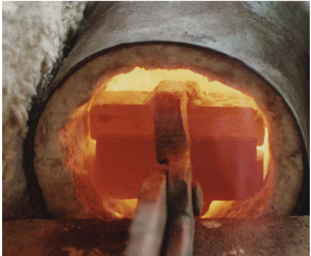
The heat tongs are getting hot in the small heat treating forge. The heating surfaces are one-inch square and four inches long, that amount of orange hot steel is necessary to get a soft back draw on a large knife.
