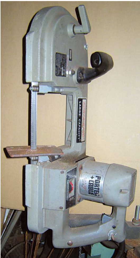
This is the Porter Cable Porta Band. It has a variable speed motor and is quite the space-saving tool.
