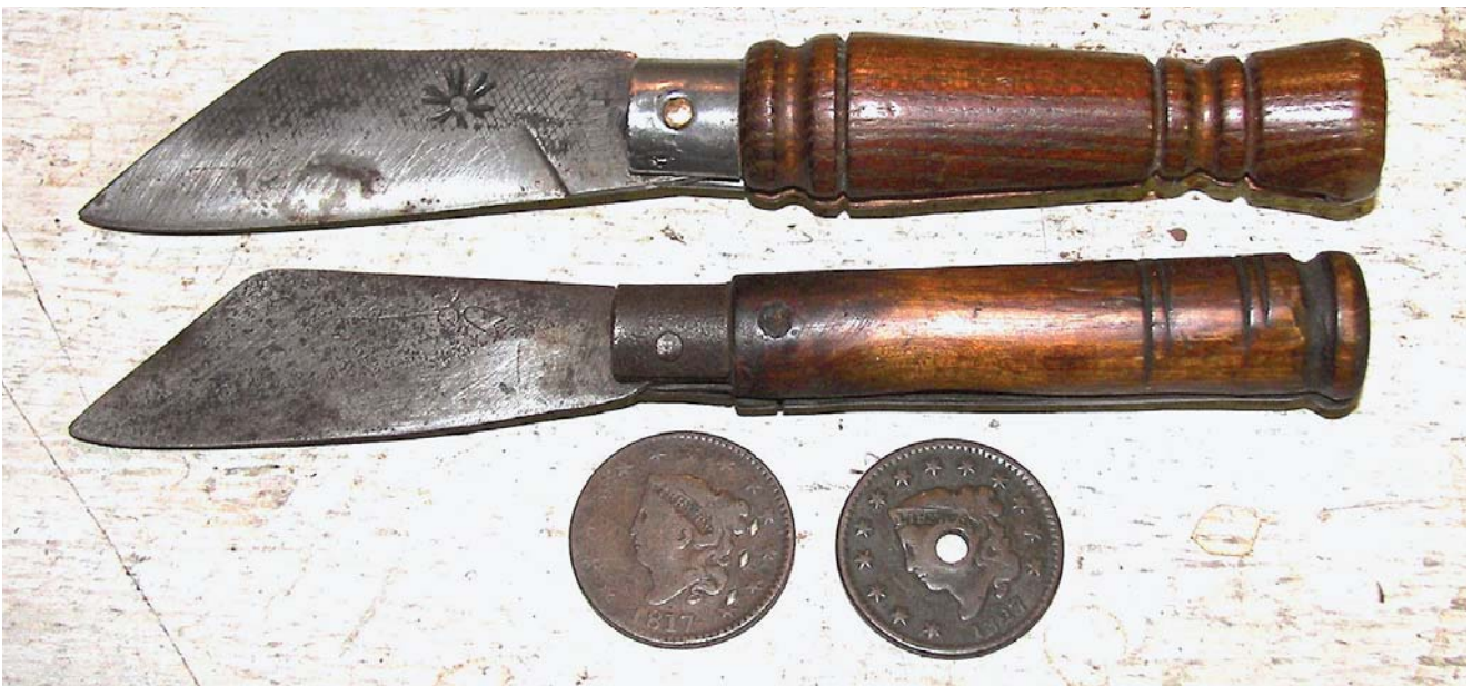
My thanks to Gene Chapman for this photo. He wrote, "The top knife I made years ago, hand forged blade from a bastard file, turned Osage Orange handle, tin coated steel bolster and a bronze blade pin. Bottom knife a recent internet auction buy, appears old and typical of other penny knives images seen on the internet. I added two old large cents, 1817 and 1827 dates."
