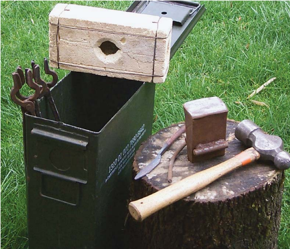
This shows Dave Rider's stump-anvil, one-brick forge, hammer and tongs, with all of it fitting into the ammo can. Note the coil spring material on the stump and one rough forged blade.
