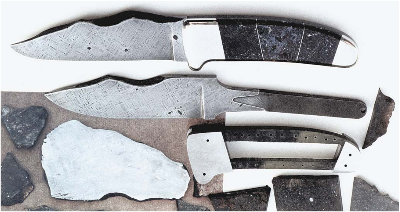
One knife is completed, the other ready for the stony meteorite slabs. Note the silver brazed tang extension.
