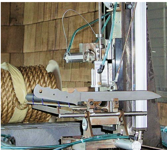
The rope cutting endurance test.
