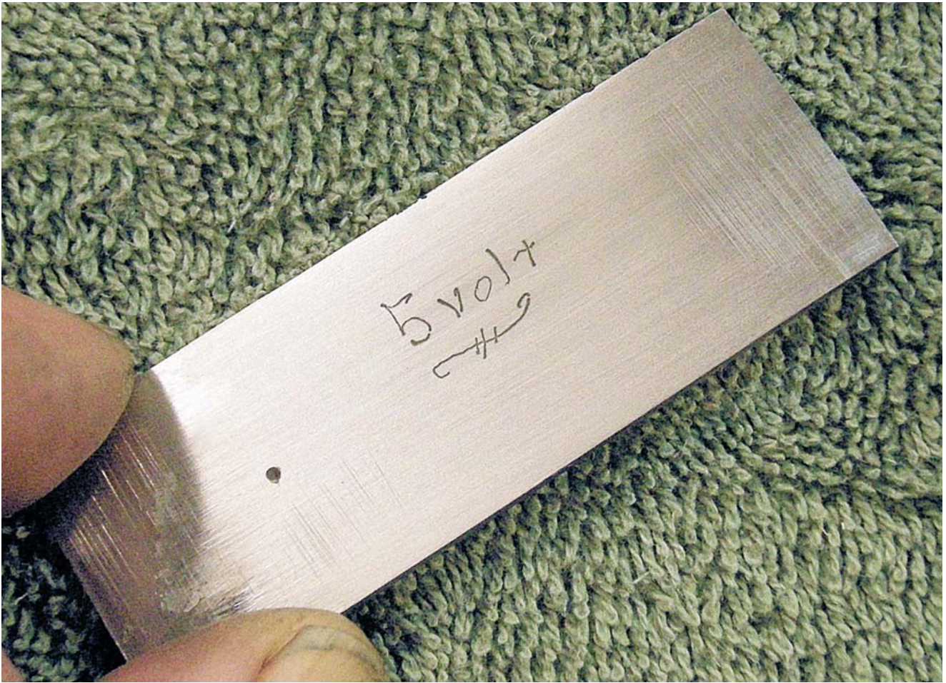
A successful etch test.
