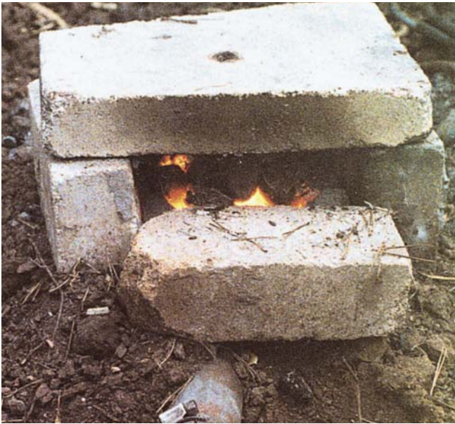
I call it the "Dirt Cheap" forge.
