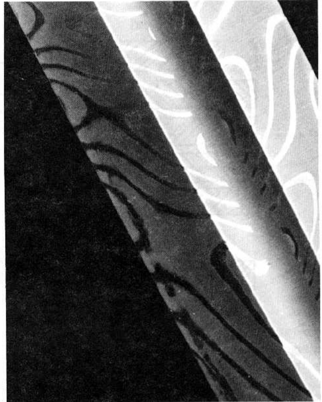
Fig. 132. Double star or chevron twist blade made by the author. Materials used: 1095 and pure nickle sheet.
