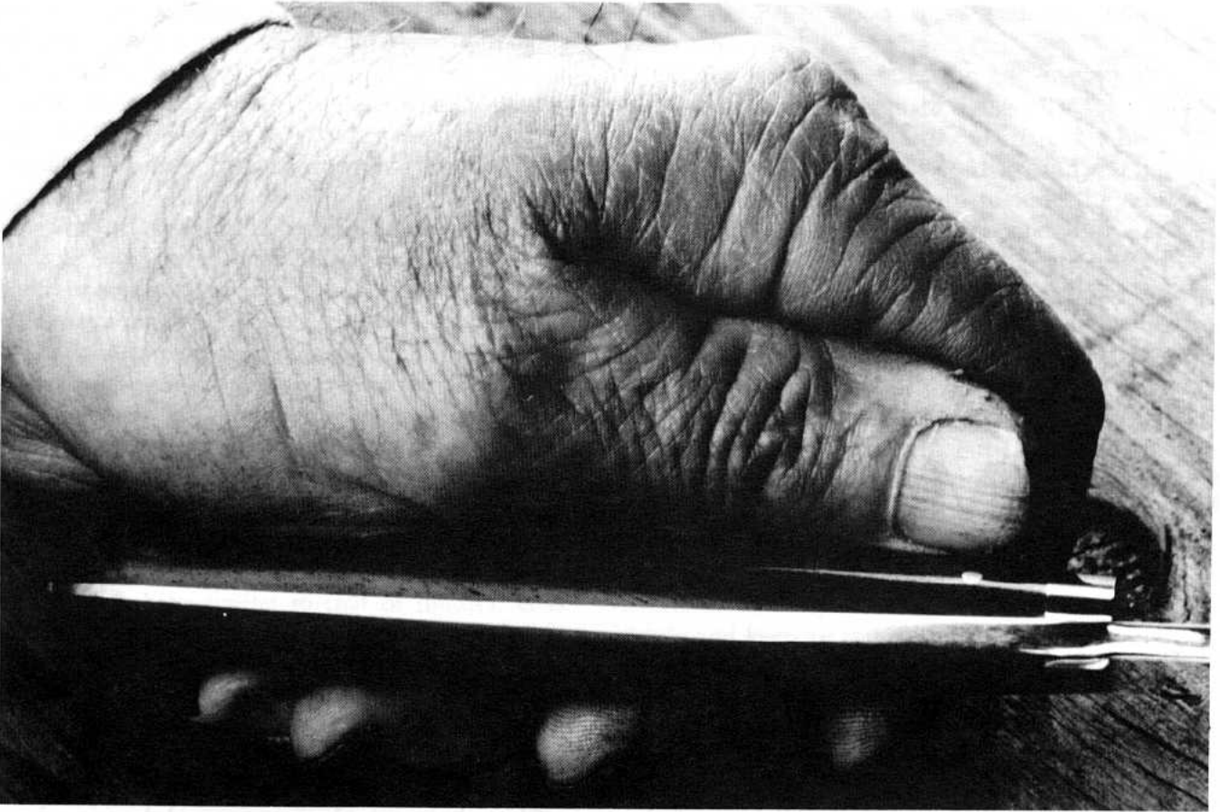
Fig. 61. A full-tang knife with the tang tapered to aid in balance
