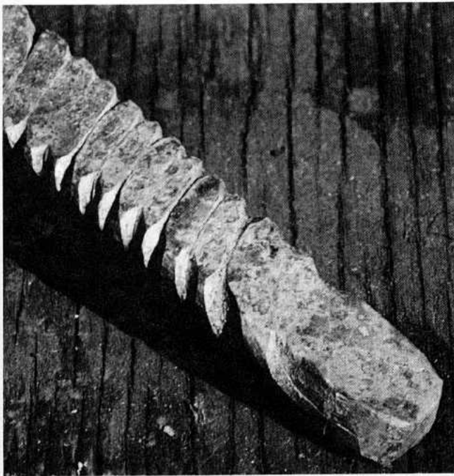
Fig. 126. The bar has been twisted and flattened and is ready to be ground true prior to further forging.
