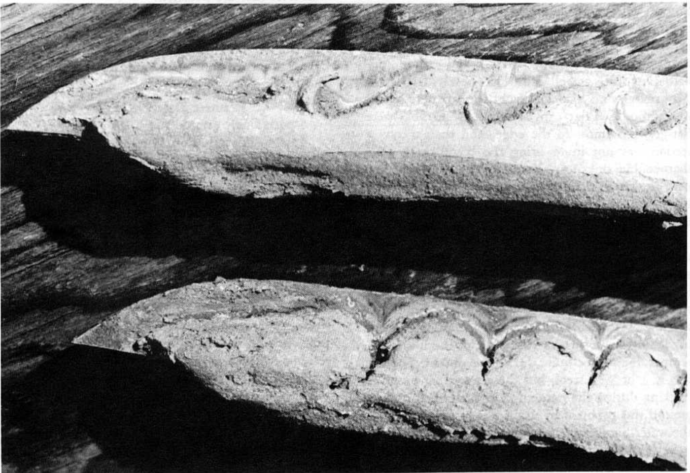
Fig. 156. Close-up of blade covered in the heat-treating clay
