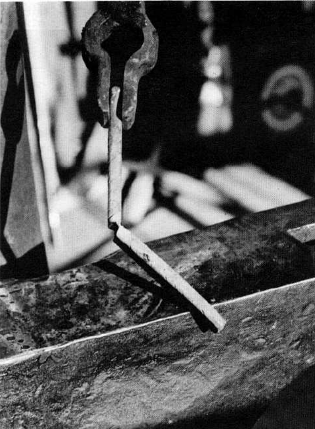
Fig. 118. The fold is started. The cut surface of the bar on the outside makes the fold tighter and easier to accomplish.
