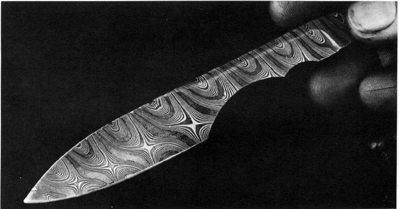
Fig. 128. A star pattern leather worker's knife made by the author. Materials used: 1095 and pure nickle sheet.
