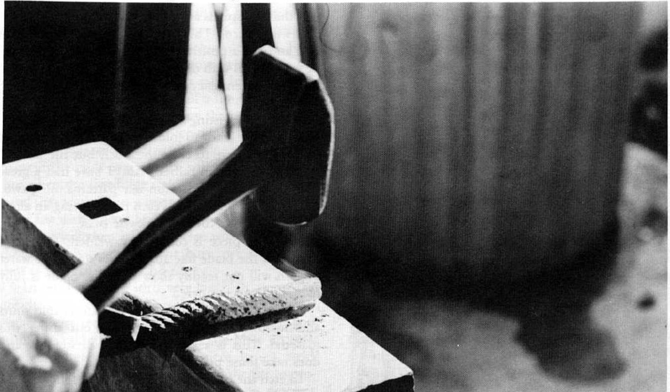
Fig. 144. Welding the cable into one piece
