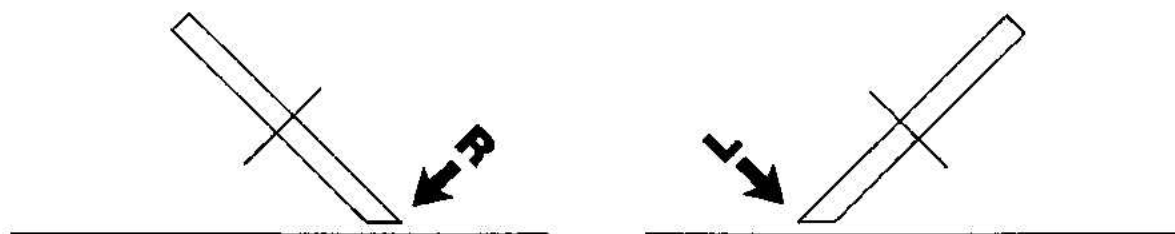
Fig. 36. . . and pack both sides by alternating edges on the anvil surface as you work the blade to the tip.
