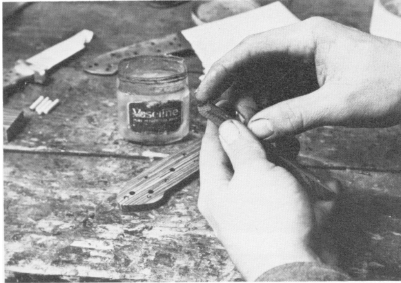
4. Putting Vaseline on' the ends of the slabs so that the epoxy won't stick there.
