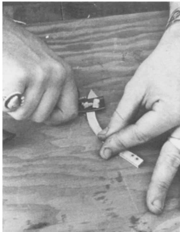
8. Shave the spacer to the proper thickness to hold the knife snugly in the case.
