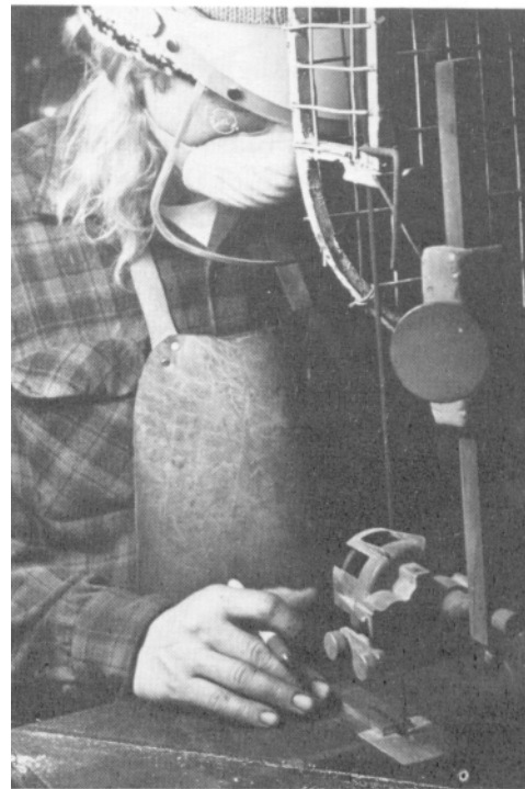
5. Cutting the slot down the center of a prospective bolster/ finger guard with a band saw.
