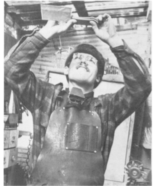
Checking for cracks between the handle and tang.
