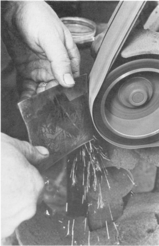
Finish the unsharpened edges of the blade. Give these areas a slightly rounded shape.
