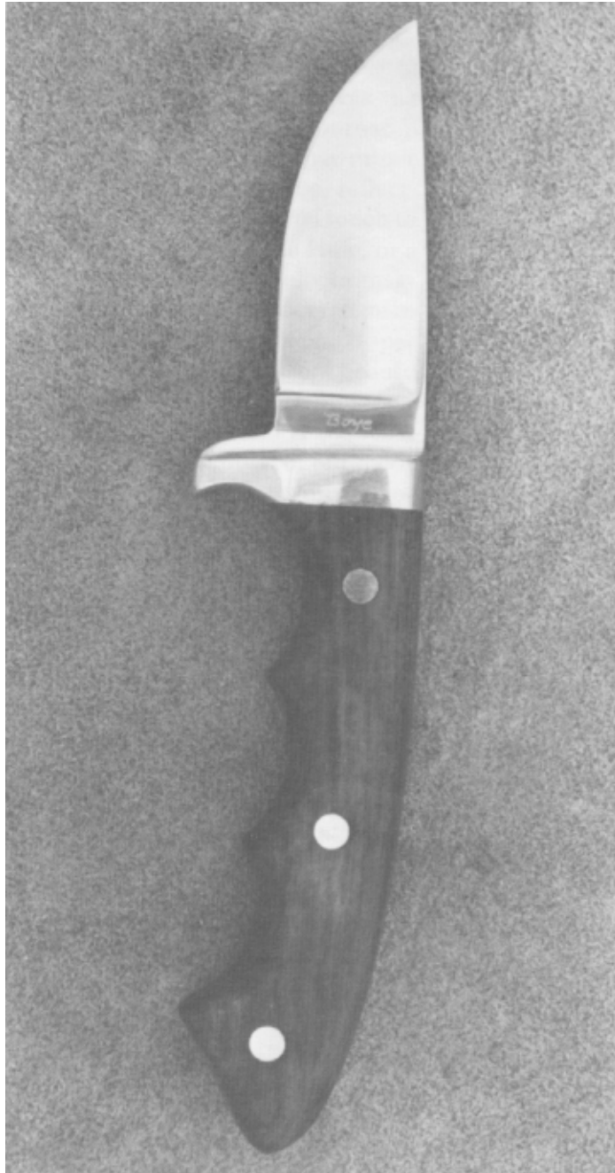
A three-fingered 2-inch utility knife with a lignum vitae handle.
