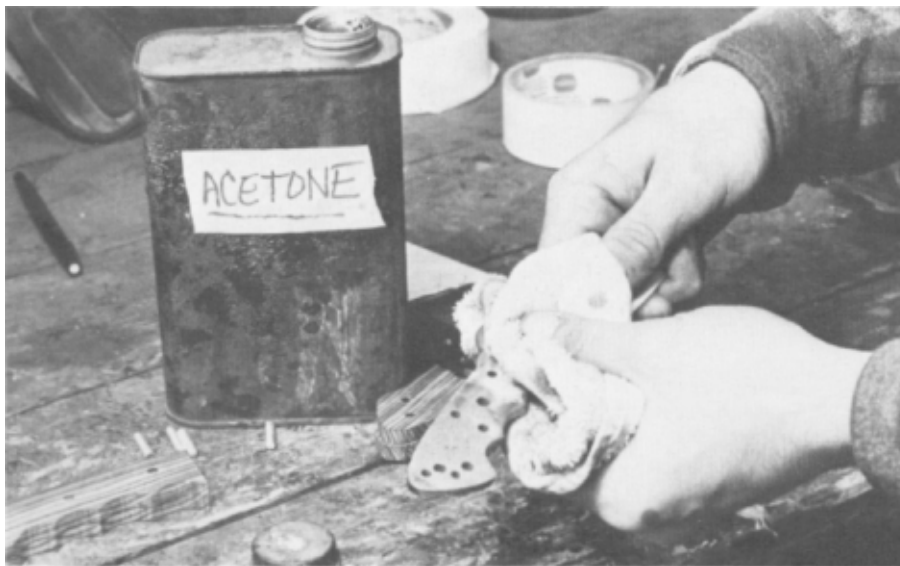
3. Cleaning off the tang with acetone.
