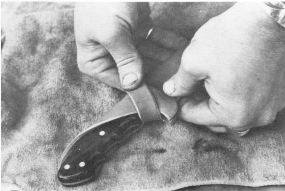
6. Complete the molding so that the snap strap fits nicely around the finger guard. It should be placed in a warm spot to dry.
