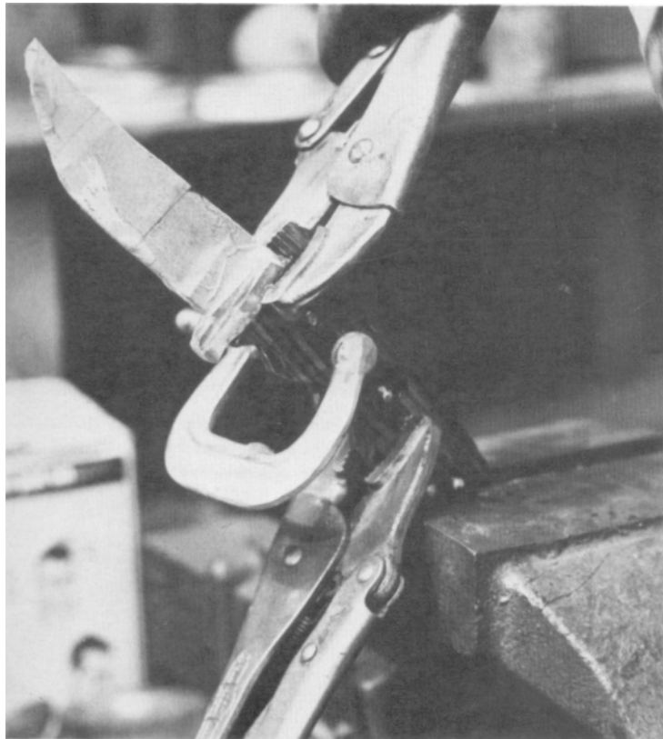
9. Undoing the snigger and squeezing the slabs tightly with the vise and clamps.
