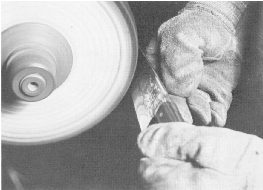
Buffing the face of the blade of a small chef's knife.
