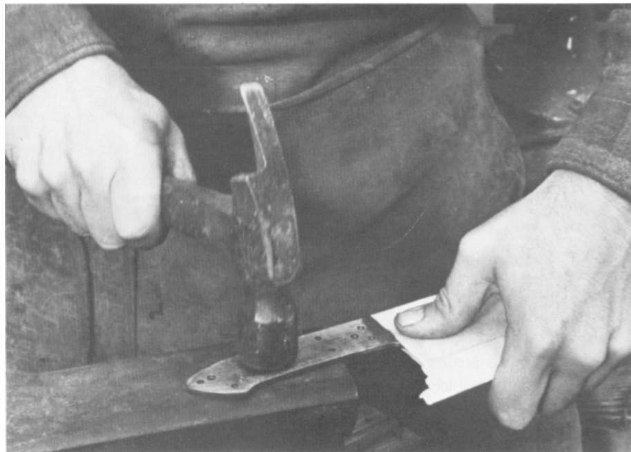
Checking for cracks between the handle and tang.
