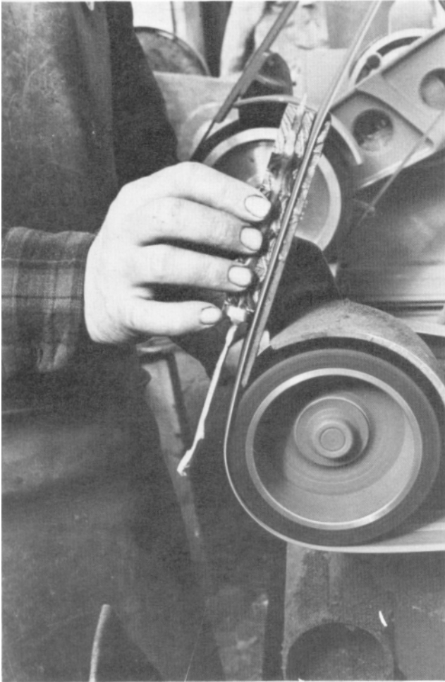
Grinding off the tops of the pins against the flat belt backing keeps the side of the knife flat and even. Otherwise the wood between the pins tends to dish out during the shaping.
