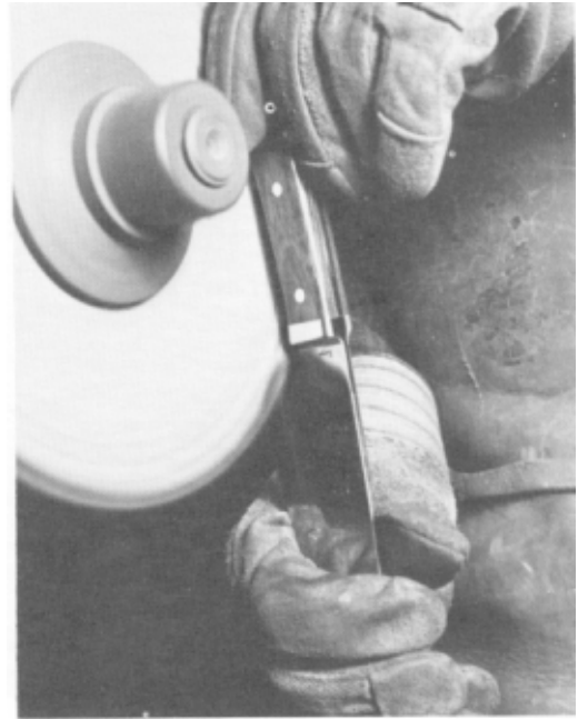
The side of the dropped edge on a chef's knife is another tricky spot to buff.
