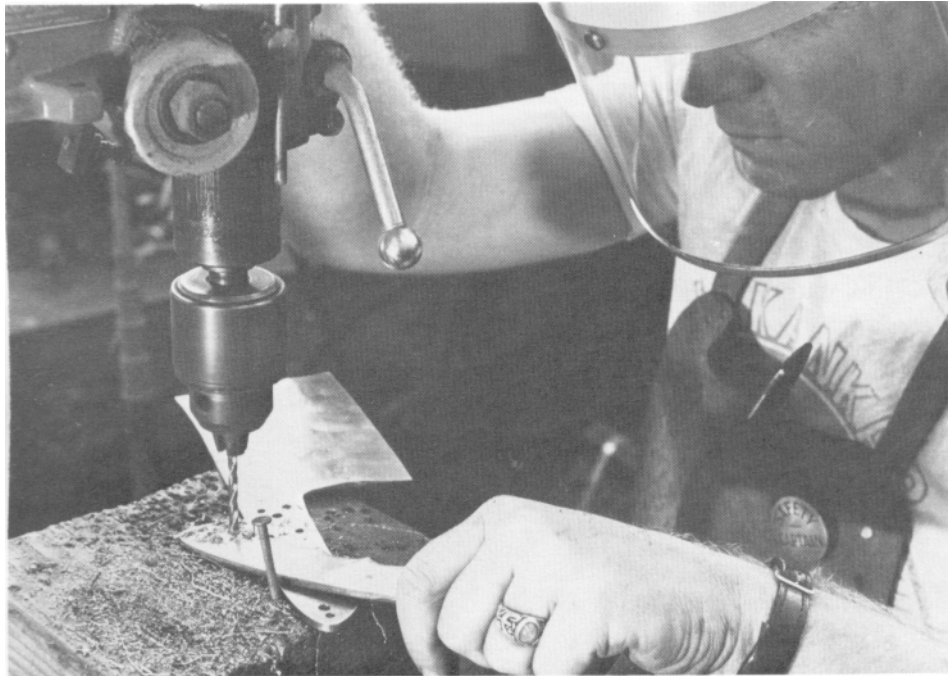
Moving a hole that was started a little off center.
