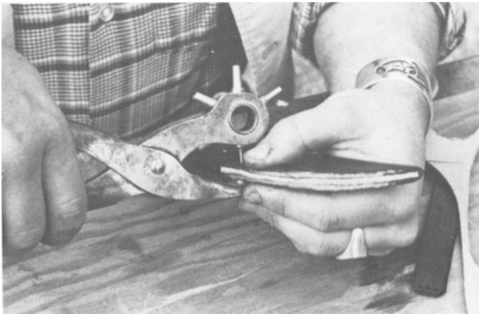
10. Punch two larger holes at the top of the blade case so there is room to begin with a quadruple stitch.
