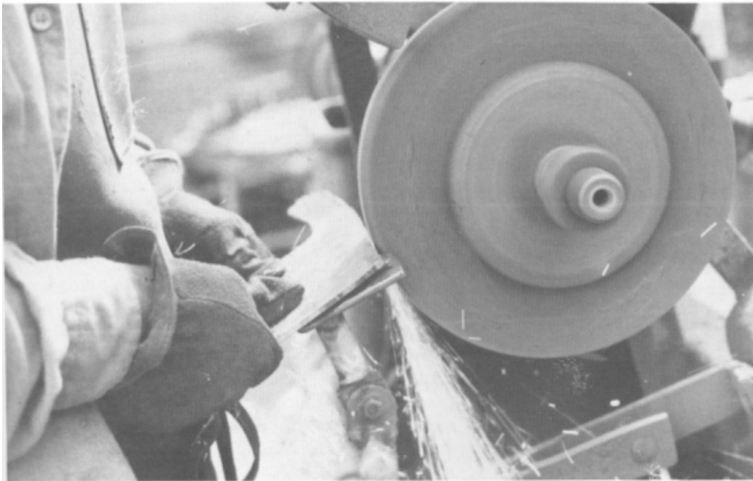
Refining the shape of a chopping knife with a heavy grindstone.
