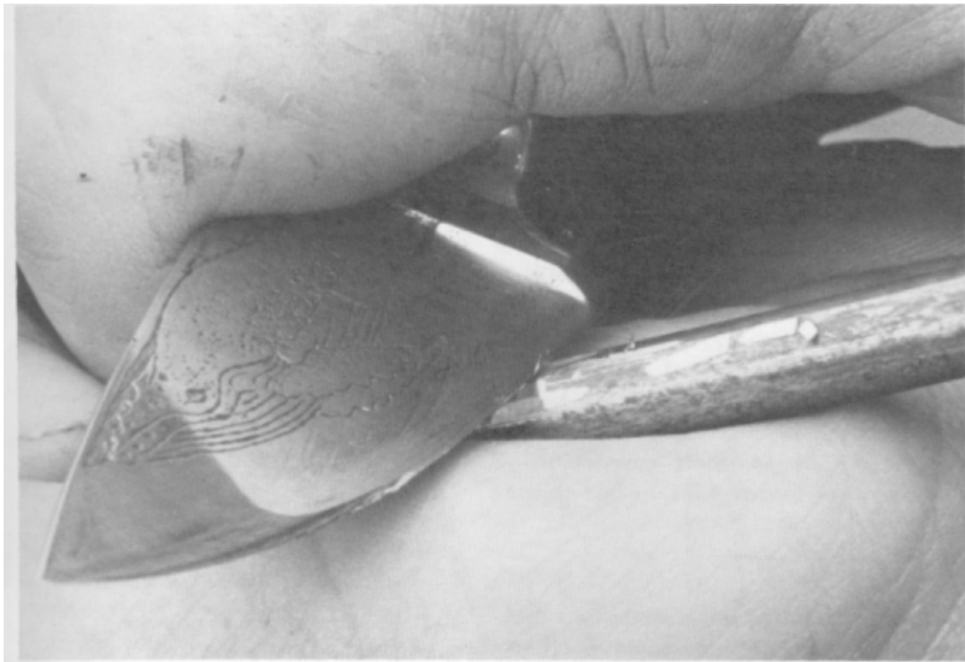
Saw-blade steel knife shaving strips of steel from a large nail, showing the difference in hardness between the two steels.
