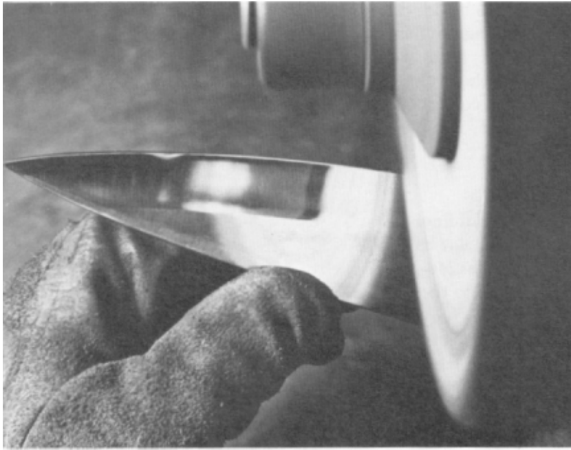
A view from the operator's position, looking down at a medium chef's knife being buffed.
