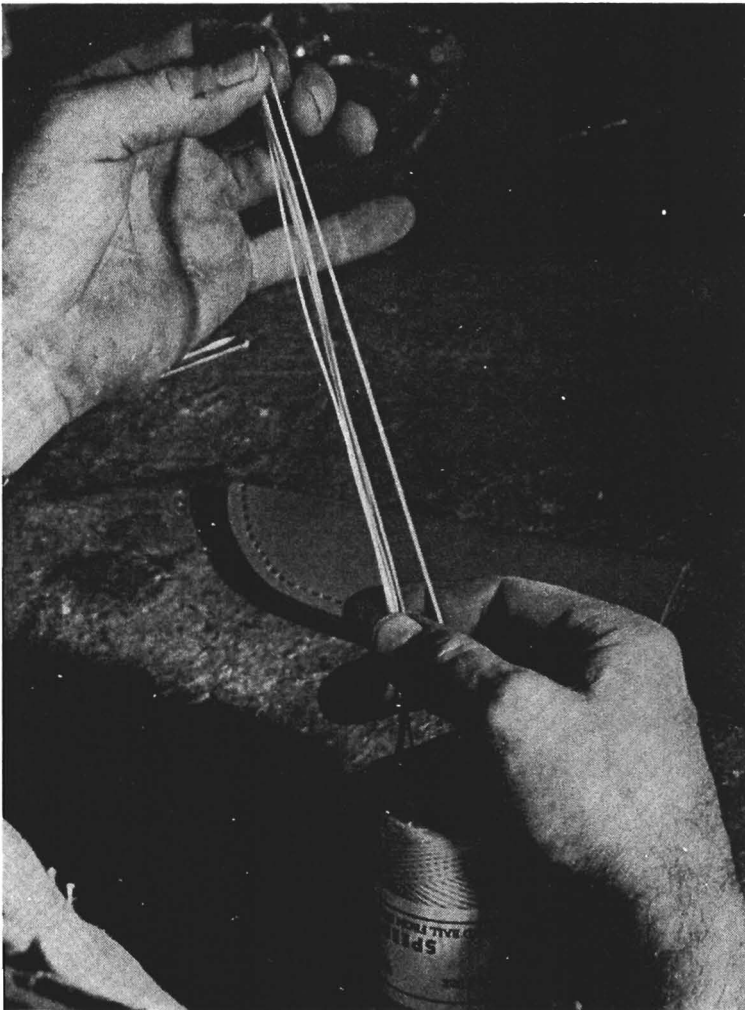
N. Author measures out waxed nylon thread to be used for stitching; length of thread should be approximately eight times length of area to be stitched.
