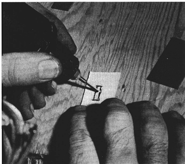
The Dremel Moto-Tool, shown here being used to cut tang slot in spacer material, is useful for a variety of knife-making chores. The author advises the purchase of a variable-speed model with ball bearings for long life and satisfactory service.
