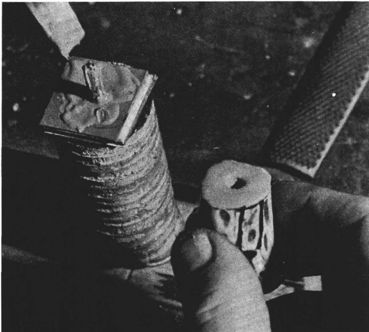
G. With handle and spacers in place, coat the tang with additional epoxy and screw the pommel into place. Allow epoxy to cure before proceeding further.
