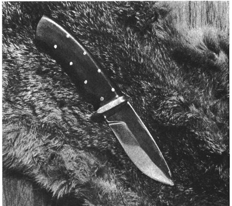
Buffalo-horn scales, pinned to tang, were used to construct this drop-point hunter. Scales and blade are from E. Christopher Firearms Company.
