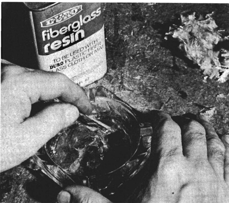
C. Chopped fiberglass is mixed into the resin with hardener added.
