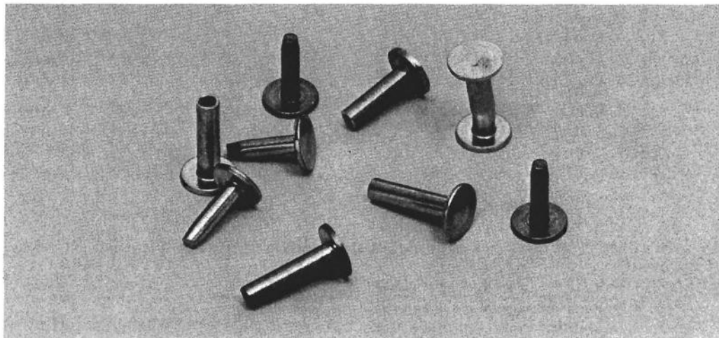
Cutlers' rivets consist of two pieces with identical heads. The shaft of one is solid, and makes a tight fit into the hollow shaft of the other piece.
