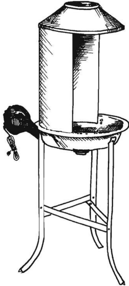
A commercially made portable forge. This small forge offers an inexpensive and practical heat source for a beginning knifemaker. They are available new and can sometimes be found for sale at farms or small industries.
