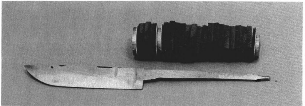
Parts of the knife before assembly. The blade has been rough filed, but further work is needed before heat treating.
