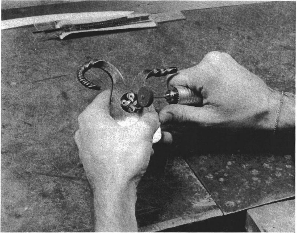
After piercing the design with the jeweler's saw, it is given relief by careful grinding with a small abrasive wheel.
