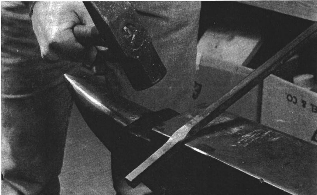
A bar of steel can be cut at red heat by setting it over the edge of the anvil like this.
