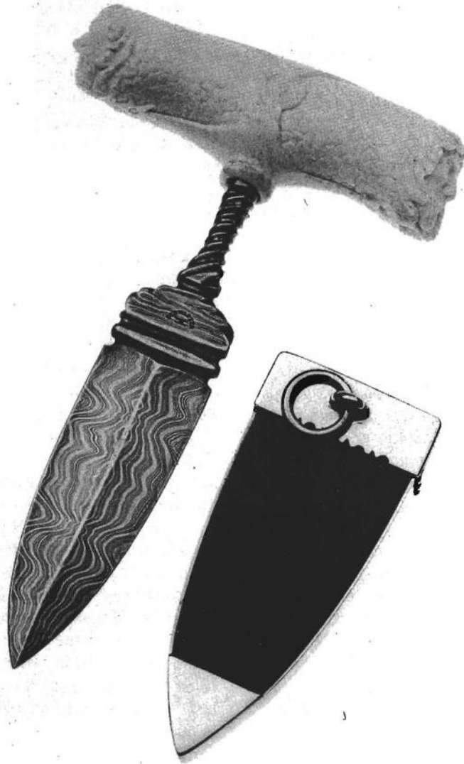
A push dagger by Stephen C. Schwarzer. The Damascus steel is set off by the twisted shank and carved ivory handle. The sheath is made of nickel silver and African frog skin. (Photo by Weyer of Toledo)
