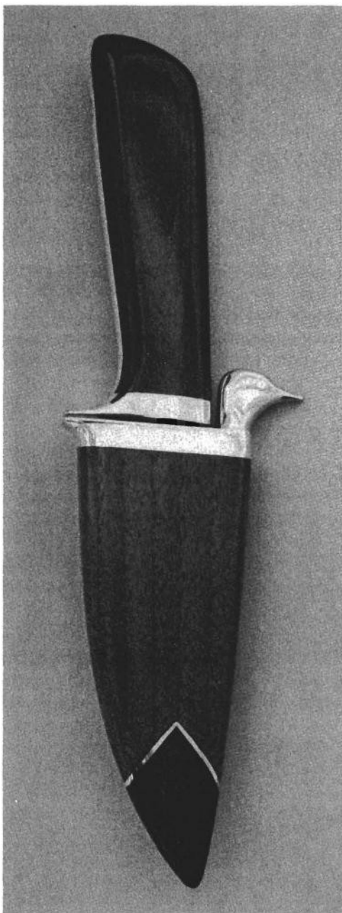
A utility knife by Alf Ward in 01 steel, brass, and walnut. Notice how the guard and the rim of the sheath work together. (Photo courtesy of the artist)
