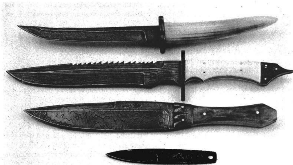
Four knives by Master Shiva Ki, illustrating a few knife formats. The blade material here is Damascus, or pattern-welded steel.
