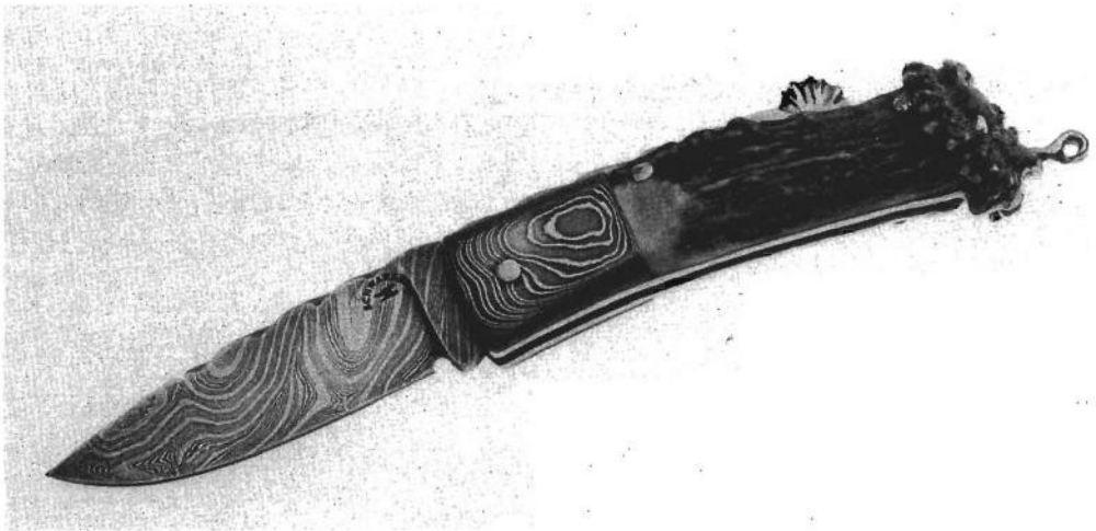
A lockback with Damascus blade and bolster by Stephen C. Schwarzer. (Photo by Weyer of Toledo)
