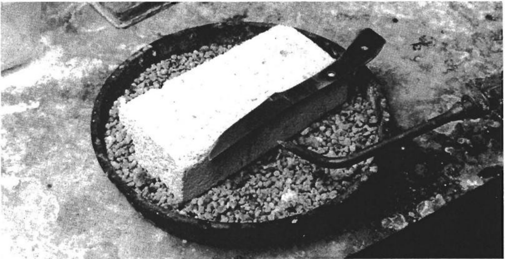
A blade is tempered over a torch flame as shown. More heat flows to the thick part of the blade, which overhangs the brick. The thin cutting edge could be further protected by setting a scrap of steel on it, or by building up a layer of clay on it.
