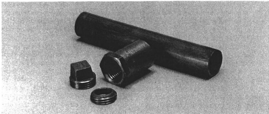
Standard plumbing fittings are used for the handle of this knife.
