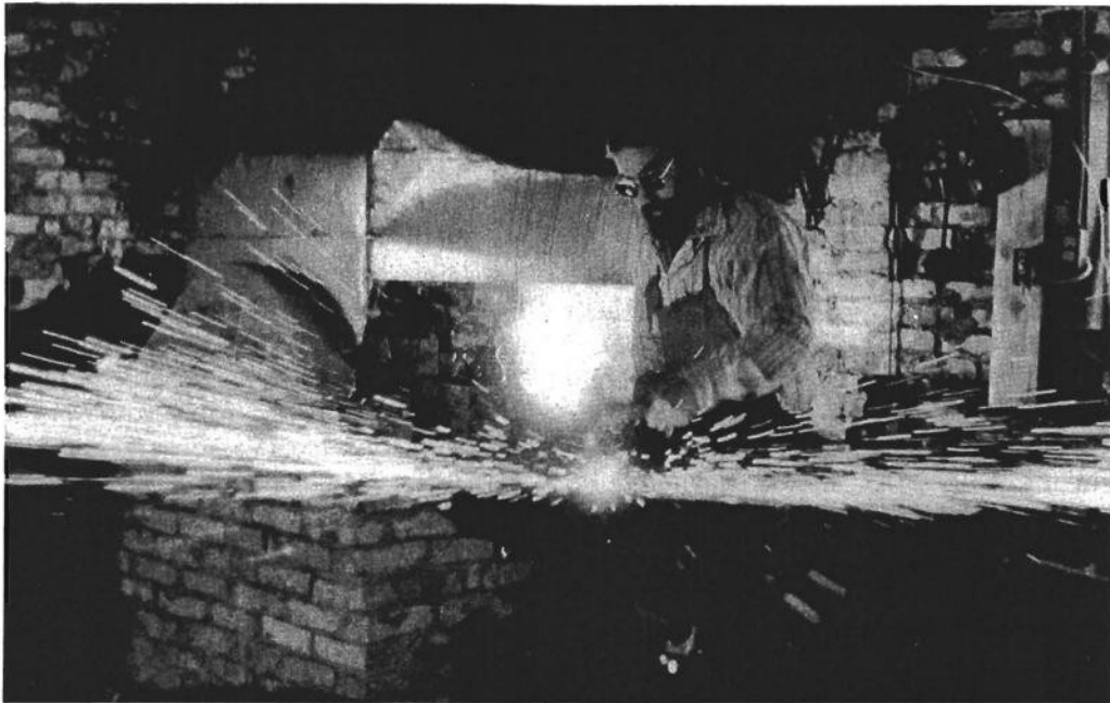
Forge-welding is always dramatic. Here Scott Lankton strikes a blow that will help fuse many layers together. (Photo courtesy of the artist)
