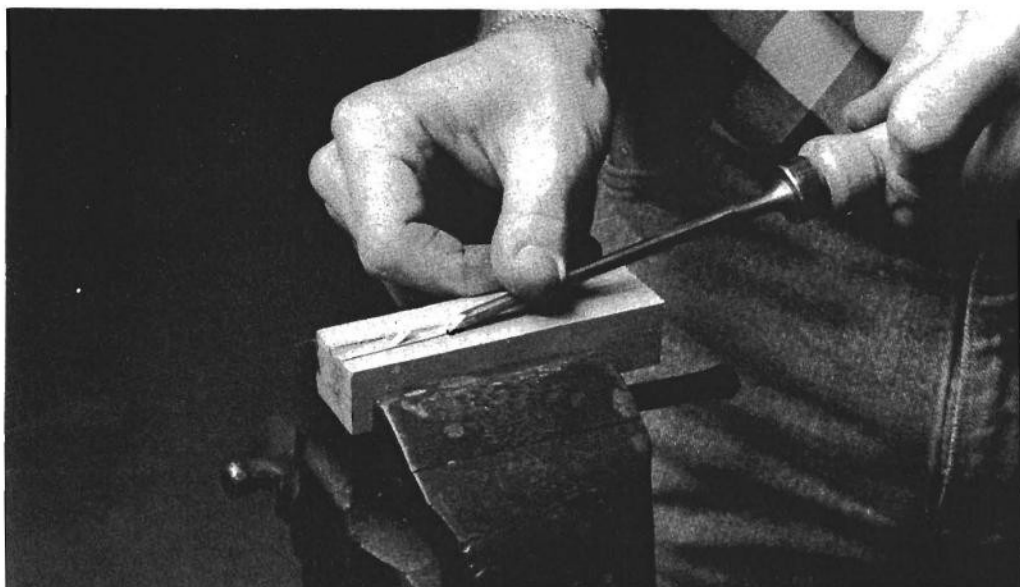
With the handle block set into the vise, carve a recess equal in depth to half the blade thickness.
