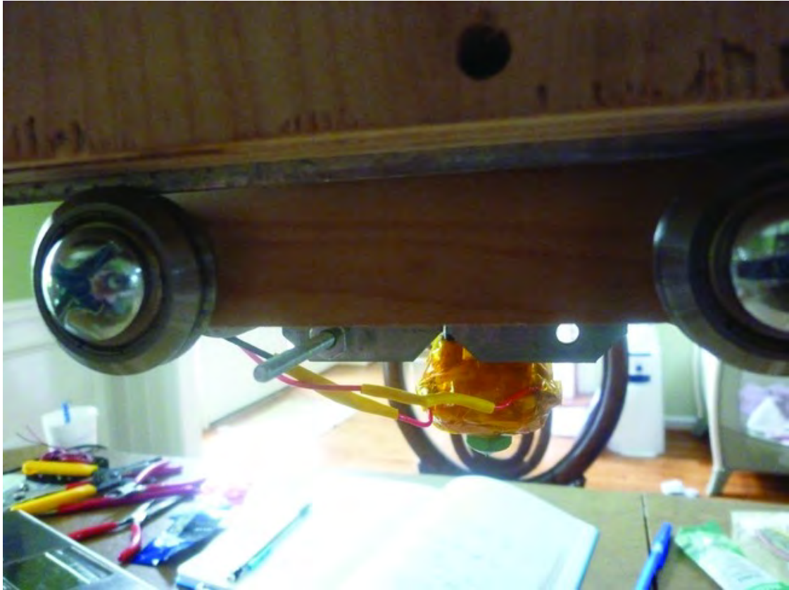
Figure 18-25. A machine screw will be used to trigger the final endstop.
