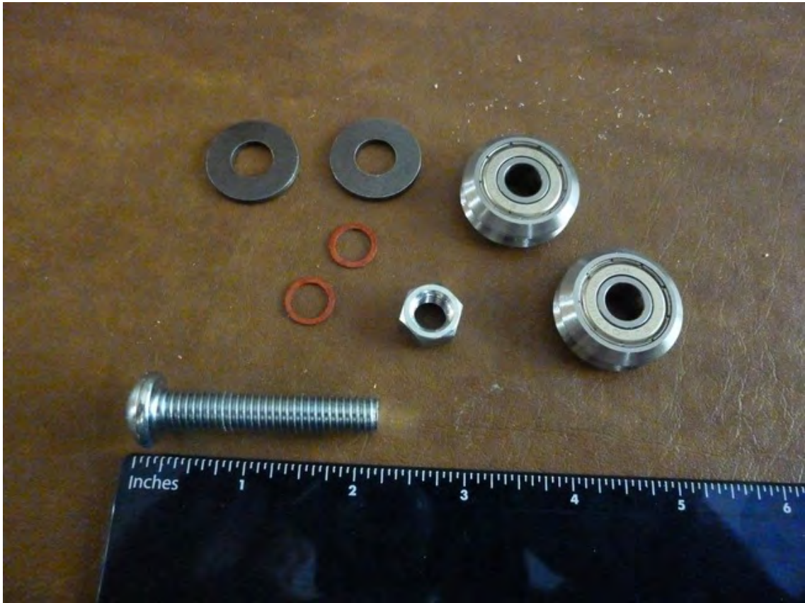
Figure 10-11. These eight pieces will make one V-groove bearing assembly.
