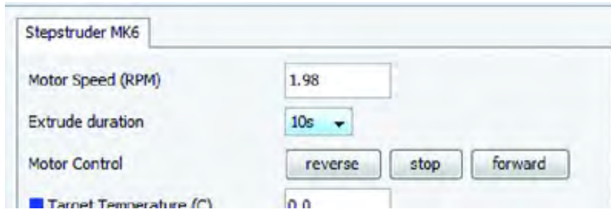
Figure 20-2. Set the Motor Speed and Extrude Duration.
