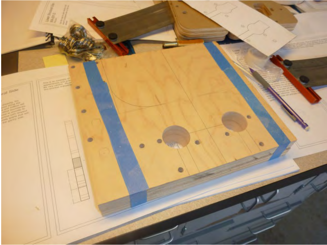
Figure 7-19. Parts A and B each have two large holes drilled.
