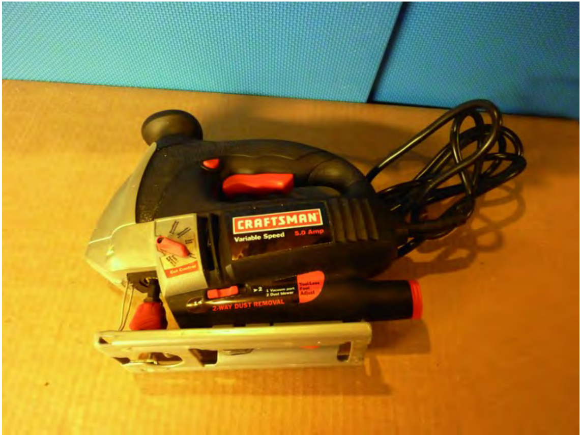
Figure 2-7. A jigsaw can help remove material in corners.
