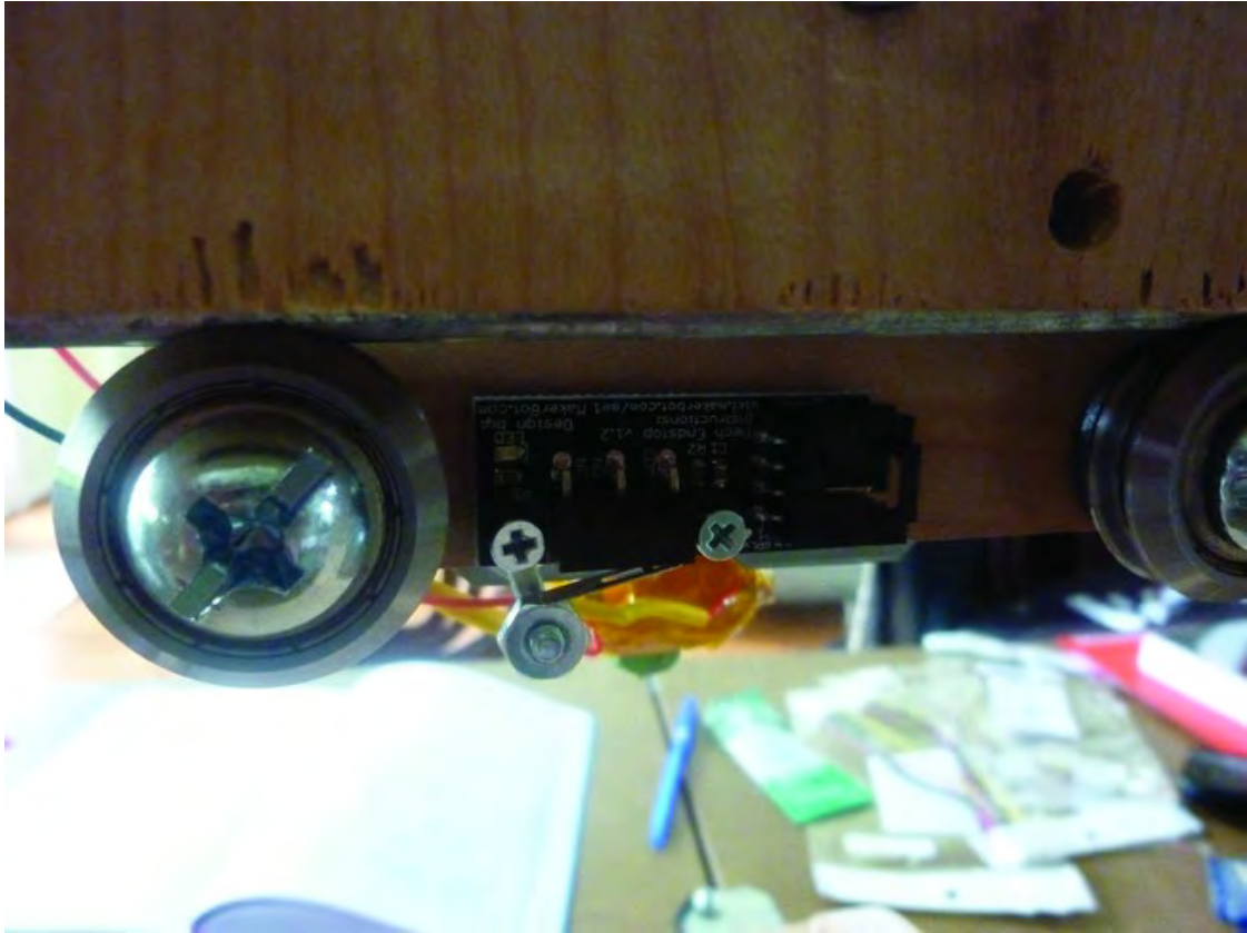
Figure 18-26. The endstop's pushbutton will be pressed by a second #6 nut.
