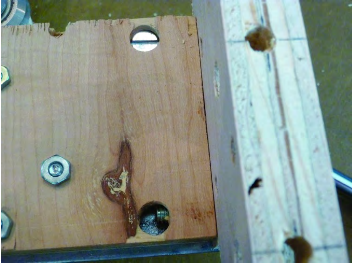
Figure 11-7. Using a bolt and barrel nut to secure the Upper Structural Side
