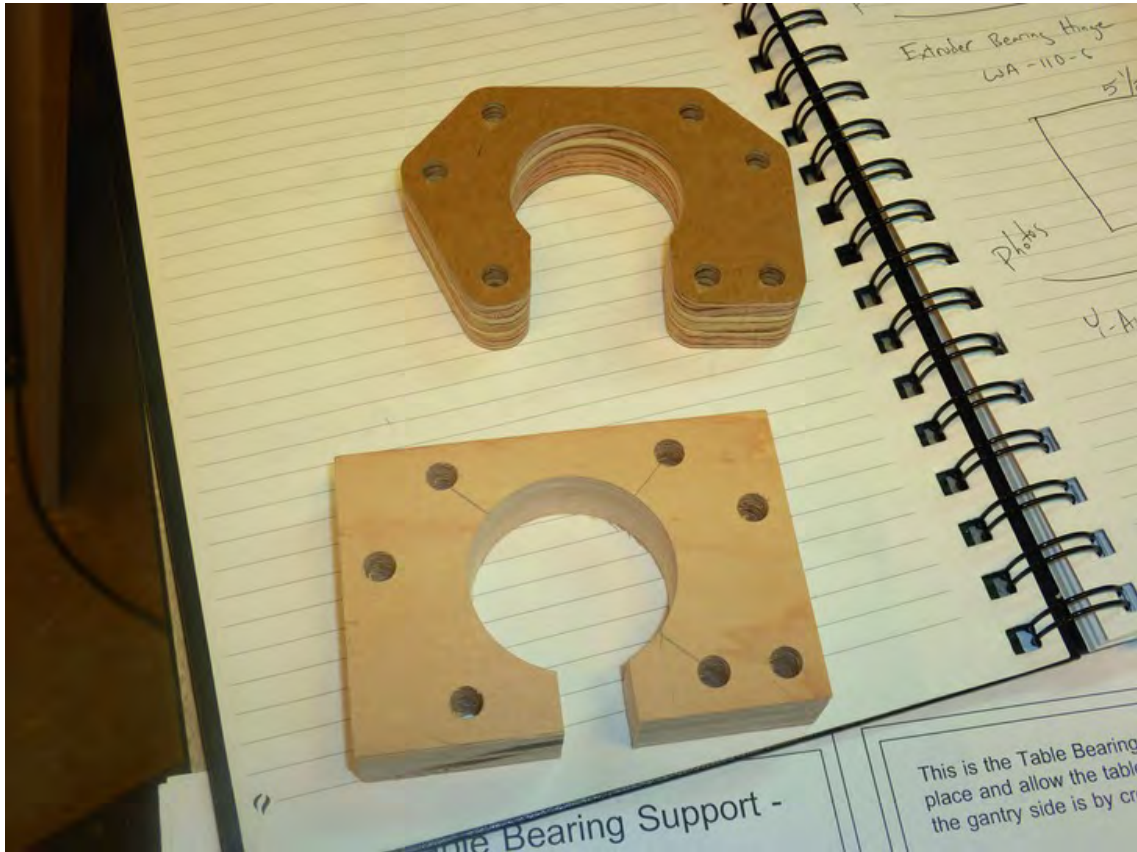
Figure 8-10. Part R in plywood (on bottom) and MDO (on top)
