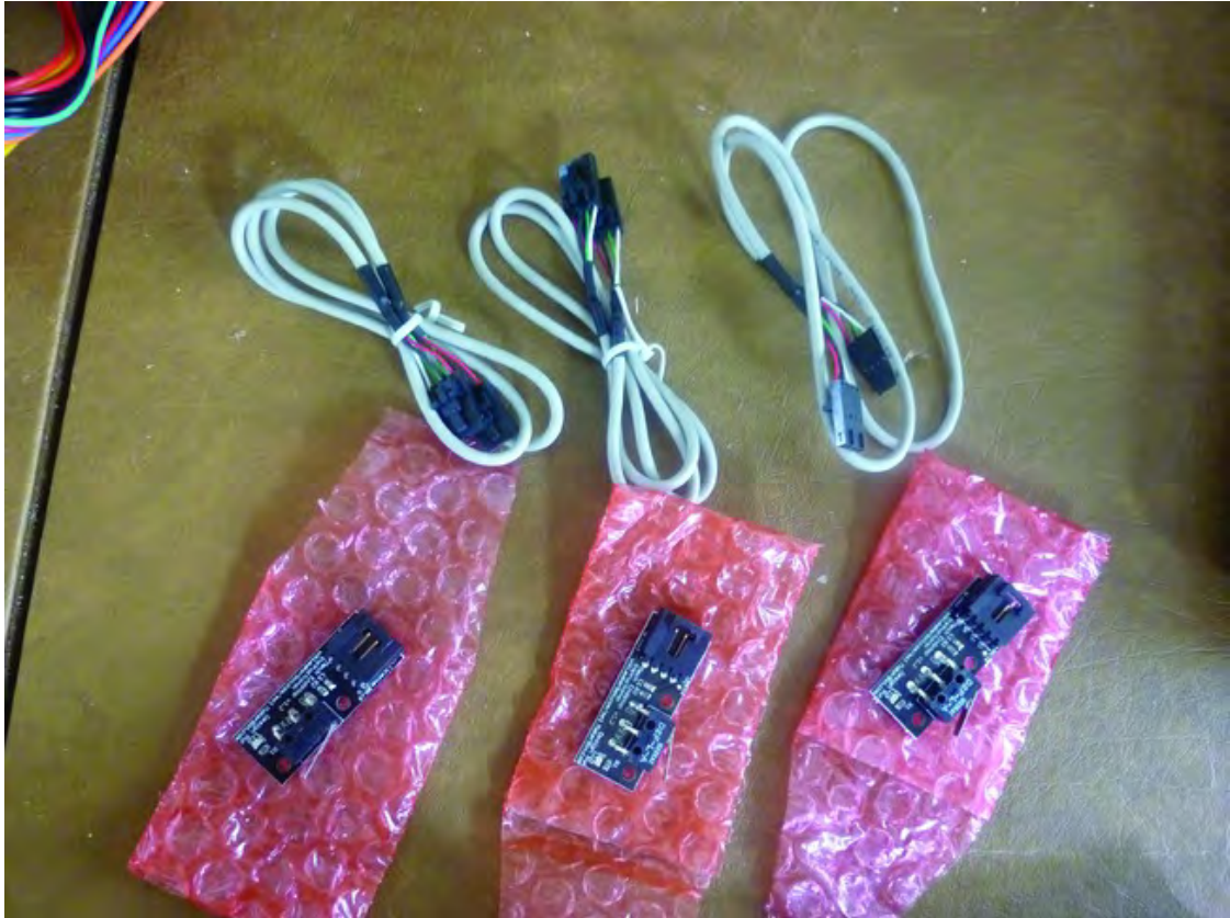
Figure 18-17. Three endstops, one per axis
