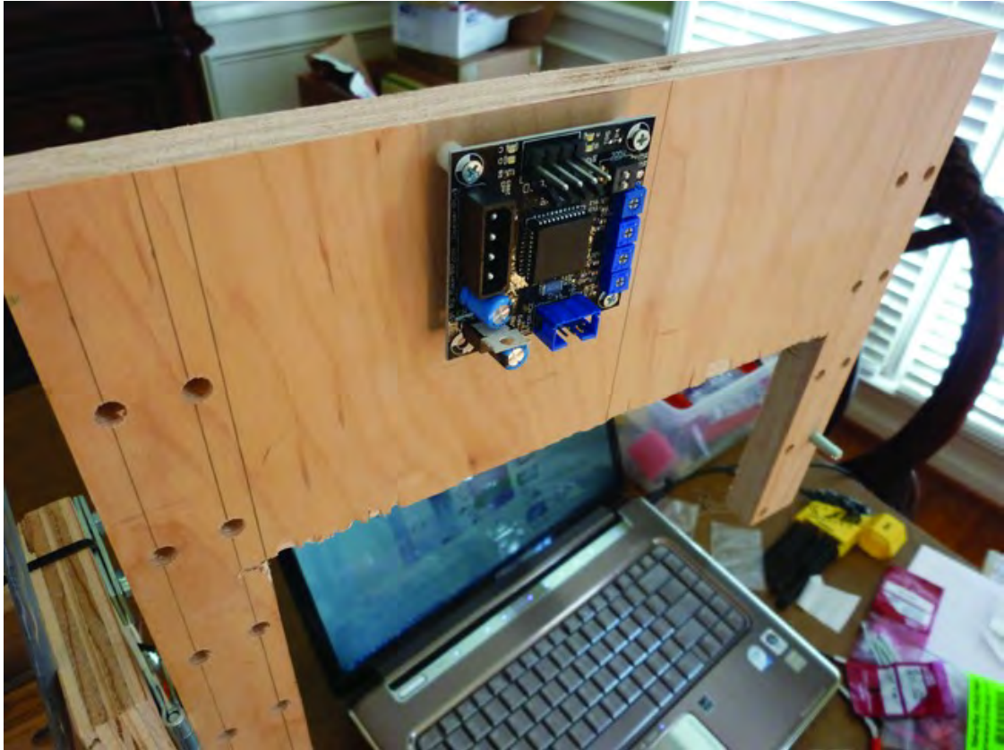
Figure 16-11. The first stepper motor driver attached to the Machine Back.
