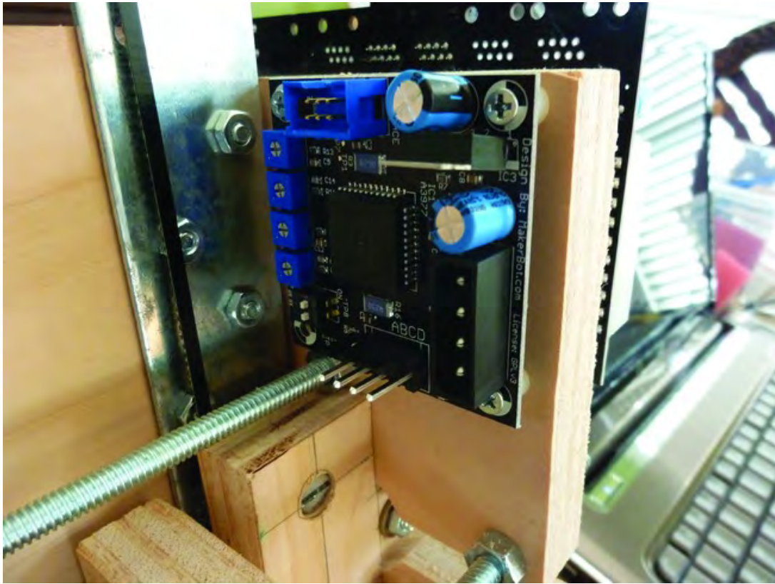
Figure 16-8. The X-axis stepper motor driver mounted on the inside of Lower Structural Side
