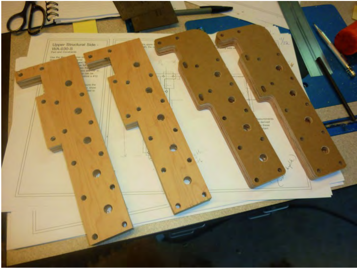
Figure 8-5. Parts F and G in plywood (left) and MDO (right)
