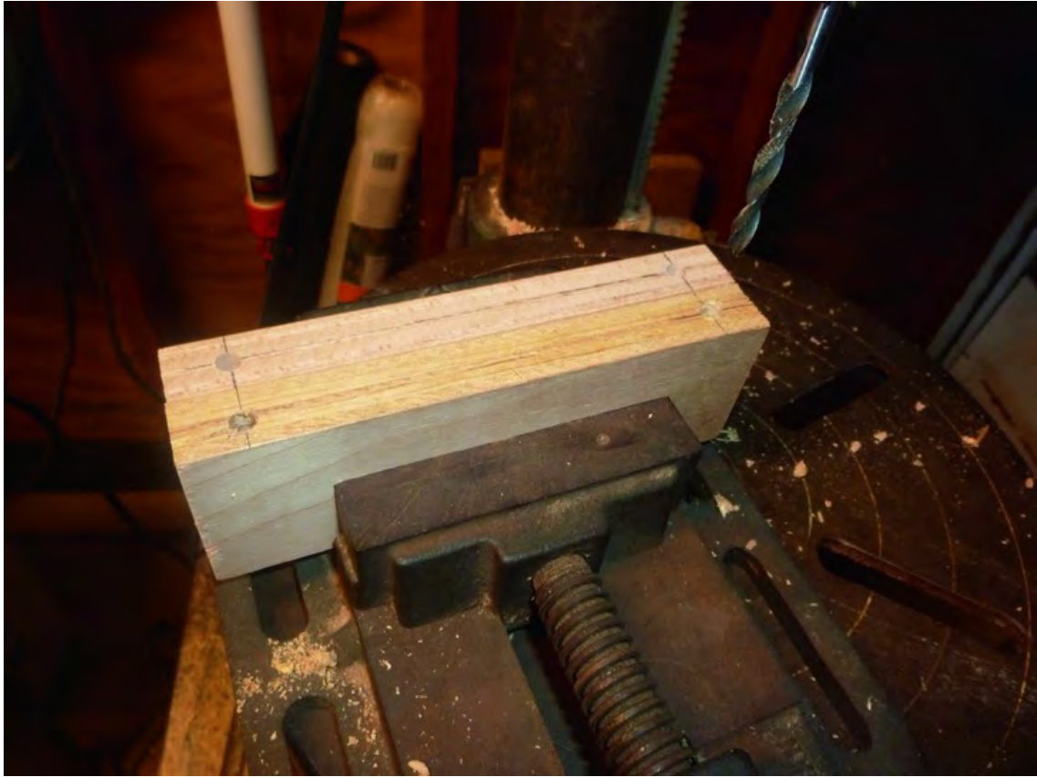
Figure 8-12. Parts I and J with 1/4" edge holes drilled by a drill press.
