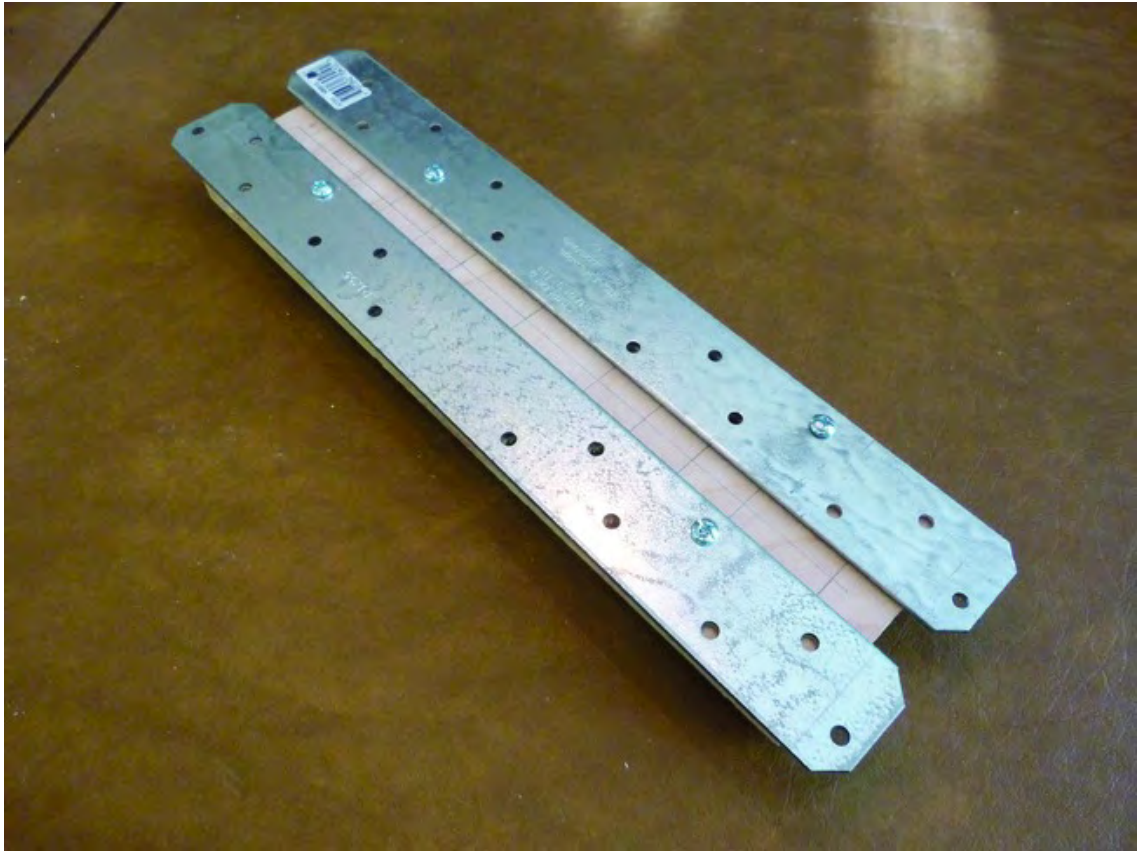
Figure 11-2. Two Strong-Tie rails attached to the Y-Axis Rail Support
