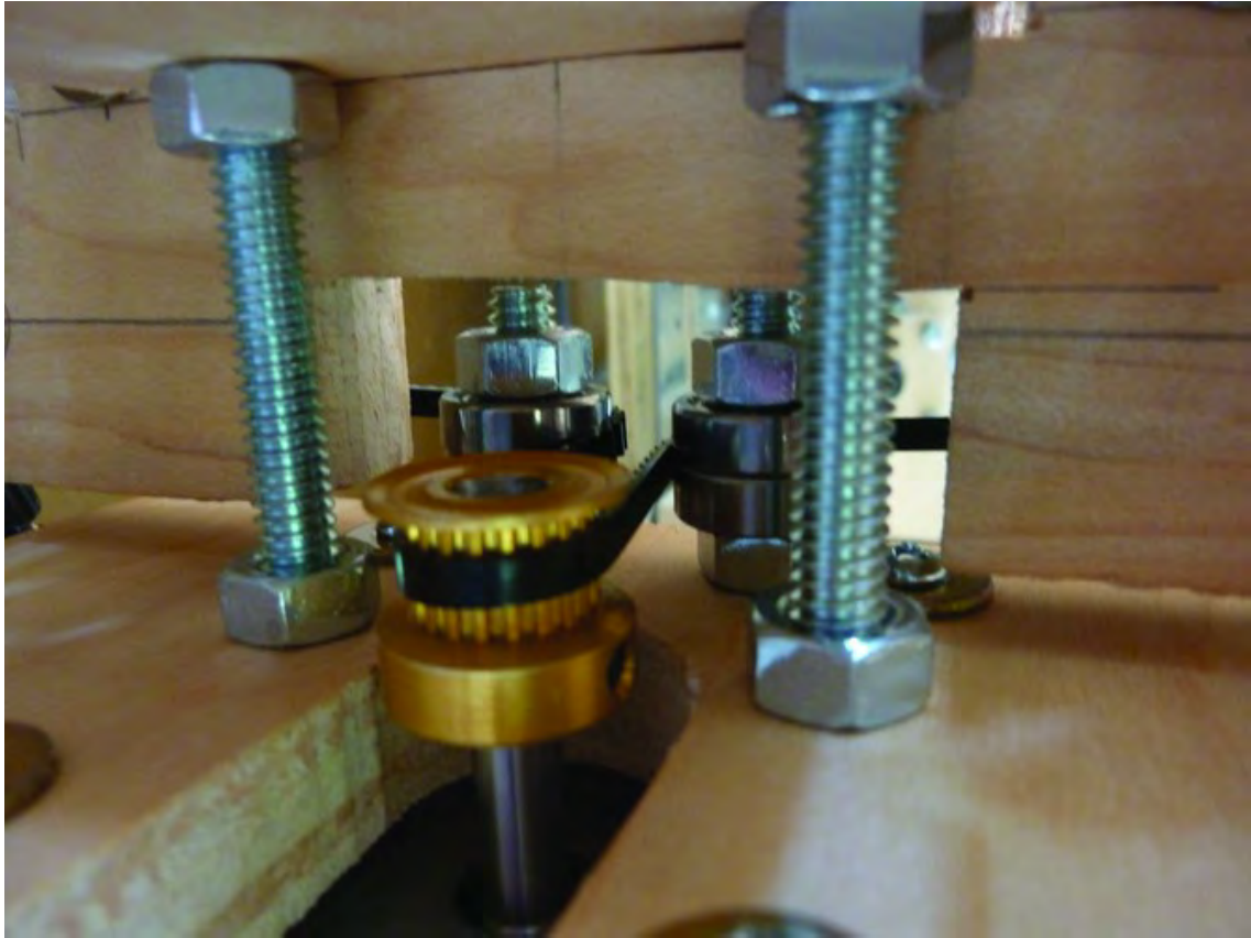
Figure 13-27. The belt wrapping over the bearings and around the pulley
