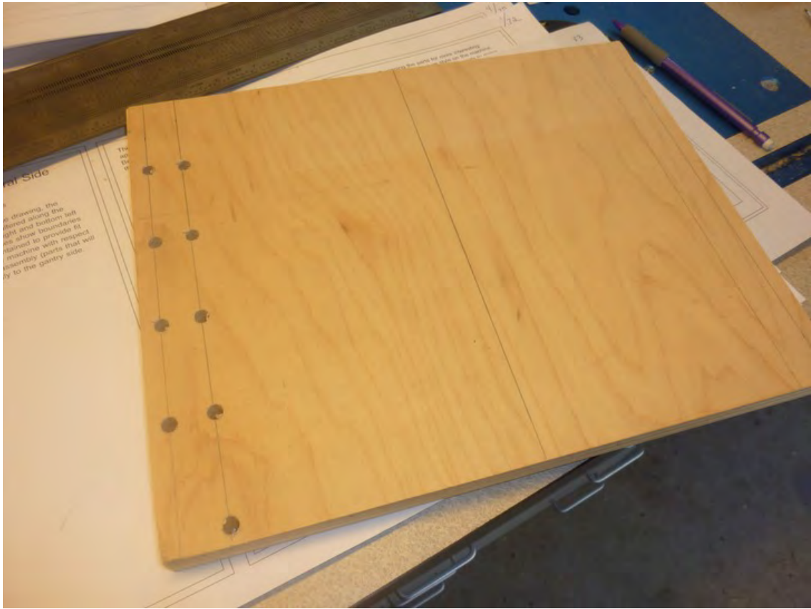
Figure 7-11. The first set of holes drilled down the left side of Part O
