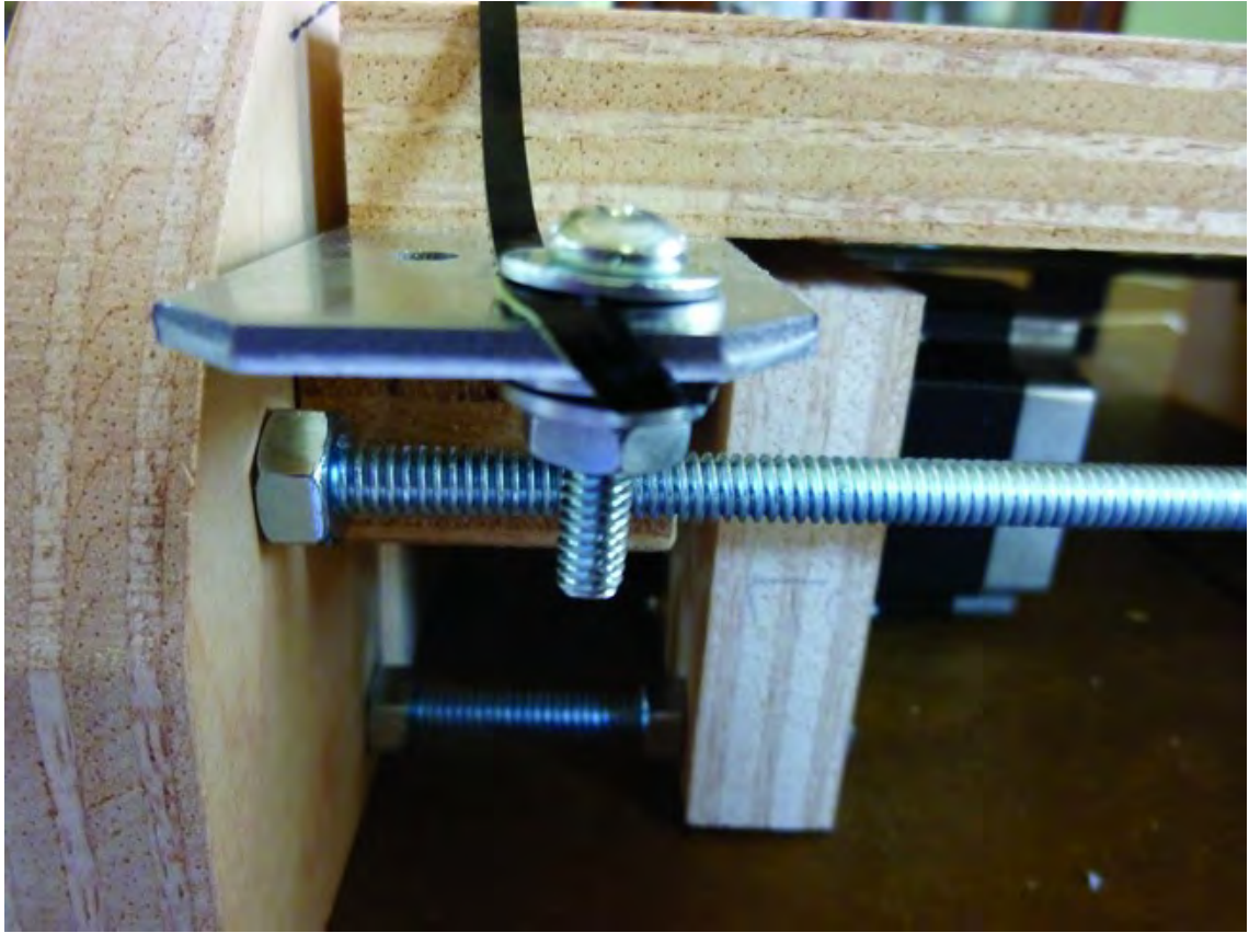
Figure 13-28. Secure the ends of the belt with washers pinching the belt above and below.
