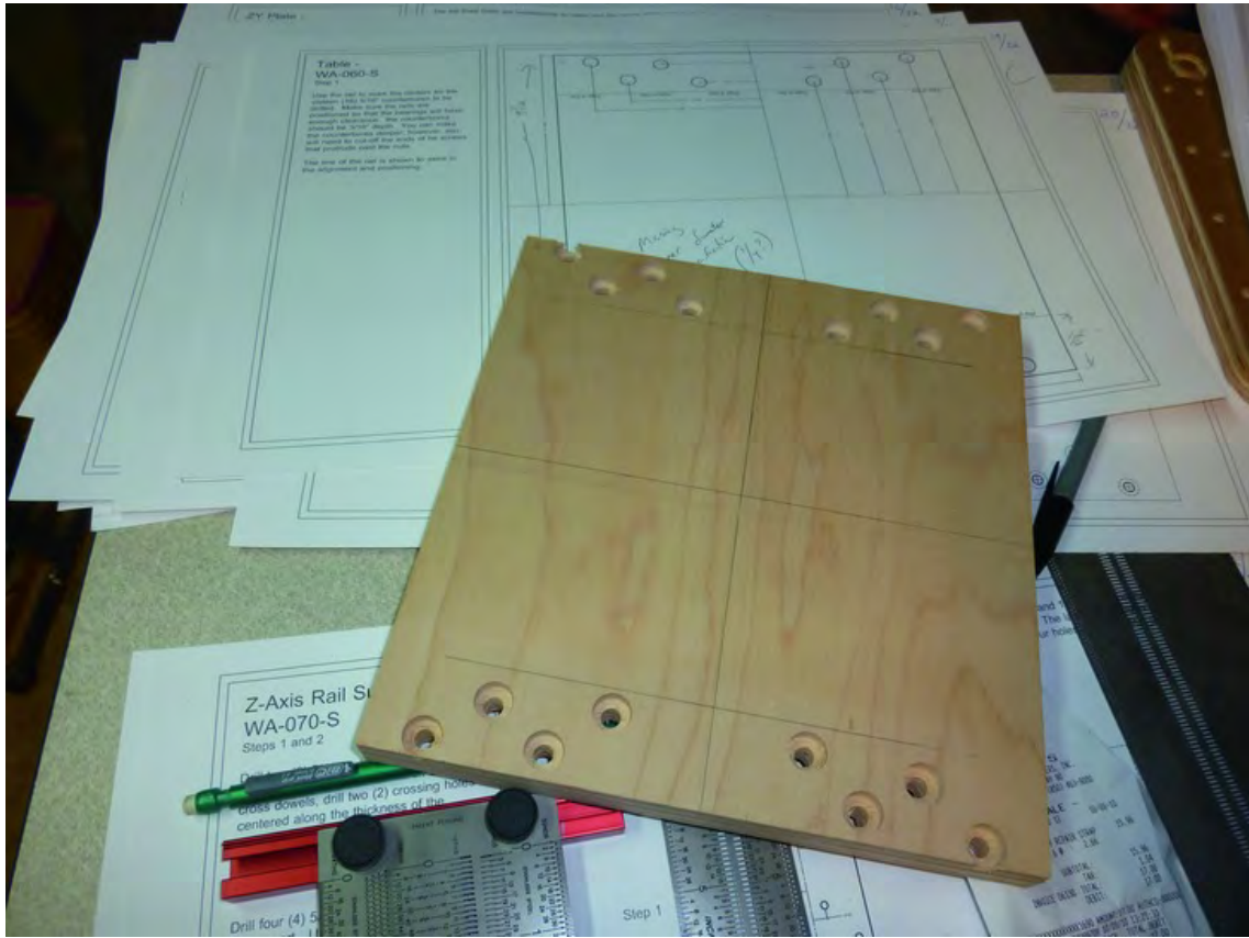
Figure 9-13. Part Part C with all holes drilled.
