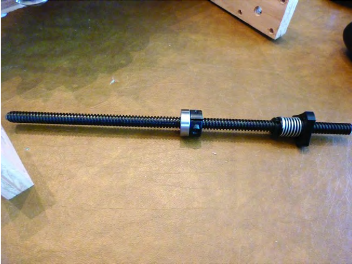
Figure 12-2. A collar and a bearing inserted onto the lead screw
