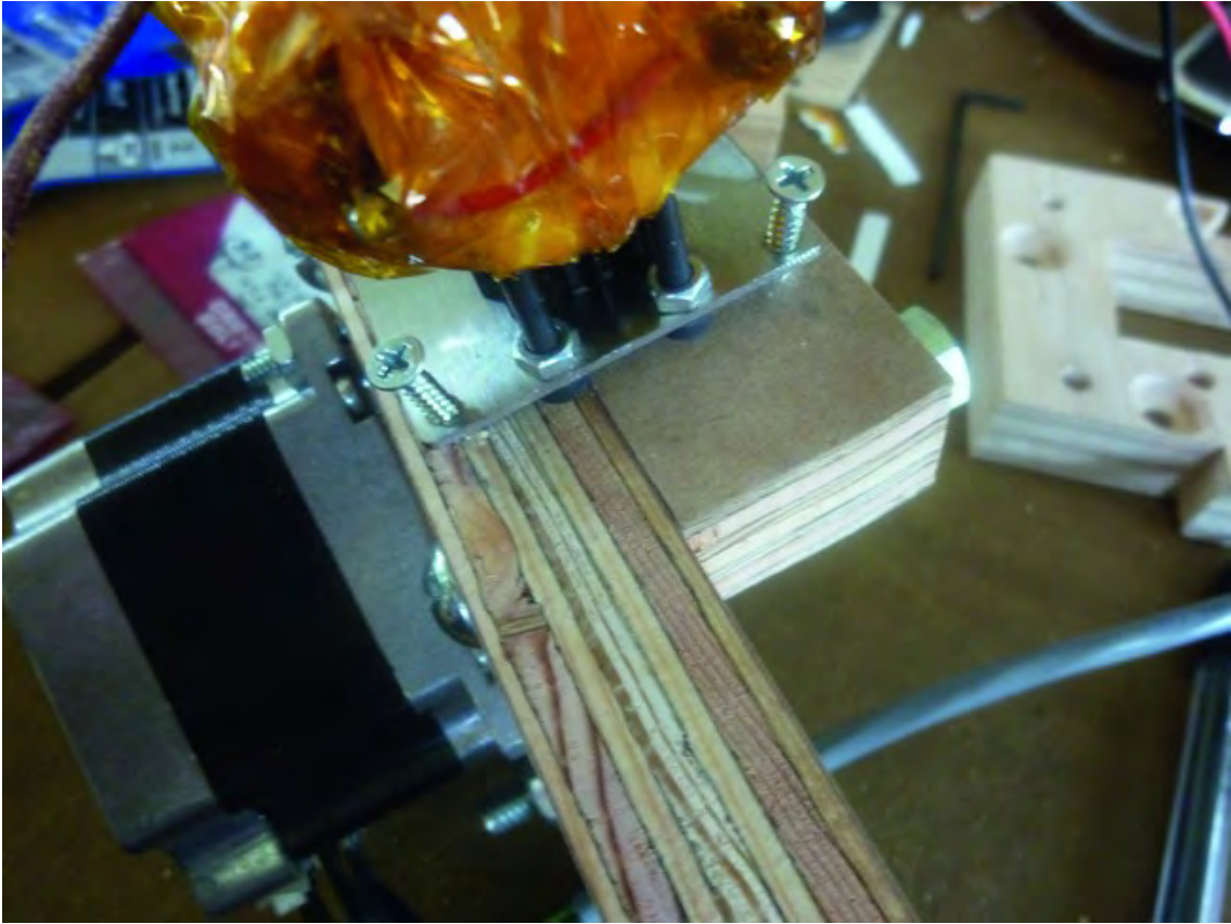
Figure 21-13. Use wood screws to attach the mounting base to Part S and Part Q.
