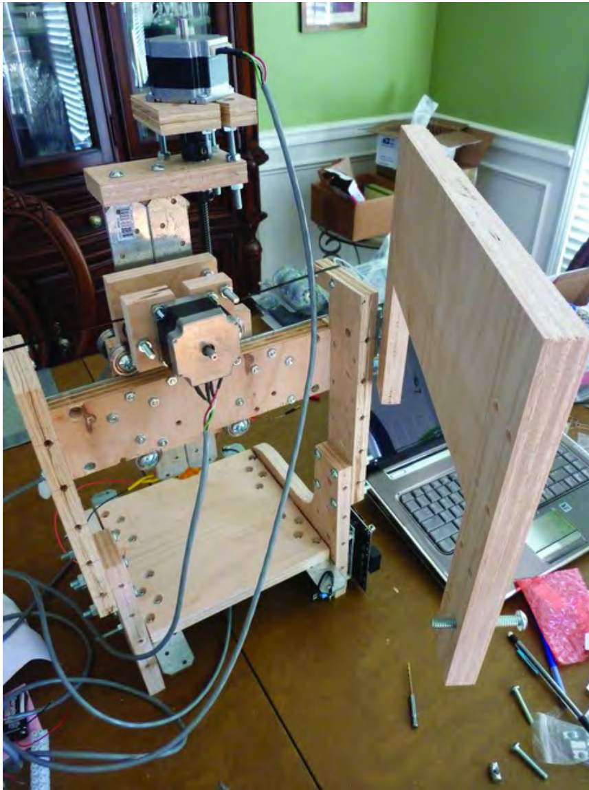
Figure 16-10. The Machine Back swings out for access to stepper motor drivers.
