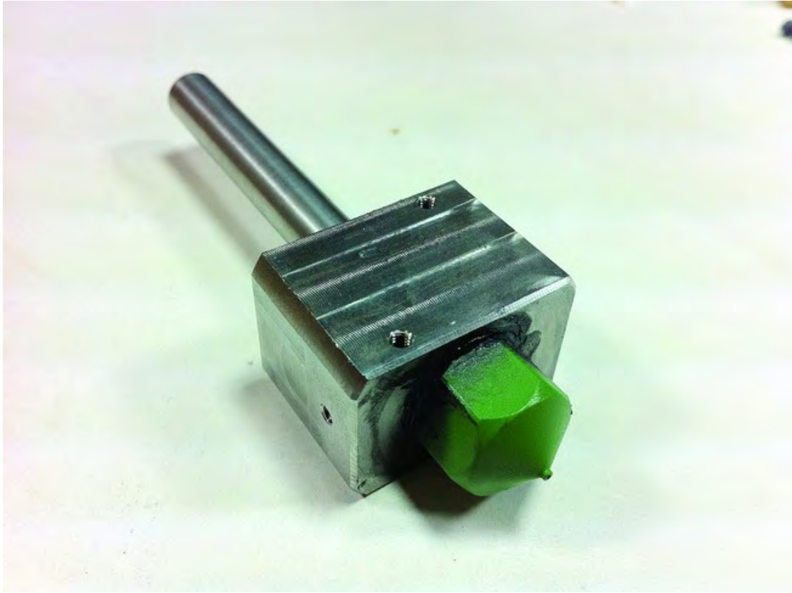
Figure 14-4. Heater core with feed cylinder and nozzle inserted
