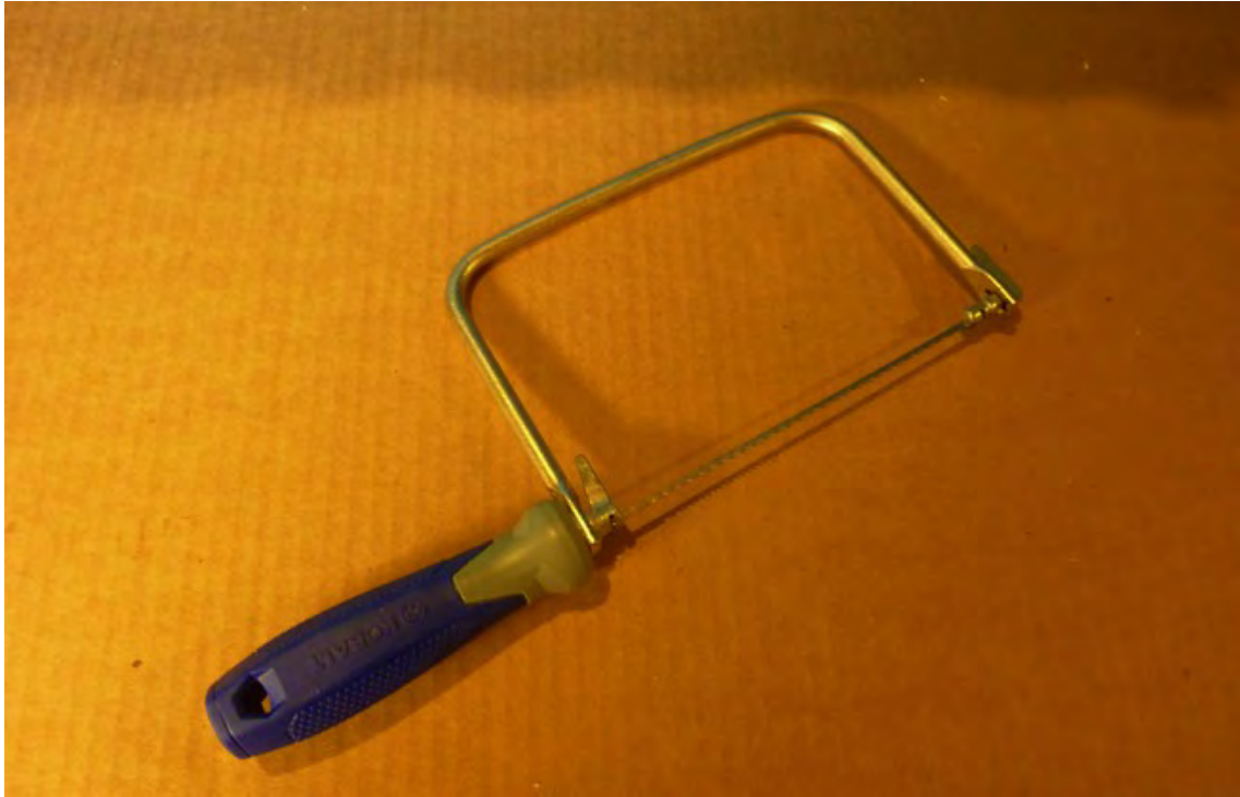
Figure 2-8. A coping saw can also cut ninety degree corners but it's a slow process.
