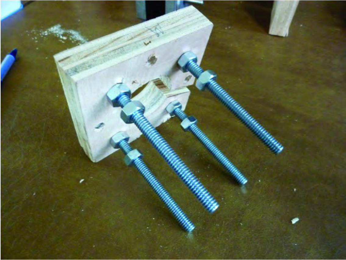
Figure 13-10. Prepare the Z-Axis Motor Mount with four machine screws.
