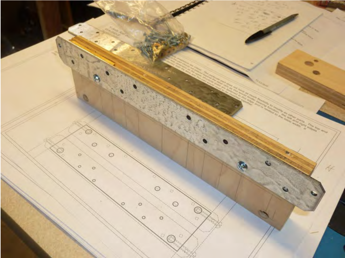
Figure 7-6. Part H with a Strong-Tie bolted on
