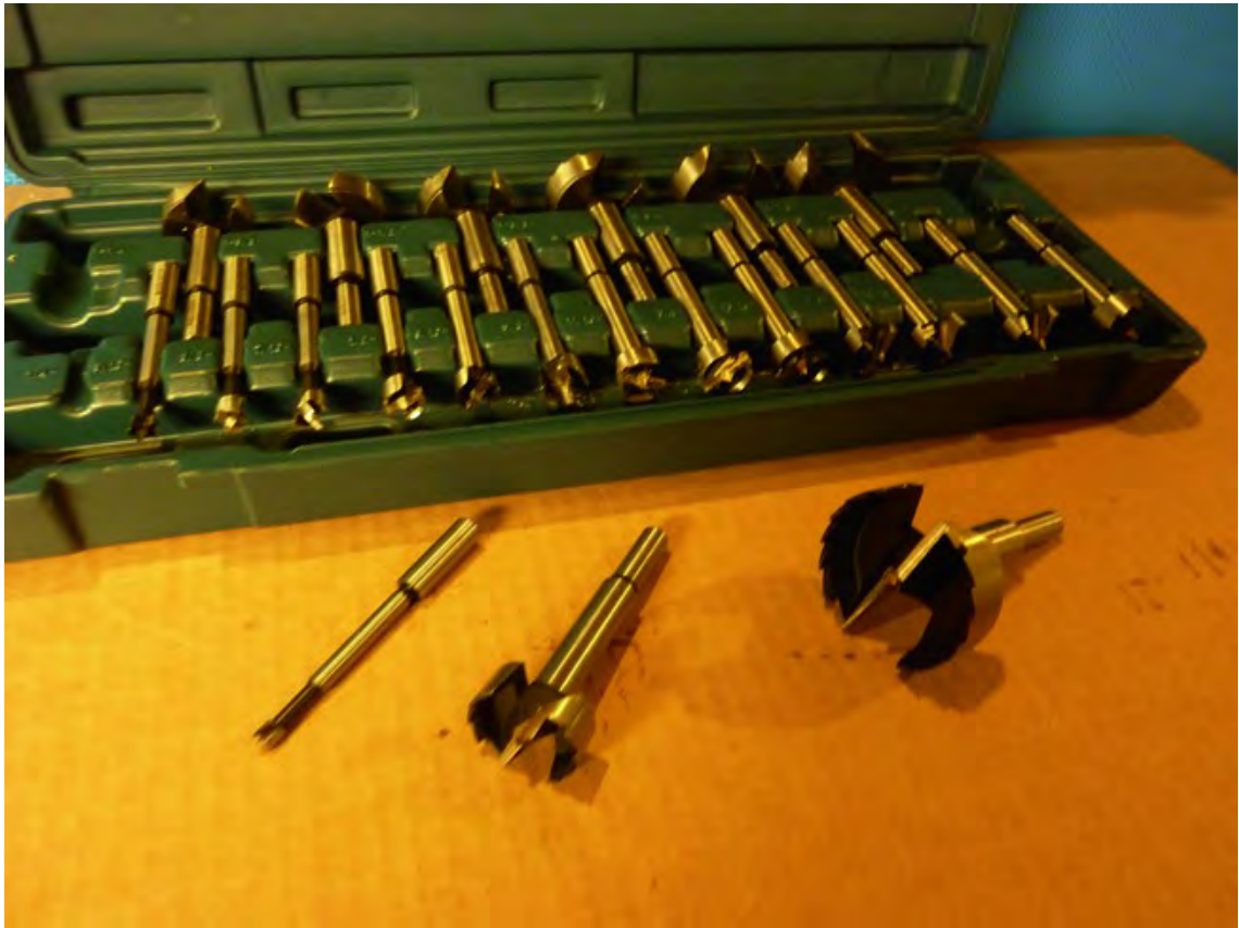
Figure 2-18. Forstner bits drill cleaner, sharper counterbore holes than standard drill bits.
