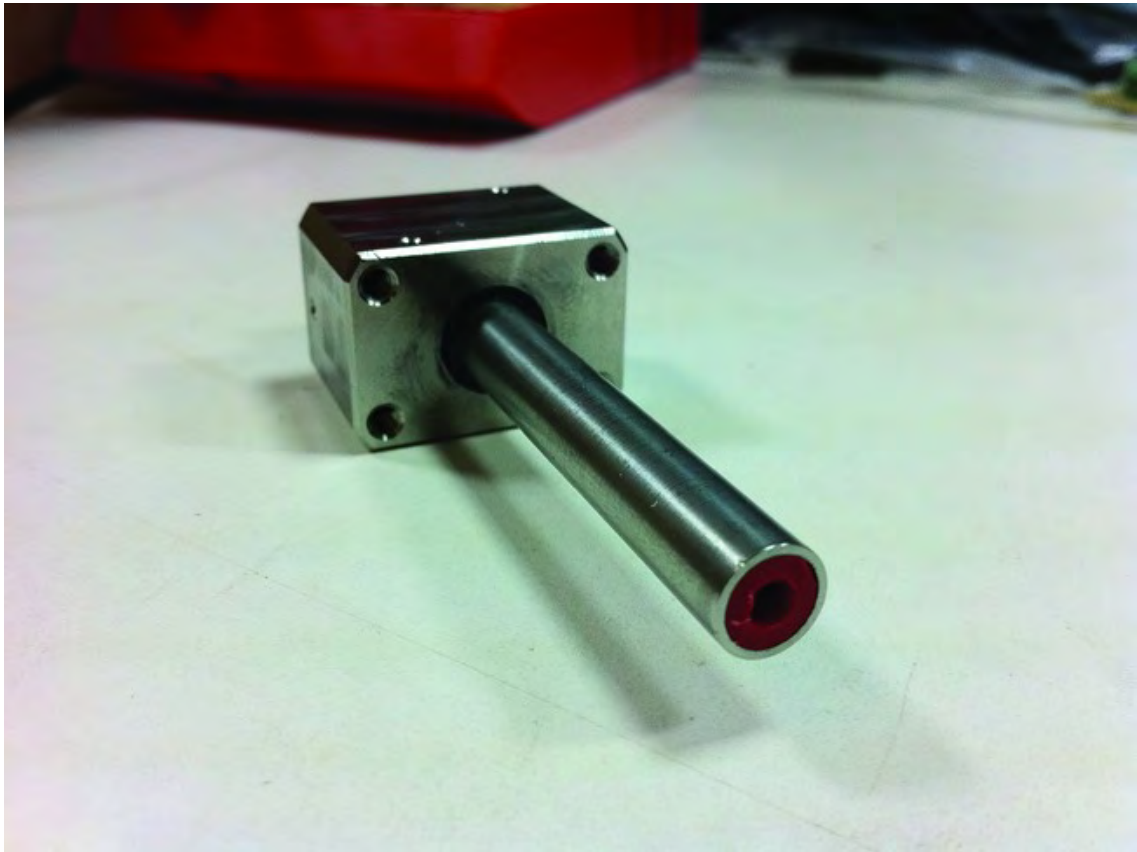
Figure 14-6. Cut the PTFE tube so it is flush with the end of the feed cylinder.
