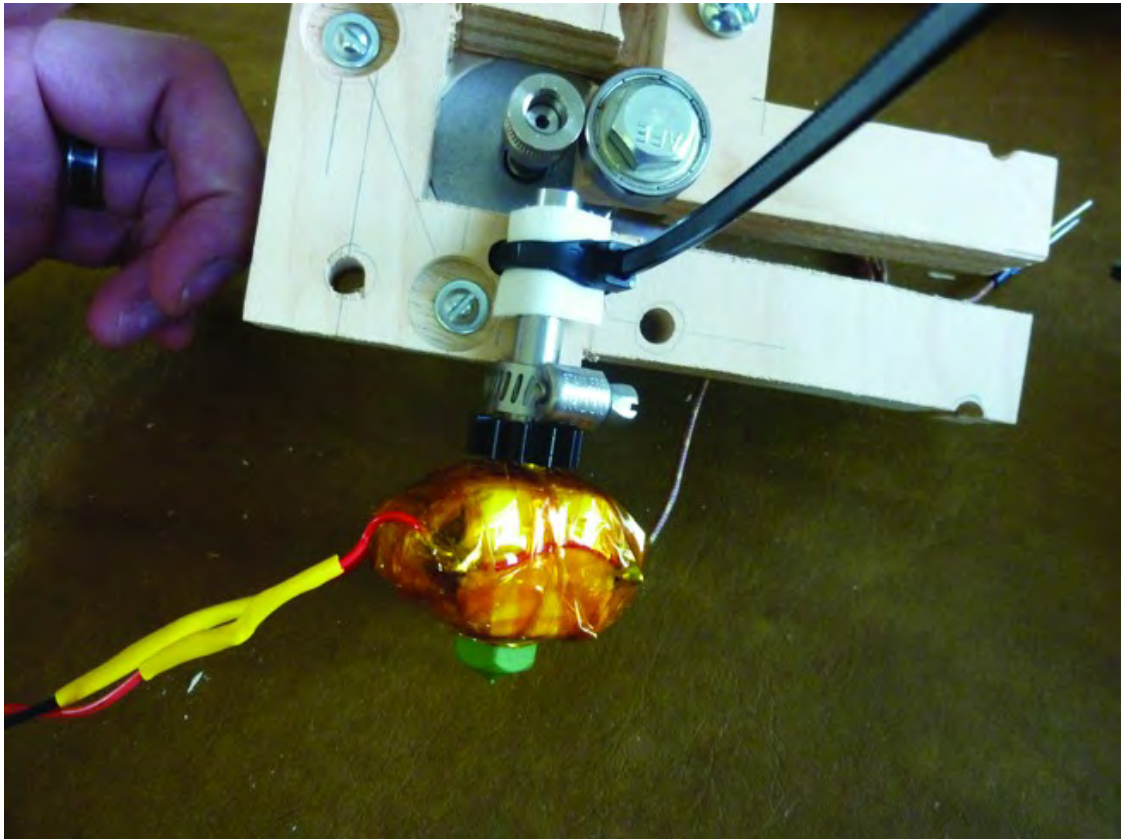
Figure 15-14. The Extruder attached to the filament feed mechanism
