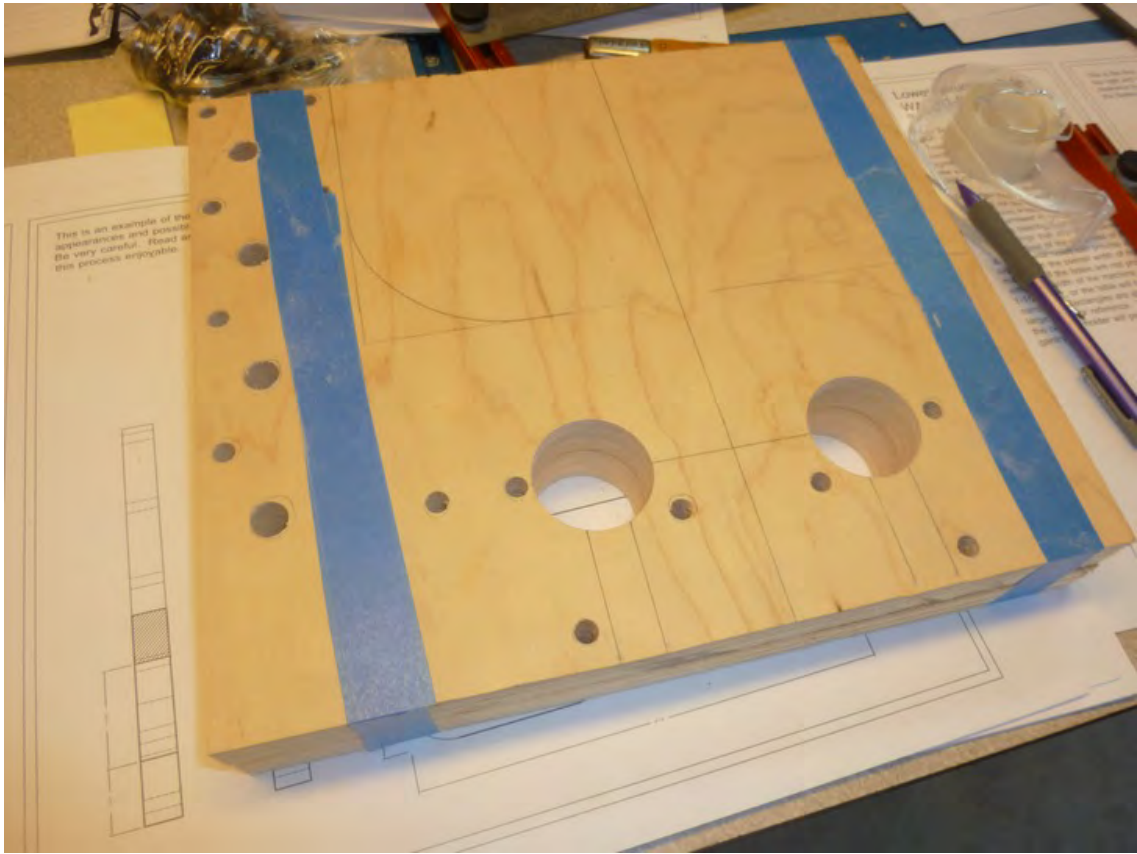
Figure 7-20. Holes drilled through Parts A and B for the barrel nuts
