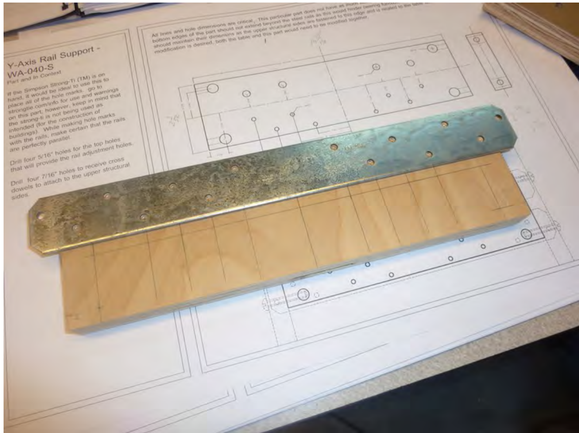
Figure 7-3. The Strong-Tie brackets will be used to mark and drill holes in Part H.
