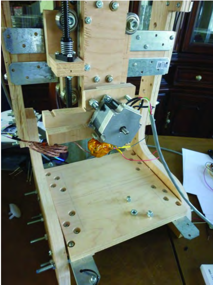
Figure 15-16. Add three 1/4" nuts to secure the mechanism in place.
