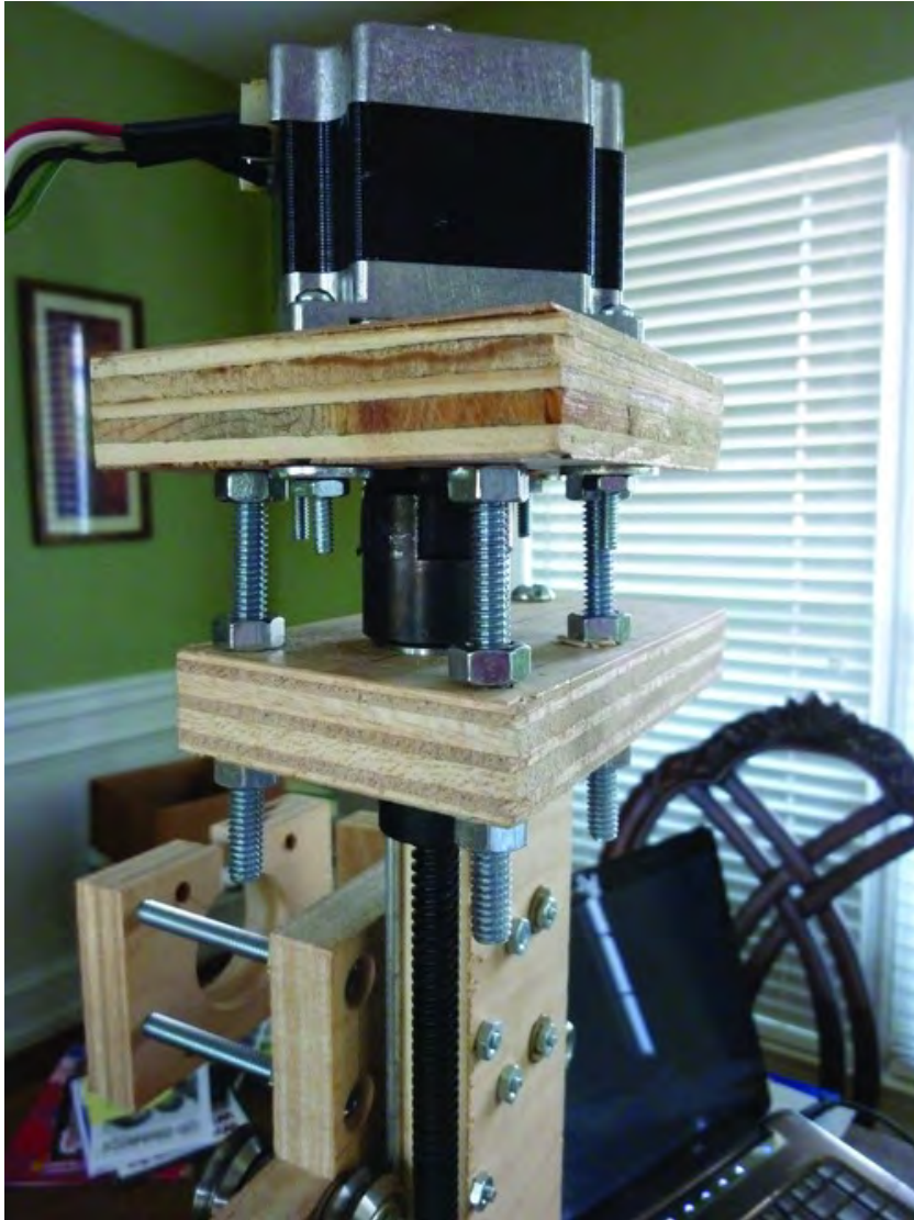
Figure 13-14. Secure the motor mount with the nuts.
