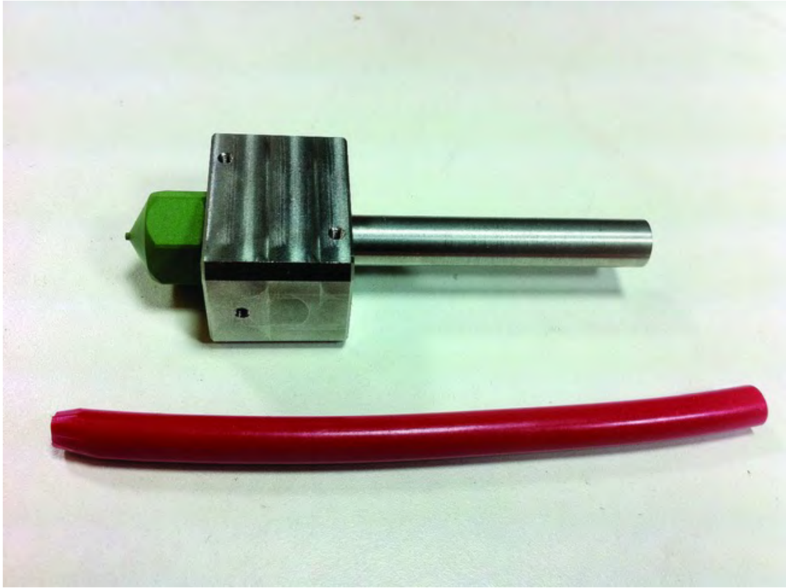
Figure 14-5. Insert the PTFE tube into the feed cylinder.
