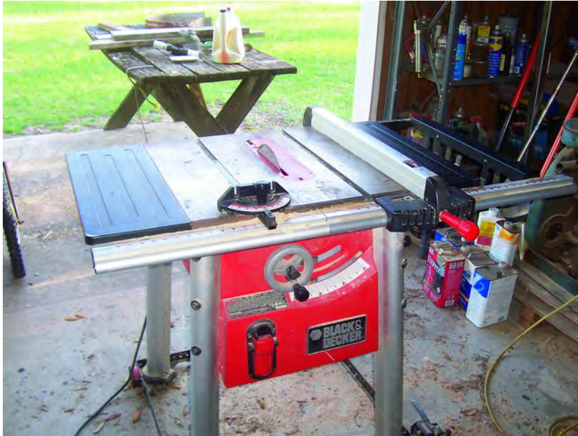
Figure 2-1. A table saw will make the accurate cuts needed for the 3DP.
