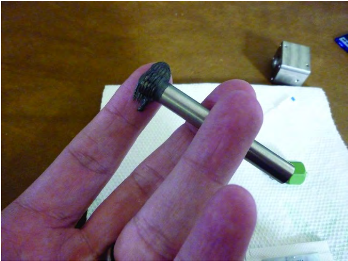
Figure 14-2. Coat the threads with a liberal amount of anti-seize grease.
