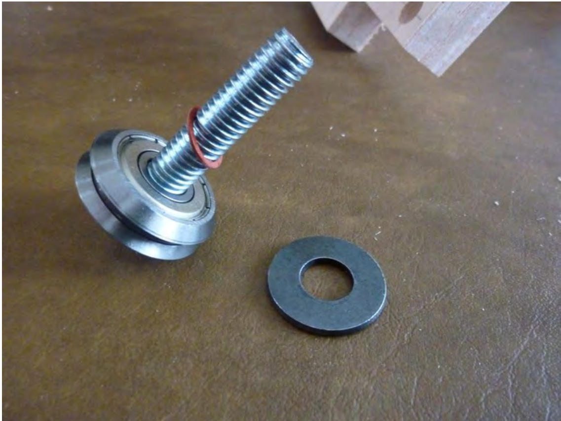
Figure 10-12. Place a V-groove bearing followed by a small red washer on to the bolt.
