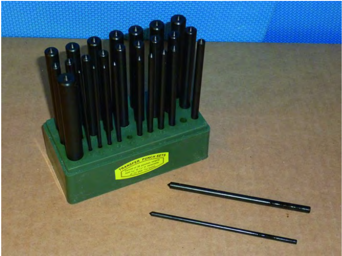
Figure 2-17. A transfer punch is helpful for marking centerpoints of drill holes.
