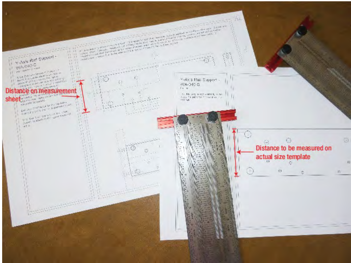
Figure 3-3. Use a ruler to compare measurements to the full-size template sheet.
