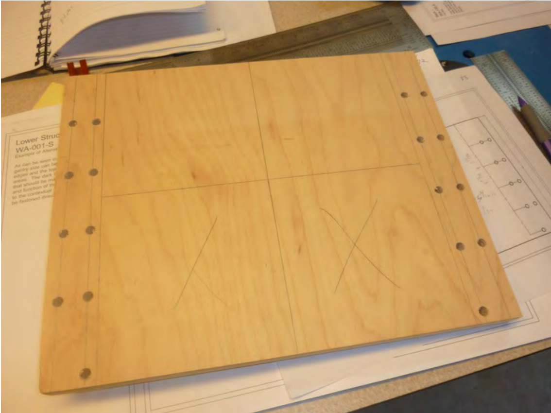
Figure 7-12. Part O with holes drilled and sections marked for removal
