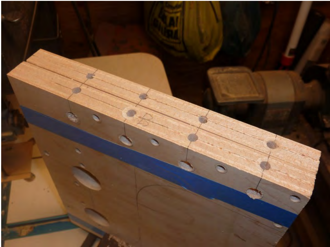
Figure 7-21. Holes drilled through the edges of Parts A and B for the barrel nuts
