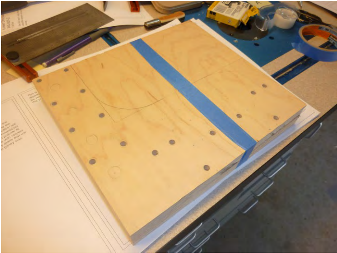
Figure 7-18. Parts A and B with all 1/4" holes drilled
