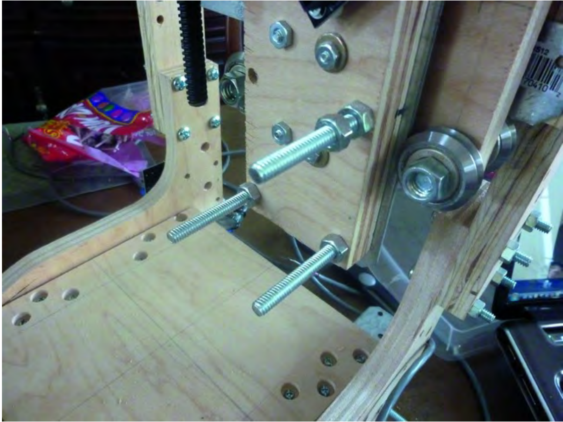
Figure 21-14. You will need three 3" machine screws to attach the Extruder Mechanism.
