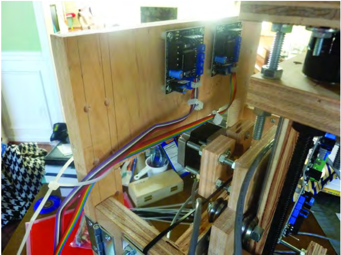
Figure 17-10. Use a plastic tie to pull the ribbons to the side, away from the motor.
