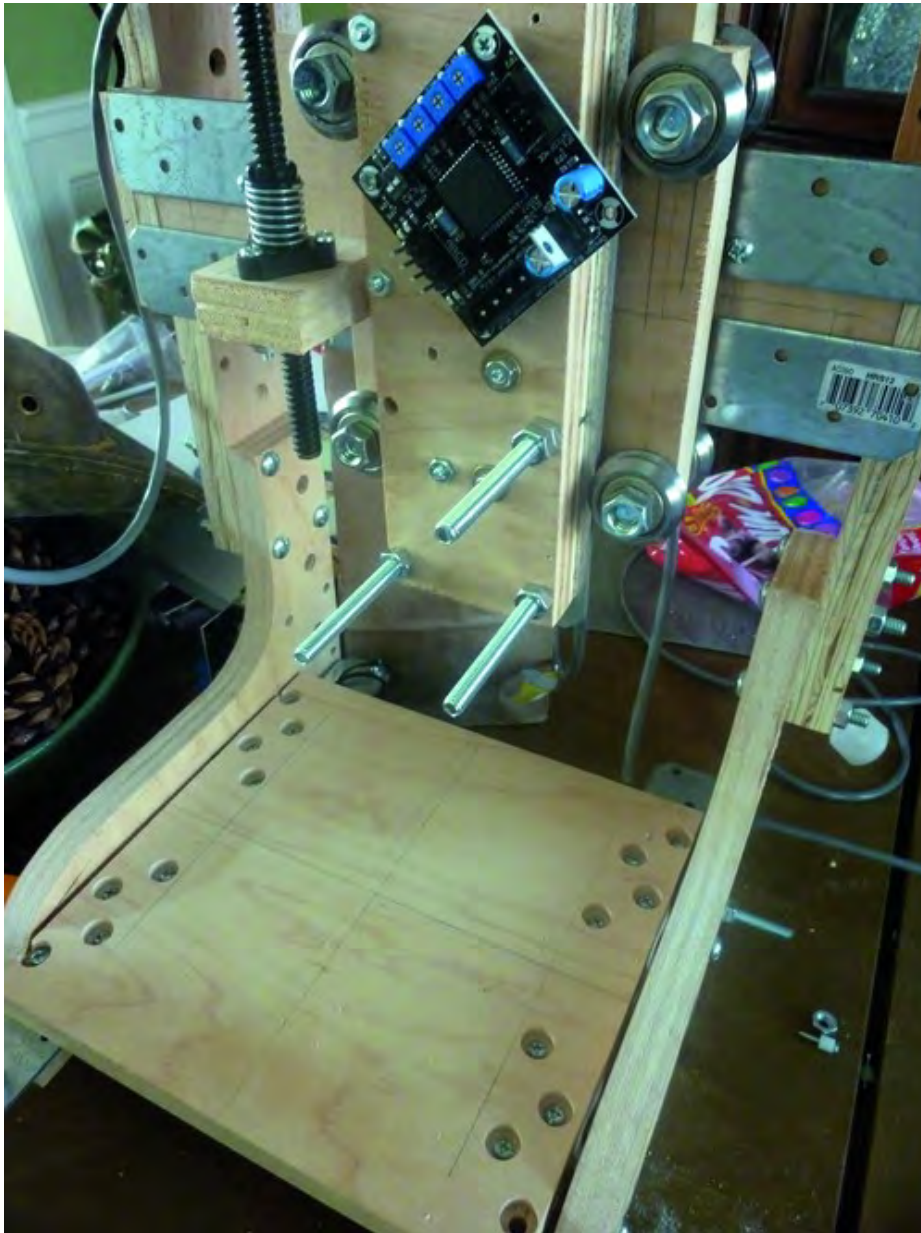
Figure 21-15. Three longer machine screws plus nuts will hold Extruder Mechanism.
