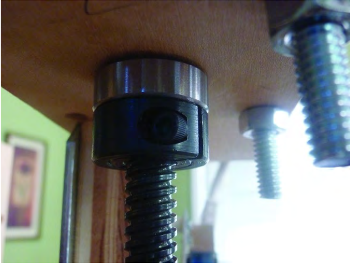
Figure 12-7. Tighten the bearing and collar against Part N.
