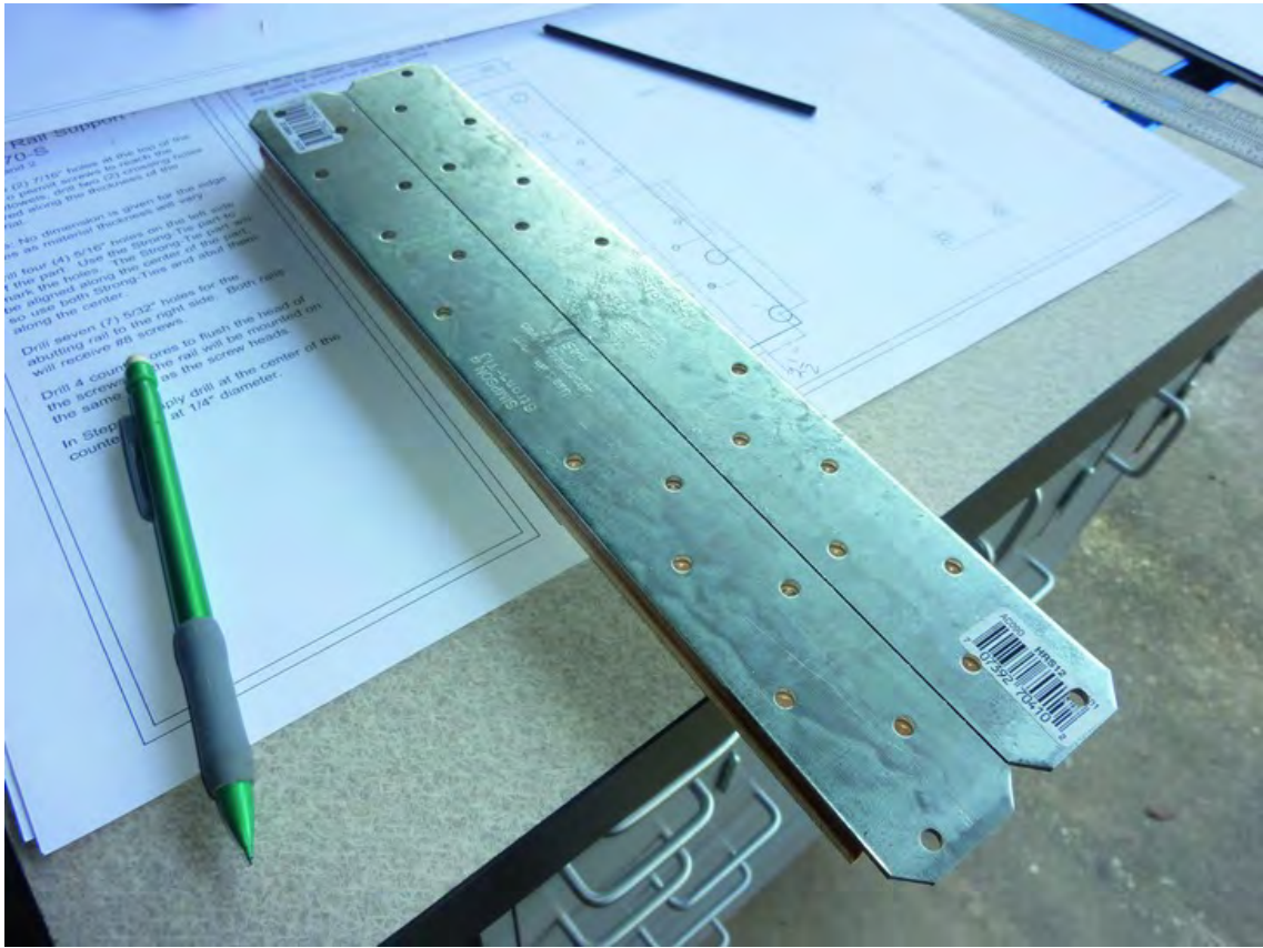
Figure 9-17. Proper placement of the two Strong-Tie brackets on Part K.
