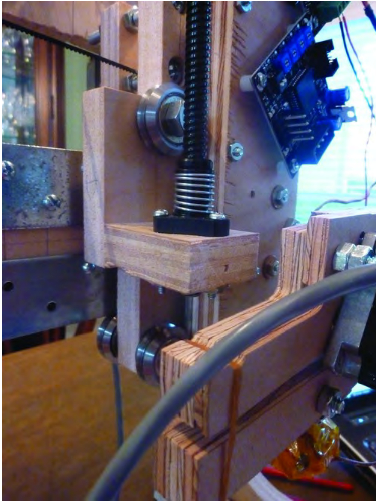
Figure 17-15. Raise the Z-axis until the lead screw is almost flush with Part N.
