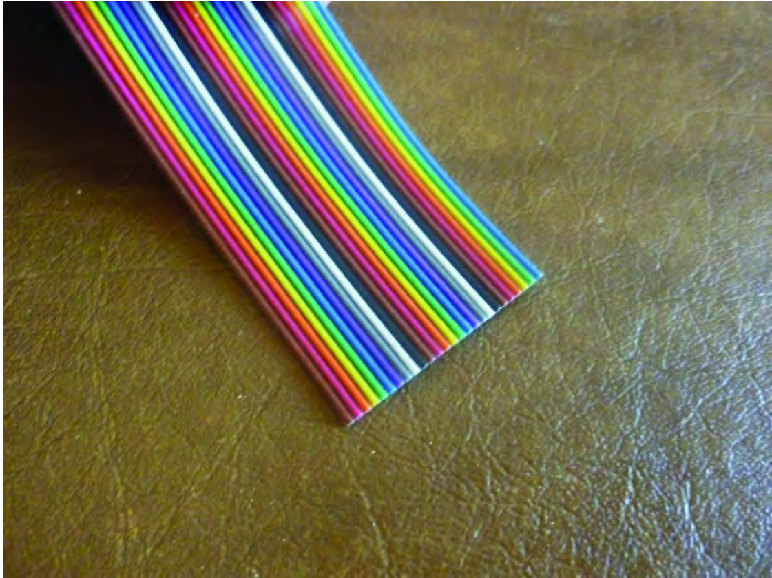
Figure 17-1. A multi-colored ribbon cable is useful for wiring the stepper motor drivers.
