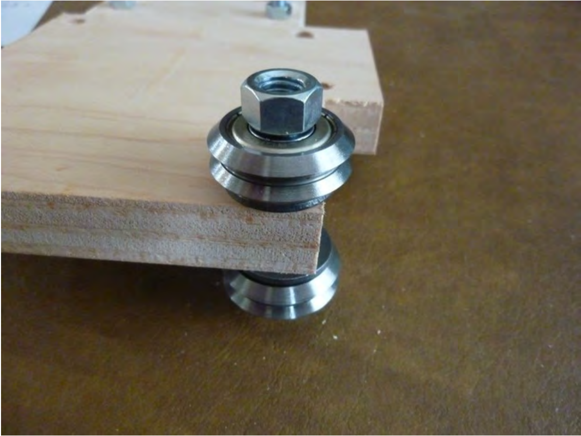
Figure 10-15. A completed V-groove assembly
