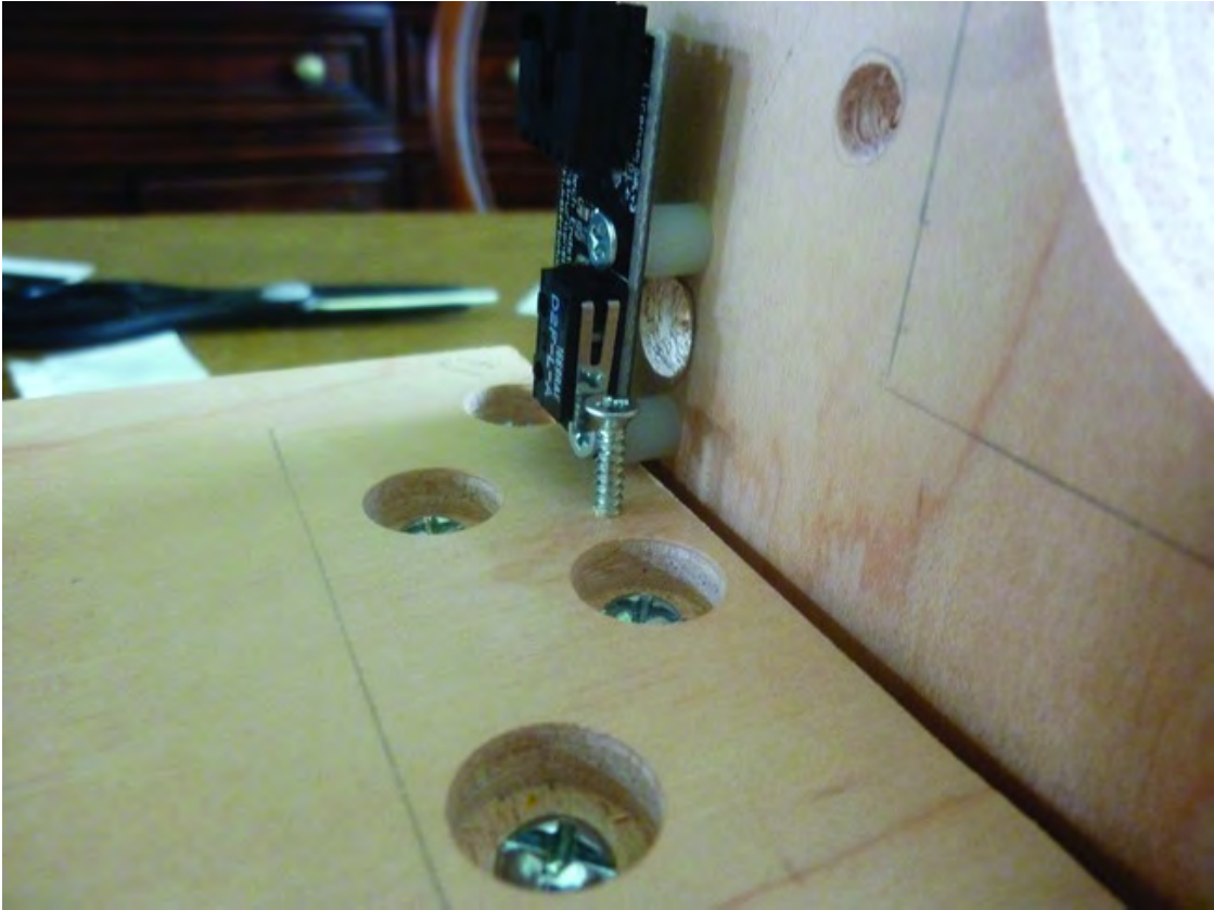
Figure 18-24. Add a wood screw to trigger the table's endstop pushbutton.
