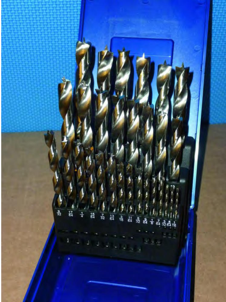
Figure 2-16. Brad point bits provide better results than spade and twisted drill bits.
