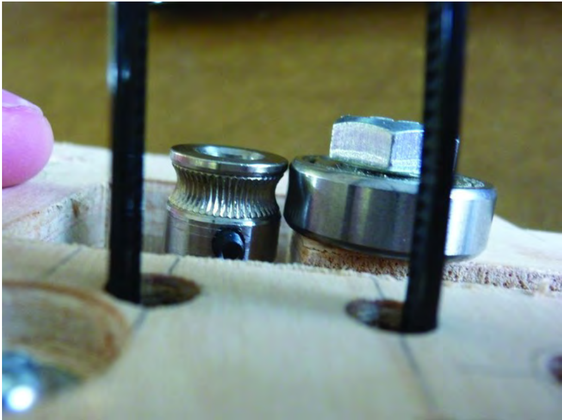
Figure 15-9. Attached the serrated collar and line it up with the bearing.
