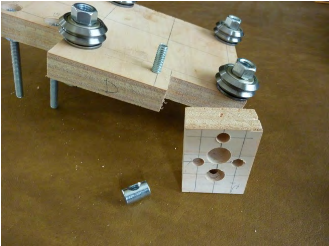
Figure 10-17. Part N will be bolted to Part D with a single bolt and barrel nut.
