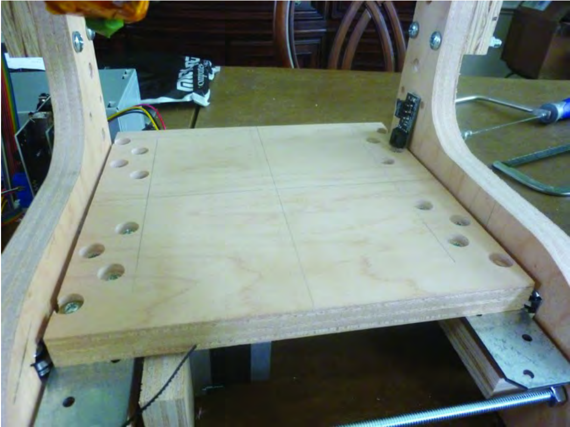
Figure 18-23. The table's endstop is mounted at the rear and to the right.
