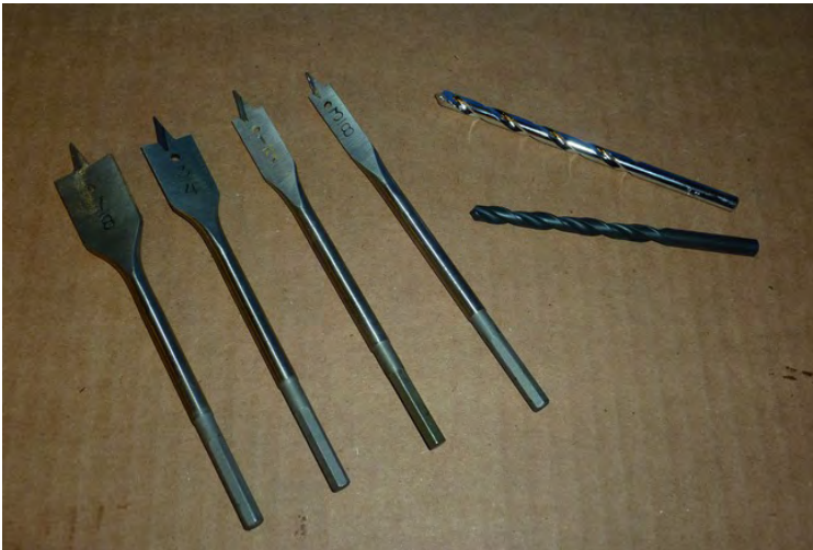
Figure 2-15. Spade drill bits (on left) and twisted bits (on right) will work for drilling straight-through and counterbore holes.
