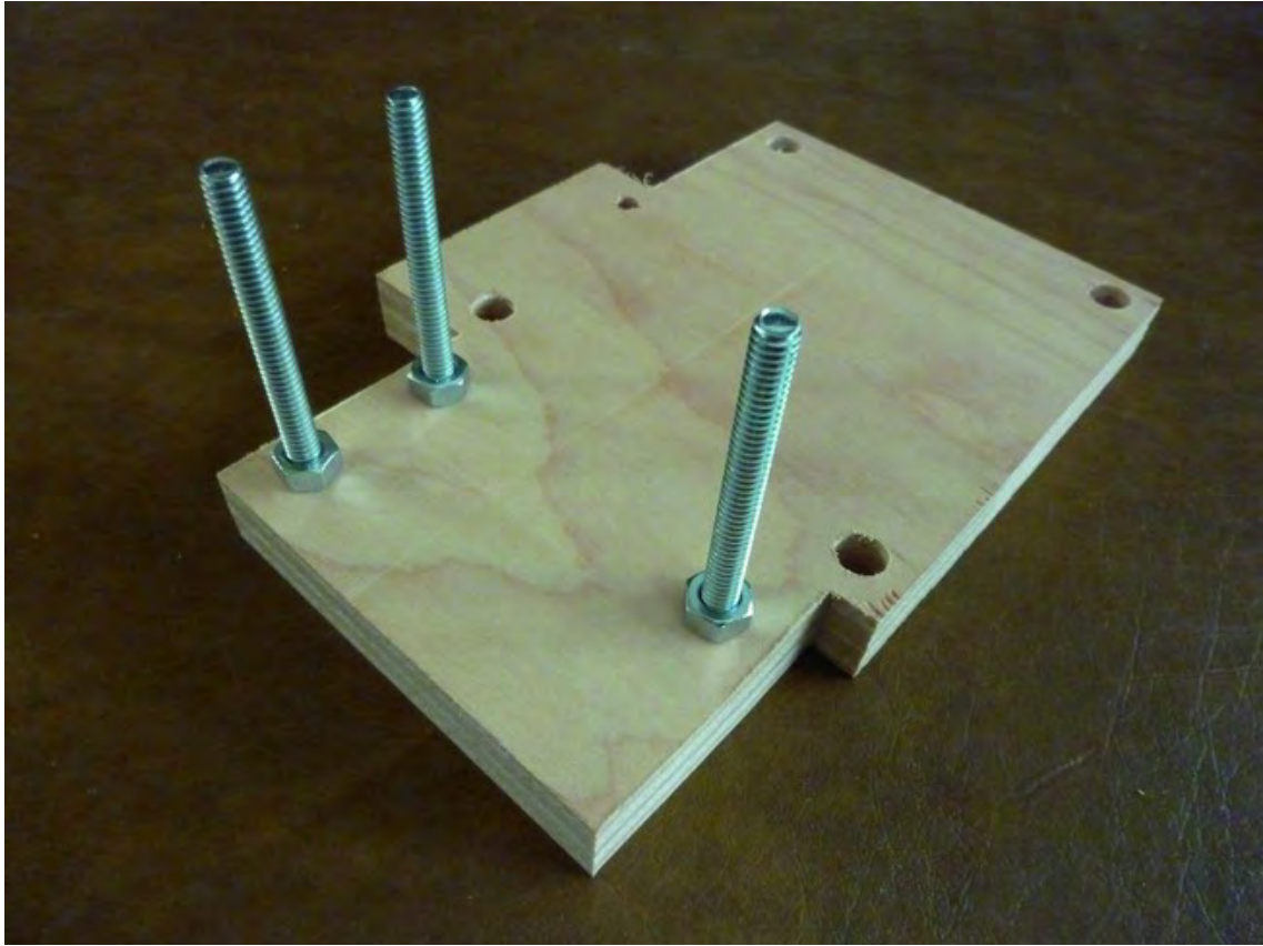
Figure 10-10. Part L with three bolts inserted
