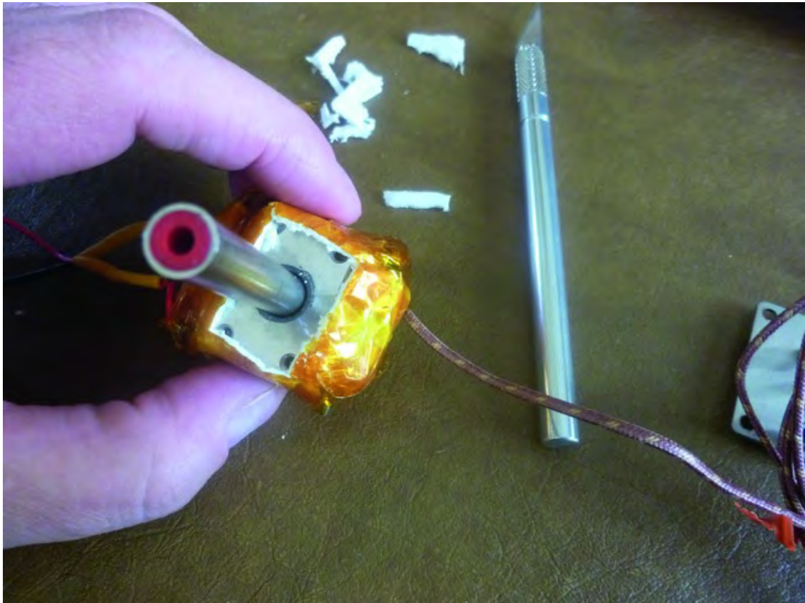
Figure 21-3. Cut away a small portion of tape to expose screw holes.
