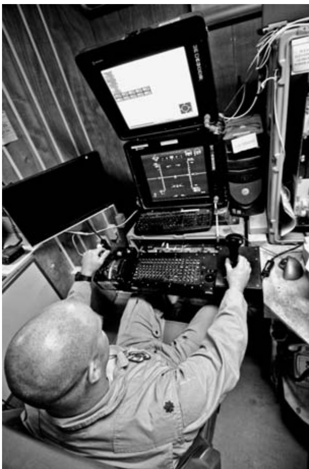
8.3 Predator on patrol, 2010: Maj. Rick Wageman operates the virtual cockpit of an MQ-1 Predator at a base in southern Afghanistan. Public domain photo by Sgt. Samuel Morse. Source: http://www.af.mil/photos/media_search.asp?q=predator . Provided as a public service by the U.S. Air Force.
