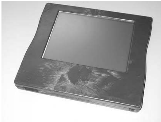
FIGURE 1.9 Infopad: UC Berkeley’s exploration of a mobile ubiquitous computing architecture. (Courtesy of Computer Science Department, University of California Berkeley.)
