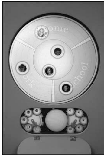
FIGURE 5.2 Whereabouts Clock interface with three specified regions representing work, home, and school, and middle region for locations other than these.
