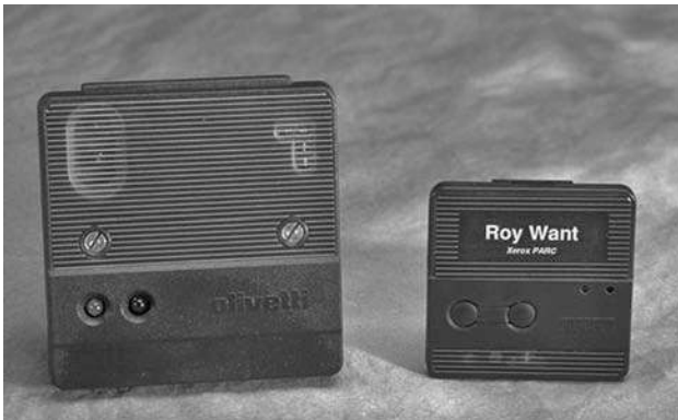
FIGURE 1.13 (a) Active Badge Sensor basestation; (b) an Active Badge. (Photo courtesy of PARC, Inc., http://www.parc.com )
