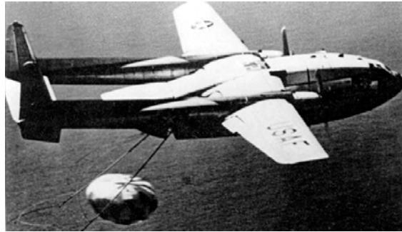
Figure 17. A C-119 snares a parachute-borne CORONA film return capsule in mid-air over the Pacific Ocean Credit: National Reconnaissance Office
