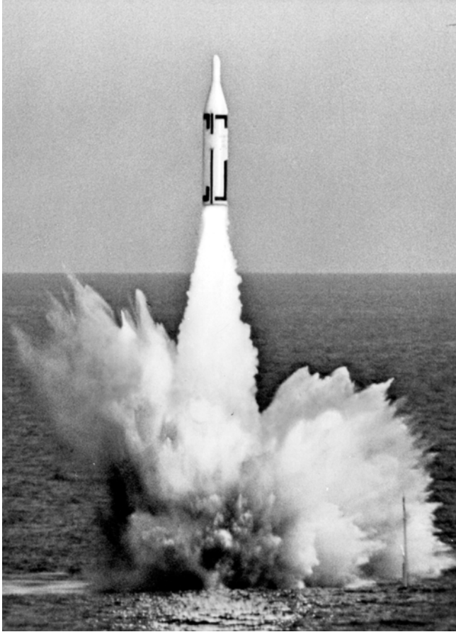
Figure 35. A Polaris submarine-launched ballistic missile (SLBM) breaks the surface having been launched underwater.
