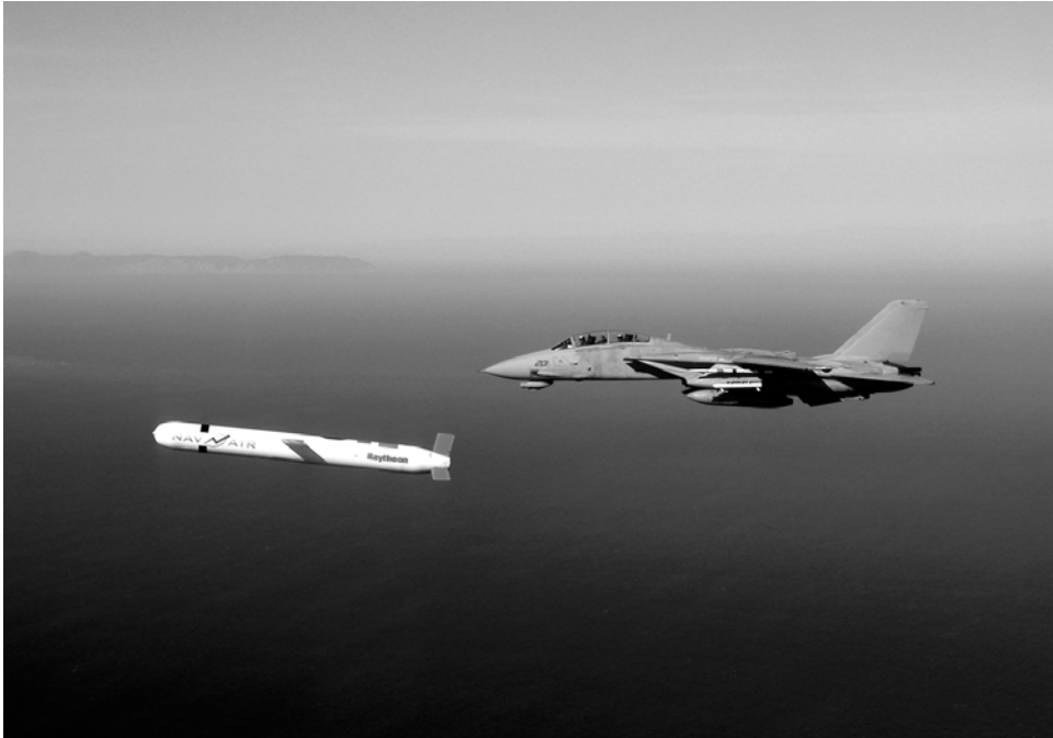
Figure 38. A Tomahawk Block IV ship- and submarine-launched cruise missile is trailed by a Navy F-14 Tomcat during a test flight. Credit: US Navy.
