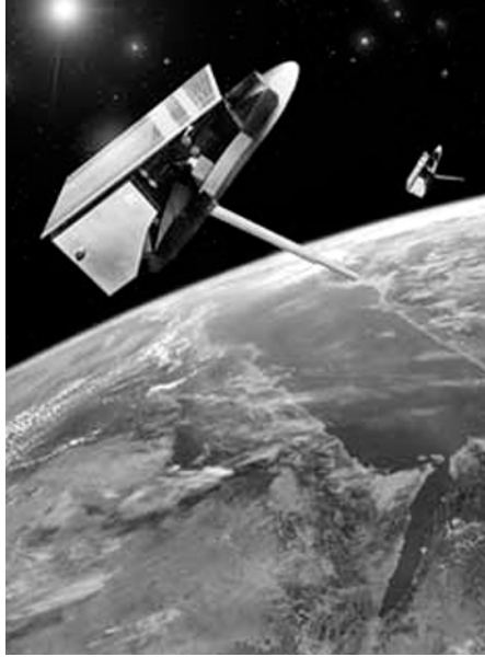
Figure 47. The small, low-cost SAR-Lupe imaging radar satellite is Germany's first military surveillance satellite system; the first of a five-satellite constellation was launched on December 19th 2006. Credit: OHB.
