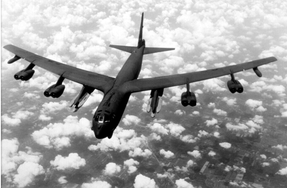
Figure 48. A B52 carrying cruise missiles on its under-wing pylons.
