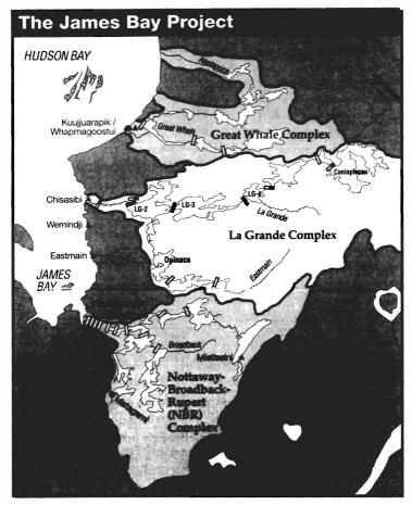
concept of diverting the Nottaway and Rupert Rivers into the Broadback through construction of at least eleven major dams. No predictions were offered as to how much territory would be flooded in this, but construction costs were projected at \$44 billion (U.S.).<sup>61</sup> Together, the three complexes which would be in place when James Bay II was complete would effect a "replumbing" of virtually all of northern Québec (see Map I).
