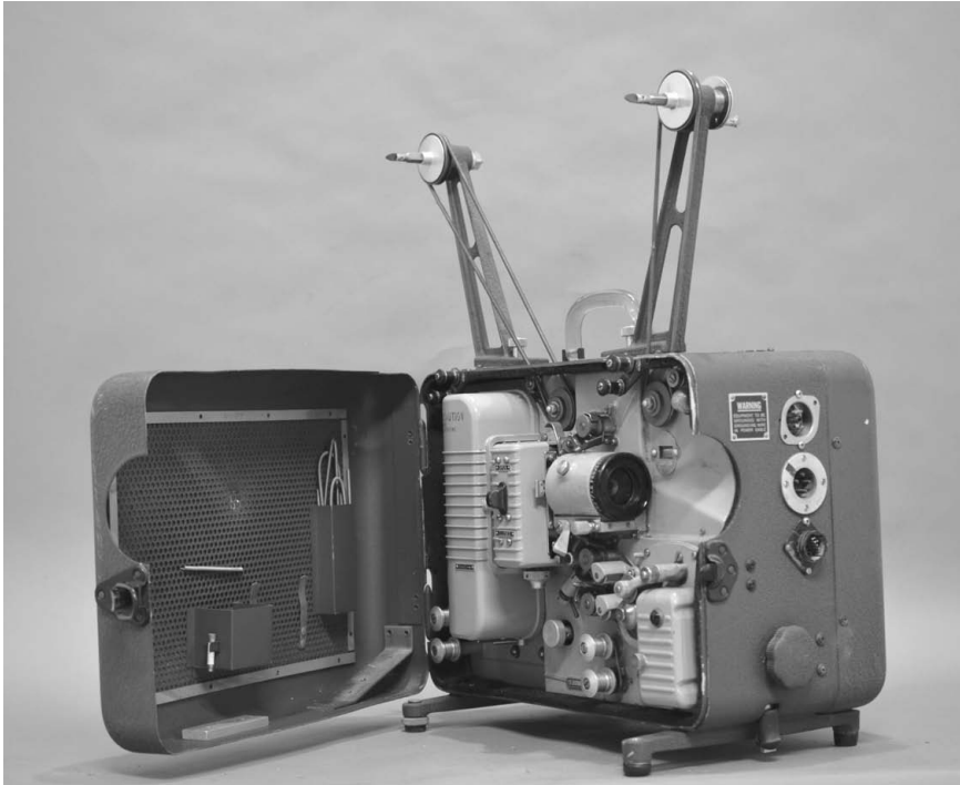
FIGURE 2.1. With its elaborate metal casings and recessed lamp, the JAN projector was designed to be rugged and reliable in everyday and extreme performance scenarios. Its handle signaled the device's portability: the JAN was designed to be carried by a single soldier. (Photo by Haidee Wasson; JAN from the Herbert E. Farmer Motion Picture Technology Collection at the University of California Hugh M. Hefner Moving Image Archive.)
