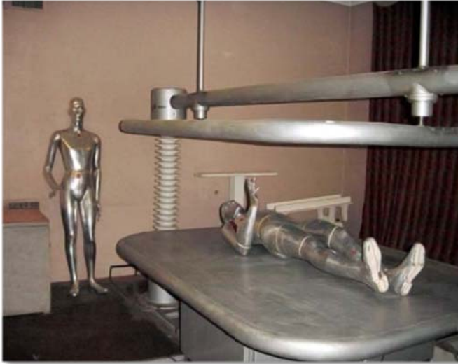
Figure 2. Experimental stand to study the EMF biological effects in the Occupational Medicine Institute of the Russian Academy of Medical Sciences.
