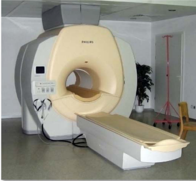
Figure 4. Typical MRI scanner. The bed lifts a human, and then the slider moves the body through the magnet.
