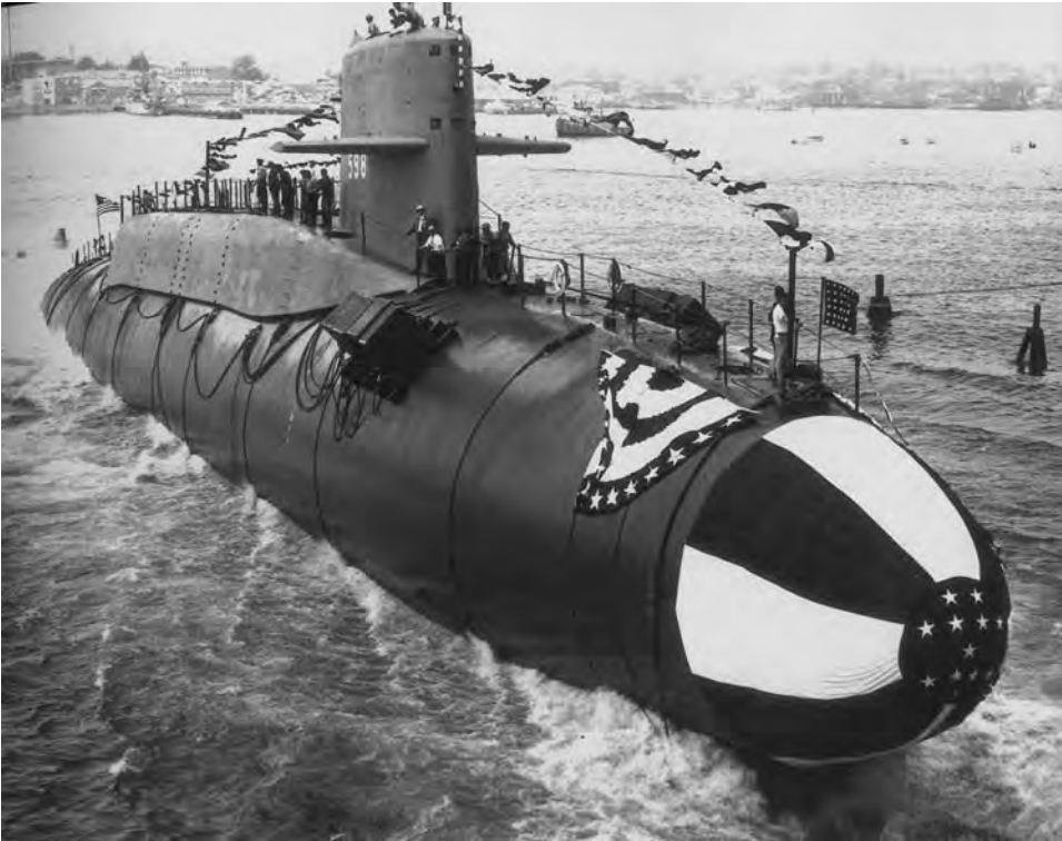
The USS George Washington , the first nuclear powered submarine designed to launch Polaris ballistic missiles while submerged, takes to the water at Groton, Connecticut, in June 1959. George Washington was built quickly by cutting an attack submarine in half and adding a missile compartment. (United States Naval Institute)
