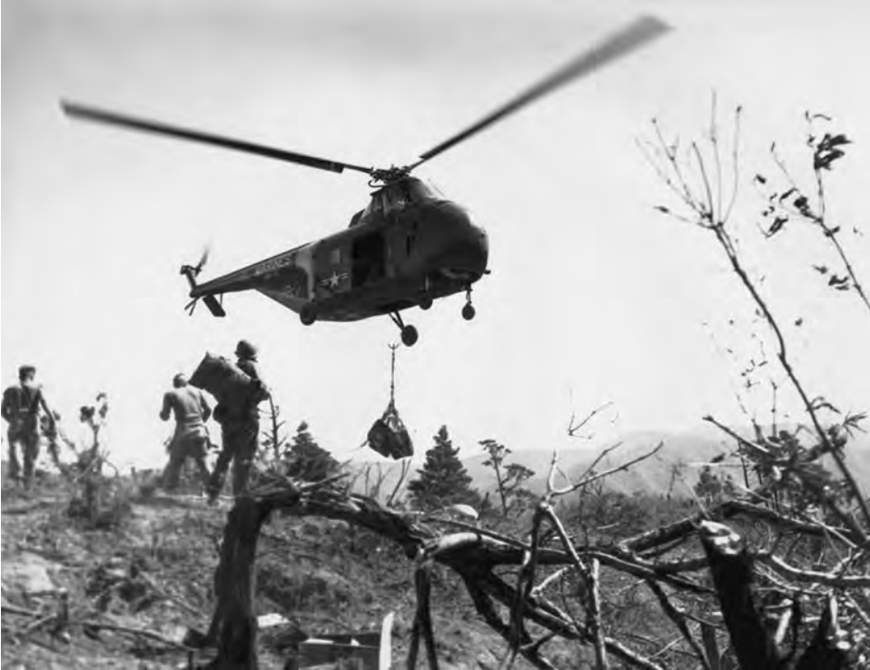
A U.S. Marine Sikorsky HRS-2 Chickasaw delivers supplies to a forward position. United Nations forces, mainly those of the United States, employed several types of helicopters in the Korean War. These rotary wing aircraft rescued downed airmen and rapidly ferried critically wounded soldiers to field hospitals. (National Archives)
