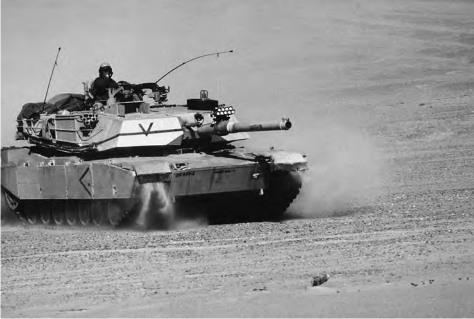
The M-1 and M-1A1 Abrams are the main battle tanks for the U.S. Army. They are fully tracked, low-profile tanks with shoot-on-the-move capability and a high degree of maneuverability. (Department of Defense)
