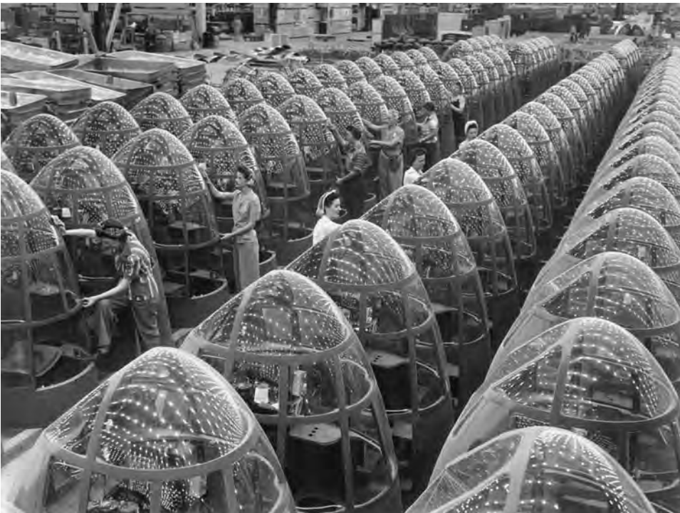
Women working in Douglas Aircraft's Long Beach, California, assembly plant during World War II complete final inspection of nose cones for A-20 attack bombers. (National Archives)
