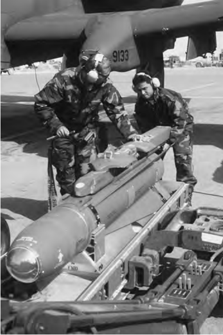
Munitions specialists from the 23rd Tactical Fighter Wing load an AGM-65 Maverick air-to-surface missile onto an A-10A Thunderbolt II prior to a sortie in support of Operation Desert Storm. (Department of Defense)
