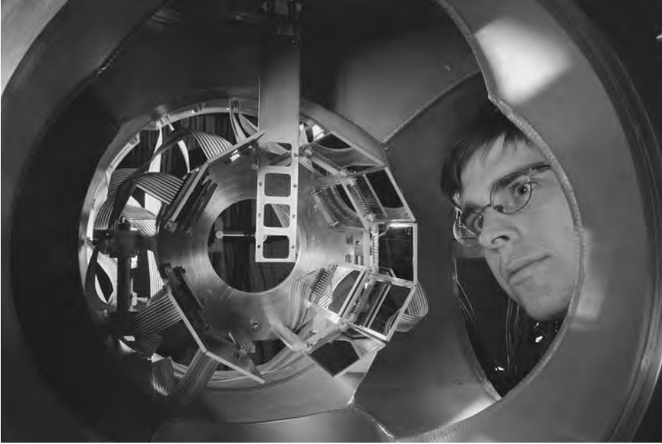
Conducting a visual inspection of the Oak Ridge Rutgers University Barrel Array, a high-resolution instrument with specialized particle detectors arranged in a barrel shape around a target. The instrument is housed at the Holifield Radioactive Ion Beam Facility at Oak Ridge National Laboratory. (Department of Energy)
