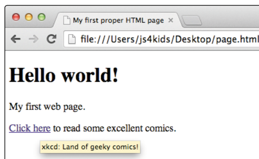
Figure 5-11: A web page containing a link to http://xkcd.com/ with a title attribute
