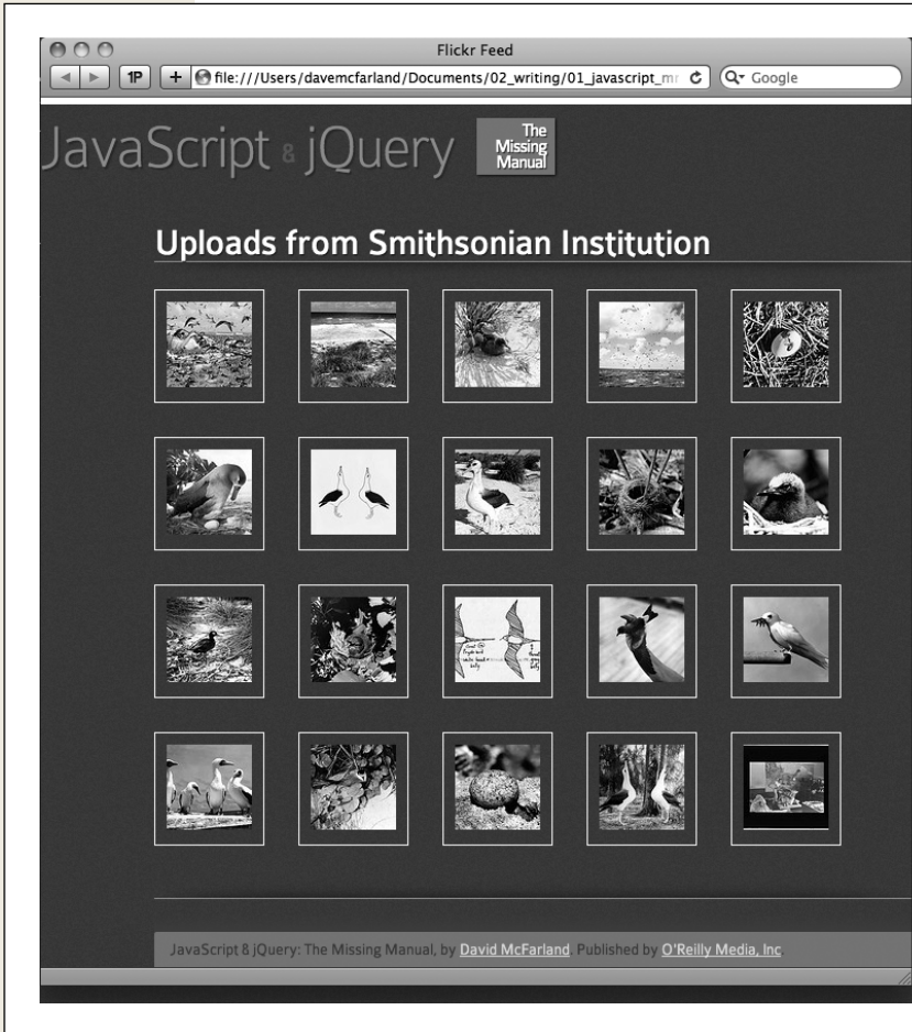
Figure 12-1: While AJAX is restricted to the requesting information from the same domain, a workaround called JSONP lets you retrieve JSON data from another site by requesting a JavaScript file from that site. This technique lets you access tweets from Twitter, maps from Google, and photos from Flickr (pictured here) and embed them directly in your own web pages.
