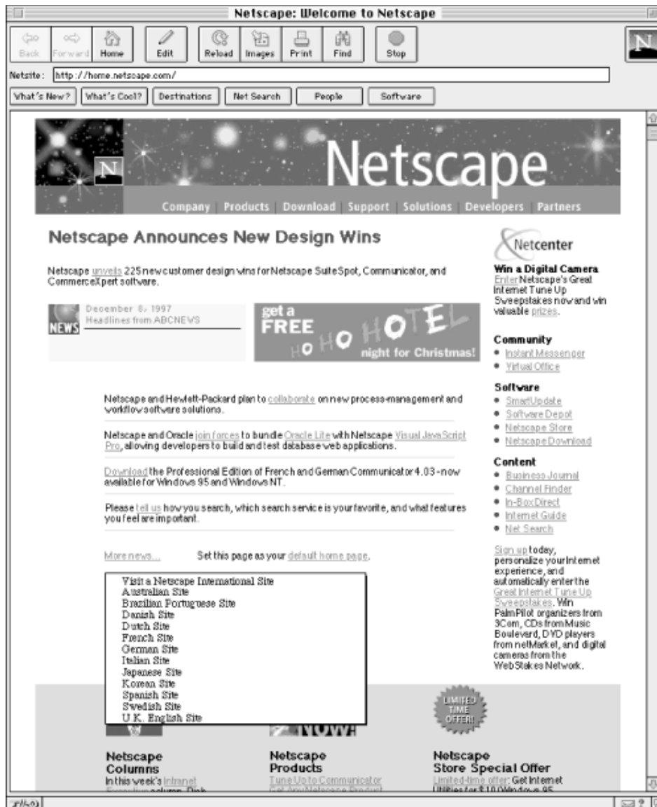
Figure 4.13. This pull-down menu enables users to select a location without first going to a separate web page. This approach avoids further cluttering the main page with a long list of locations.
