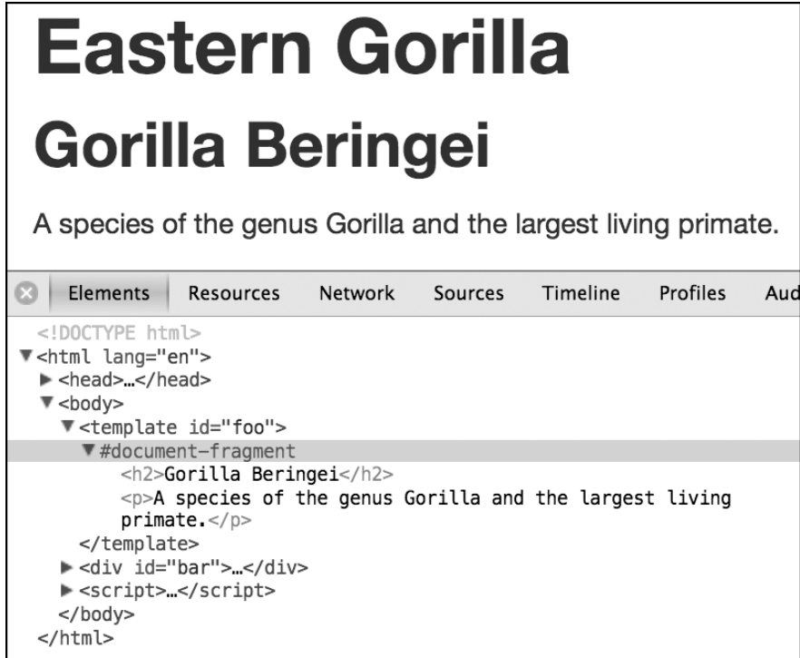
Figure 11-1: The code inspector shows the contents of the template element, which exists outside the regular DOM.
