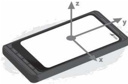
Figure 6-3: Movement along the three-dimensional axes (This image is taken from the Mozilla Developer Network [MDN] article, "Orientation and Motion Data Explained": http://developer.mozilla.org/en-US/docs/DOM/Orientation_and_motion_data_explained/ . It is used under a Creative Commons license.)
