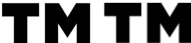
Figure 7-1: Detail from a scaled-up image in SVG (left) and PNG (right); the SVG is noticeably sharper and clearer.
