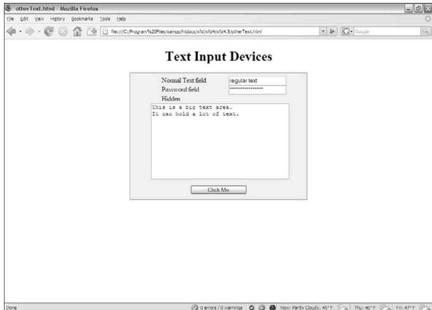
Figure 5-10: Passwords, hidden fields, and text areas all look the same to JavaScript.
