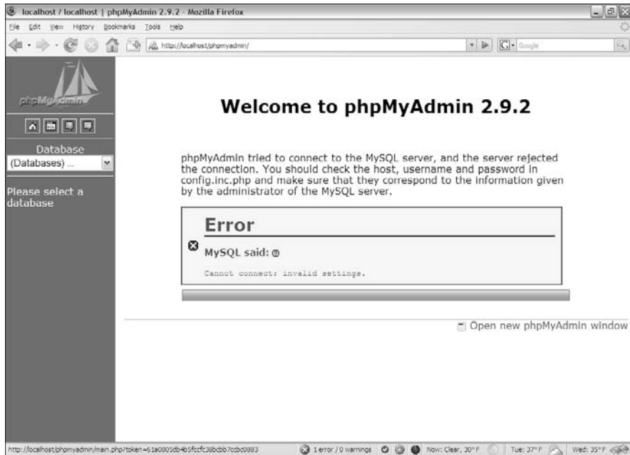
Figure 1-9: That message can't be good. Maybe I should have left it vulnerable.
