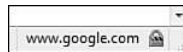
Figure A.3 Web browsers display an icon to indicate the page you are viewing came via an SSL connection.
