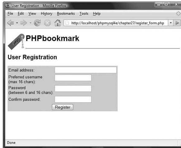
Figure 27.4 The registration form retrieves the details needed for the database. This form requires users to type their passwords twice, in case they make a mistake.
