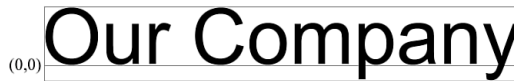
Figure 22.6 Coordinates of the bounding box are given relative to the baseline. The origin of the coordinates is shown here as (0,0).
