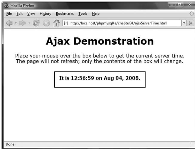
Figure 34.3 The result from the server is displayed in the div called show-time ; mousing over the area again results in another invocation of the script.
