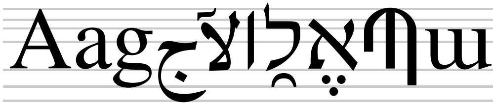
Figure C-7: The relevant heights, with overshoot, of a number of glyphs in various scripts (Latin, Arabic, Hebrew, Armenian). The font is Omega Serif.
