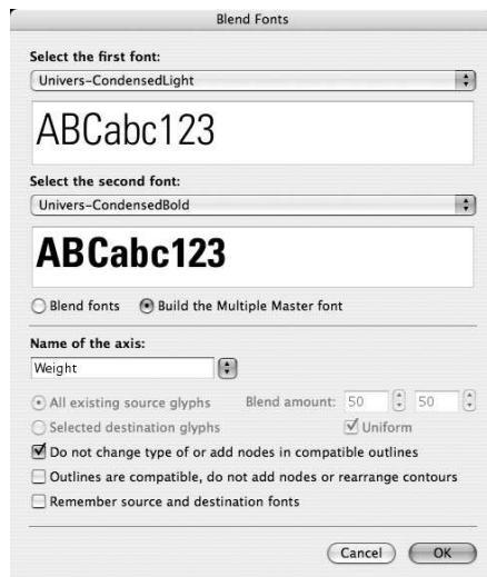
Figure 12-10: The window for creating Multiple Master fonts from two ordinary fonts taken as master designs: the fonts Univers 47 (light condensed) and Univers 67 (bold condensed).
