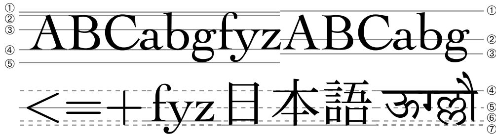
Figure 10-8: Different SVG metric properties, specific to the font-face element. Left: (1) ascent, (2) cap-height, (3) x-height, (4) alphabetical, (5) descent. Right: (1) overline-position, (2) strikethrough-position, (3) underline-position, (4) hanging, (5) mathematical, (6) alphabetical again, (7) ideographic.
