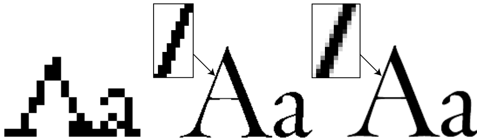
Figure 6-5: The letters ‘Aa’ in Agfa’s splendid font Throhand , at 128 points. From the left: display without ATM; display with ATM but without glyph smoothing; and display with ATM and with glyph smoothing.
