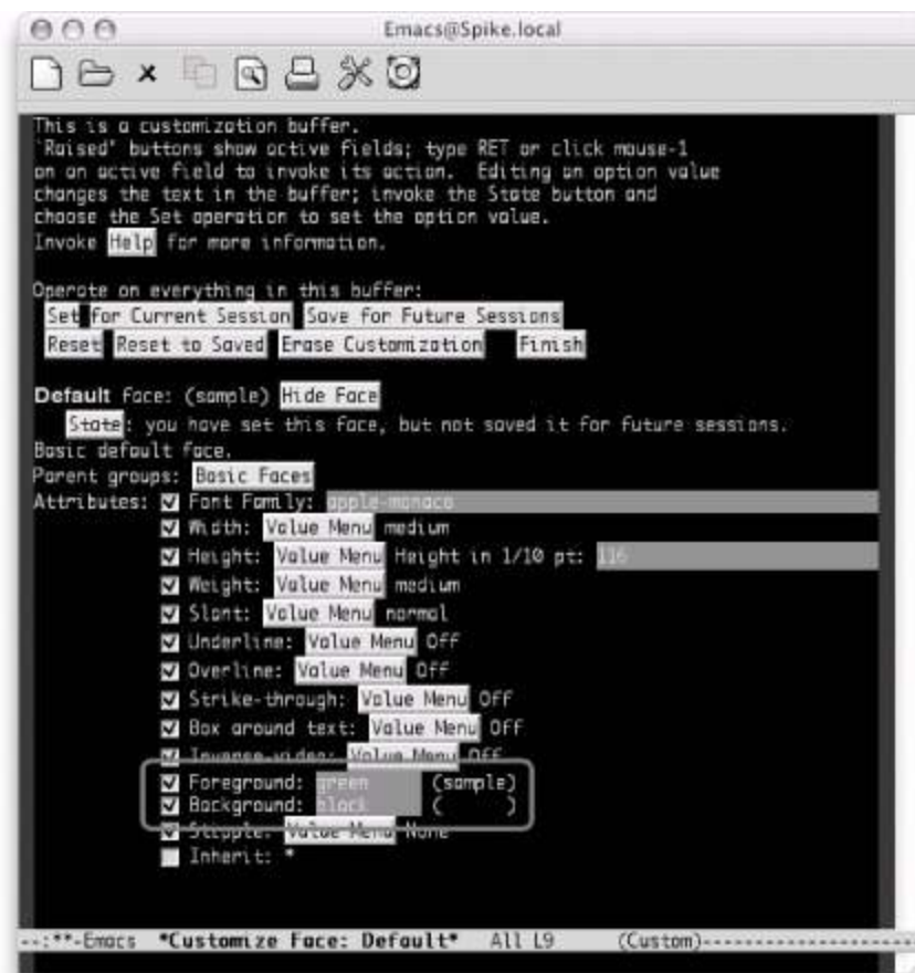
Figure 10-11. Changes to the default font colors effectively set the foreground and background colors for Emacs (Mac OS X)
