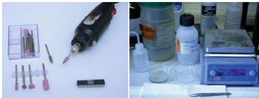
Fig. 7.2 Chip decapsulation tools
