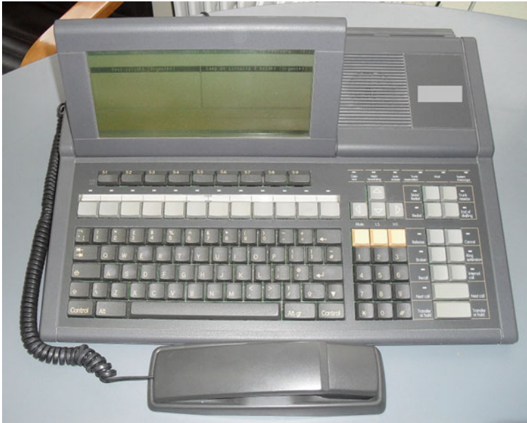
Fig. 3.14 A typical PBX operator's console
