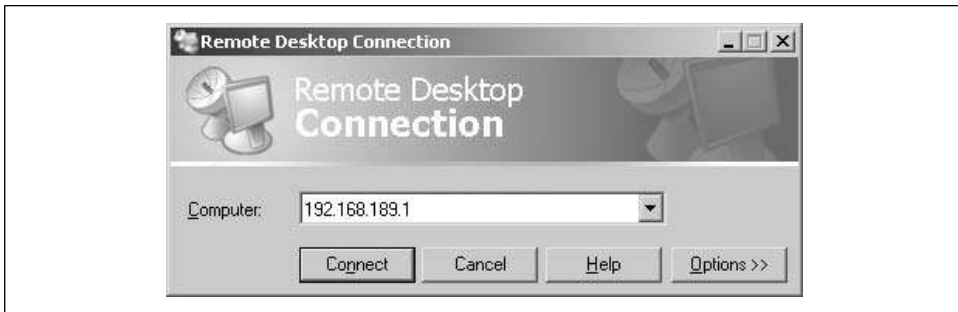
Figure 8-10. Connecting to RDP using the Remote Desktop client
