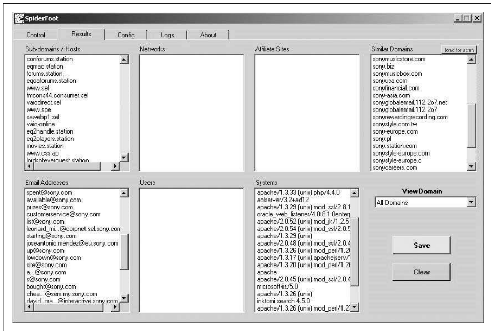
Figure 3-8. Using SpiderFoot to perform host, domain, and user enumeration
