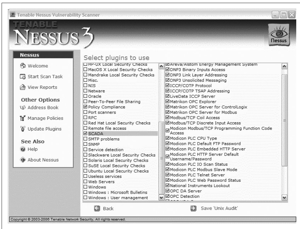
Figure 4-2. Nessus scan options for SCADA systems
