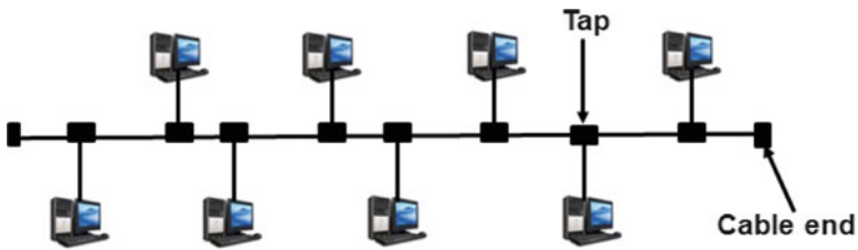
Fig. 2.3 Illustration of bus topology
