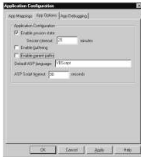
Figure 7.3 Disabling Parent Paths Prevents an Attacker from Using “../” Directory Notation to Gain Access to Files Not in Your Web Root
