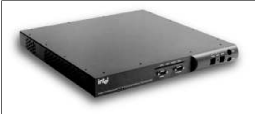
Figure 14.13 External View of the Intel NetStructure 7110 e-Commerce Accelerator
