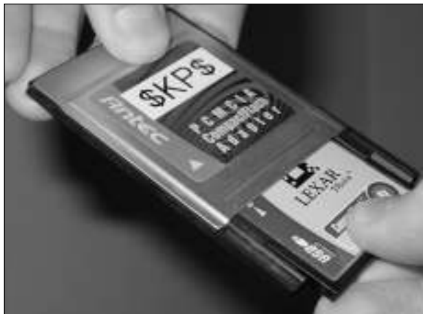
Figure 14.14 Placing the CompactFlash Card into a PCMCIA CompactFlash Adapter
