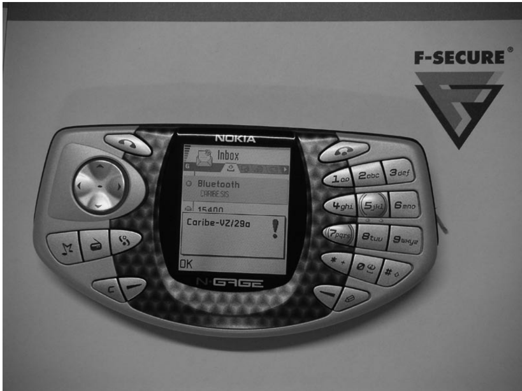
Figure 2.6 This Variant of Cabir Gives Credit to the 29A Group That Disclosed Source Code for the Virus in an E-zine
