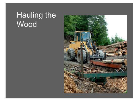
At the back of the sawmill is a large ramp made of steel I-beams with a series of toothed, geared wheels that move the logs into the building. The logs come in on trucks (big packets!) with about 50-60 logs apiece and are unloaded onto the ramp with the skid-loader.
