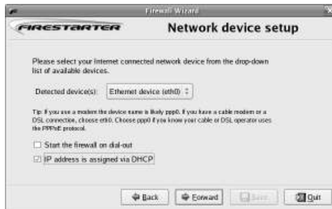
Figure 9.14 Firestarter Network Device Setup
