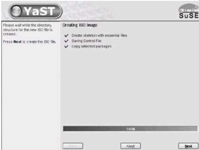
Figure 5-8: SUSE Autoyast ready to create the ISO image
