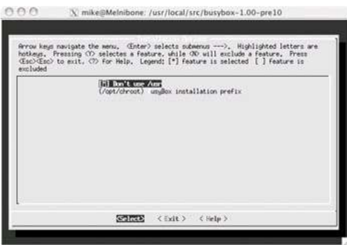
Figure 9-2: Set the BusyBox installation target to the chroot environment.
