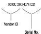
Figure 3-3: The anatomy of a MAC address
