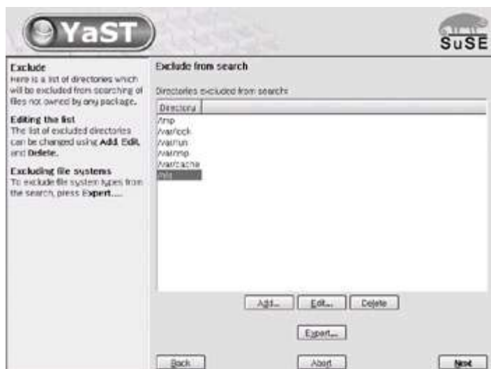
Figure 5-11: YaST2 backup showing exclusion of the /nfs mounted resources
