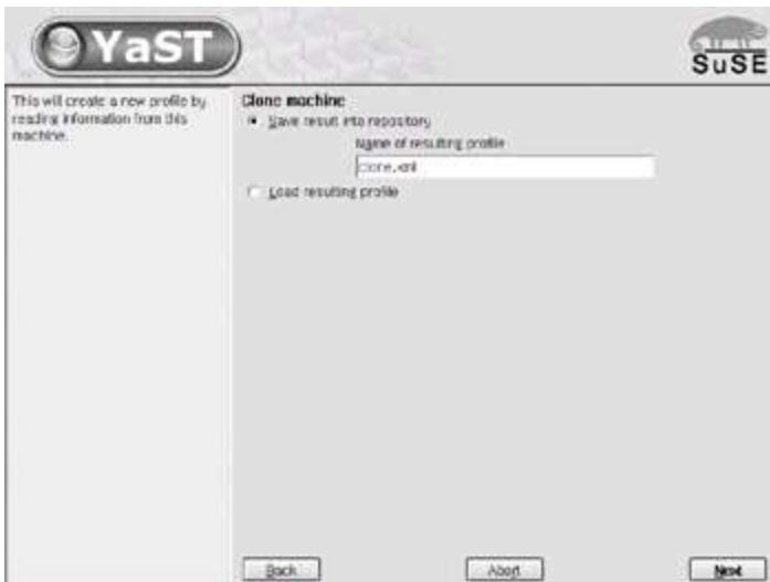
Figure 5-4: SUSE Autoyast showing entry of the filename clone.xml
