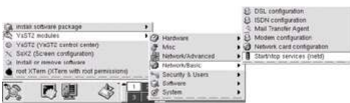
Figure 2-3: YaST2 menu hierarchy for invoking inetd services GUI
