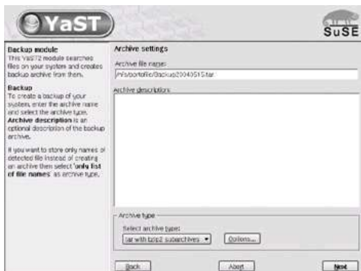
Figure 5-10: YaST2 backup showing selection of backup archive location and type
