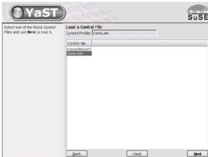
Figure 5-6: SUSE Autoyast selection of the clone.xml profile
