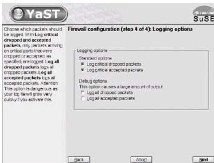
Figure 3-9: SUSE Linux Firewall Configuration (Step 4 of 4): Logging Options
