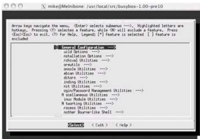
Figure 9-1: The make menuconfig step for BusyBox
