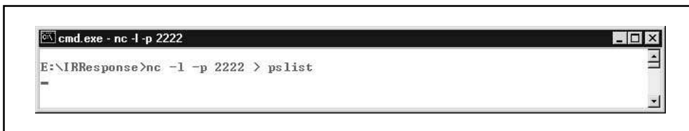
Figure 5-3. Setting up the netcat listener on the forensic workstation
