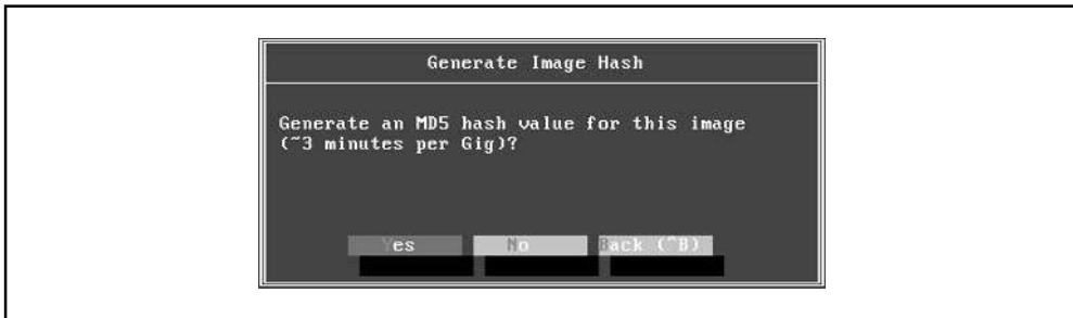
Figure 7-13. EnCase's option to perform MD5 hashing
