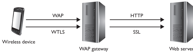
Figure 7-59 A WAP gateway is required to translate WAP protocols to Internet protocols.
