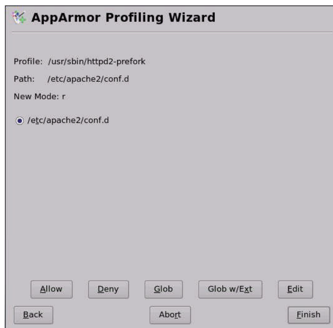
Figure 1: The Learning Mode exception requires you to allow or deny access to a specific resource.
