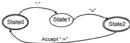
Figure 13-46. A finite state automaton that recognizes the assignment operator “:=” from its two characters colon and equal sign.
