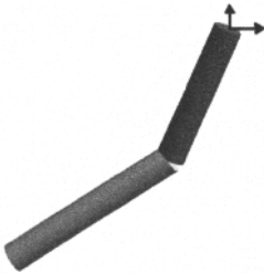
Figure 15-76. A 3D visualization from a 3D animation of the double pendulum with cylindrical geometries of the bodies. The inertial system frame (world object) is shown at the top.
