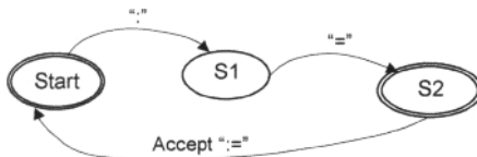
Figure 13-40. A finite state automaton that recognizes the assignment operator “:=” from its two characters colon and equal sign.
