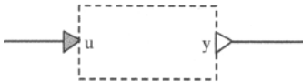
Figure 5-24. A MISO block with an input signal type RealInput and an output signal RealOutput .
