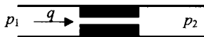
Figure 14-7. Nonlinear flow resistance from turbulent flow caused by a sudden change of the area of the tube, e.g. an orifice, a bend, or a valve.
