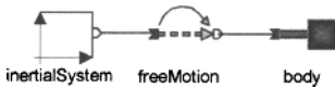
Figure 15-66. Connection diagram for the free-flying body model using the old Modelica 2.2 Modelica.Additions MBS library.
