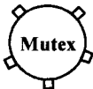
Figure 13-97. Class Mutex for mutual exclusion of a common resource, here configured with 5 mutex ports of type MutexPortIn .
