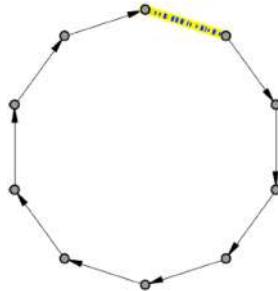
Figure 2.3. The road is a closed circuit composed of one-way edges of single-lane traffic. At initialization, the vehicles all start on the same edge
