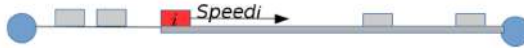
Figure 2.7. The Underwood-Forward model allows all vehicles to travel at the speed limit when they are alone, but forces them to reduce their speed as a function of the number of vehicles present in front of them on the edge, as well as the capacity of this part of the edge
