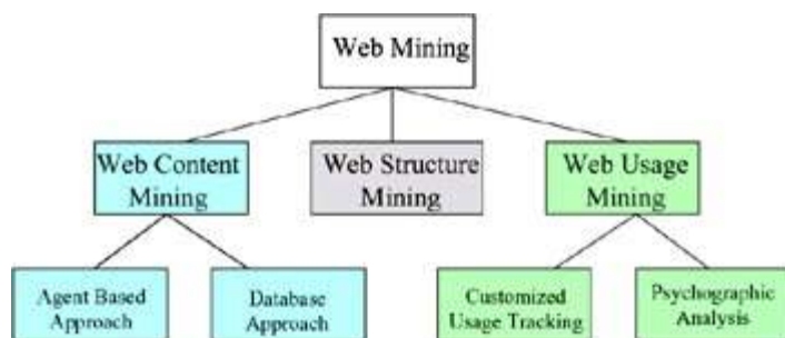
Figure 1: Taxonomy of Web Data Mining (Adapted from Pyle, 1999, and Srivastava et al., 2000)
