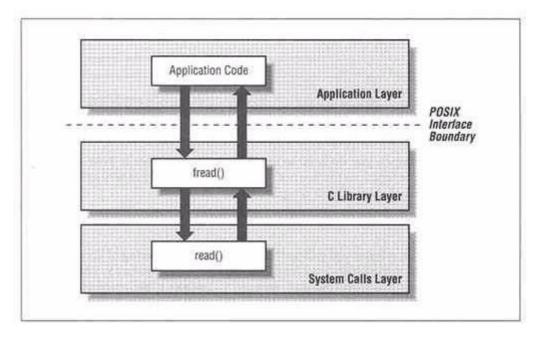
Figure 5-1. Traditional UNIX software layers
