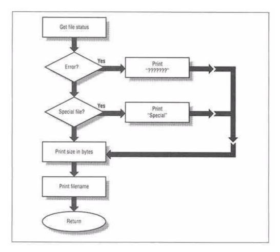
Figure 2-2. Flowchart for print\_dir\_entry()
