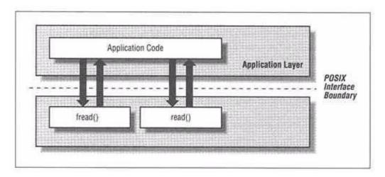
Figure 5-2. Possible POSIX software layers
